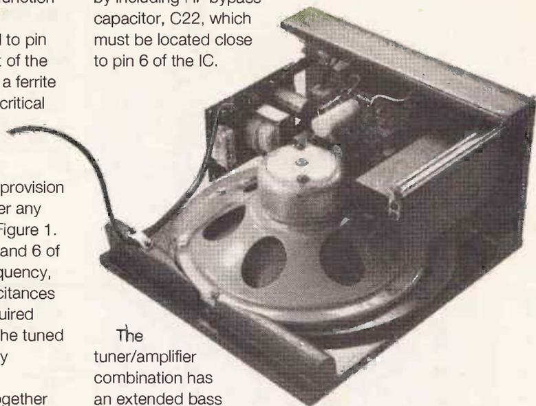
The tuner/amplifier combination has an extended bass response and constructors who wish to try a large speaker in a cabinet of suitable size will find that the value of output coupling capacitor, C27, is big enough to fully exploit this. It can be reduced to 470µF, without any audible drop in bass response, when a 130 or 150mm speaker is fitted in a small cabinet.
