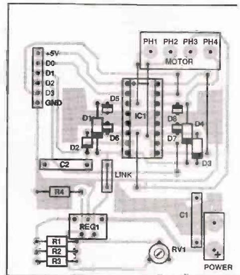
Figure 9: PCB component overlay
