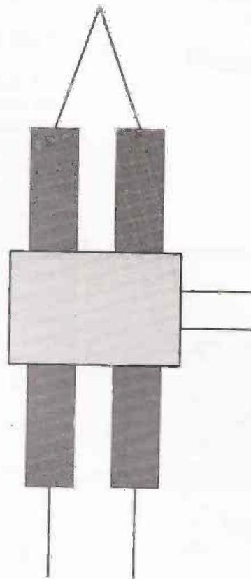
Figure 9a: Plan view of Fluxgate Magnetometer, showing sense winding arrangement
