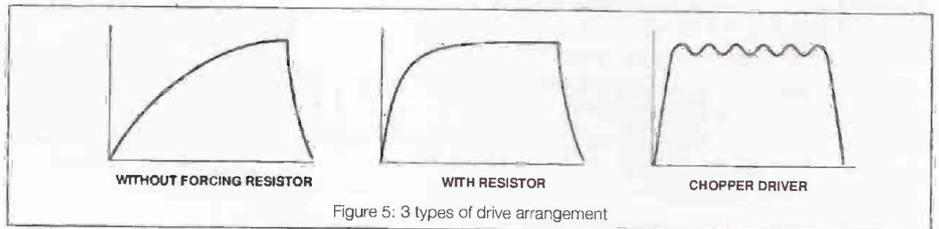
Figure 5: 3 types of drive arrangement
