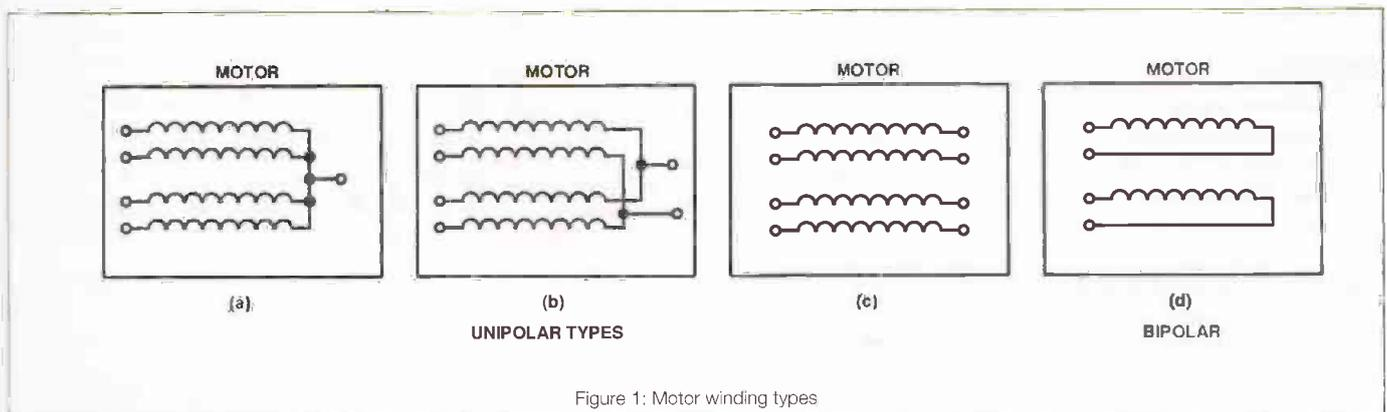
Figure 1: Motor winding types
