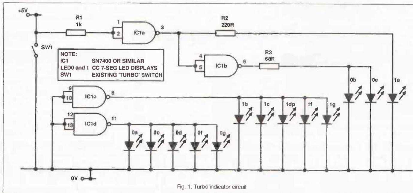
Fig. 1. Turbo indicator circuit
