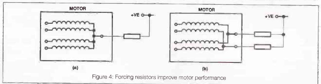
Figure 4: Forcing resistors improve motor performance
