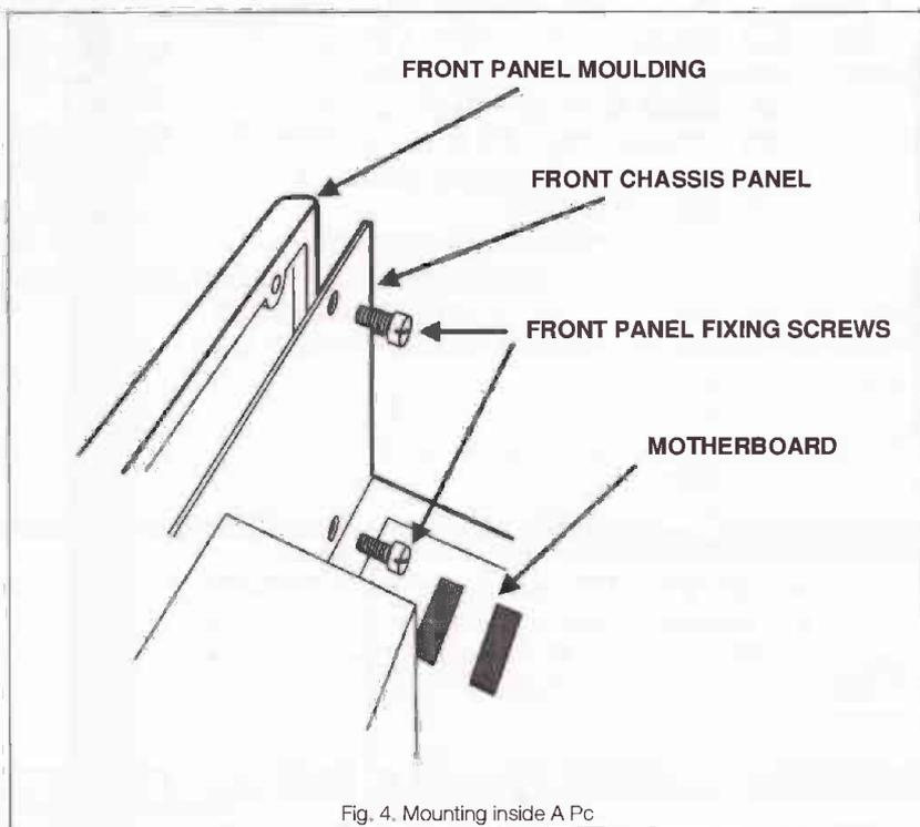
Fig. 4. Mounting inside a PC
