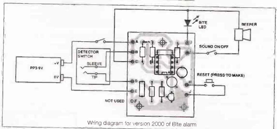
Wiring diagram for version 2000 of Bite alarm
