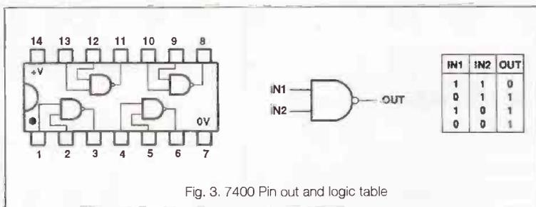
Fig. 3. 7400 Pin out and logic table
