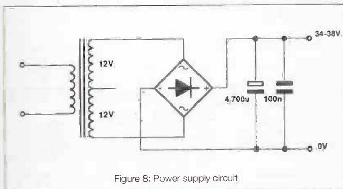
Figure 8: Power supply circuit
