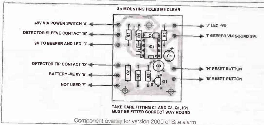
Component overlay for version 2000 of Bite alarm
