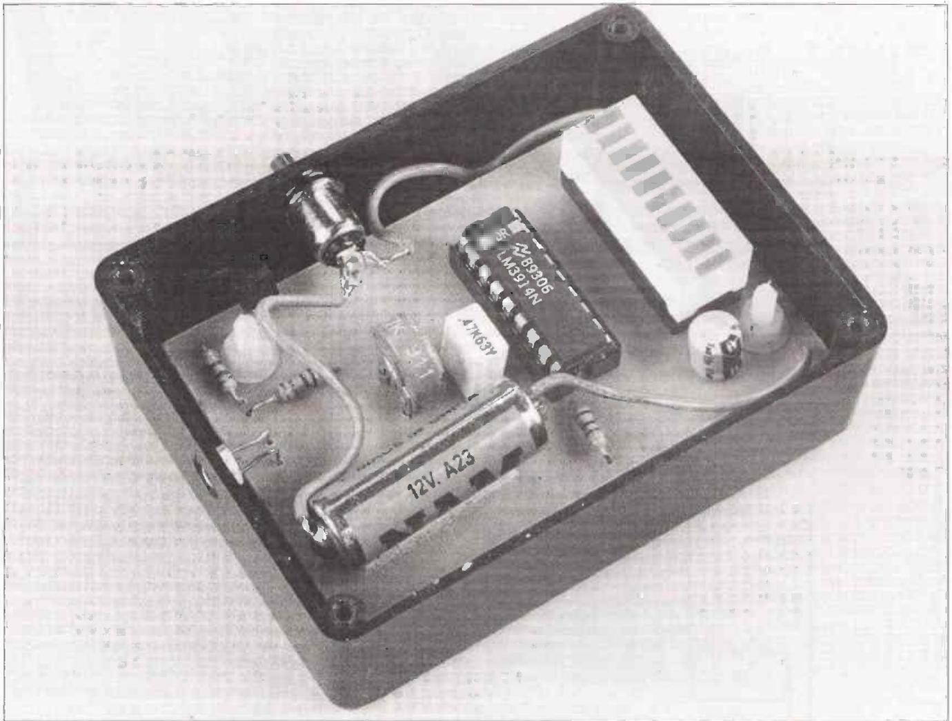
voltage provided by Q1 collector needs to be divided by four. This is achieved when VR1 wiper is at approximately mid-track position. However, the voltage at the wiper may be adjusted through wide limits. This provides the adjustment for the correct operating levels and will be made at the end of construction.
