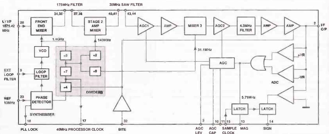
Block diagram of a GP1010 GPS chip
