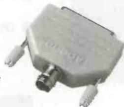
The ADC-10 gives your computer a single channel of analog input. Simply plug into the parallel port.
