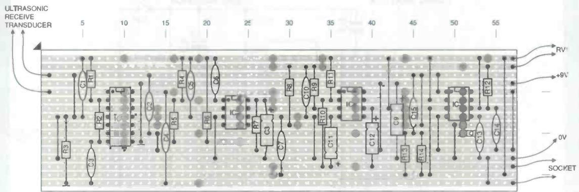
NOTE: STRIPBOARD MAY BE CUT THROUGH AT COLUMN 28 FOR STACKING INTO SMALLER BOX, WITH SHORT WIRE LINKS BETWEEN HOLES 27 AND 29 ON TRACKS C, D, H, J, K, L, M, N, S
