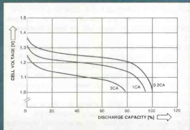
Figure 6: Discharge characteristics as a function of discharge rate. (Courtesy Varta Ltd.)
