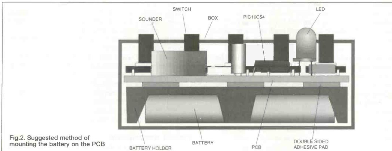
Fig.2. Suggested method of mounting the battery on the PCB
