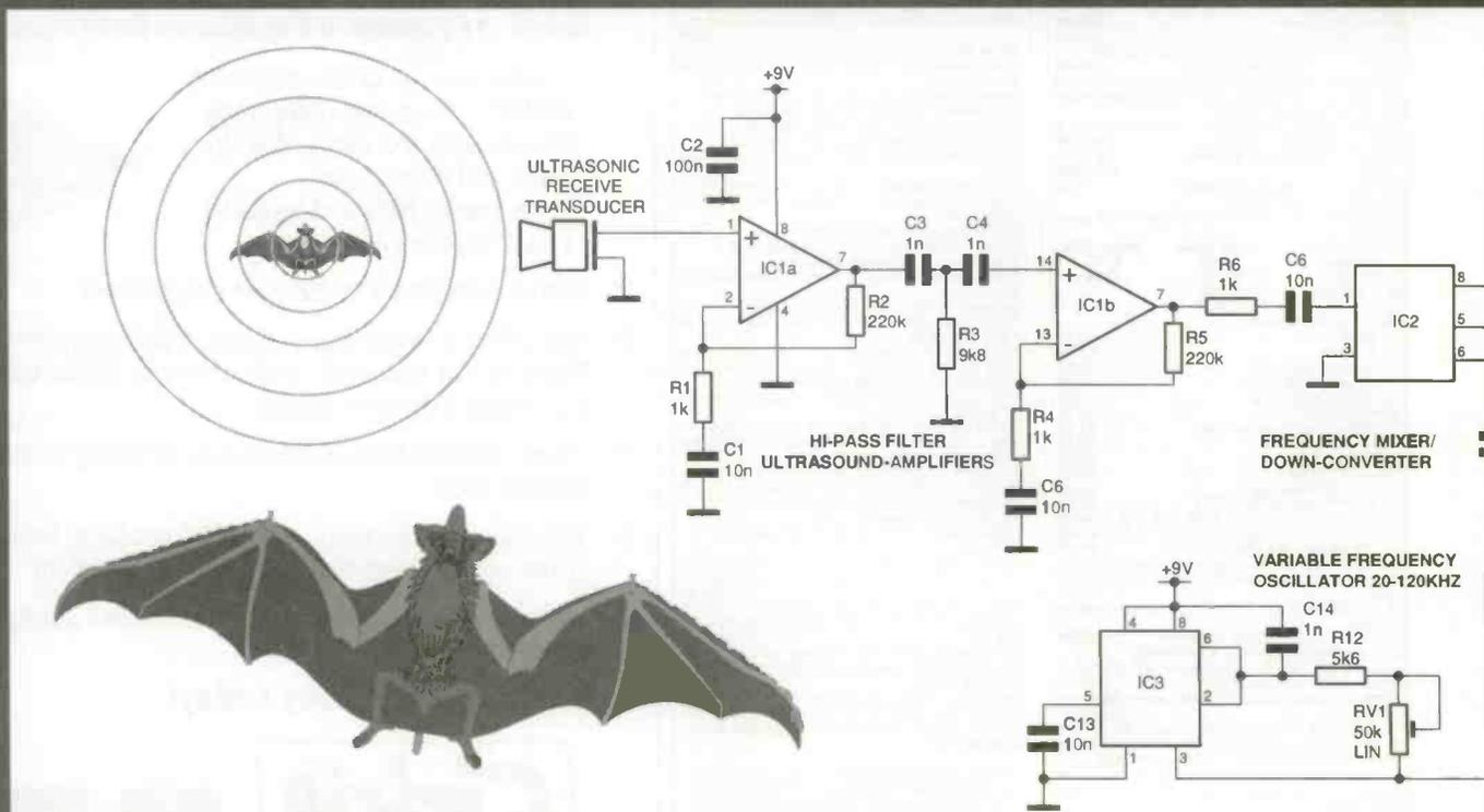
Fig.1. Circuit diagram for heterodyne bat-detector
