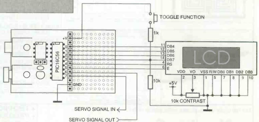
Fig.1. Circuit diagram for STAMP based servo checker
