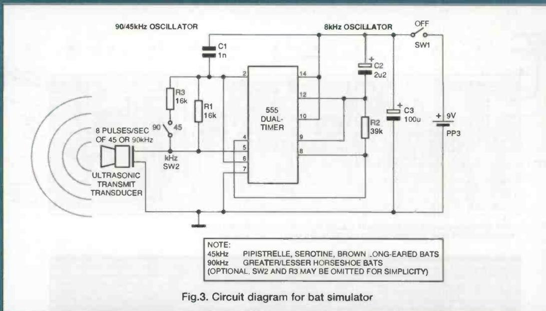
Fig.3. Circuit diagram for bat simulator
