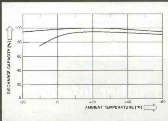
Figure 8: Discharge capacity as a function of temperature for NiMH cells
