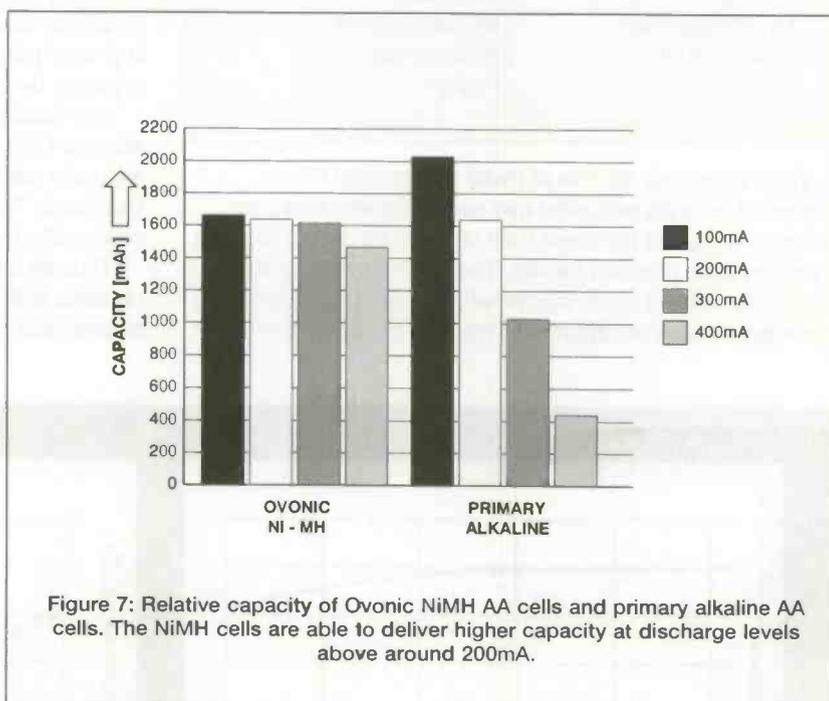
Figure 7: Relative capacity of Ovonic NiMH AA cells and primary alkaline AA cells. The NiMH cells are able to deliver higher capacity at discharge levels above around 200mA.
