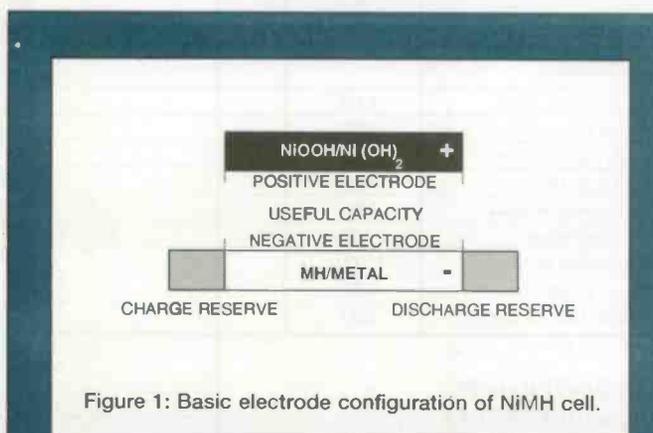
Figure 1: Basic electrode configuration of NiMH cell.
