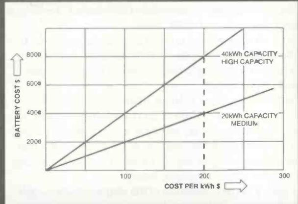
Figure 11: Estimate of range of costs for a range of battery capacities in kWh as a function of cost per kWh (20 kWh medium range/capacity :40 kWh high range/capacity).
