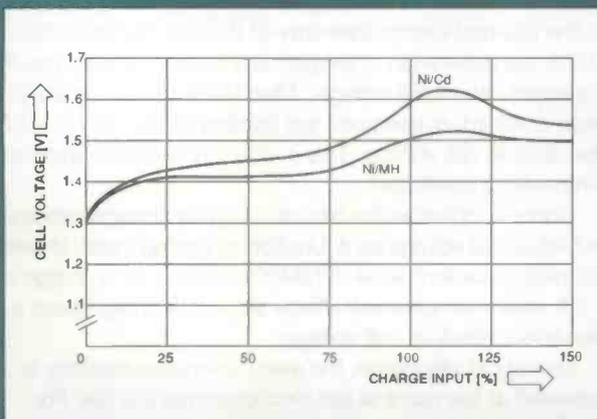
Figure 5: Typical charging characteristics of individual cell voltage as a function of charge input showing relative performance of NiMH and NiCd cells for a charge rate of 1 CA. (Courtesy Varta Ltd.)
