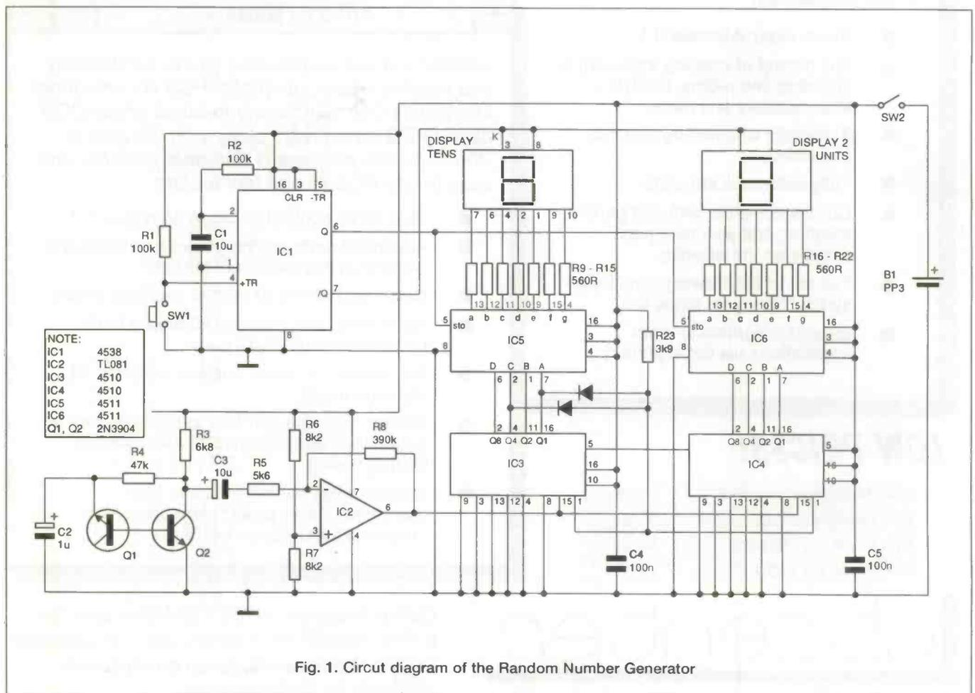
Fig. 1. Circuit diagram of the Random Number Generator
