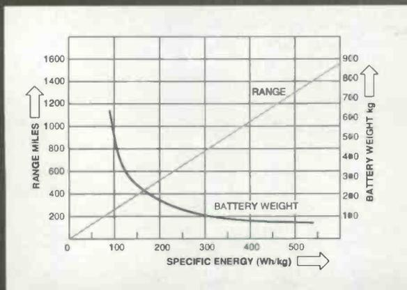
Figure 10: Dashed line: range of 'Impact' type EV with NiMH batteries as a function of specific energy of the batteries. Solid line: Mass of battery for equivalent range capacity of 250 miles for 'Impact' type car as a function of specific energy of batteries
