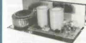
**OMP/MF 200 Mos-Fet Output power 200 watts R.M.S. into 4 ohms, frequency response 1Hz - 100KHz -3dB, Damping Factor >300, Slew Rate 50V/uS, T.H.D. typical 0.001%, Input Sensitivity 500mV, S.N.R. -110 dB. Size 300 x 155 x 100mm. PRICE £64.35 + £4.00 P&P**
