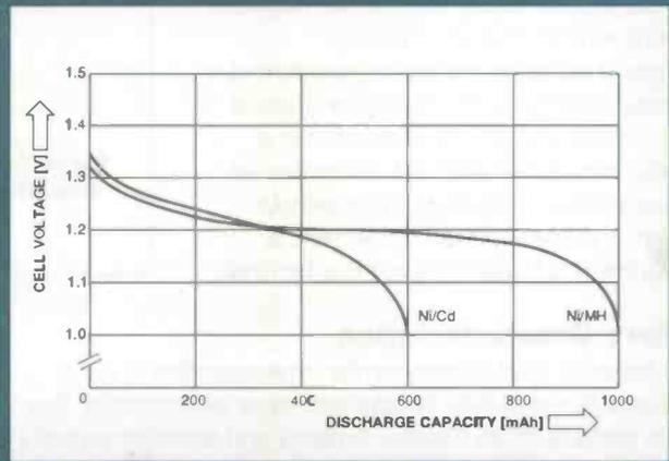
Figure 4: Discharge curve of Varta AA cells compared with conventional NiCd AA cell. (Courtesy Varta Ltd.)
