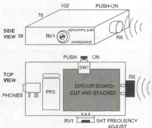
Fig. 6. Bat detector housing
