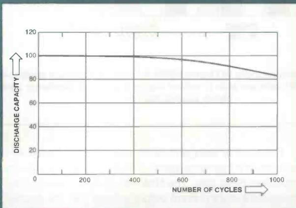
Figure 3: Life expectancy of standard NiMH cell for 0.25 CA charge and 0.25 CA discharge conditions. (Courtesy Varta Ltd.)
