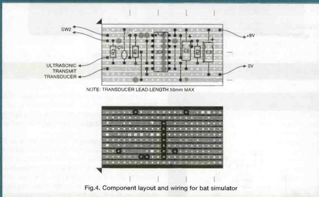
Fig.4. Component layout and wiring for bat simulator
