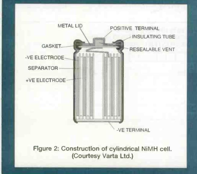
Figure 2: Construction of cylindrical NiMH cell. (Courtesy Varta Ltd.)
