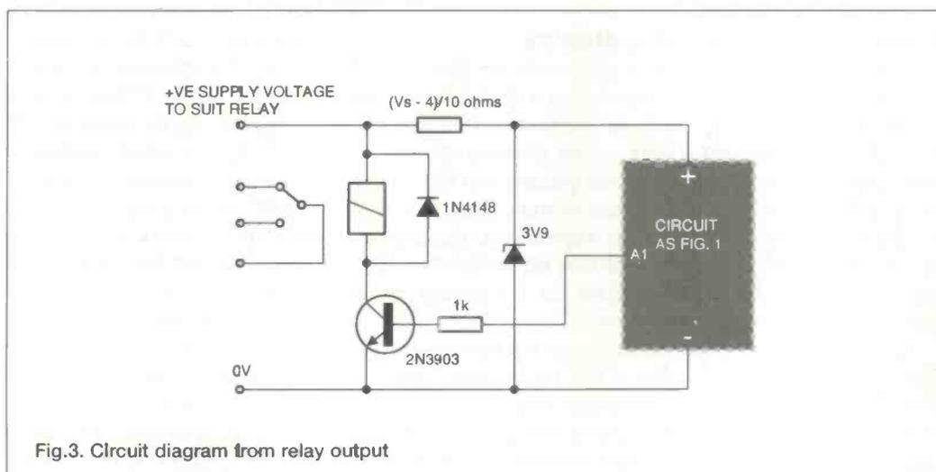
Fig.3. Circuit diagram from relay output
