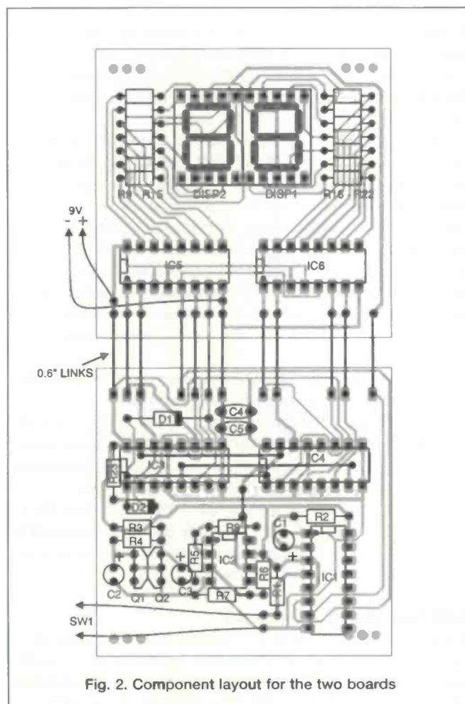
Fig. 2. Component layout for the two boards
