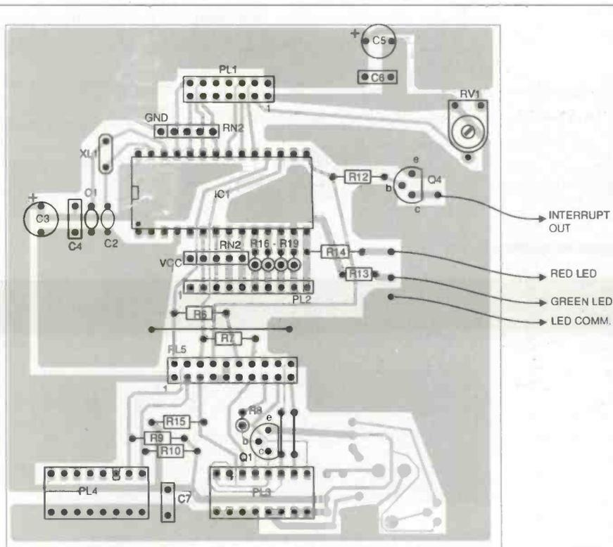
Fig.10. Component overlay for auxiliary board.
