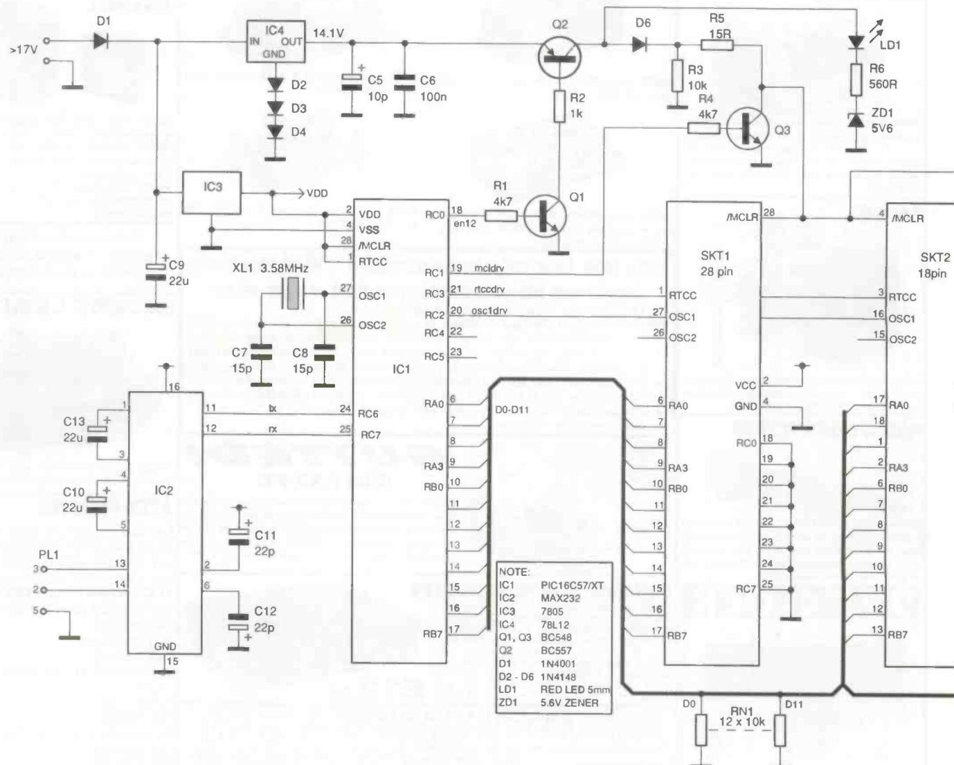
Fig.1. PIC programmer circuit
