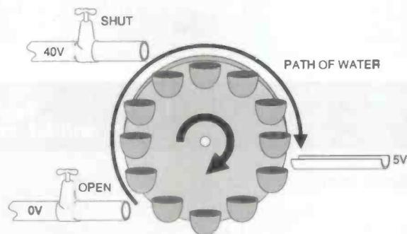
Fig.3. The water-wheel analogy: while the top tap is open (Fig 3a), the water wheel is pushed round faster and faster, building up momentum; when the top tap is shut (Fig3b), the water wheel scoops up water from the lower tap, losing momentum.
