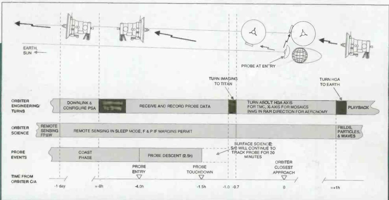
Figure 14: Data capture and relay of Huygens probe data by the Cassini orbiter. (Courtesy ESA)
