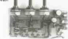
3 channel wireless sound to light system, mains operated, separate sensitivity adjustment for each channel, 1,200 watt power handling. Microphone included. £16.45 Kit no 1014.
