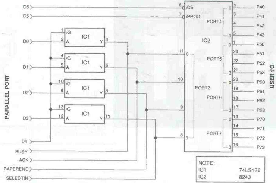
Fig.4. A 74LS based port extender
