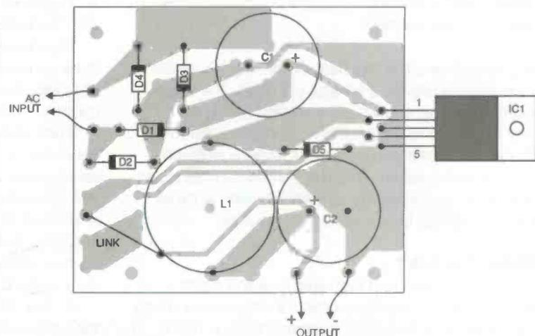
Fig 7. PCB layout for the switcher for 5, 12 and 15V. Note the alternative positions for different versions of L1. Note also that several holes are not used in this version. Be careful with the orientation of C1. The PCB tracking connecting C2, L1, the output and the feedback may look odd, but it is correct (the shape is to minimise the effect of ripple current).
