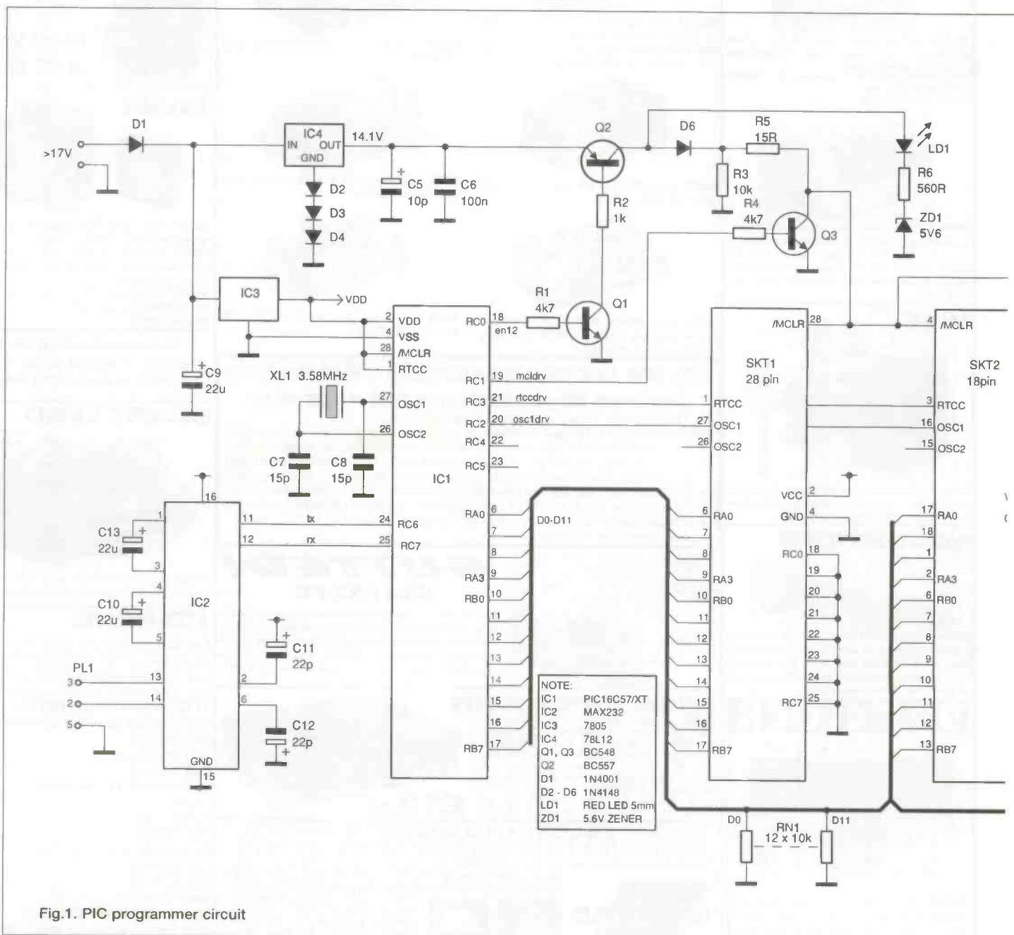
Fig.1. PIC programmer circuit
