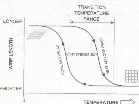
Fig.1. Temperature vs SMA wire length
