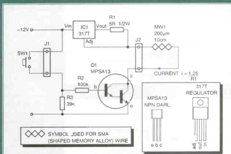
Fig.2. SMA wire driver circuit
