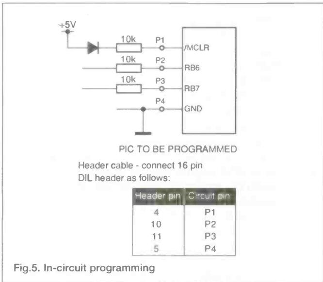
Fig.5. In-circuit programming
