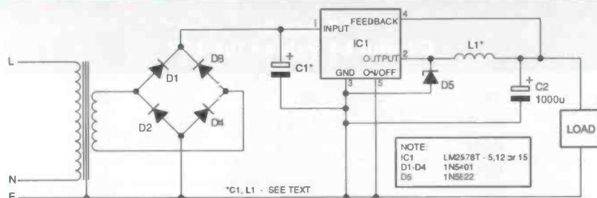
Fig 6. The switcher circuit for fixed 5, 12 and 15 V supplies.
