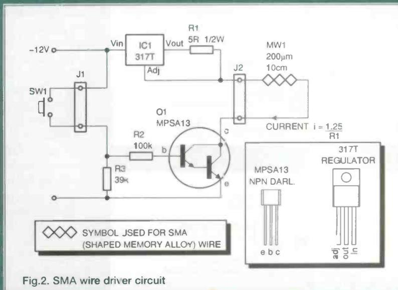
Fig.2. SMA wire driver circuit
