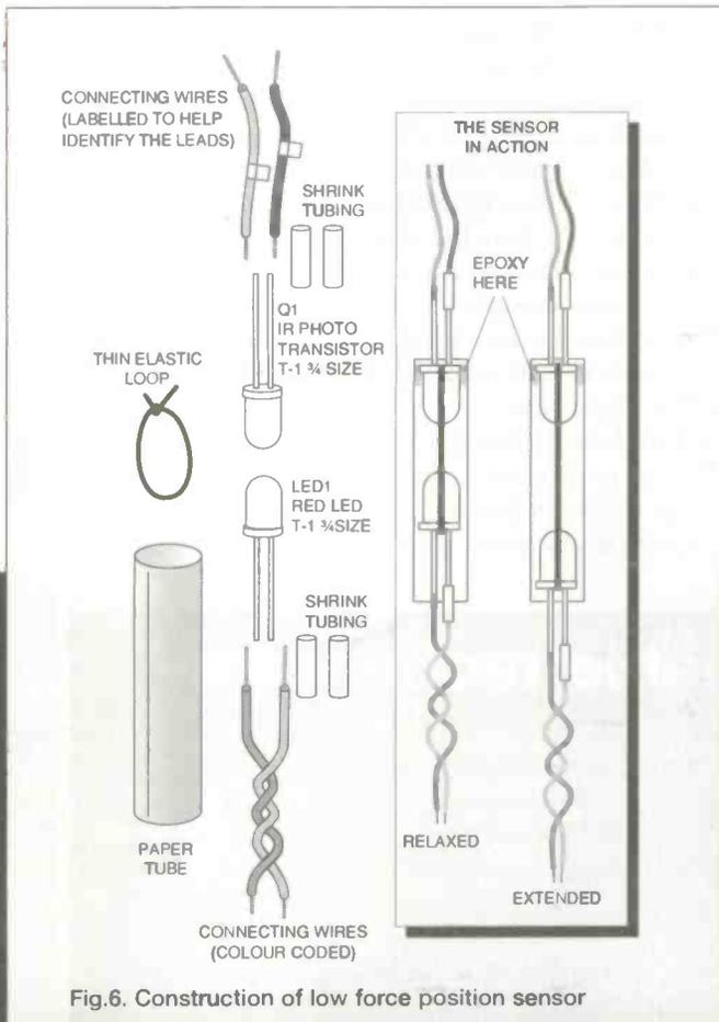
Fig.6. Construction of low force position sensor
