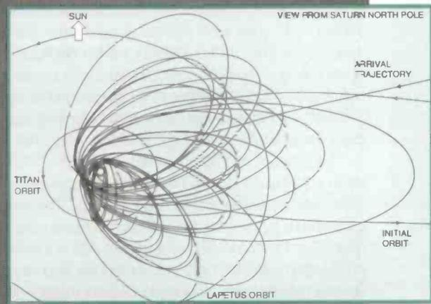
Figure 10. Sequence of orbits planned for the Cassini orbiter craft (Courtesy ESA).
