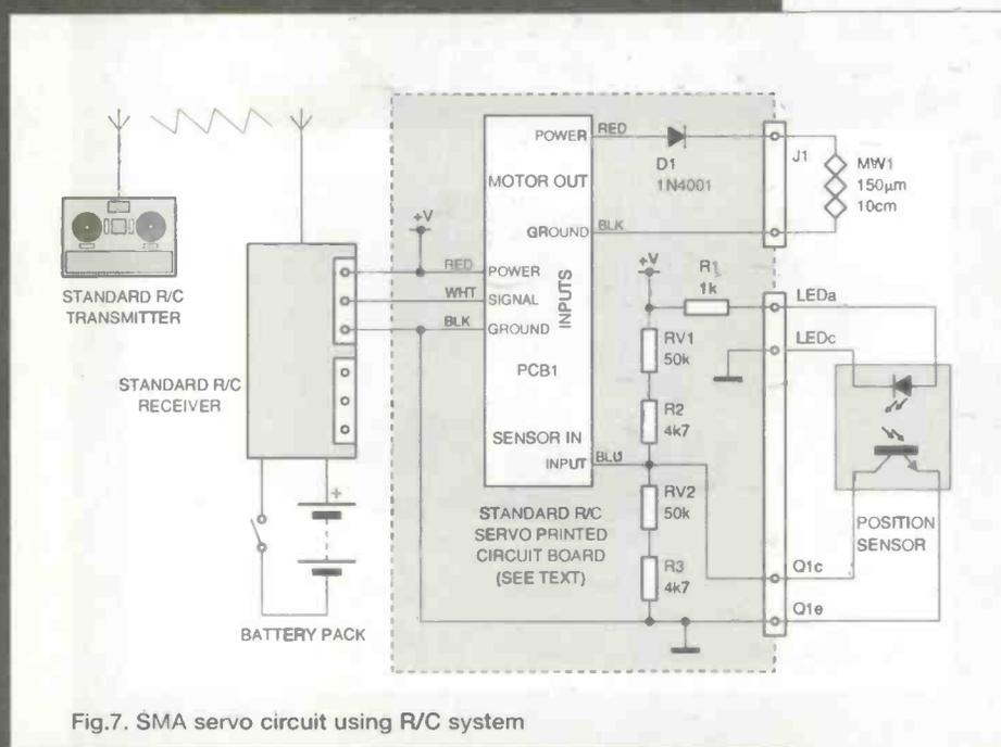
Fig.7. SMA servo circuit using R/C system
