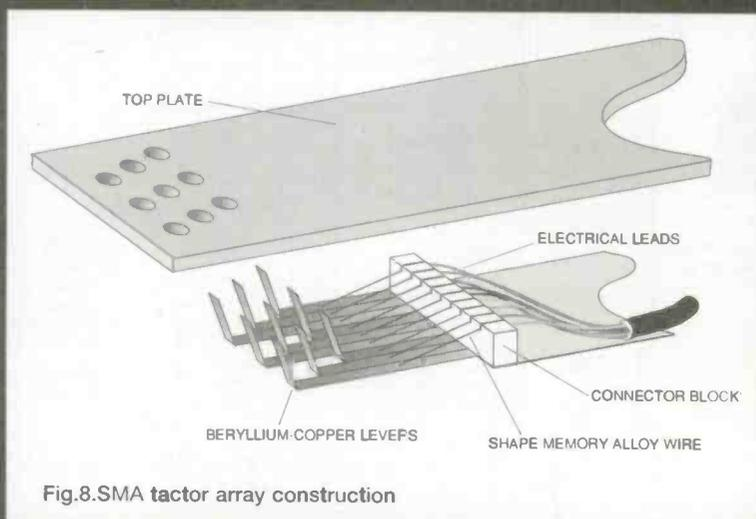
Fig.8.SMA tactor array construction
