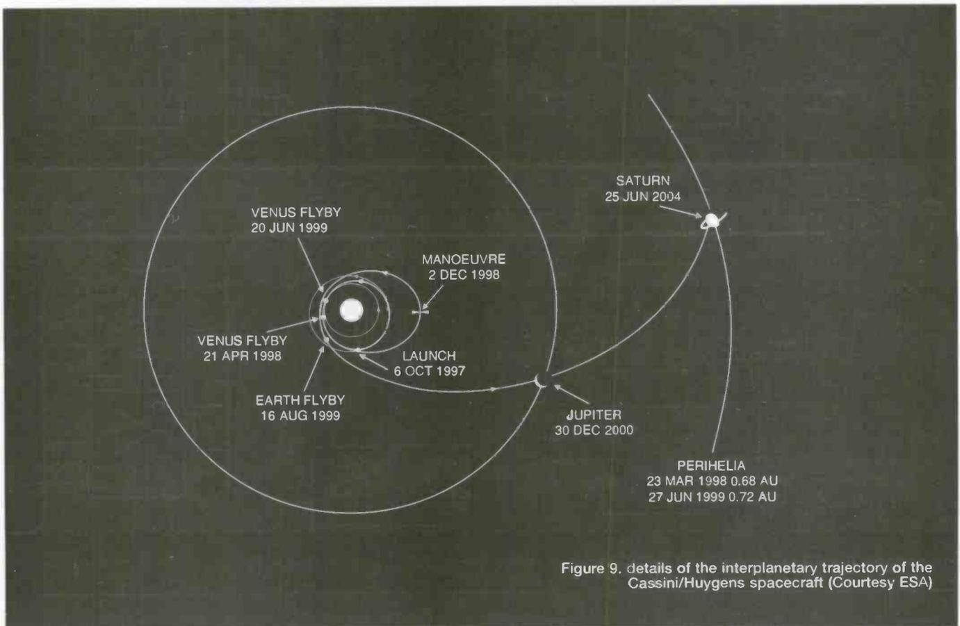
Figure 9. details of the interplanetary trajectory of the Cassini/Huygens spacecraft (Courtesy ESA)
