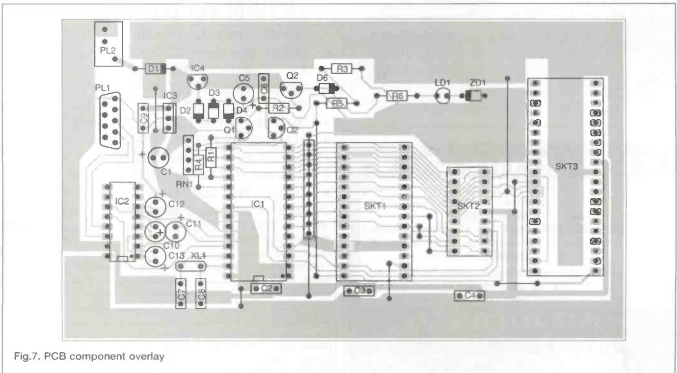
Fig.7. PCB component overlay
