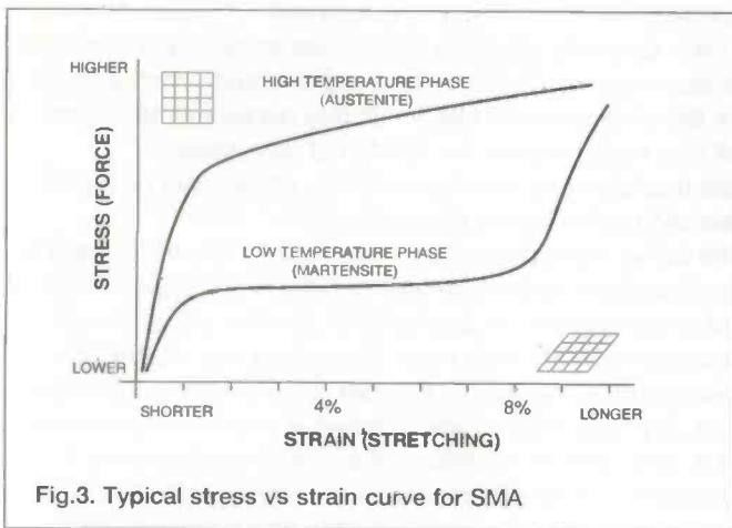
Fig.3. Typical stress vs strain curve for SMA
