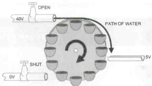
Fig 3. Essential switcher action: while the transistor conducts, current flows through the inductor, building up the magnetic field; when the transistor is off, current flows from the diode, but from ground to positive due to the action of the inductor.
