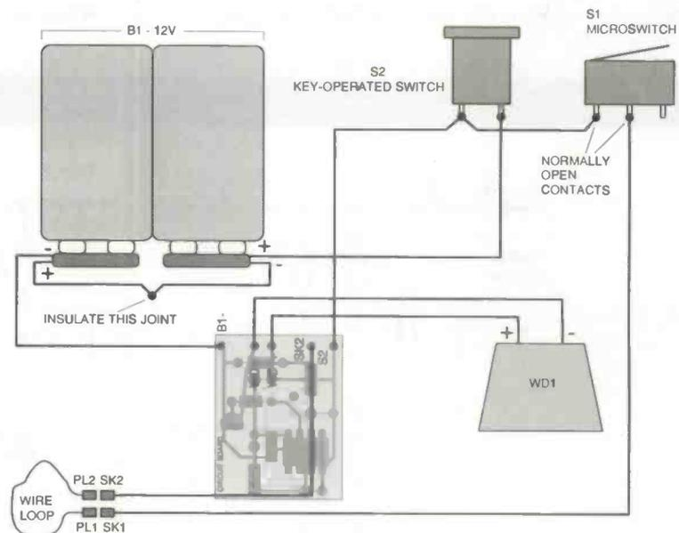
Fig. 3. Bicycle loop alarm wiring diagram
