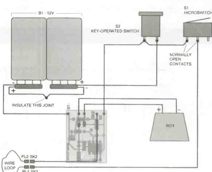
Fig. 3. Bicycle loop alarm wiring diagram
