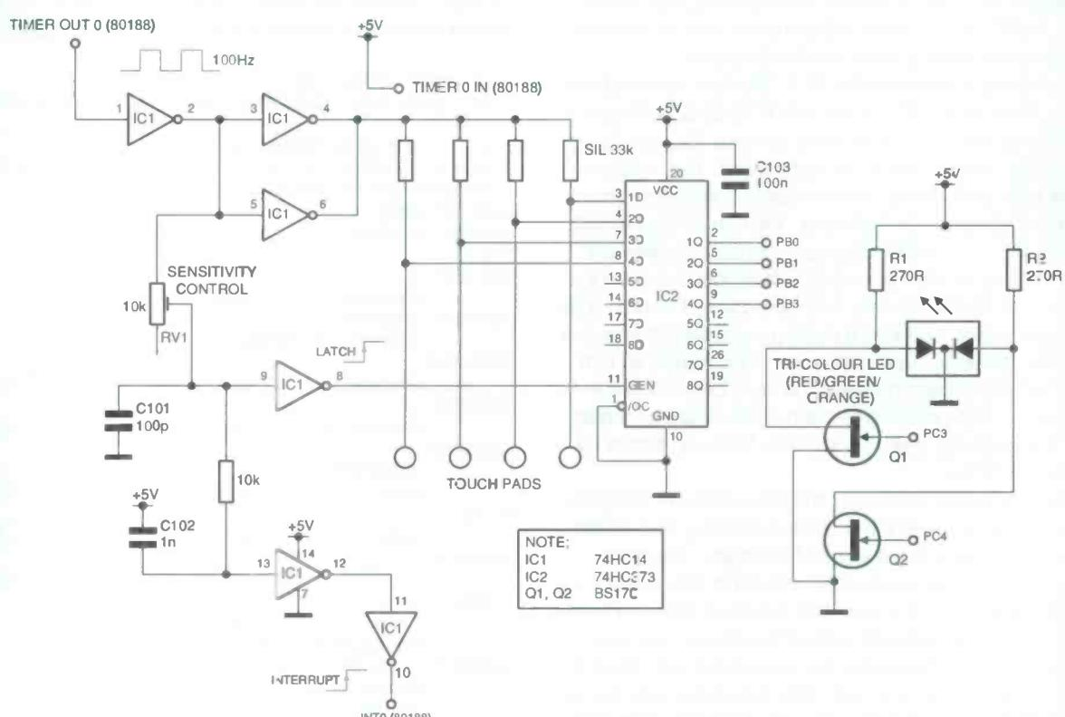
Fig. 2. Touch switch circuit diagram
