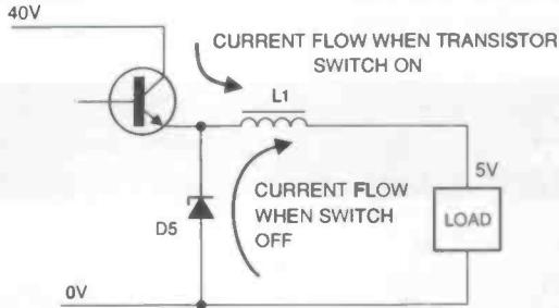
Fig.2. The essential elements of the switcher are the switch itself, an inductor, a capacitor and a controlled oscillator.
