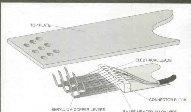
Fig.8 SMA tactor array construction
