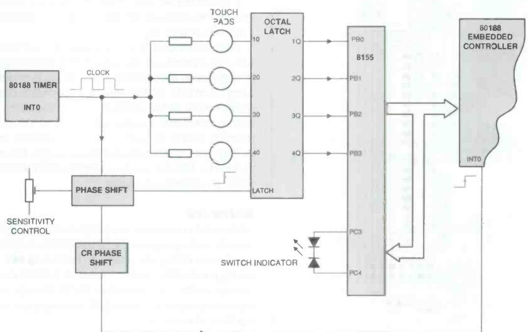
Fig. 1. Touch switch interface block diagram
