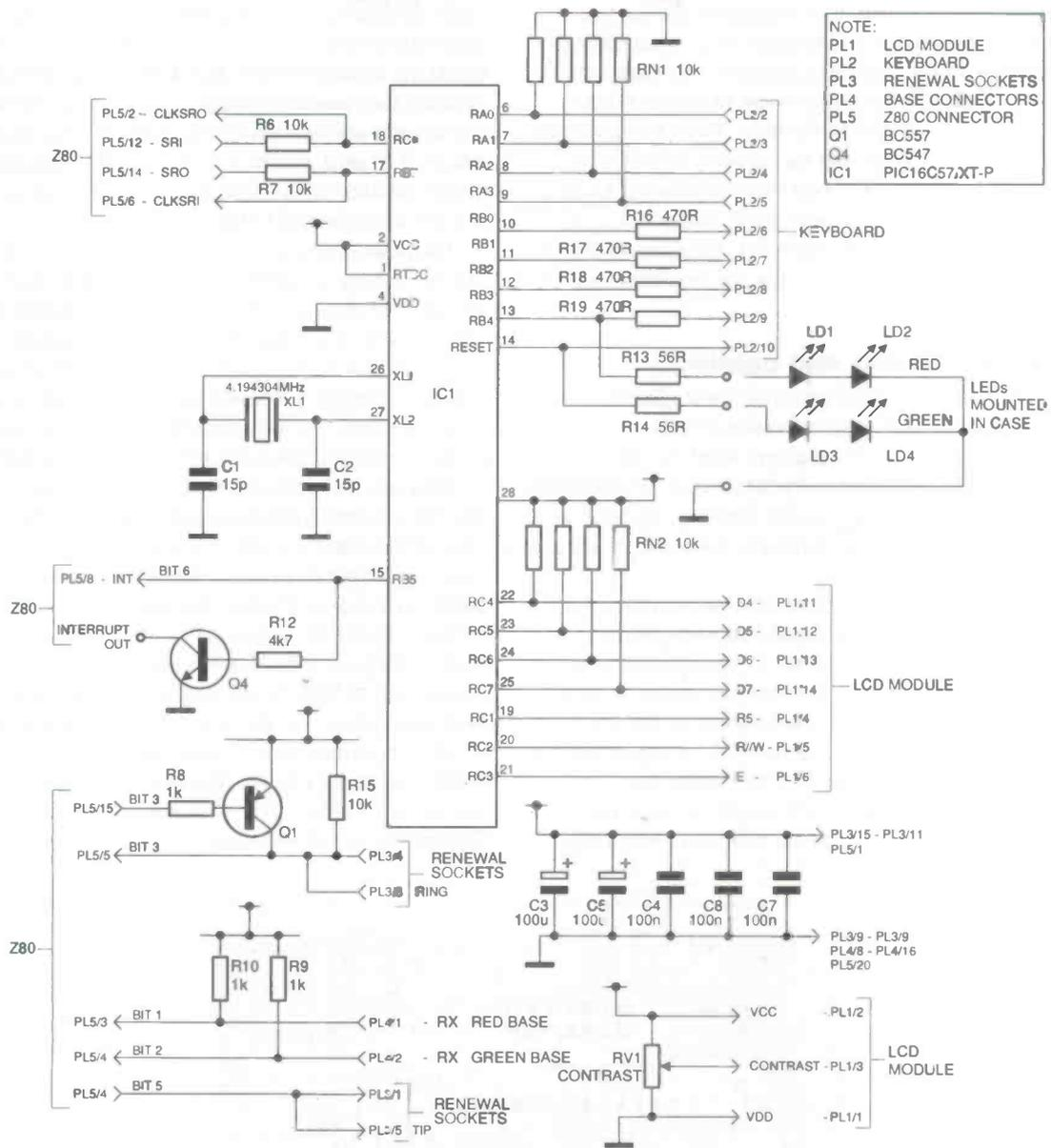
Fig.8. Circuit diagram for auxiliary board
