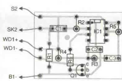
Fig. 2. Bicycle loop alarm PCB component overlay
