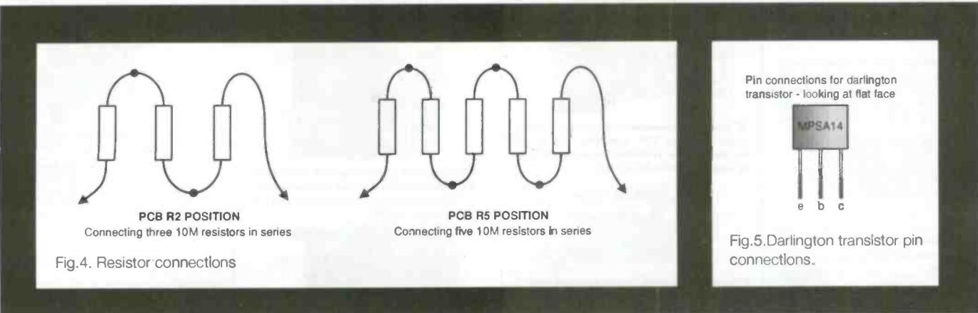
Pin connections for darlington transistor - looking at flat face
