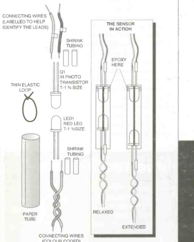
Fig.6. Construction of low force position sensor
