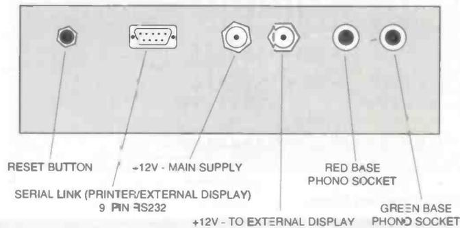
Fig.12. Connectors on rear of case
