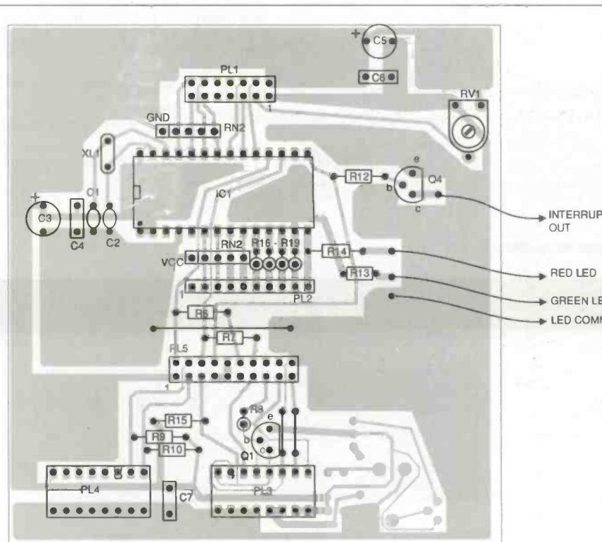
Fig.10. Component overlay for auxiliary board.
