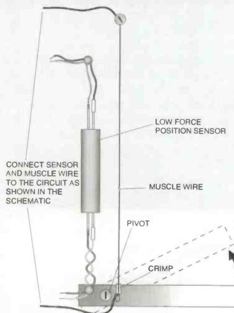
Fig.4. SMA wire based servo mechanism
