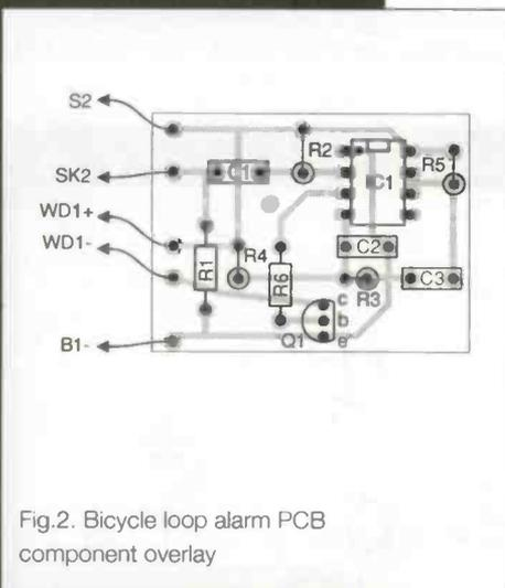
Fig. 2. Bicycle loop alarm PCB component overlay
