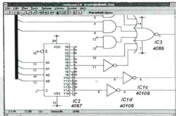
**Busses and Power rails handled easily using Global Nets on PRO+**
