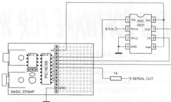
One of the commonest requirements in any microcontroller application is to input and process analog data. This could be simply a variable voltage signal from some other piece of equipment, or it could be the output from some sort of measurement circuit, perhaps measuring temperature, pressure, strain, pH, etc. In this short article, we look at the hardware and software required to interface an 8-bit serial analog-to-digital converter to the Parallax BASIC Stamp.
