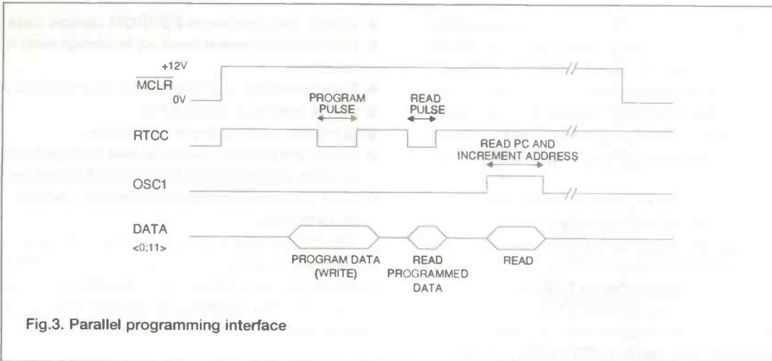
Fig.3. Parallel programming interface
