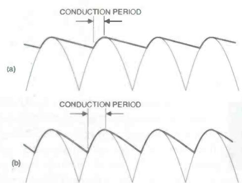
Fig 5. In Fig 5a, a high reservoir capacitance value leads to the very short conduction time; In Fig 5b, the conduction time is increased but so is ripple. So long as the unregulated voltage is above the operating margin needed by the regulator, high ripple can lead to higher efficiency.
