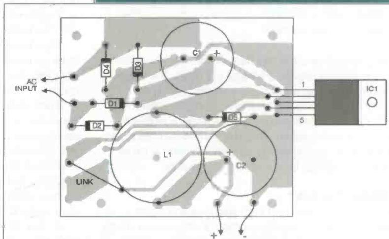
Fig 7. PCB layout for the switcher for 5, 12 and 15V. Note the alternative positions for different versions of L1. Note also that several holes are not used in this version. Be careful with the orientation of C1. The PCB tracking connecting C2, L1, the output and the feedback may look odd, but it is correct (the shape is to minimise the effect of ripple current).
