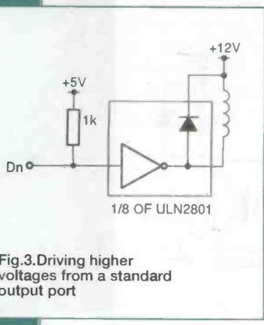
**Fig.3.** Driving higher voltages from a standard output port
