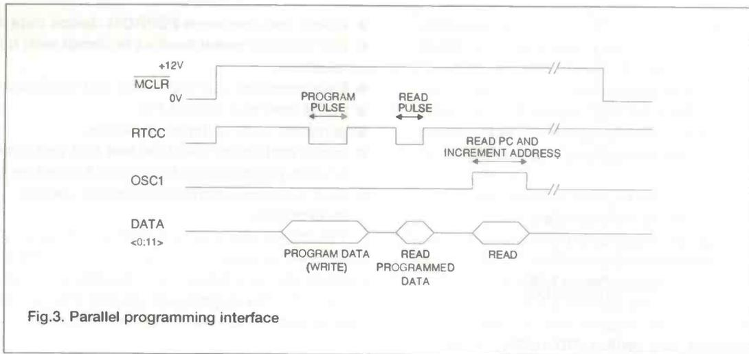
Fig.3. Parallel programming interface
