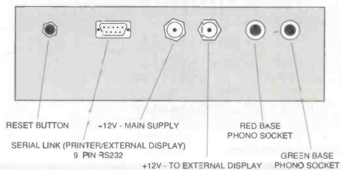
**Fig.12. Connectors on rear of case**
