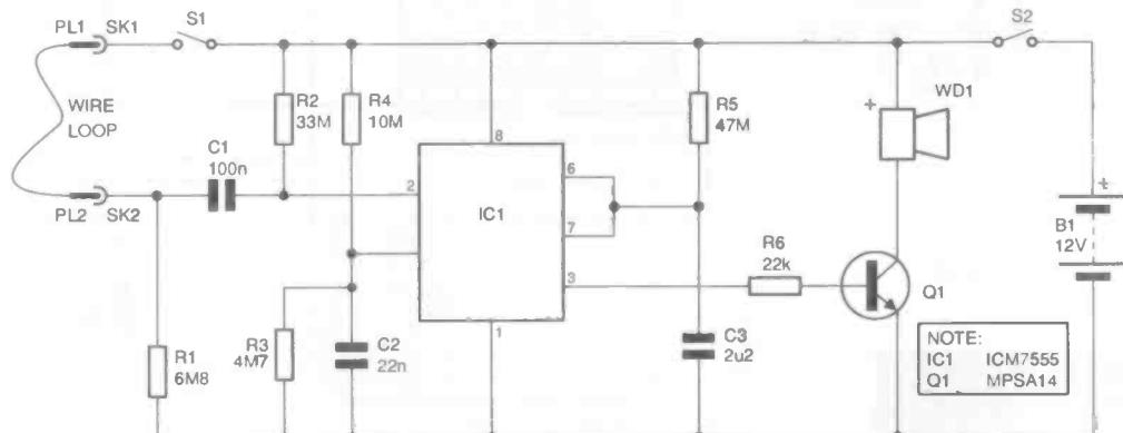
Fig.1. Bicycle loop alarm circuit diagram
