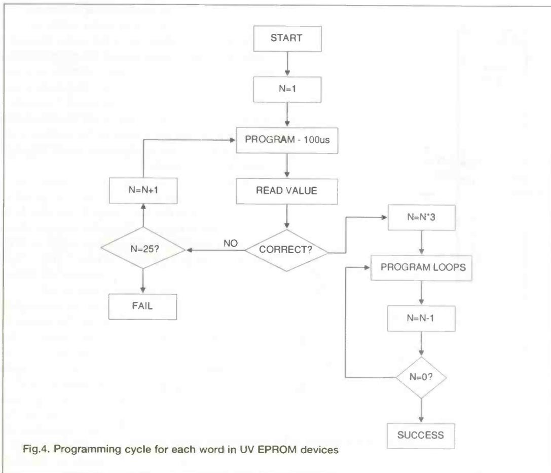
Fig.4. Programming cycle for each word in UV EPROM devices
