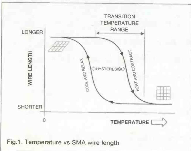
Fig.1. Temperature vs SMA wire length
