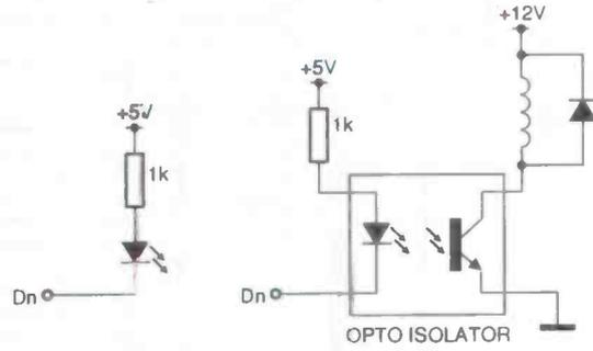
Fig. 2. Optoisolator circuit for computer interface designs.
