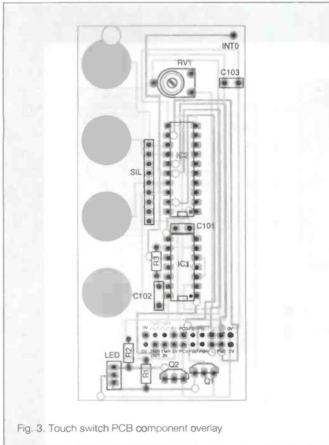
Fig. 3. Touch switch PCB component overlay
