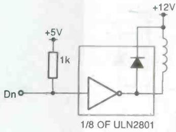
Fig.3. Driving higher voltages from a standard output port
