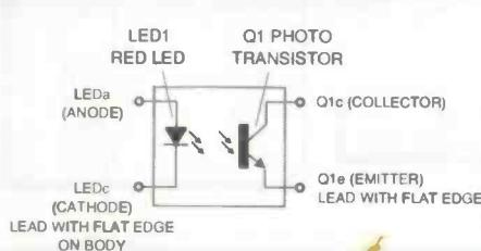
Fig.5. Low force position sense circuit
