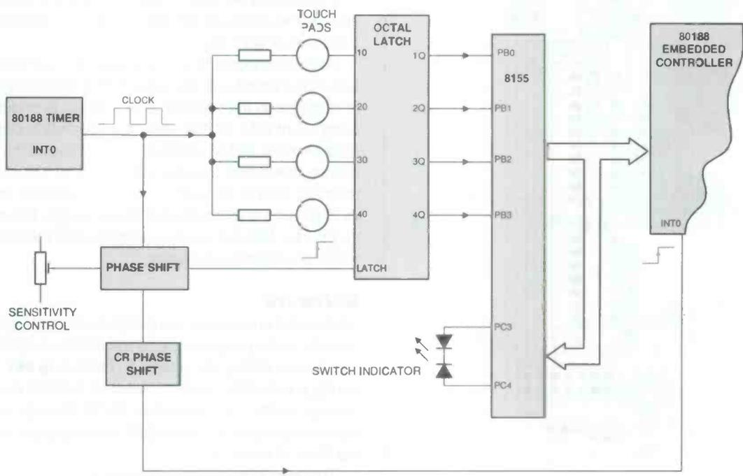
Fig. 1. Touch switch interface block diagram
