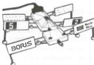
Fascinating, highly processed Shape Memory Alloy wires that actually contract when electrically heated producing a useful amount of force.
