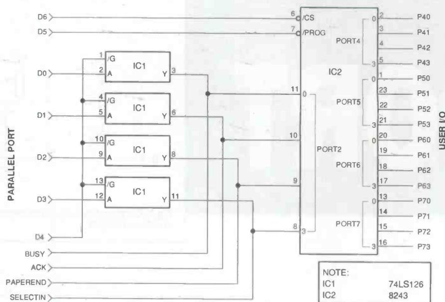
**Fig.4.A** 74LS based port extender
