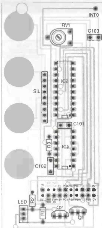
Fig. 3. Touch switch PCB component overlay
