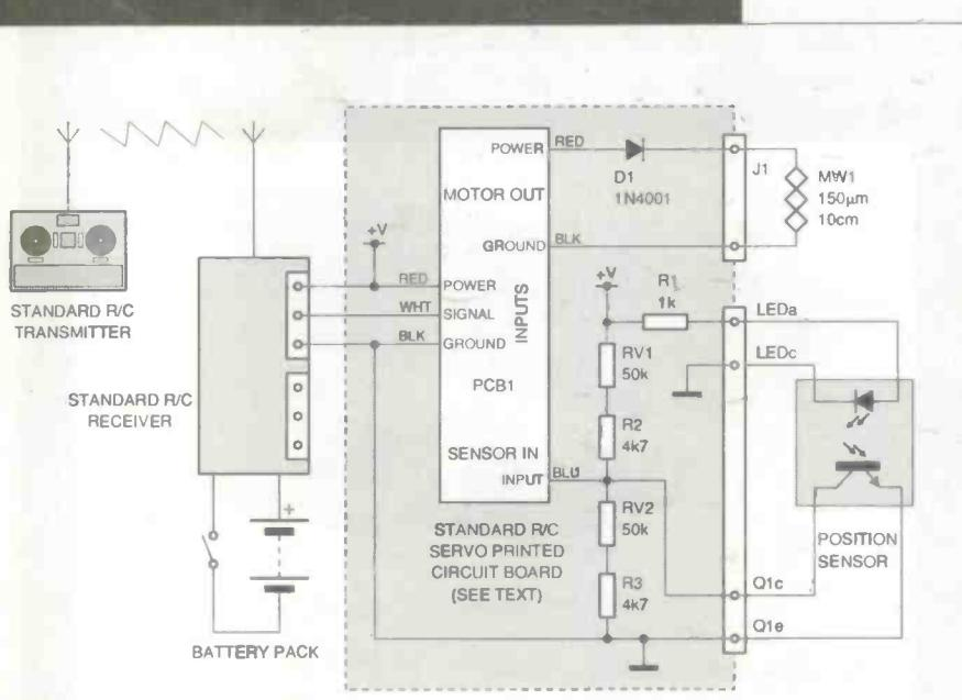
Fig.7. SMA servo circuit using R/C system
