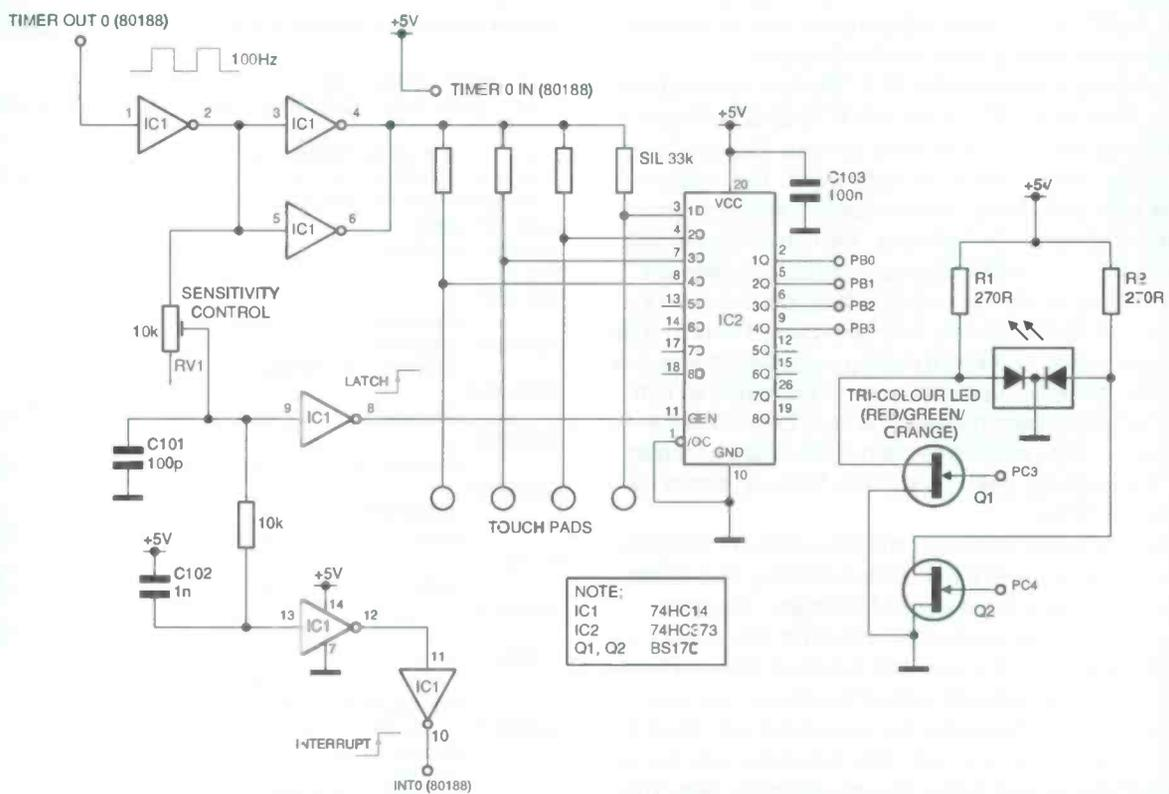
Fig. 2. Touch switch circuit diagram
