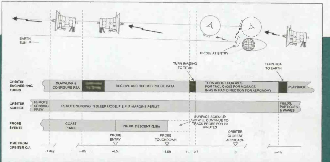
Figure 14: Data capture and relay of Huygens probe data by the Cassini orbiter. (Courtesy ESA)
