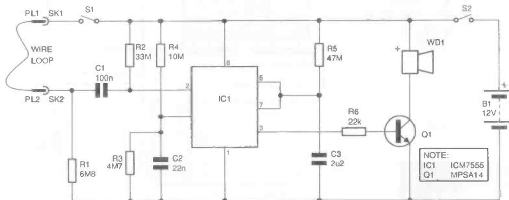
Fig. 1. Bicycle loop alarm circuit diagram
