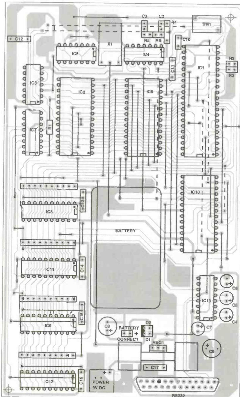
Fig.9. Component overlay for main processor
