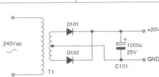
Fig.2. Circuit diagram of PIC programmer power supply
