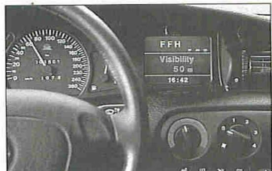
Figure 2: Opel Concept Car: Display indicates measured visibility derived from infra-red backscatter signals
