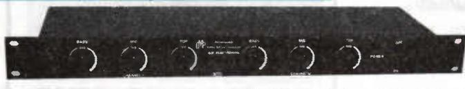
Advanced 3-Way Stereo Active Cross-Over, housed in a 19" x 1U case. Each channel has three level controls: bass, mid & top. The removable front fascia allows access to the programmable DIL switches to adjust the cross-over frequency: Bass-Mid 250/500/800Hz, Mid-Top 1.8/3/5KHz, all at 24dB per octave. Bass invert switches on each bass channel. Nominal 775mV input/output. Fully compatible with OMP rack amplifier and modules.
