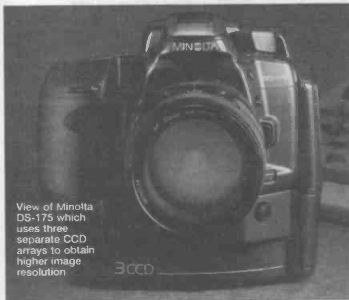
View of Minolta DS-175 which uses three separate CCD arrays to obtain higher image resolution
