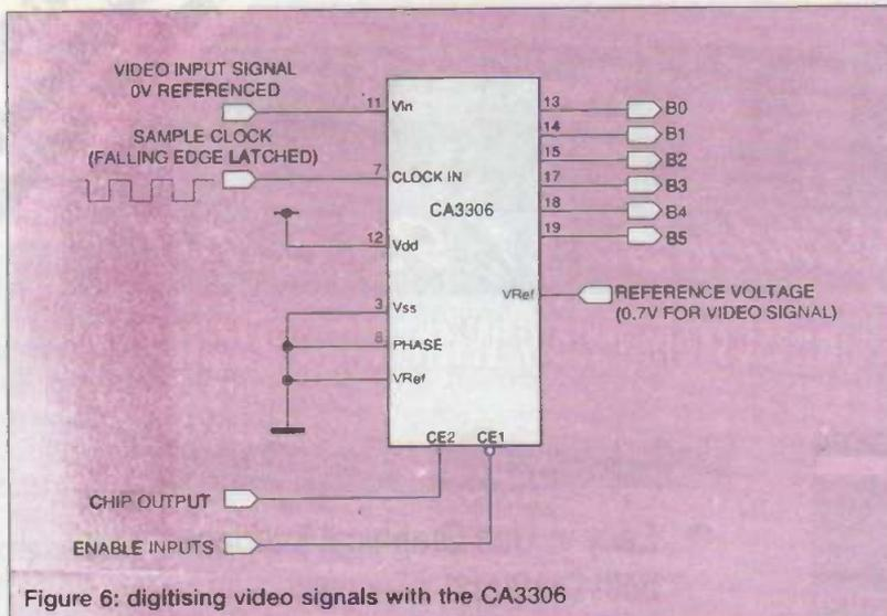
Figure 6: digitising video signals with the CA3306
