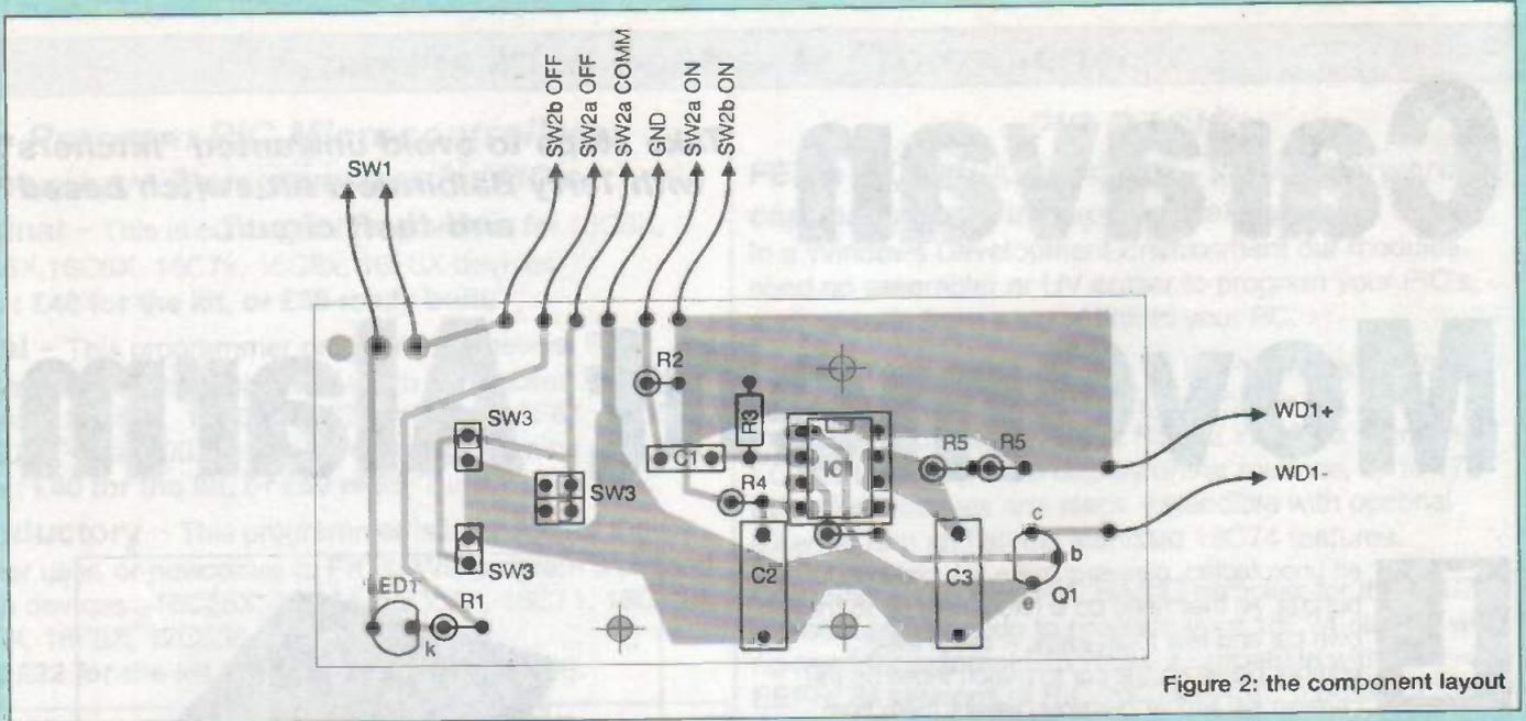
Figure 2: the component layout
