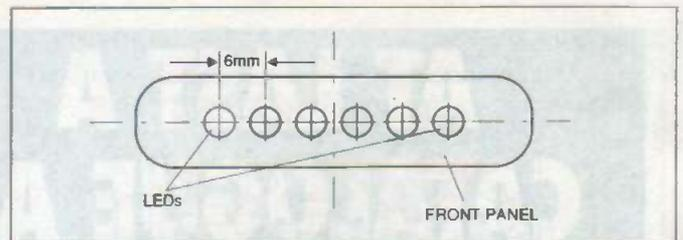
Figure 5: guide to drilling the LED holes - 3mm diameter - in the front panel
