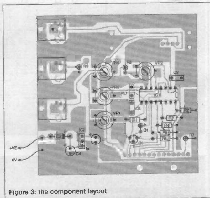
Figure 3: the component layout
