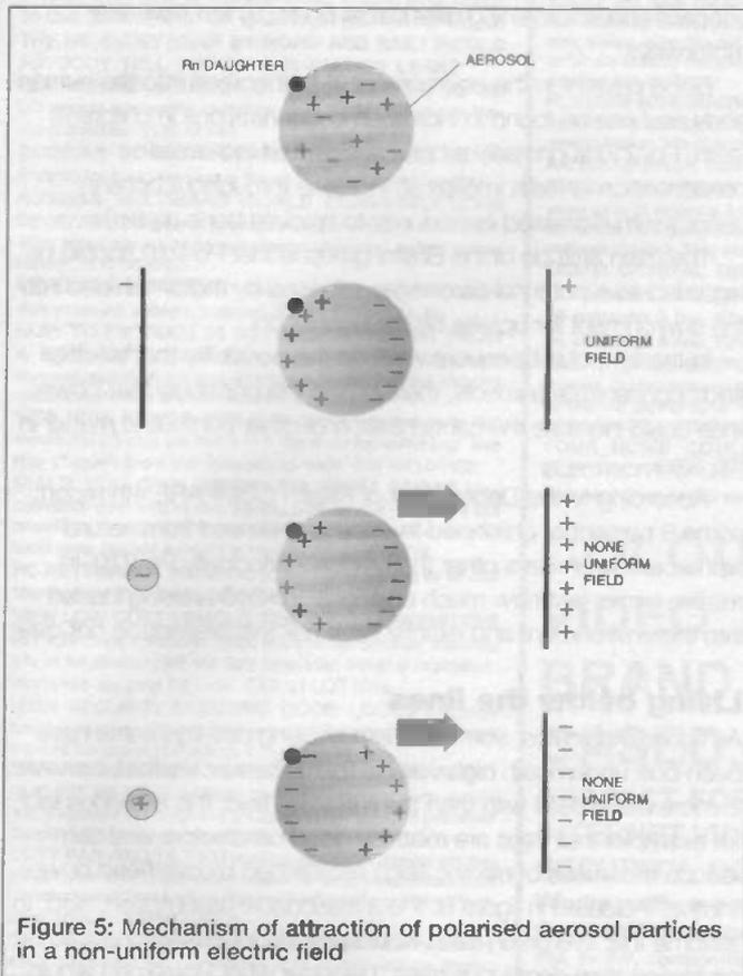
Figure 5: Mechanism of attraction of polarised aerosol particles in a non-uniform electric field
