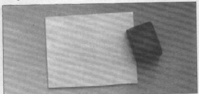
Cleaning the copper board with a mildly abrasive pad (not supplied). Wire wool can also be used.
