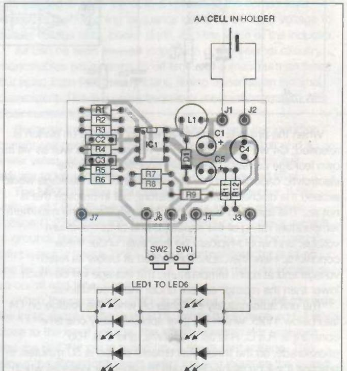
Figure 4: the component layout and offboard wiring
