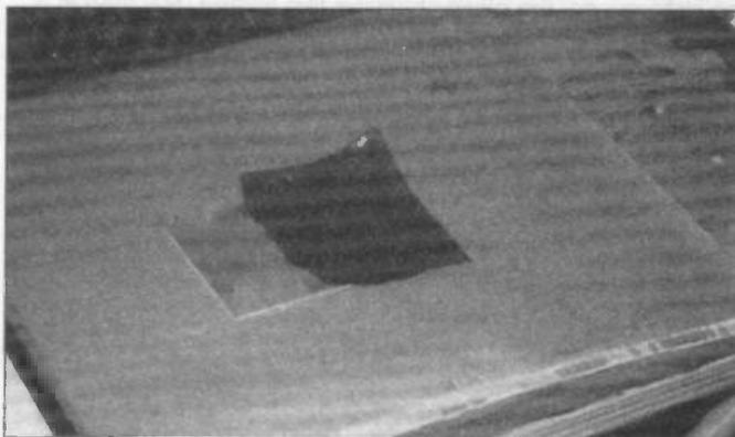
Image transferring to the copper plate - the image shows black through the film backing. The unadhered edges tend to curl up when heated, but the ironed-on area should lie flat.
