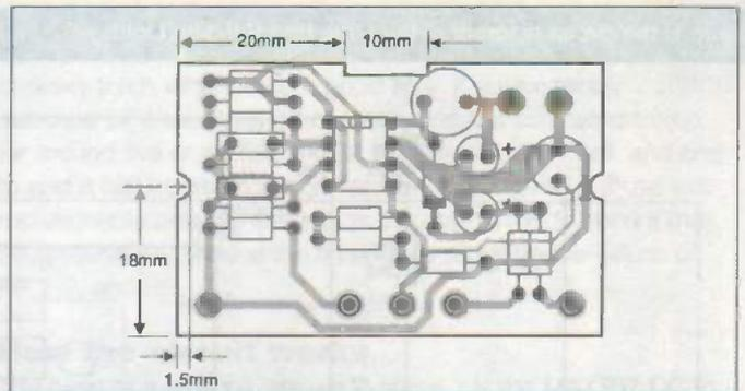
Figure 3: a guide to the cutouts to be filed in the pcb if using the case specified
