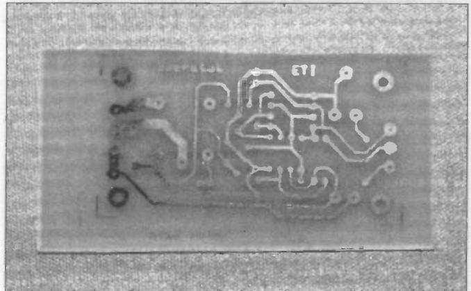
The board after emerging from the etching tray. The resist may appear partly blue and partly grey at this stage, but both will clean off with the stripper provided.
