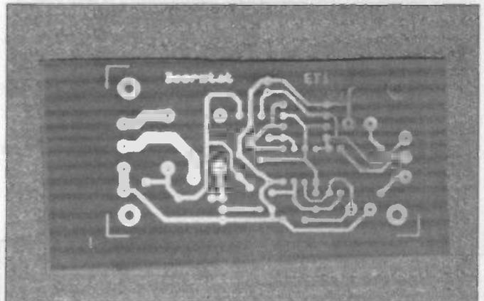
The board etched and cleaned and ready to drill. It may not be quite as "sharp" as an industrially-produced board, but the results are good nevertheless - and much cheaper.
