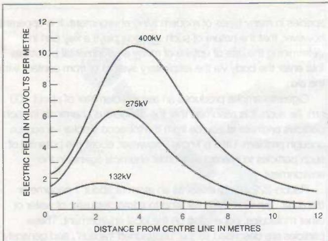
Figure 4: Typical values of electric field for a range of high voltage transmission lines which typically carry a pair of transmission lines about the mid plane of such systems. (Courtesy NRPB)
