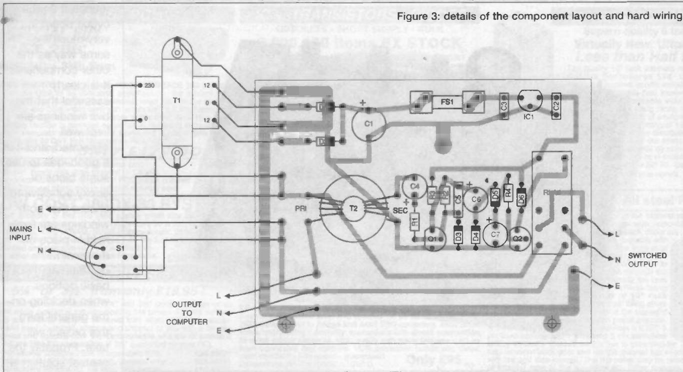
from the mains supply. T1 is the step-down and isolation transformer in the power supply unit, which is a conventional 12 volt stabilised design. D1 and D2 provide full-wave rectification, and C1 is the smoothing capacitor. IC1 is a small (100 milliamp) voltage regulator, which is more than adequate in this application where the maximum current drain is only about 50 milliamps. Protection against overloads is provided by fuse FS1, and IC1's built-in output current limiting circuit.
