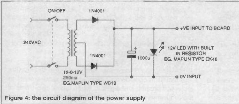
Figure 4: the circuit diagram of the power supply
