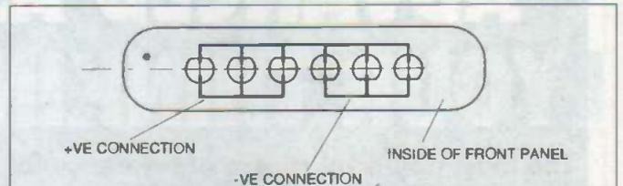
Figure 6: wiring up the LEDs
