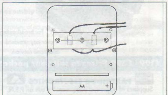
Figure 9: Inside of the the case lid, showing the approximate position of the Veroboard supporting the microswitches, the wiring to the switches, and the bolts securing the board to the case lid.
