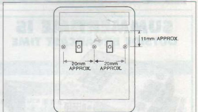
Figure 8: the top of the specified case, showing the position of the microswitches and 6mm bolts screws. See text. The Veroboard fitted inside the lid must clear the taller components on the PCB
