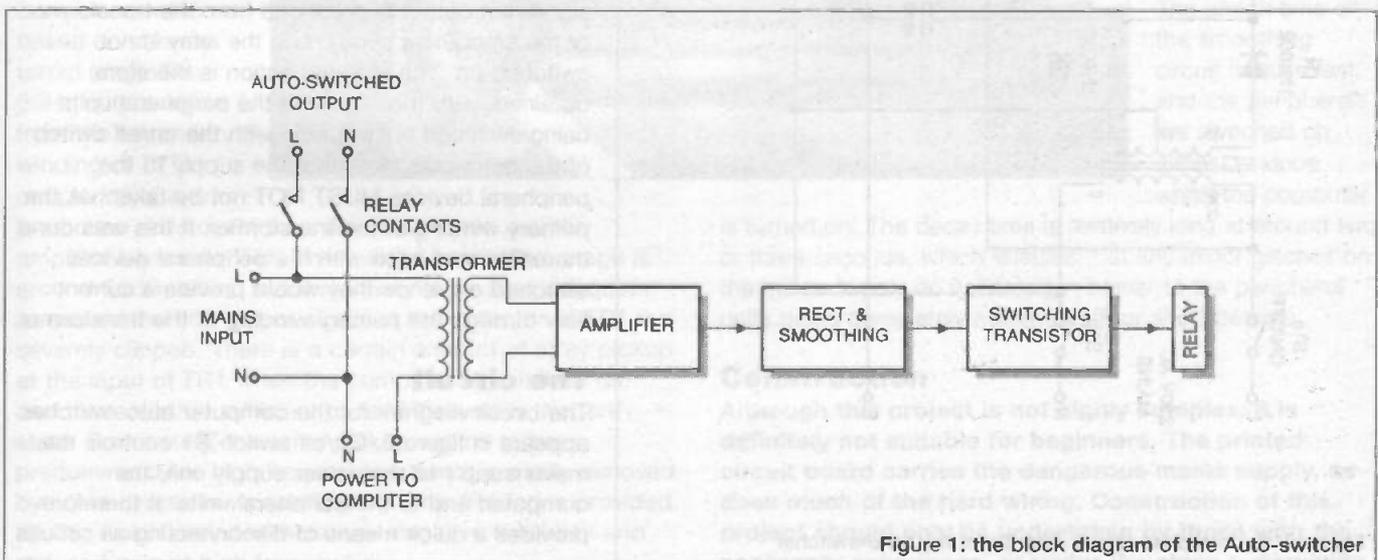
Figure 1: the block diagram of the Auto-switcher
