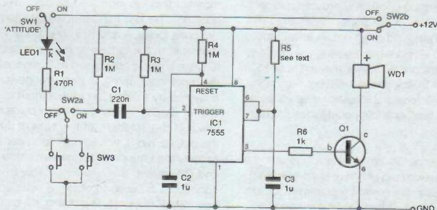
Figure 1: the circuit of the Caravan Movement Alarm
