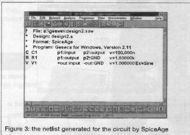
Figure 3: the netlist generated for the circuit by SpiceAge
