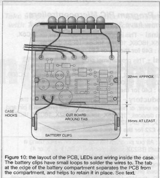
Figure 10: the layout of the PCB, LEDs and wiring inside the case. The battery clips have small loops to solder the wires to. The tab at the edge of the battery compartment separates the PCB from the compartment, and helps to retain it in place. See text.
