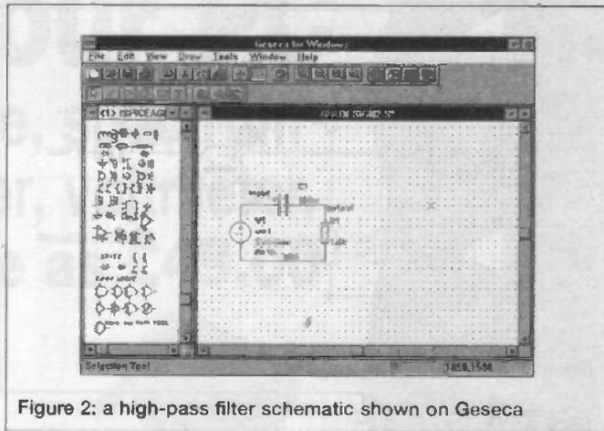
Figure 2: a high-pass filter schematic shown on Geseca
