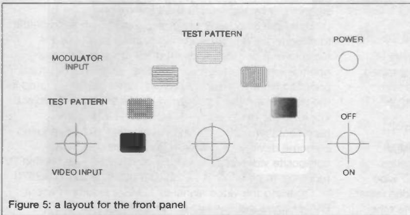
Figure 5: a layout for the front panel
