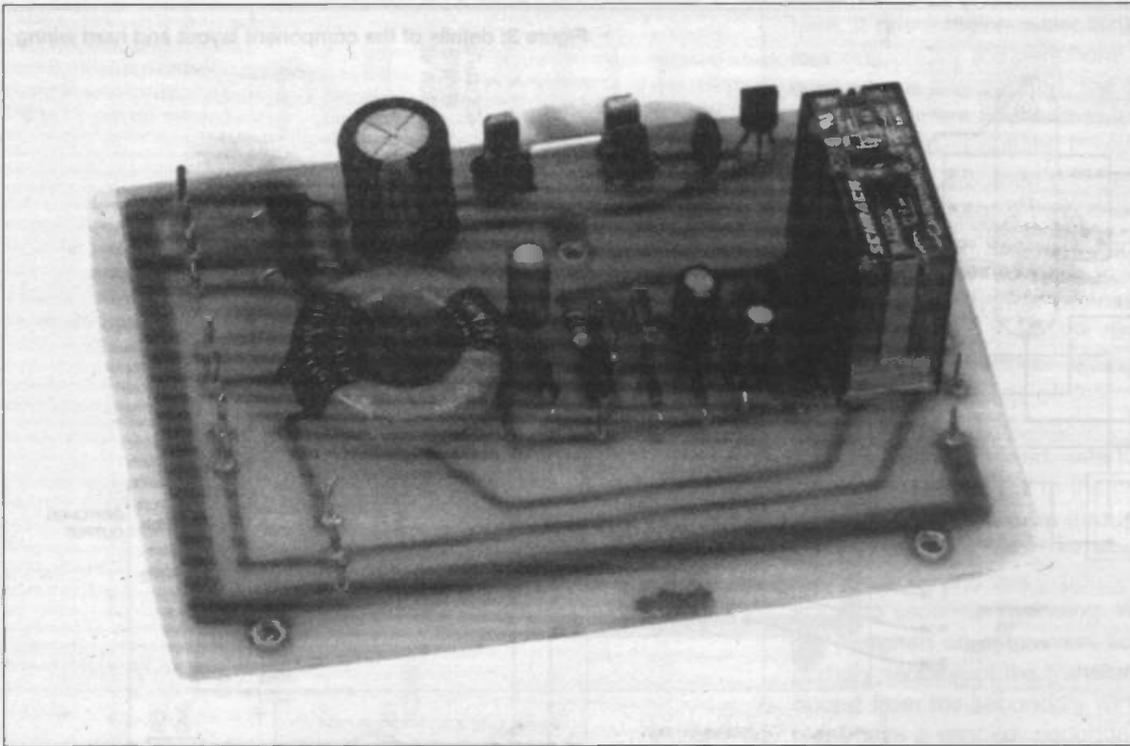
mounted on the circuit board in very much the same way as the other components. It is clearly essential that the two windings are kept well separated, and it is a good idea to use some blobs of epoxy adhesive to ensure that both windings are firmly held in place on the toroid.
