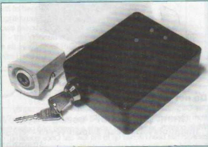
The main unit has the key-operated on/off switch mounted on the side. There is also an "attitude" slide switch on top which works in conjunction with a red light-emitting diode.
