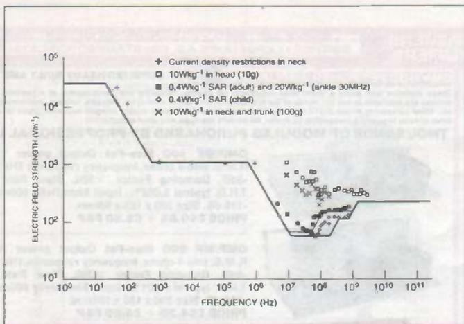
Figure 9: NRPB investigation levels for electric fields between 0 to 300 GHz and with specific SAR restrictions indicated
