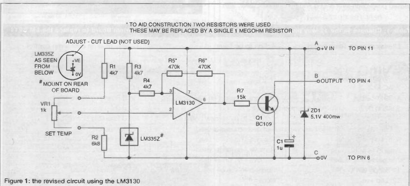
Figure 1: the revised circuit using the LM3130
