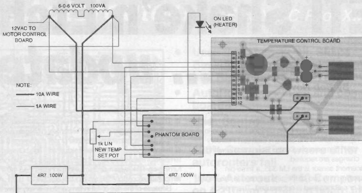
Figure 3: the new connections to the temperature control board
