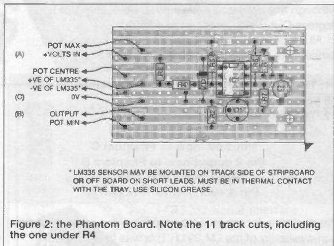
Figure 2: the Phantom Board. Note the 11 track cuts, including the one under R4
