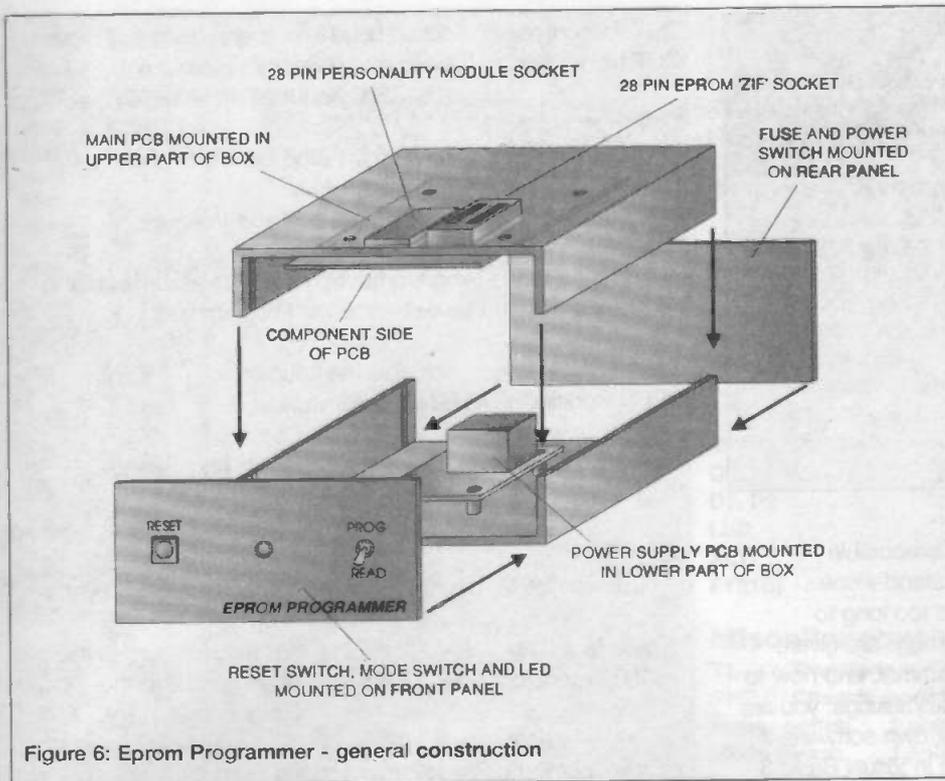
Figure 6: Eprom Programmer - general construction
