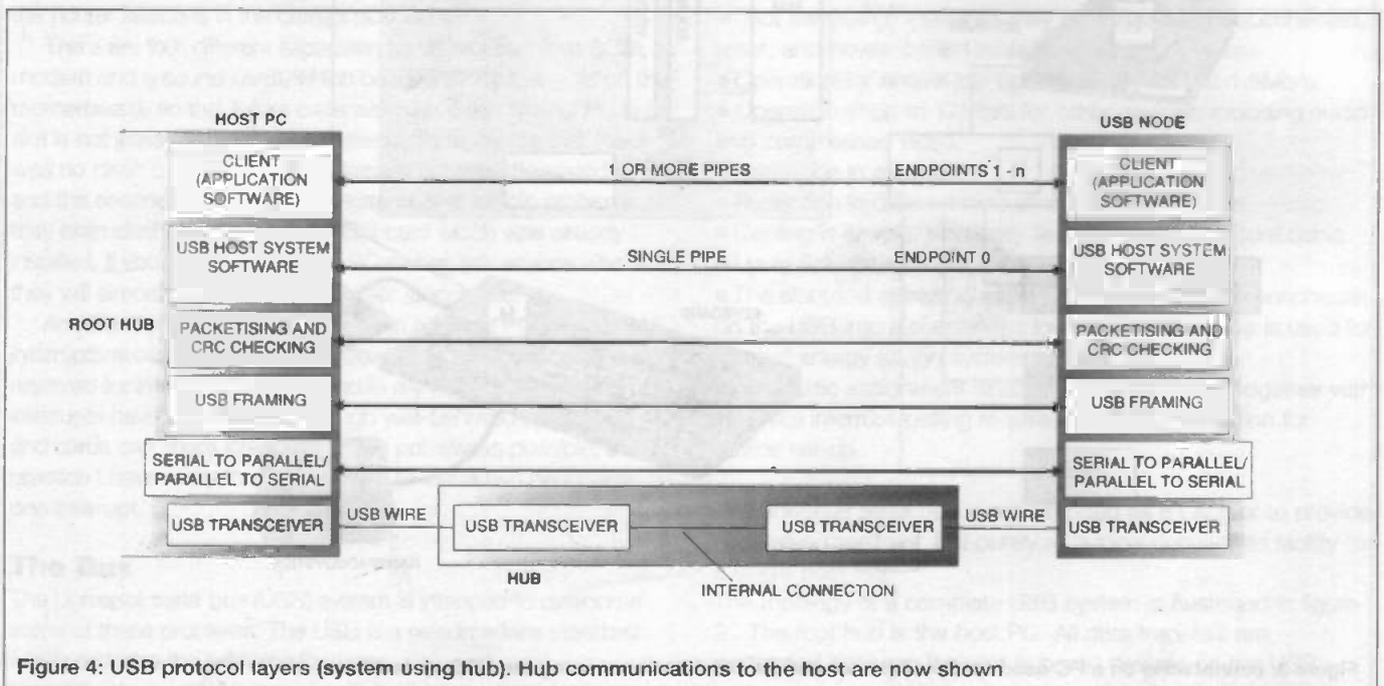
Figure 4: USB protocol layers (system using hub). Hub communications to the host are now shown
