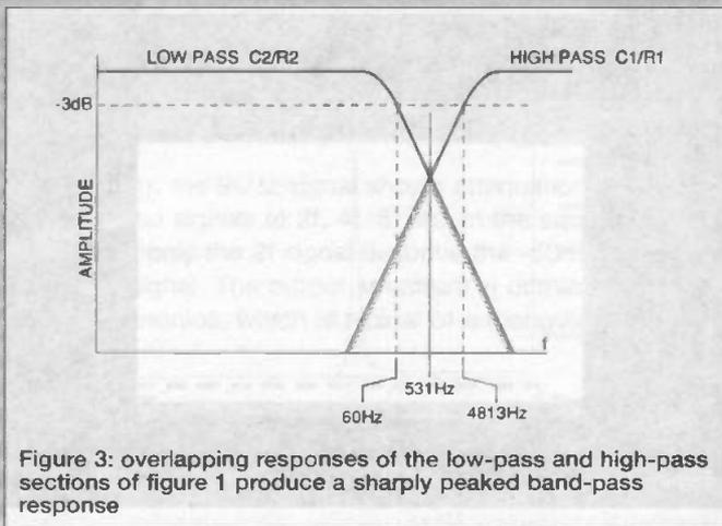
Figure 3: overlapping responses of the low-pass and high-pass sections of figure 1 produce a sharply peaked band-pass response
