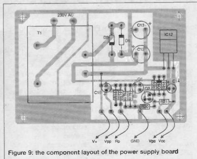
Figure 9: the component layout of the power supply board
