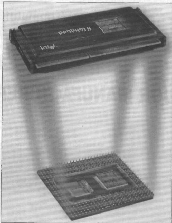
The Pentium II's write-combining technology, which combines multiple writes to one region of memory (for example, a video controller frame buffer) declared as WC type in a single burst write operation, can be used to get very high graphics I/O performance.
