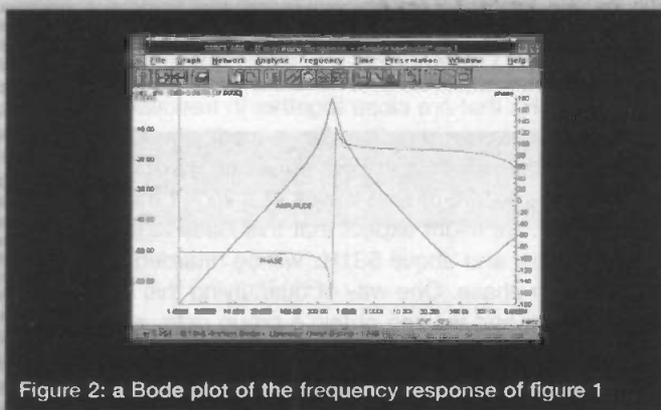
Figure 2: a Bode plot of the frequency response of figure 1
