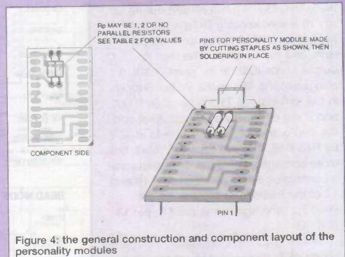
Figure 4: the general construction and component layout of the personality modules
