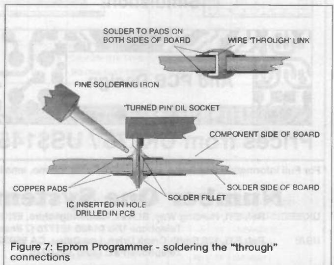
Figure 7: Eprom Programmer - soldering the "through" connections
