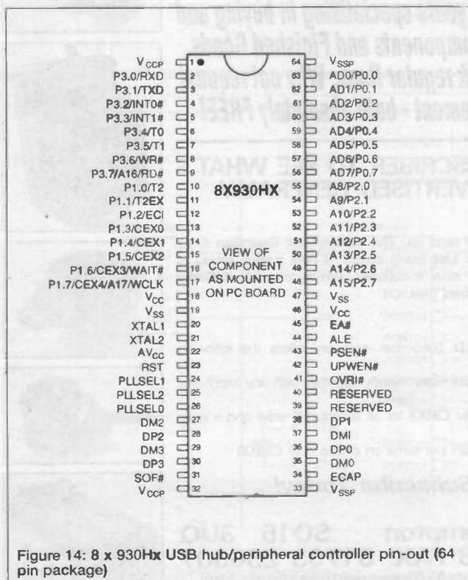
Figure 14: 8 x 930Hx USB hub/peripheral controller pin-out (64 pin package)
