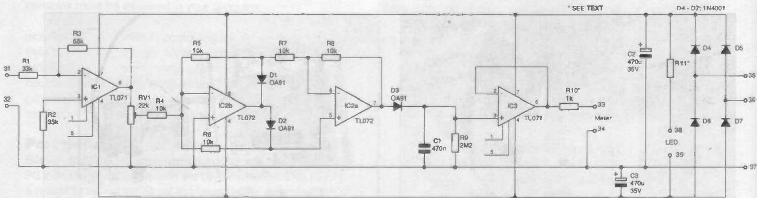
Figure 1: the circuit of the Peak Reading VU meter with power supply
