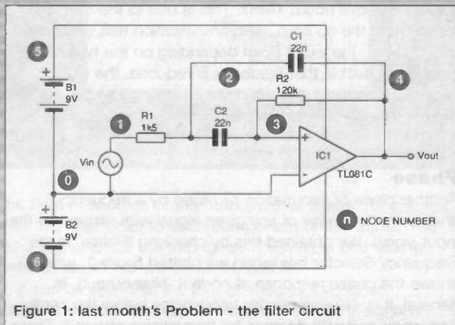
Figure 1: last month's Problem - the filter circuit
