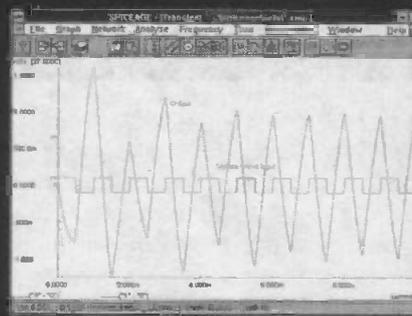
Figure 8: transient analyses of input and output demonstrate what the filter does to a square-wave signal
