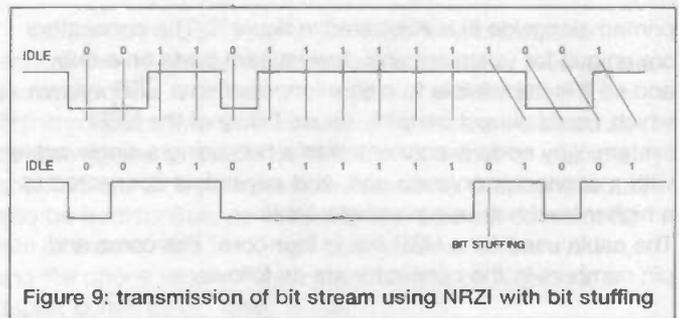
Figure 9: transmission of bit stream using NRZI with bit stuffing
