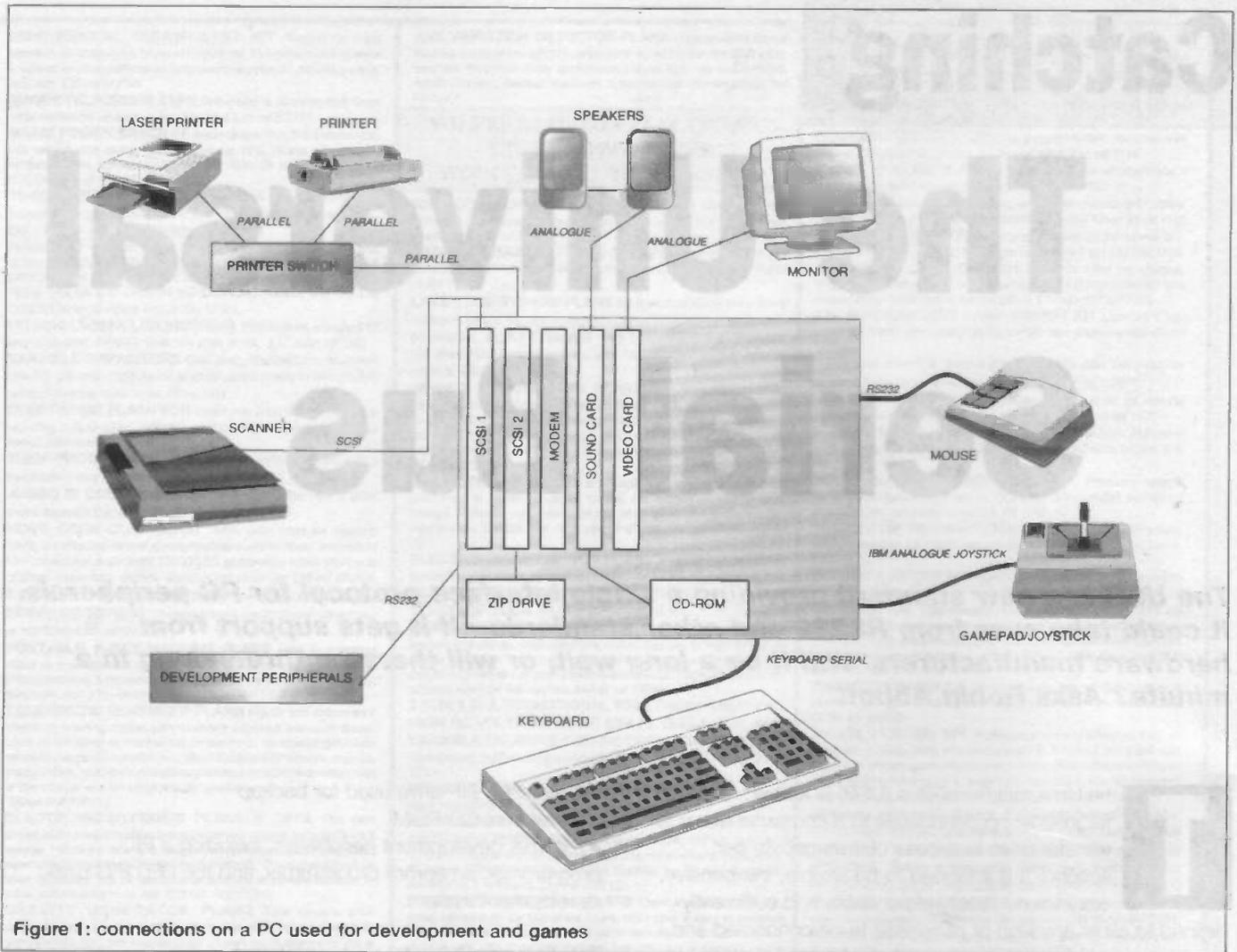
Figure 1: connections on a PC used for development and games
