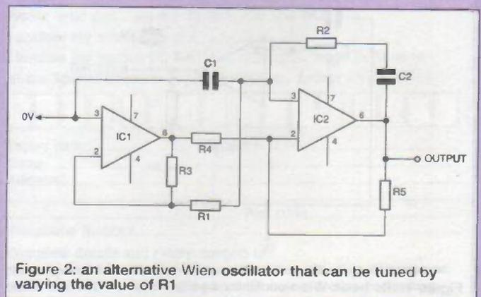
Figure 2: an alternative Wien oscillator that can be tuned by varying the value of R1
