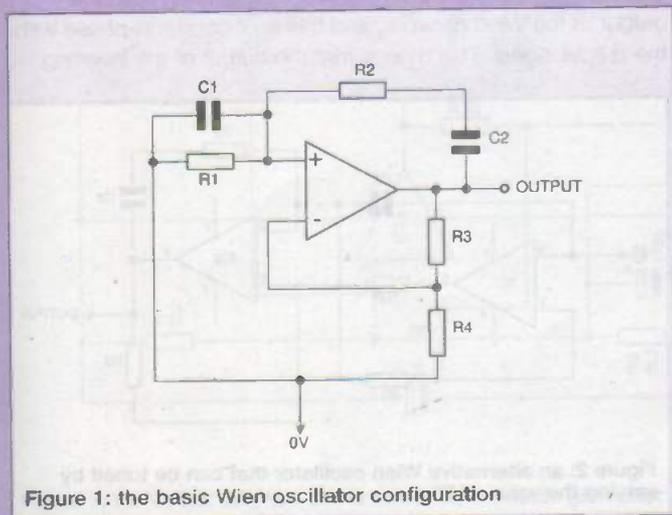
Figure 1: the basic Wien oscillator configuration
