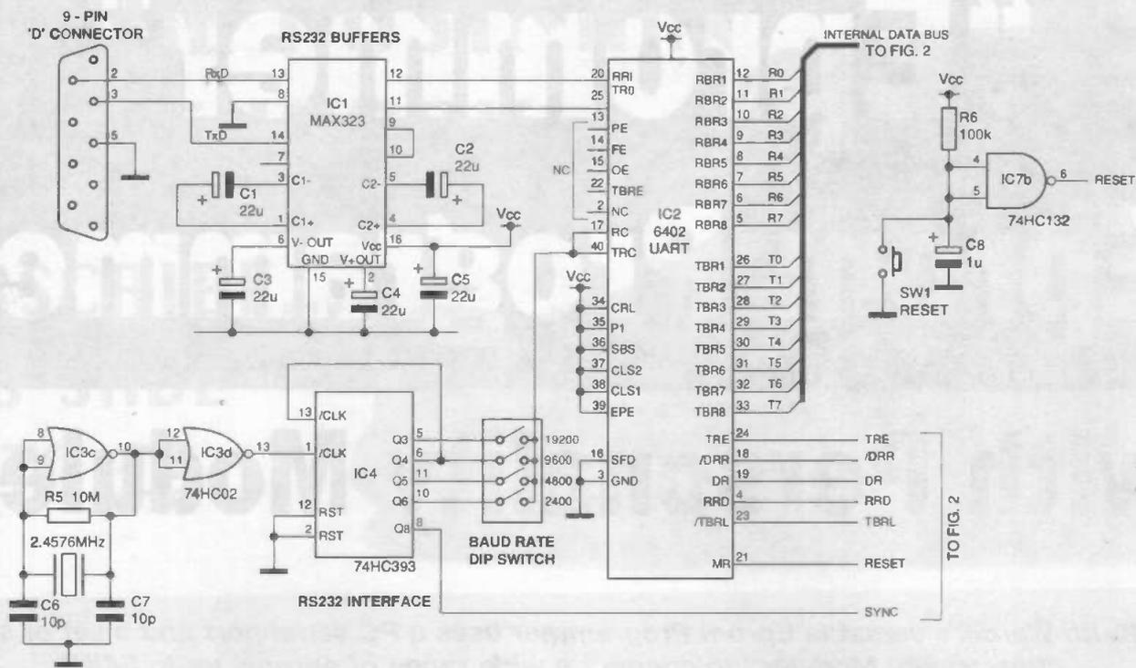
Figure 1: the Eprom Programmer serial interface circuit
