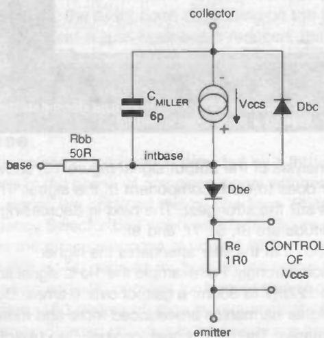
Figure 11: the 'nnp' transistor model is basic but quick-running
