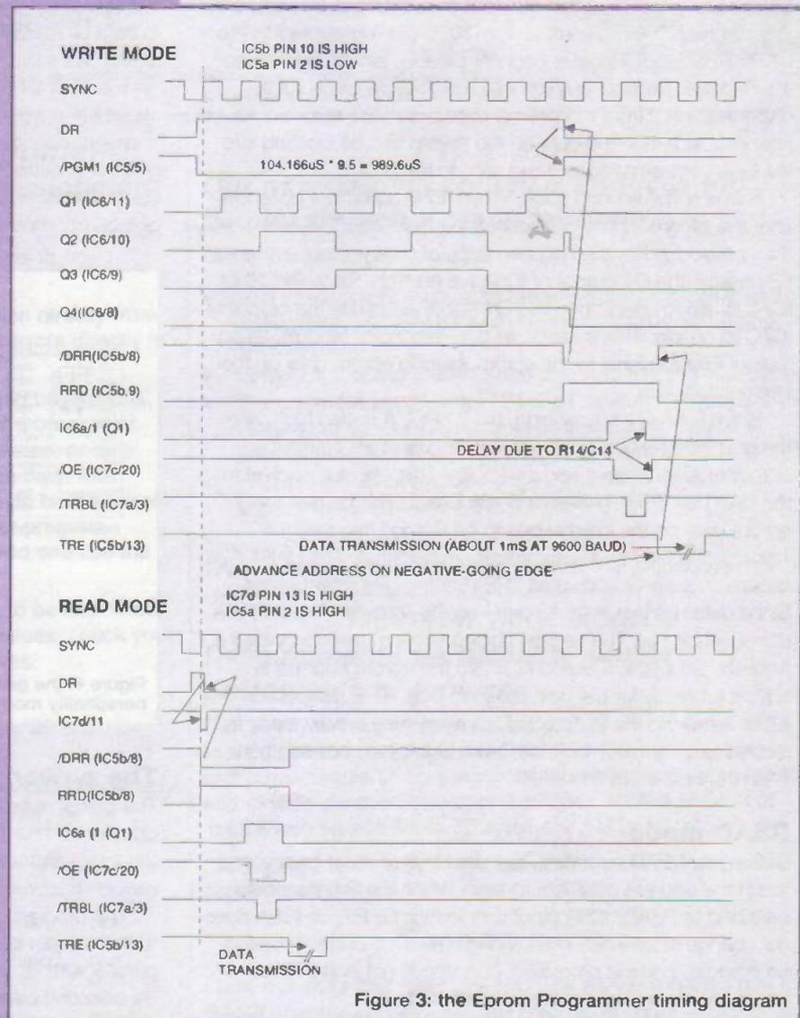
Figure 3: the Eprom Programmer timing diagram
