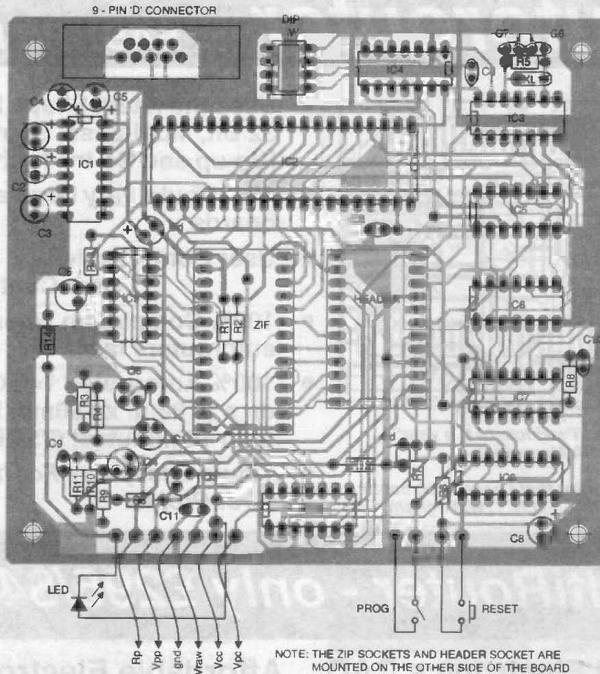
Figure 6: the component layout of the main board
