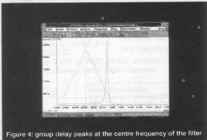
Figure 4: group delay peaks at the centre frequency of the filter
