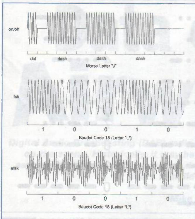
Figure 2: on-off keying (Morse) contrasted with frequency shift keying (Baudot) and audio frequency shift keying (Baudot). The frequencies are no typical, and have been chosen to stress the differences.
