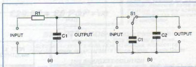
Figure 2: (a) conventional C-R low-pass filter and (b) the switched capacitor equivalent
