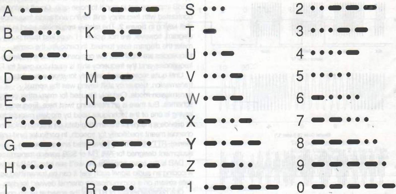
Figure 1: the Morse code alphabet, showing the relative symbol lengths
