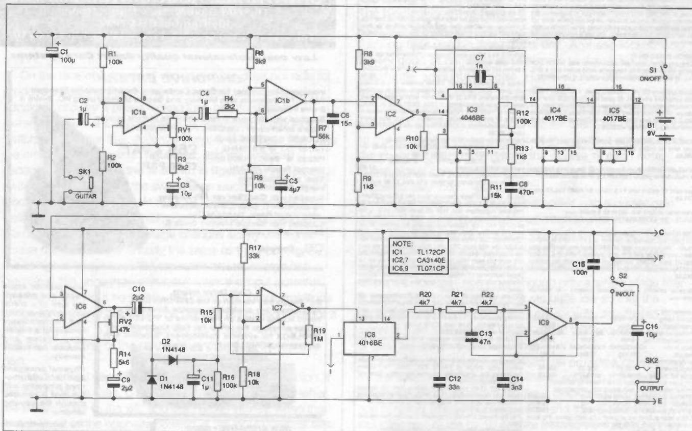
Figure 4: the circuit of the Tracking Filter Effects Unit
