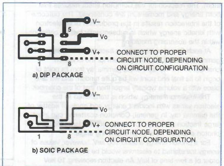
Figure 10: a) standard connection configurations: b) corresponding board layouts for input guard for OPA129
