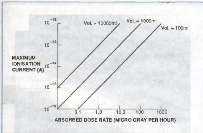
Figure 6: calculated values of maximum collected current for 'perfect' ionisation chambers of different volume as a function of absorbed dose rate in micro Gy per hour
