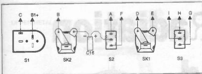
**Figure 8: details of the hard wiring (use in conjunction with figure 6)**
