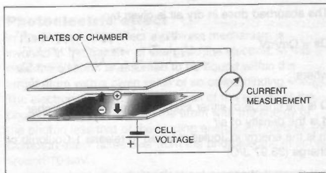
Figure 2: the basic design of ionisation chamber
