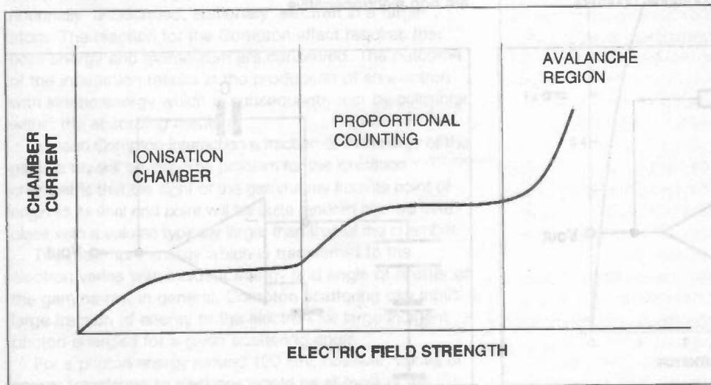
Figure 3: response of ionisation chamber as a function of established electric field. At increasing field value the chamber enters a region of proportional counting followed by an avalanche region as used in Geiger-Muller configuration
