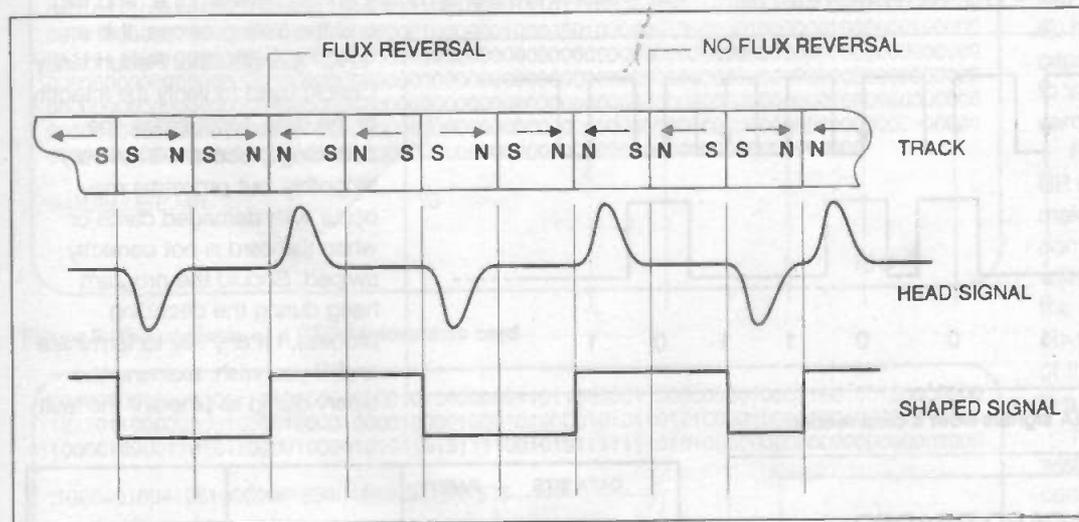
Figure 2: Reading a magnetic track
