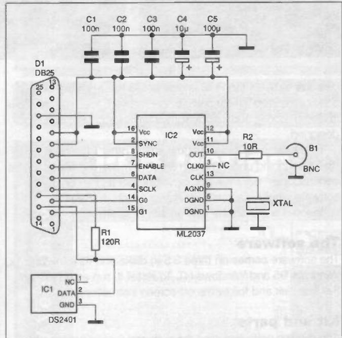
Figure 1: the circuit of the sinewave generator
