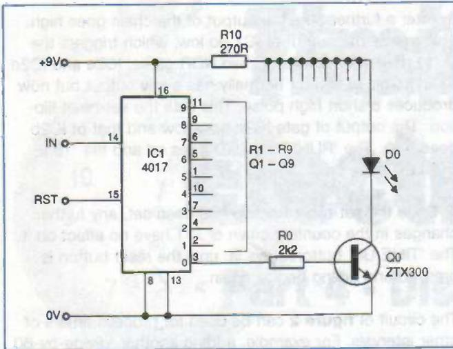
Figure 4: a process timer with up to 10 LEDs in its display. D1 - D9 are at top right.
