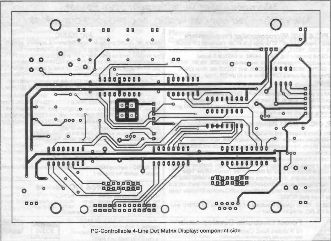
PC-Controllable 4-Line Dot Matrix Display: component side
