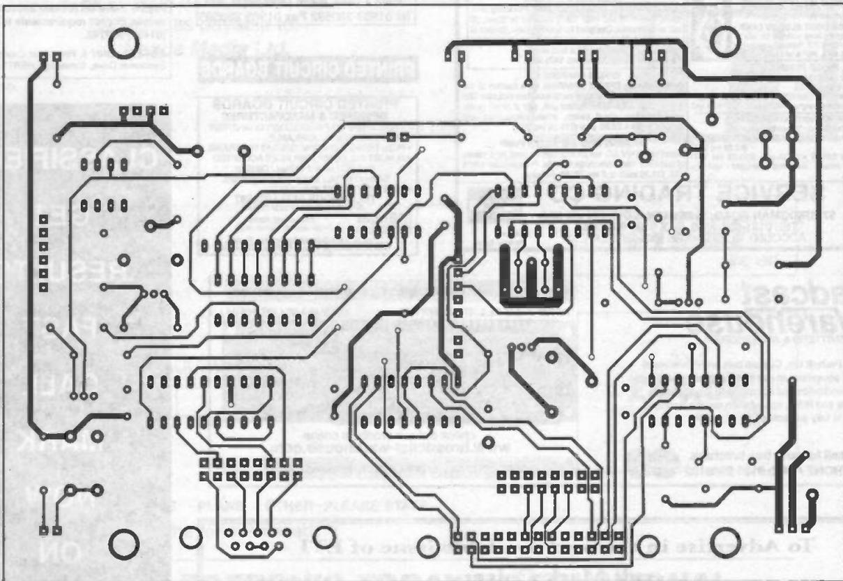
PC-Controllable 4-Line Dot Matrix Display: track side
