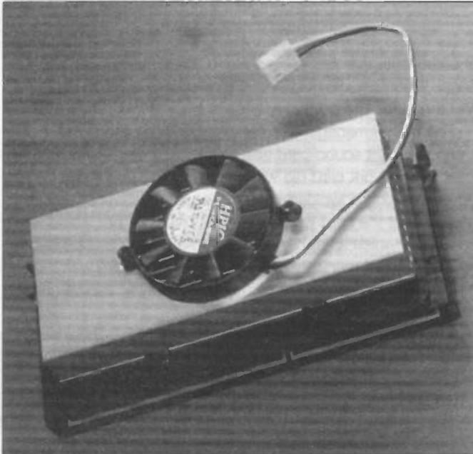
The CPU cooler mounded on the Pentium II CPU module
