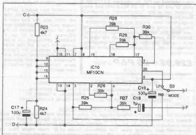
Figure 5: The circuit of the switched capacitor filter
