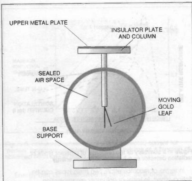
Figure 1: the basic structure of gold leaf electroscope
