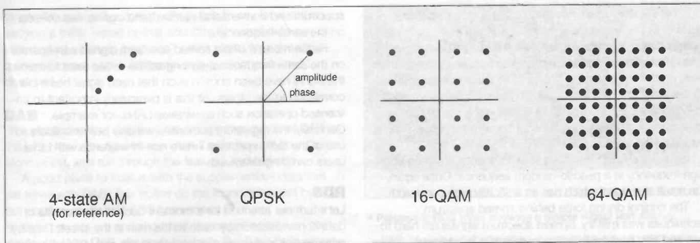
Figure 6: A common technique of summarising the amplitude and phase combinations is with a constellation diagram in which each combination is a vector, the length of which is the amplitude and the angle, the phase. Constellation diagrams using a vector with length = amplitude and angle = phase, for typical QPSK, 16QAM and 64QAM systems. The constellation of a four-state amplitude modulated signal is also shown for reference.
