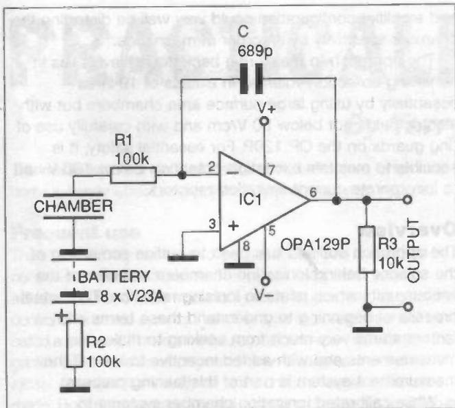
Figure 11 : circuit diagram of the ionisation chamber and associated electronics
