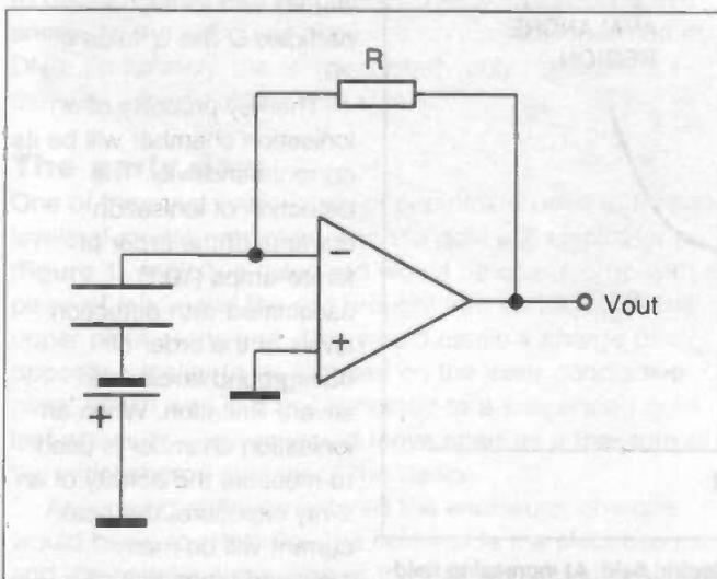
Figure 5a: the basic design of charge integration circuit
