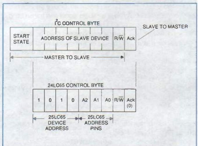
Figure 2: the control byte for the 24LC65
