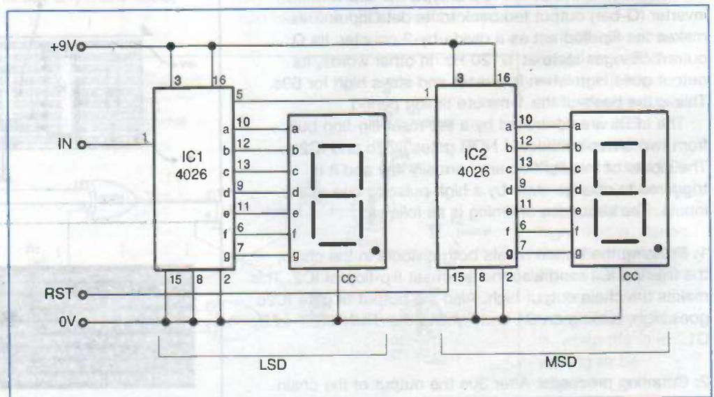
Figure 5: an elapsed-time timer with a two-digit display
