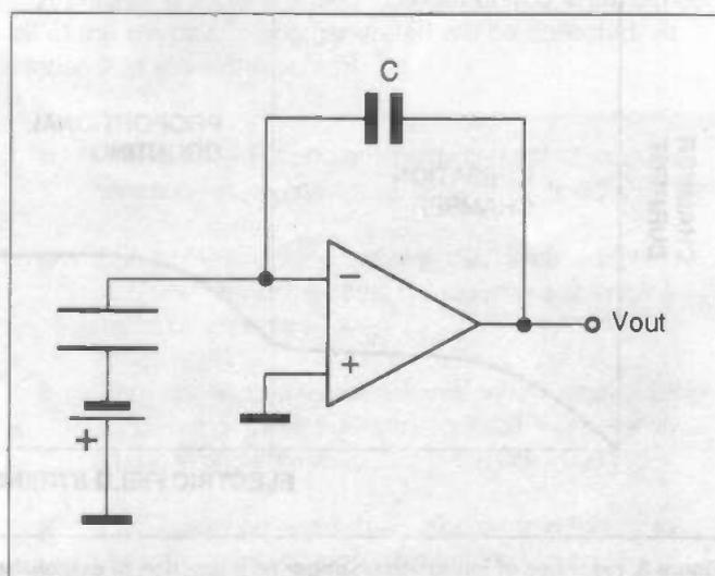
Figure 5b: the basic design of current to voltage converter circuit
