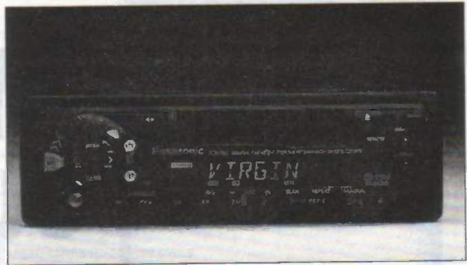
A Panasonic RDS tuner showing a simple digital text display
