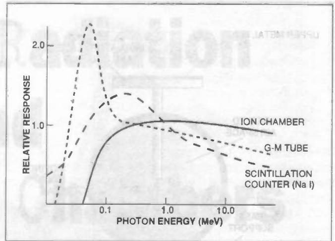
Figure 4: a summary of the response of different types of radiation detector as a function of photon energy
