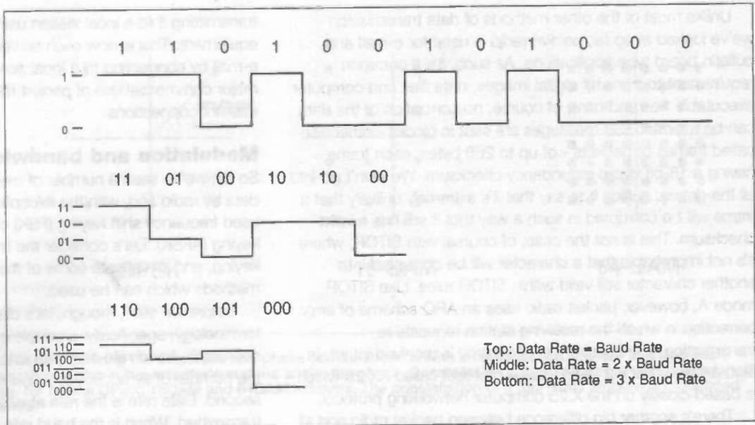
Figure 4: different applications of "data rate" and "baud rate"
