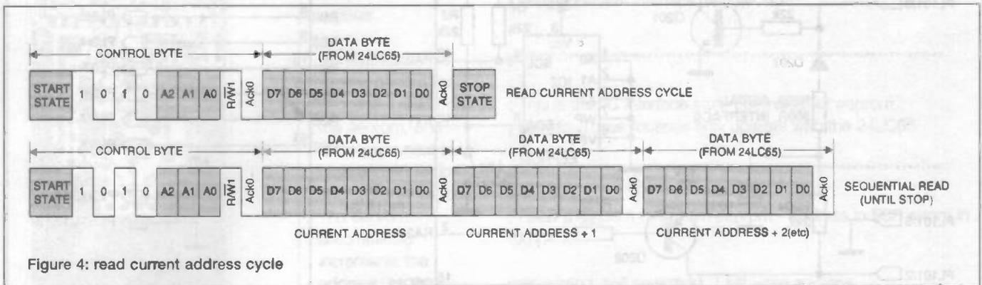
Figure 4: read current address cycle
