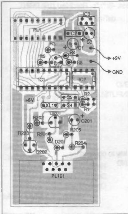
Figure 8: the component layout of the PIC card
