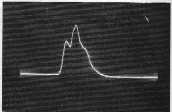
The trace produced by a 2.6 kHz ceramic filter and its matching transformers with the probe gain set high and probe used with the wobulator. The comparisons suggested confirm the linearity of the probe when its gain is set high and also reveal the way in which the shape of the IF passband is largely determined by any filter elements.
