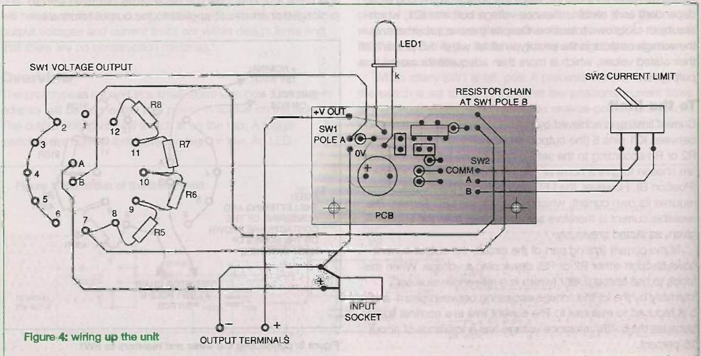
Figure 4: wiring up the unit
