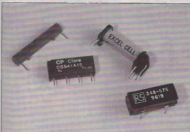
Left to right: encapsulated reed switch; single in line (sil) reed relay; stand-type reed relay; reed relay in dual in line (dil) package
