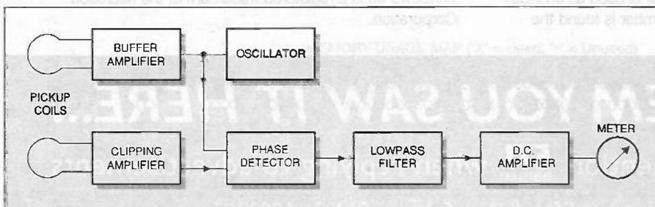
Figure 1: the block diagram of the cable detector
