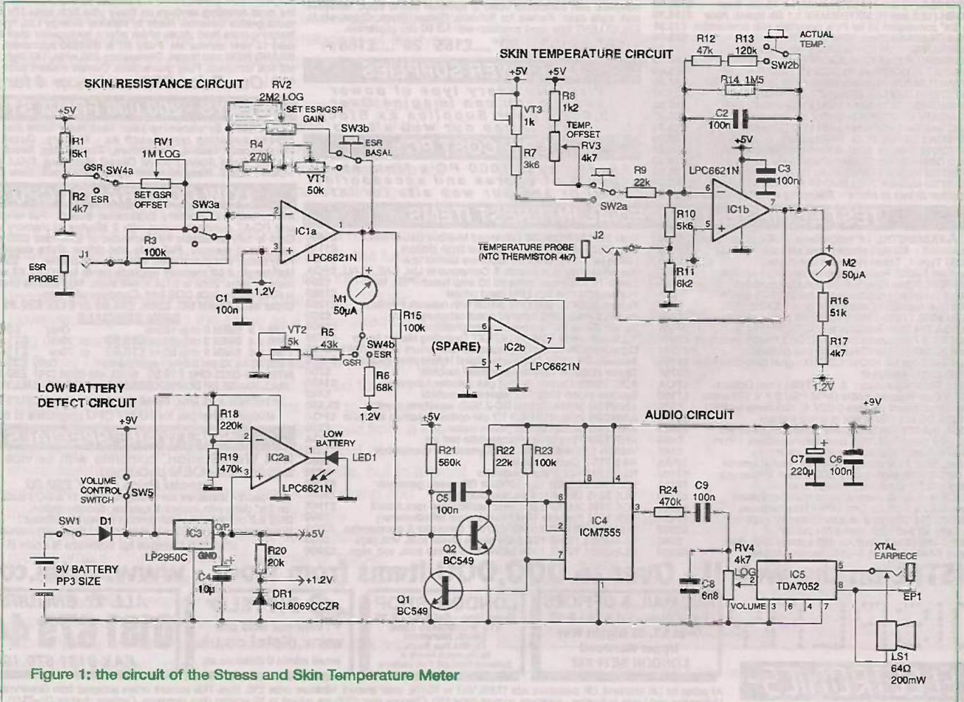
Figure 1: the circuit of the Stress and Skin Temperature Meter
