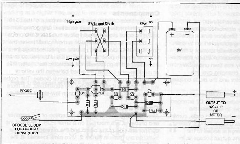
Figure 2: the component layout of the RF probe
