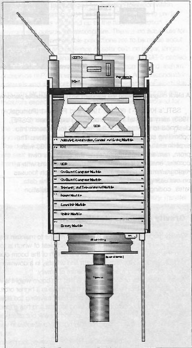
Another view of modular construction: modules stacked to form a PicoSat, built for the USAF.
