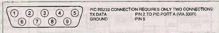
Figure 2: RS232 9-pin D connector (female) viewed from solder side
