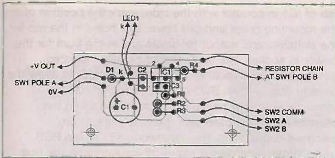
Figure 2: the component layout of the Switch Volt
