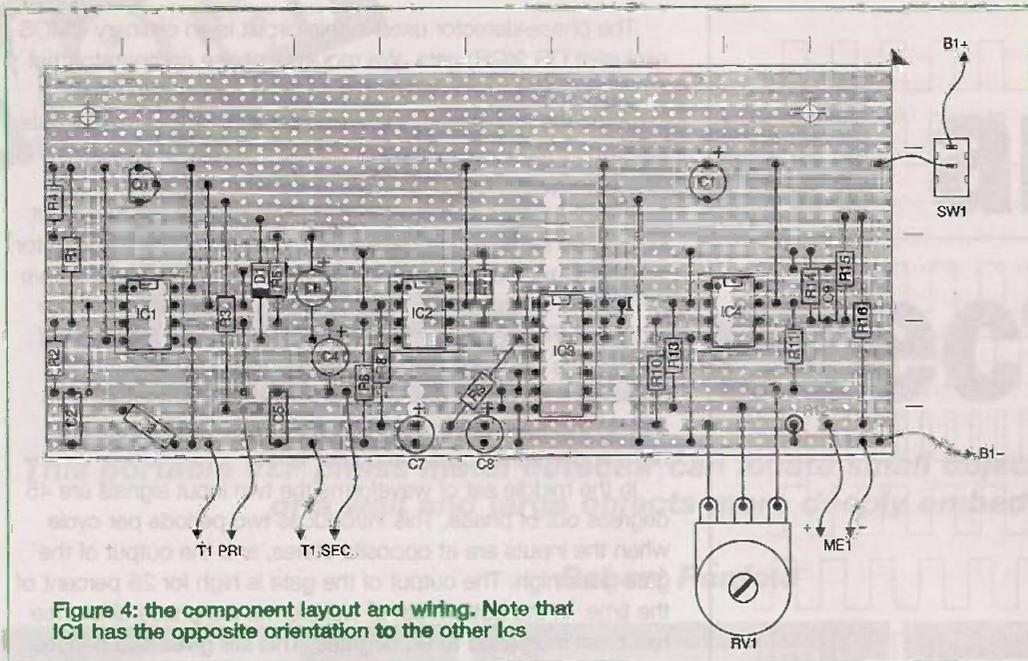
Figure 4: the component layout and wiring. Note that IC1 has the opposite orientation to the other ICs
