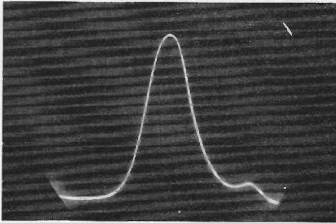
The trace produced by an inexpensive 4 kHz mechanical filter and its matching transformers, with the probe gain set high and used with the wobulator described last month. (Compare with photograph on page 56 of last month's ETI showing the response of the filter and the subsequent IF strip).
