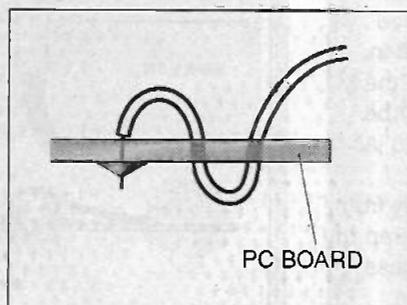
Figure 4c: wire locking on the offboard wiring pads
