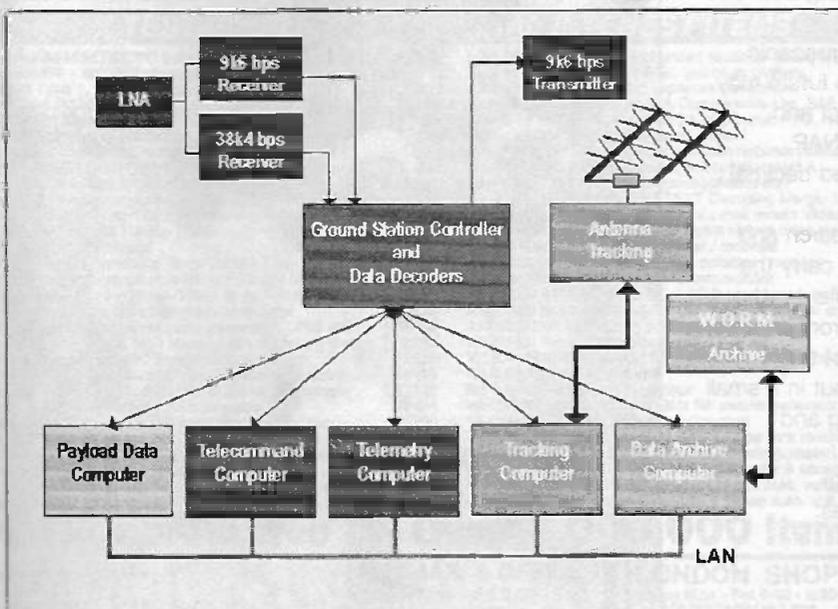
The typical SSTL mission control block diagram, showing the many computers to and from which data, control commands and programming updates are sent during a mission
