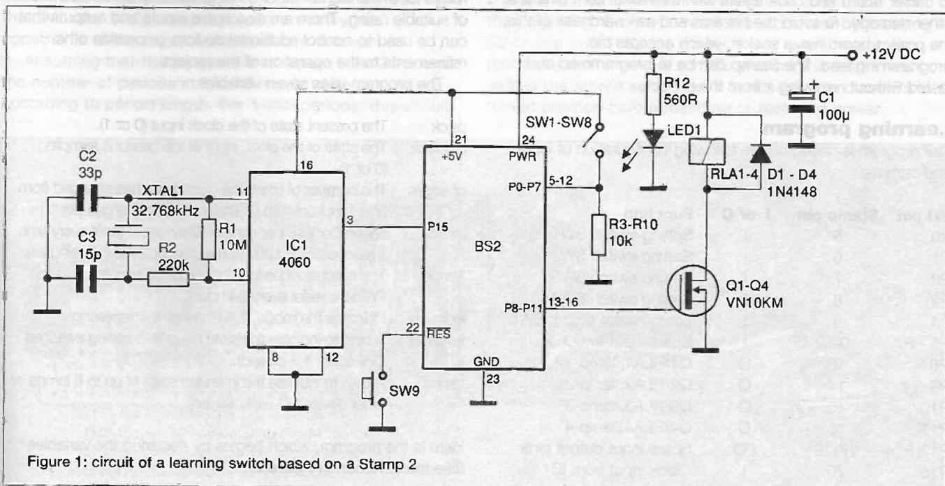
Figure 1: circuit of a learning switch based on a Stamp 2
