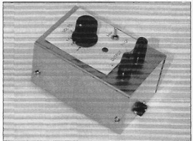
indicator both confirms that the circuit is operating, and indicates a short-circuit condition or an attempt to draw excessive current, by going out. A pair of terminals connect the circuit on test.
