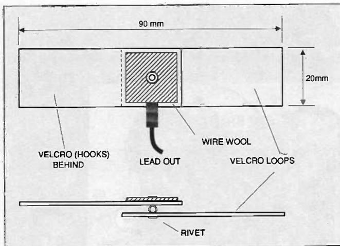
Figure 5a: construction of two ESR finger pads
