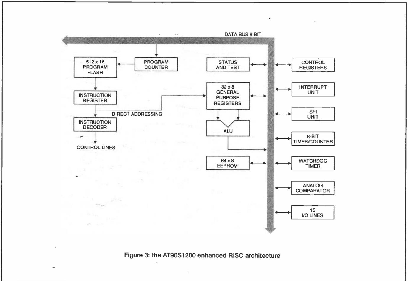
Figure 3: the AT90S1200 enhanced RISC architecture
