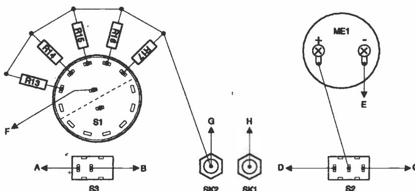
measuring very low value capacitors. On the prototype, SK1 and SK2 are one-millimetre sockets mounted about 15 millimetres apart. Many capacitors will plug straight into these, but a set of small test leads fitted with miniature crocodile clips must be made up so that small printed circuit mounting capacitors can be tested.
