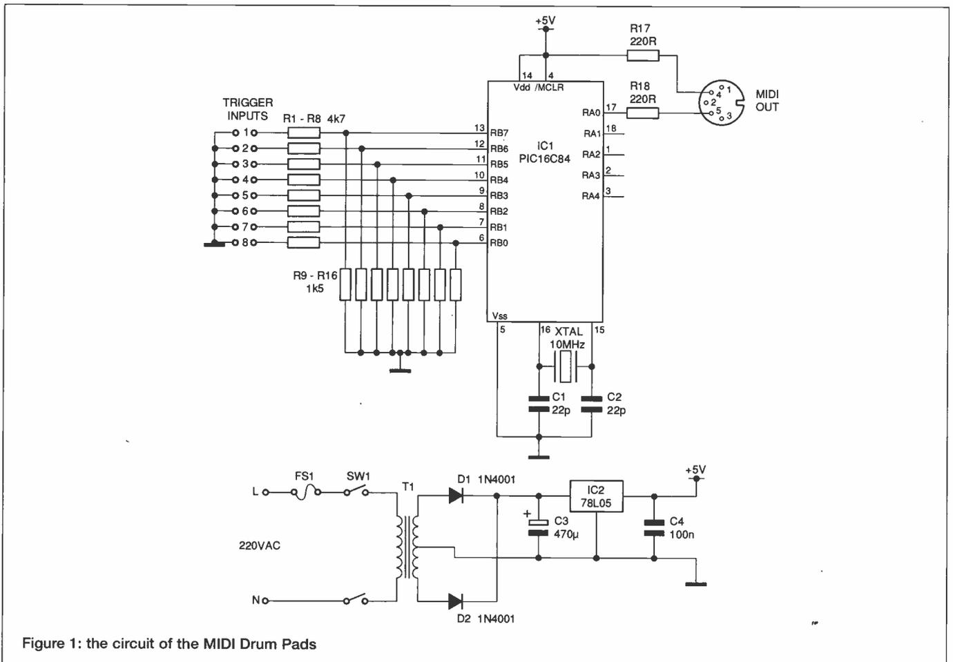
Figure 1: the circuit of the MIDI Drum Pads
