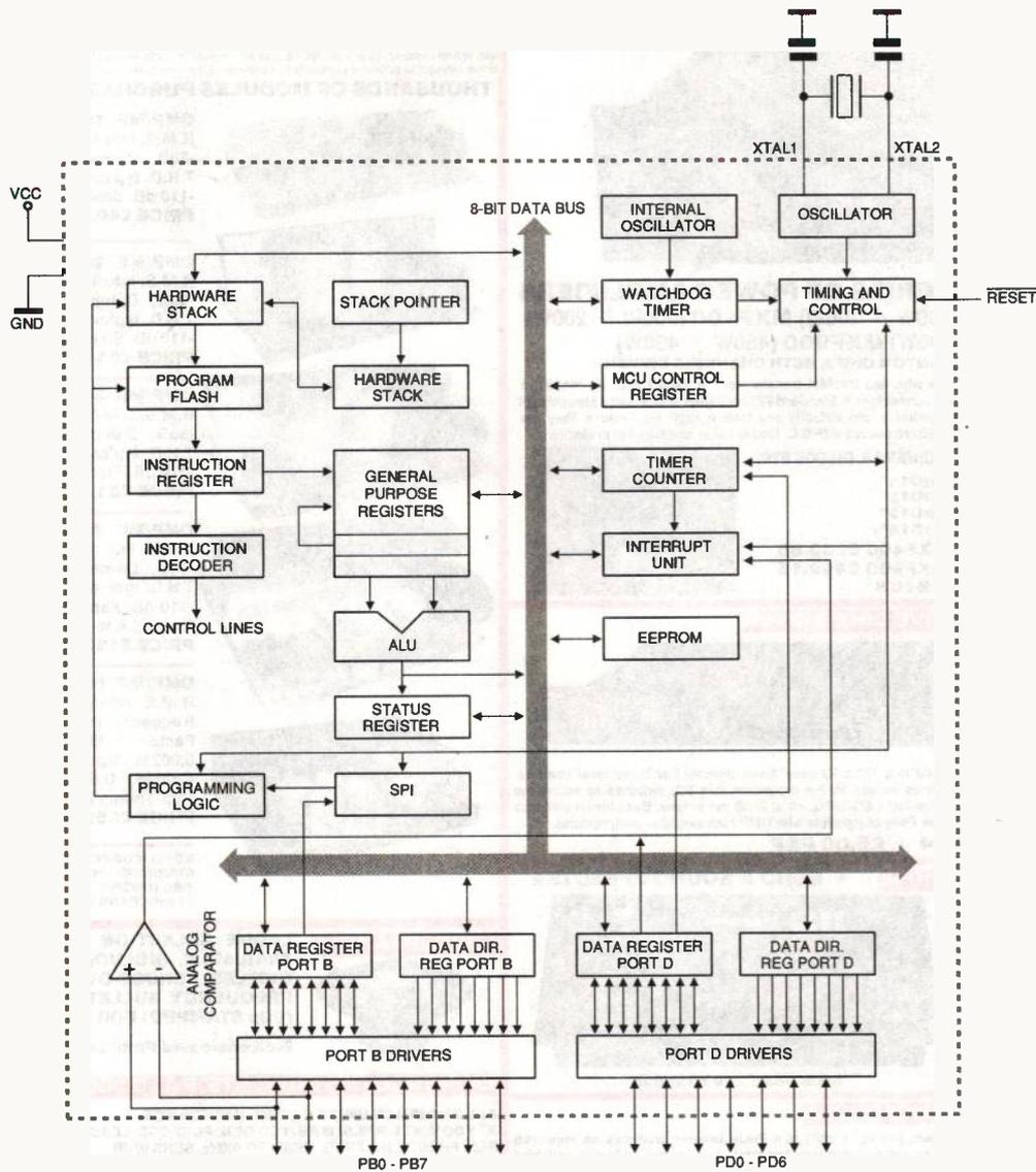
Figure 1: the block diagram of the AT90S1200
