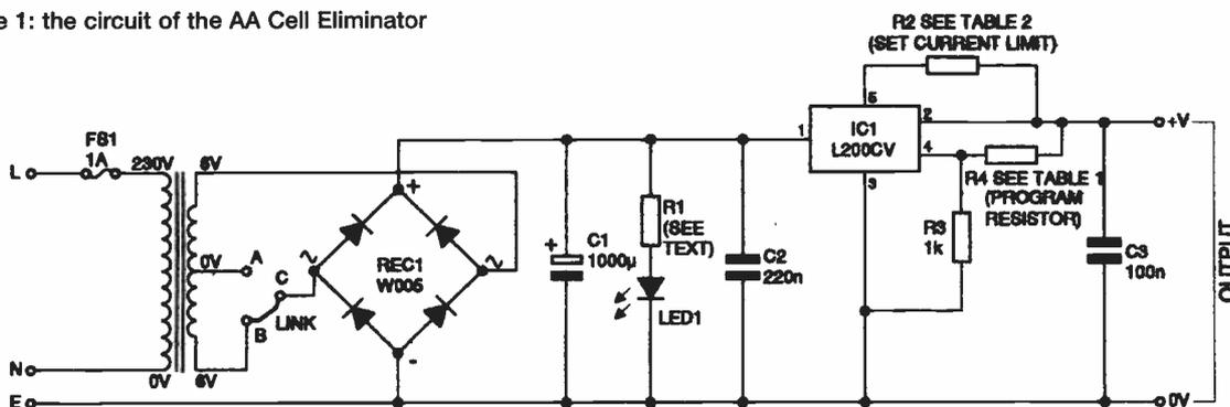
connected in series, that is, by connecting C to B as shown) or 6V (with the link connecting C to A instead - this uses only one secondary section). For equipment designed for two cells, the latter is used. For three or four cells, both secondaries will be needed. The mains earth wire is connected to the case and also runs through to the negative (0V) output terminal.
