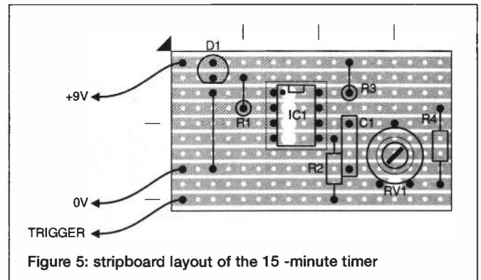
Figure 5: stripboard layout of the 15 -minute timer
