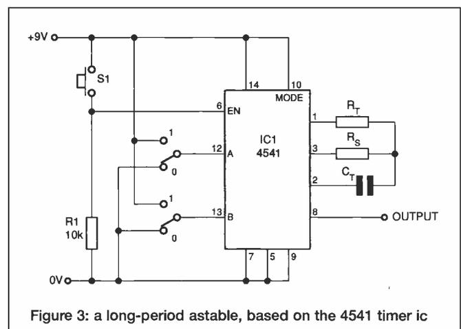
Figure 3: a long-period astable, based on the 4541 timer ic
