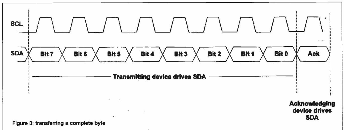
Figure 3: transferring a complete byte
