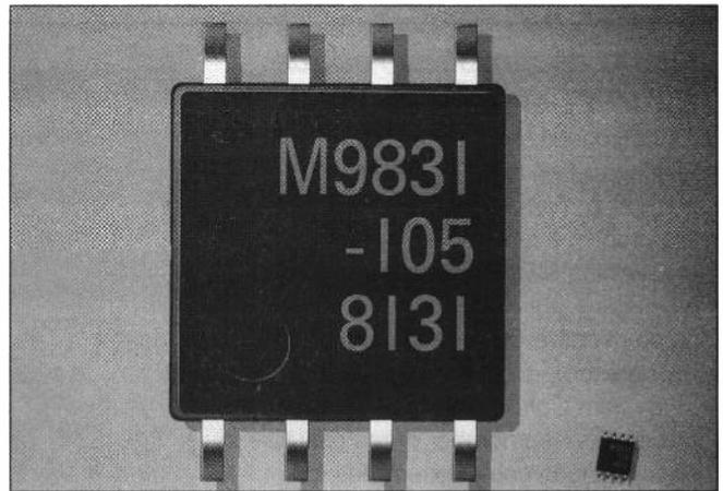
(small outline package) is 6.8 x 5mm and holds a 10-bit DAC, a low-pass filter and 384 kbits of Mask rom. The power supply ranges from 2 to 5.5 volts, offering different voltage availability for different applications.
