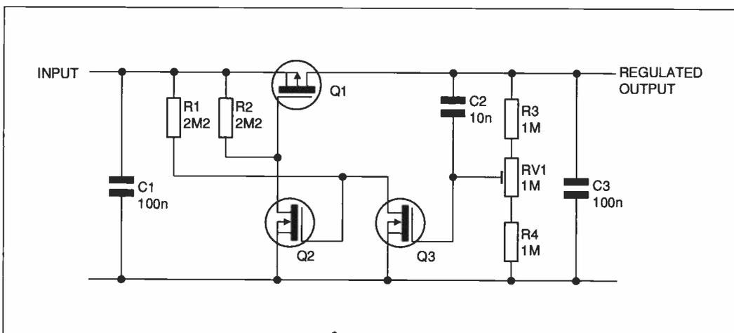
Figure 1: a very low power mosfet voltage regulator
