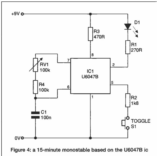
Figure 4: a 15-minute monostable based on the U6047B ic
