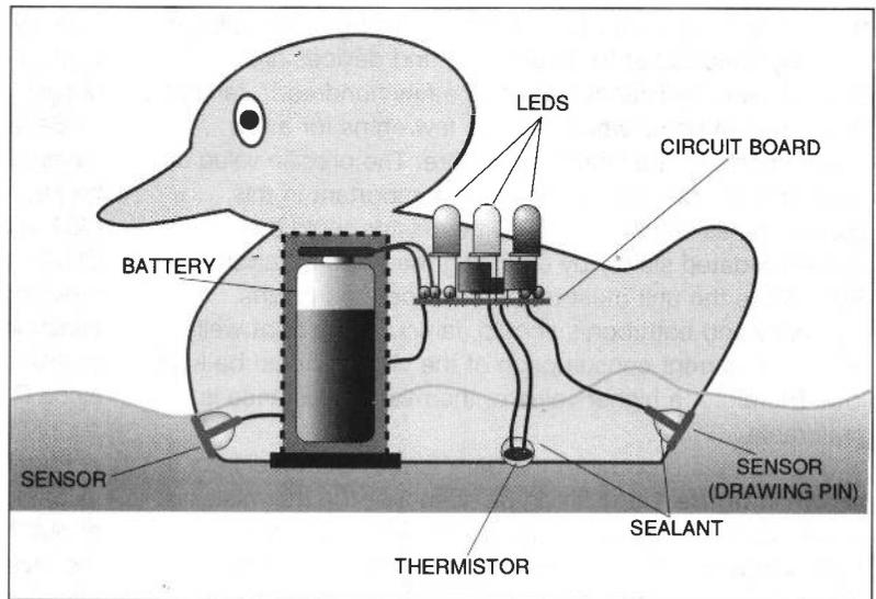
Figure 3: a suitable internal arrangement in a duck
