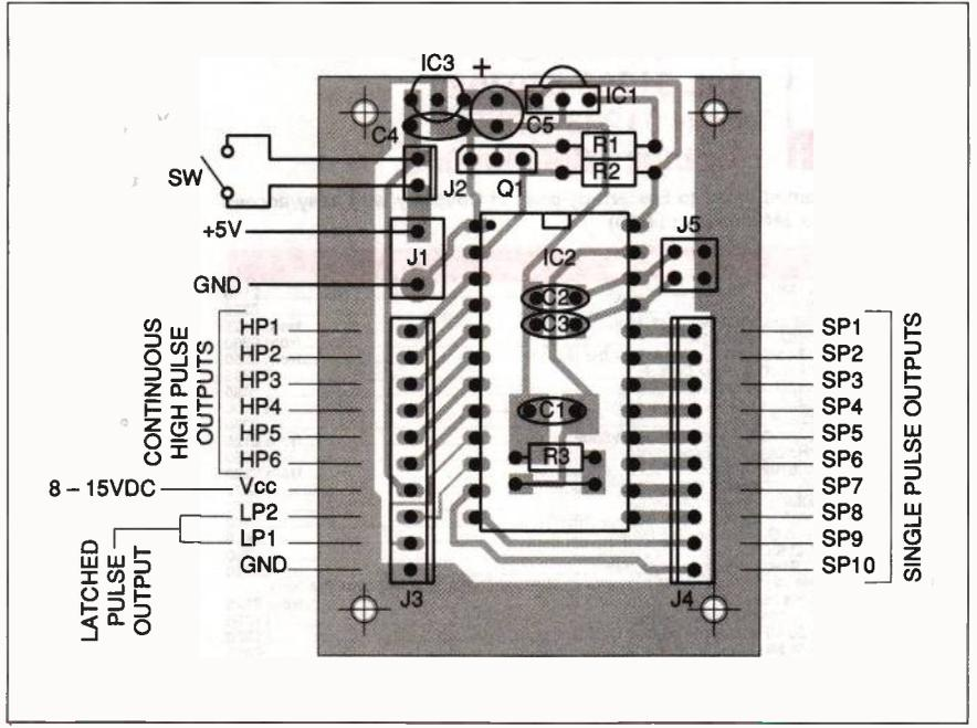
Figure 9: the handset unit with the Receiver PCB Figure 10: the component layout of the remote control receiver board
