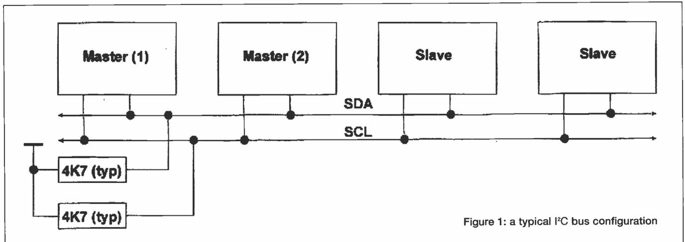
Figure 1: a typical I<sup>2</sup>C bus configuration
