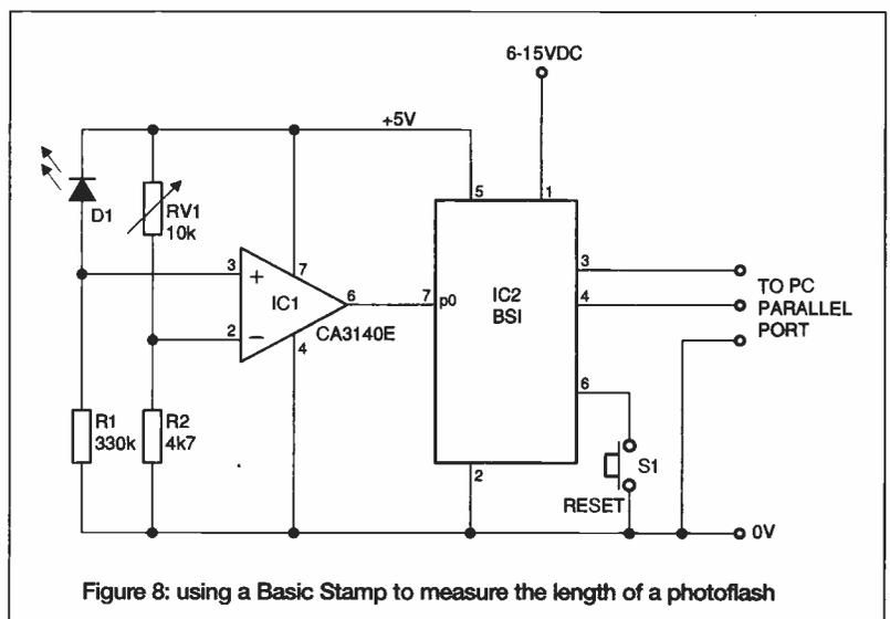
Figure 8: using a Basic Stamp to measure the length of a photoflash
