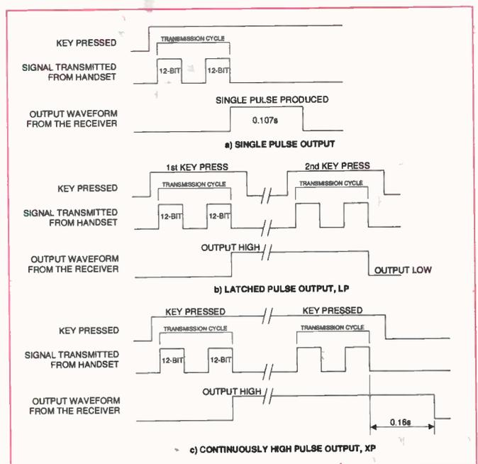
Figure 2: waveforms of the controlled outputs on the receiver board
