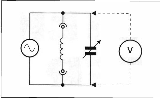
**Figure 2: method of deriving the Q factor from the magnification effect of a tune circuit:  $Q = V_{mag}/V_{in}$**
