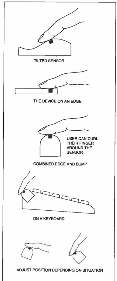
Various configurations for mounting the sensor in equipment. The sensor has a very small footprint, but is not ideal for a completely flat surface
