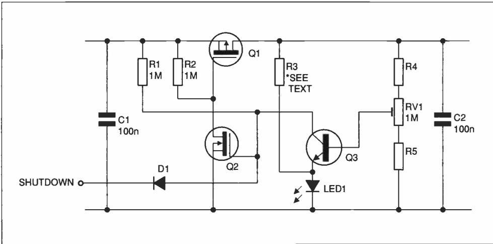
Figure 2: a low power voltage regulator with improved stability
