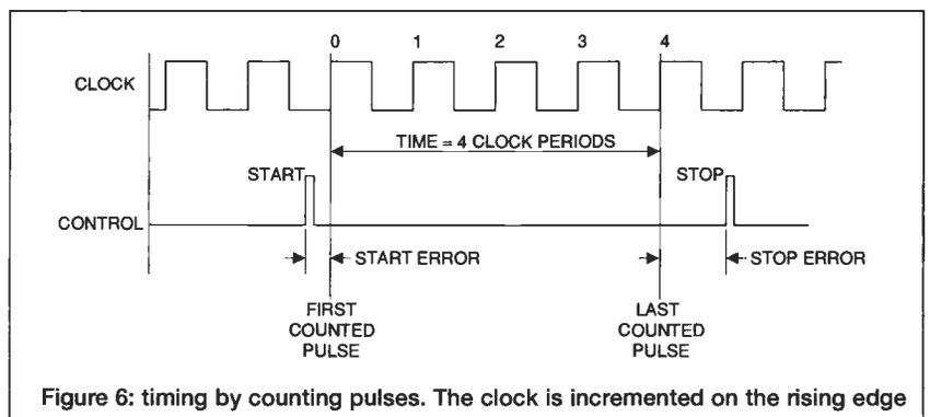
Figure 6: timing by counting pulses. The clock is incremented on the rising edge
