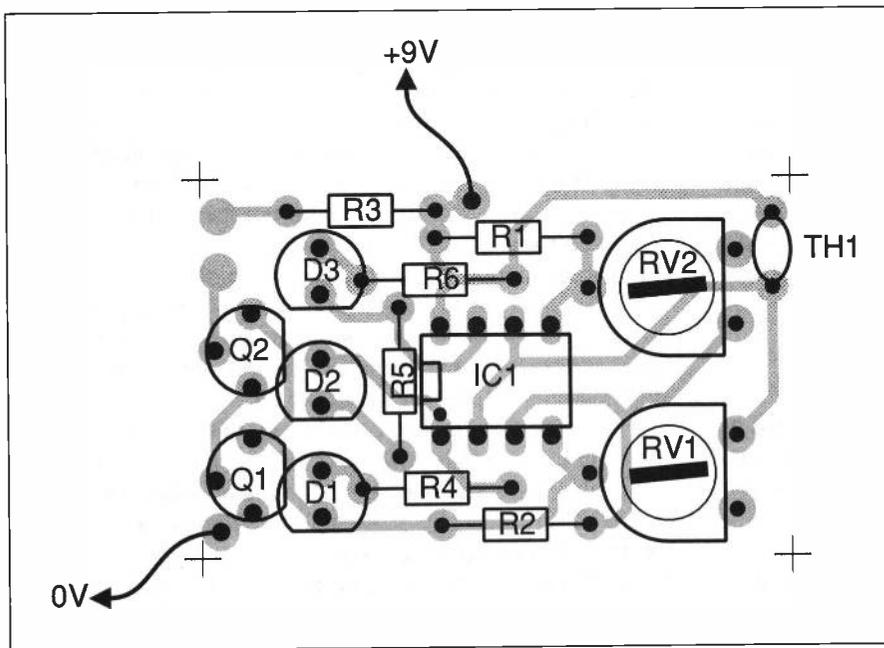
Figure 2: the component layout
