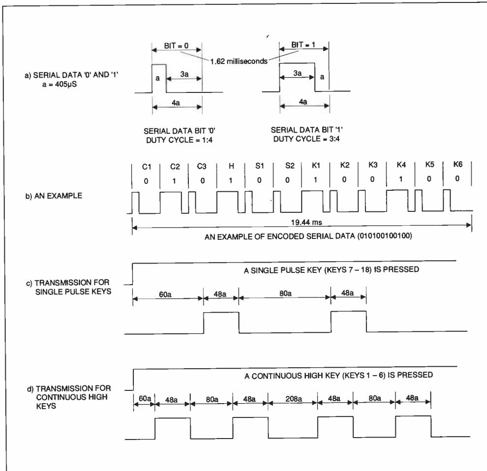
Figure 6: the format of the encoded serial data
