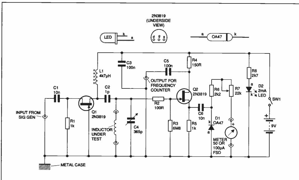
**Figure 3: the circuit of the Q meter adapter**
