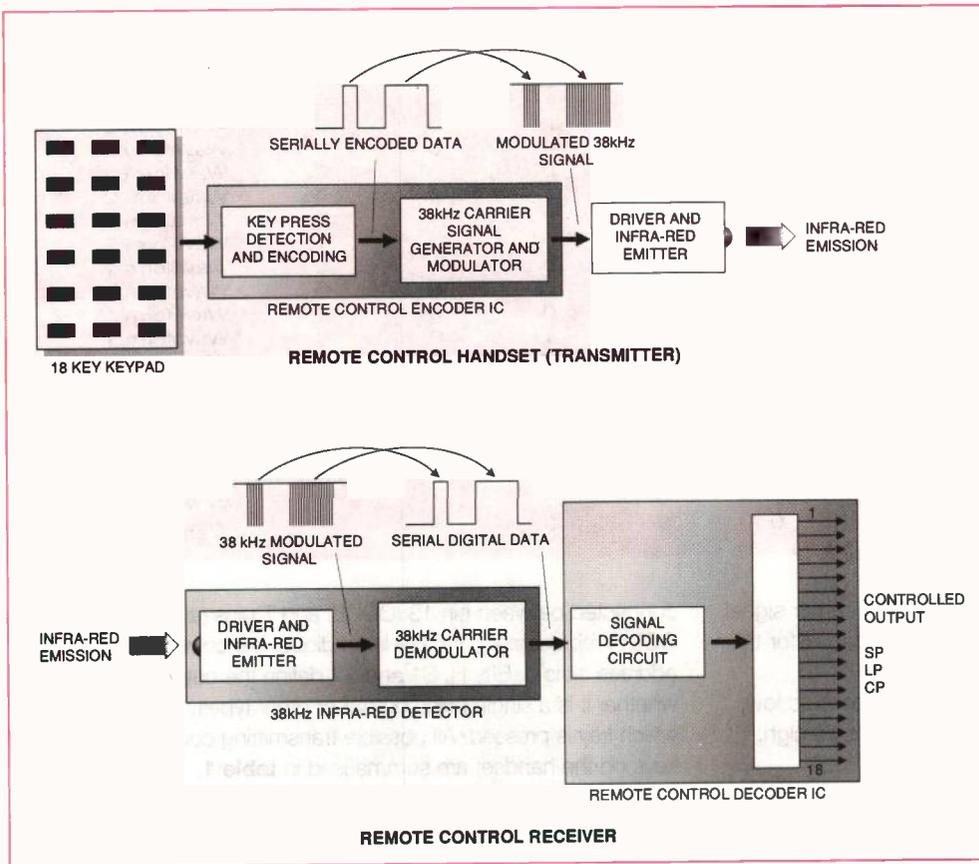
Figure 3: the principle of a typical remote control system
