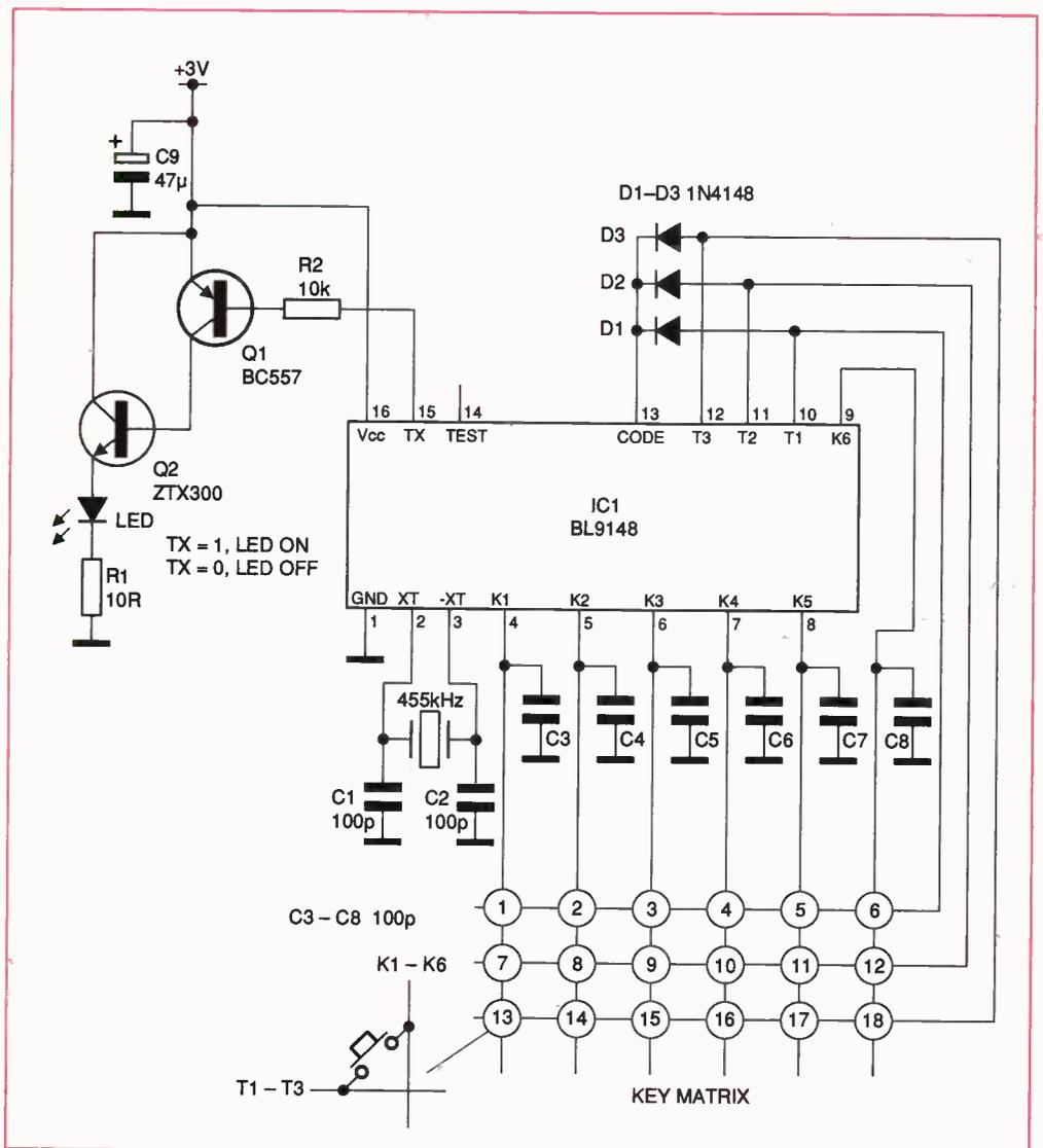
**Figure 4: the circuit diagram of the remote control transmitter**
