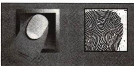
The image presented to the sensor is captured. An on-board 8-bit ADC digitises the array output which is converted to a grayscale image
