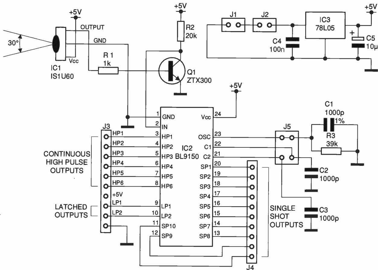
Figure 7: the circuit of the remote control receiver
