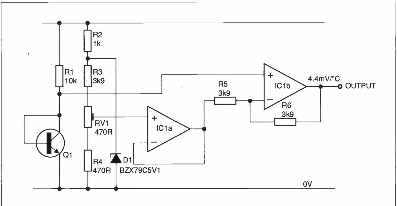
Figure 3: using a transistor as a good, low-cost temperature sensor
