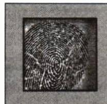
During image capture, automatic on-chip adjustments to sensitivity and gain control are made to obtain the best image. Integrated temperature and resistance sensors make it very difficult to fool the sensor
