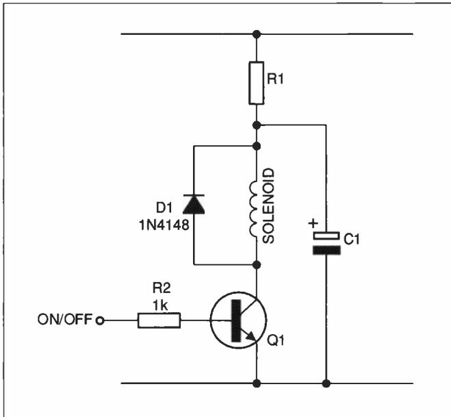
Figure 4: a simple way to reduce the power dissipated in a solenoid
