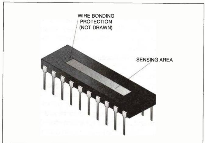
The FC15A140 FingerchipTM die chip showing the sensing area
