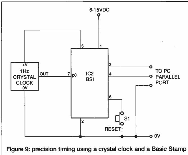
Figure 9: precision timing using a crystal clock and a Basic Stamp
