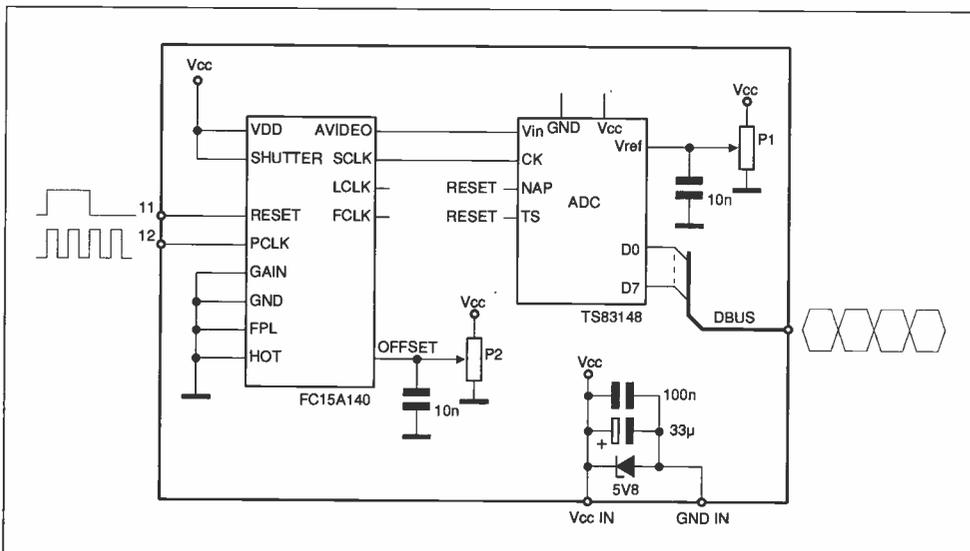
A final system implementation of the FC15A140 directly connected with the ADC, and using the rule "one clock stroke, one data". Future versions will integrate to ADC on the chip
