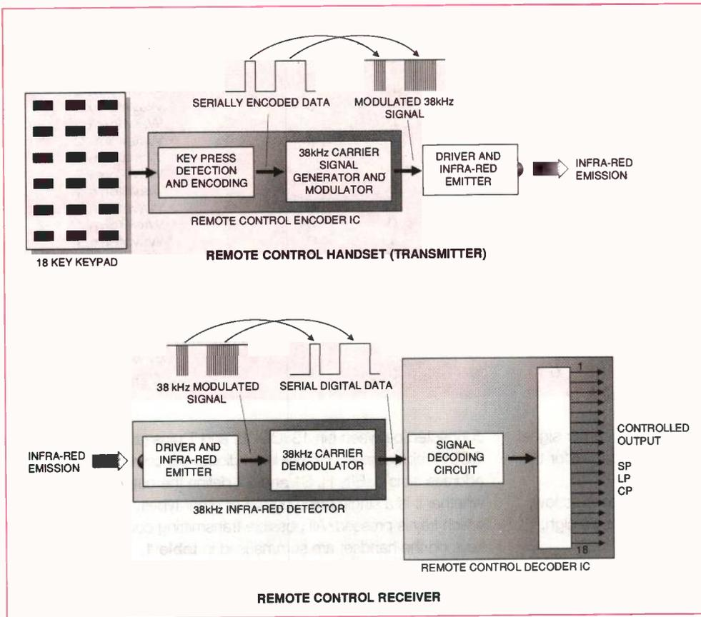
Figure 3: the principle of a typical remote control system
