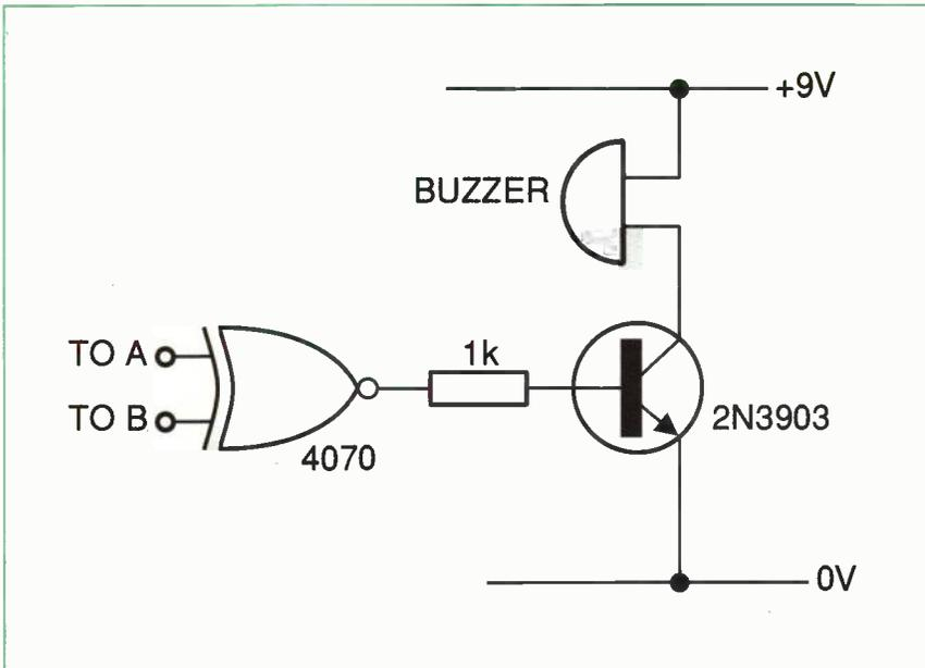
Figure 4: adding an over/under temperature alarm
