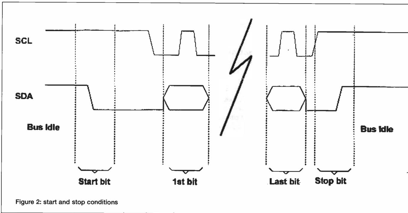
access. The slave checks the address, and if it is correct responds as defined by the master. In any transfer there will be eight bits and one acknowledgement bit sent. The acknowledgement bit is always sent by the device which is reading from the bus: if the master is transferring to the slave, the slave device acknowledges; if the slave is transferring to the master, the master acknowledges.
