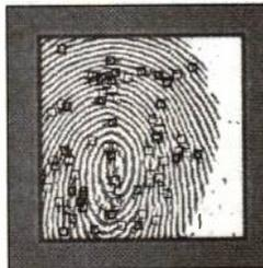
The minutia (ridge endings and bifurcations) of the fingerprint are identified. A set of minutia unique to that fingerprint is extracted and stored as a minutia template of that individual
