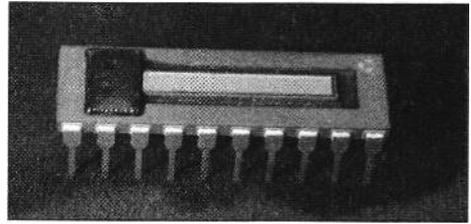
The FC15A140 Fingerchip™ with the sensor in the middle and the connections covered at the left hand end.
