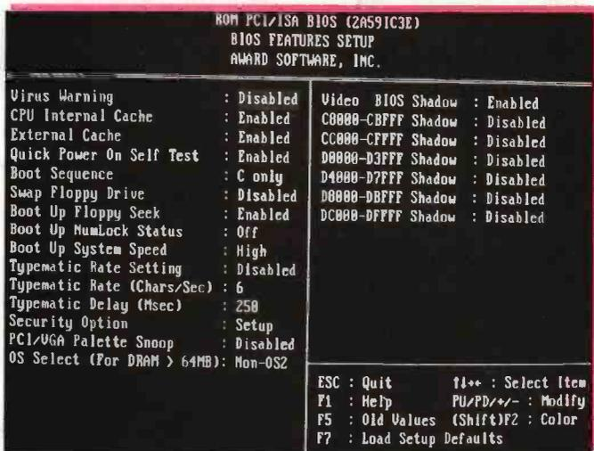
The BIOS Features Setup enables you to select the boot drives and search sequence. As with other sections of the BIOS, the default settings should give good results.
