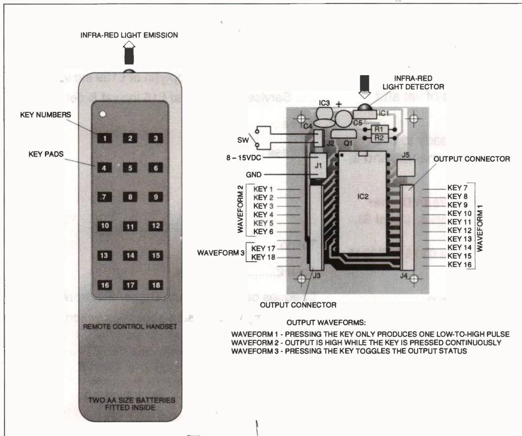
Figure 1: the 18-channel infra-red remote control system
