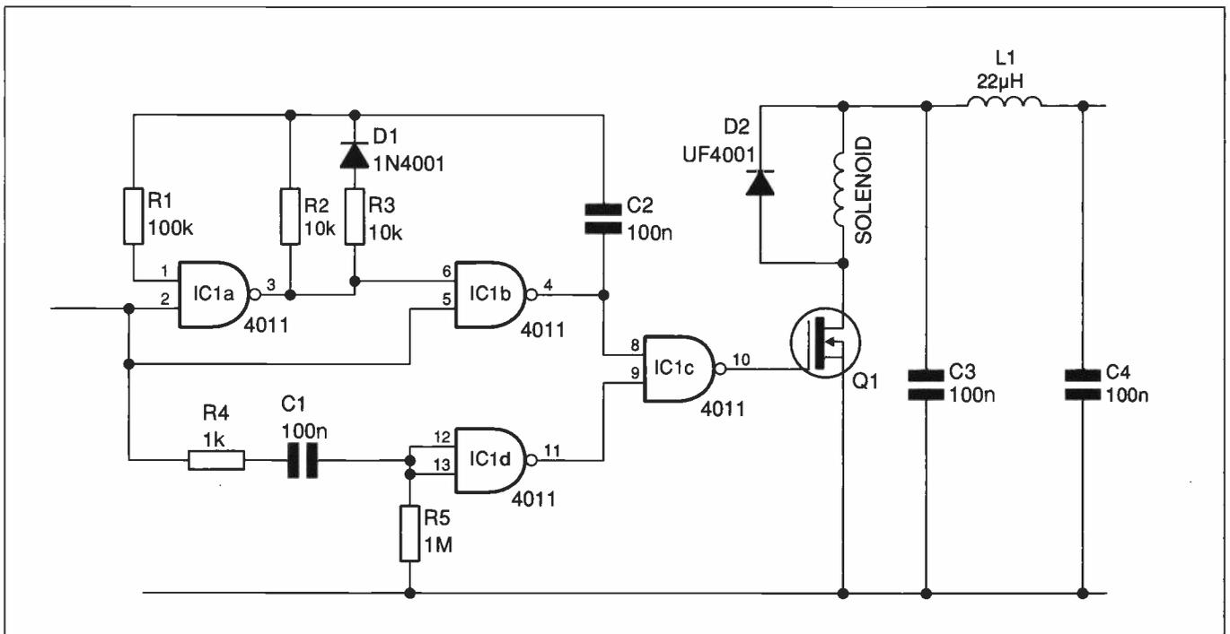
Figure 5: a way to minimise the power drawn by a solenoid where power consumption is critical
