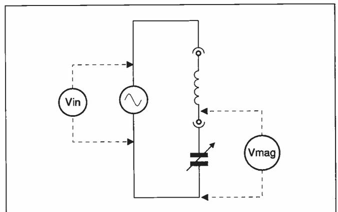
**Figure 1: method of deriving the Q factor from the selectivity of a tune circuit:  $Q = \text{resonant frequency}/\text{bandwidth at } 0.707 \text{ of } V \text{ at resonance}$**
