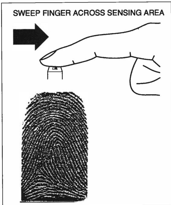
Movement of the finger across the sensing area, and the area of fingerprint imaged
