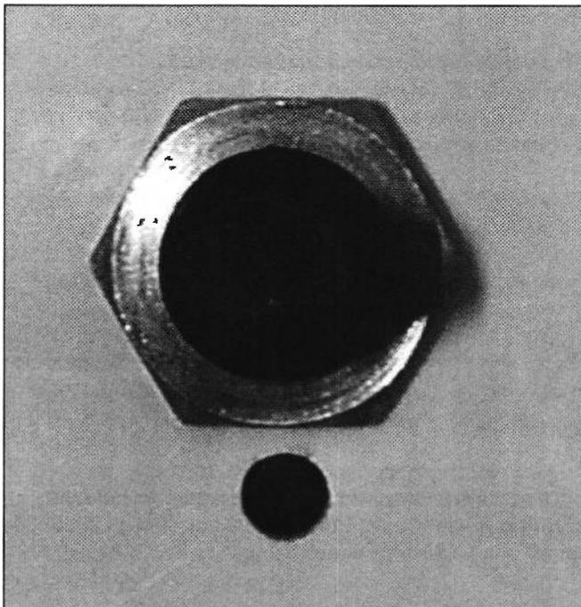
the potentiometer from rotating in use if the fixing nut worked loose and the control knob was turned hard to its limit (as happens all too easily). The whole body would then turn, and this could even result in the connecting wires breaking off. Unsecured pots work loose quite easily, and it really spoils the look and feel of a construction to have a "free floating" pot on the front panel.
