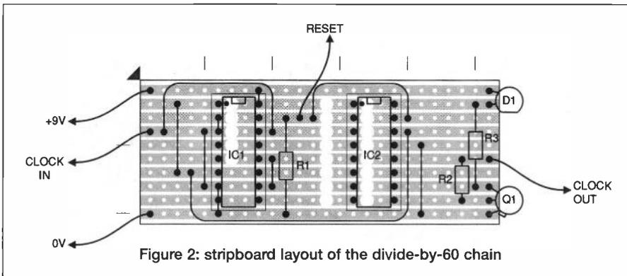
Figure 2: stripboard layout of the divide-by-60 chain
