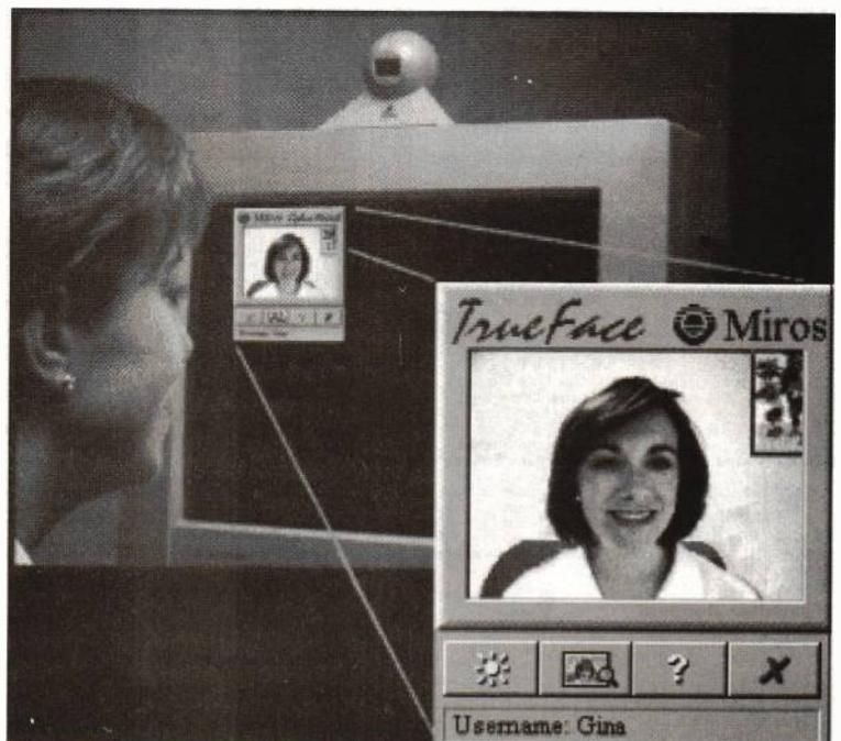
A monitor-top camera sends the image to Trueface recognition software
