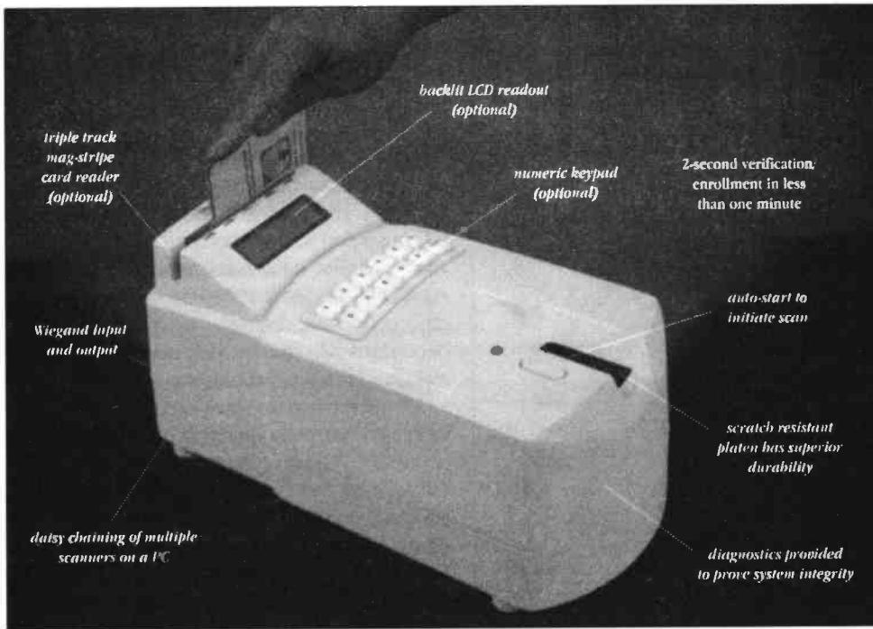
**Ultra-Scan Series 700 ID Station™ with integrated finger scan, cardswipe and keypad options**
