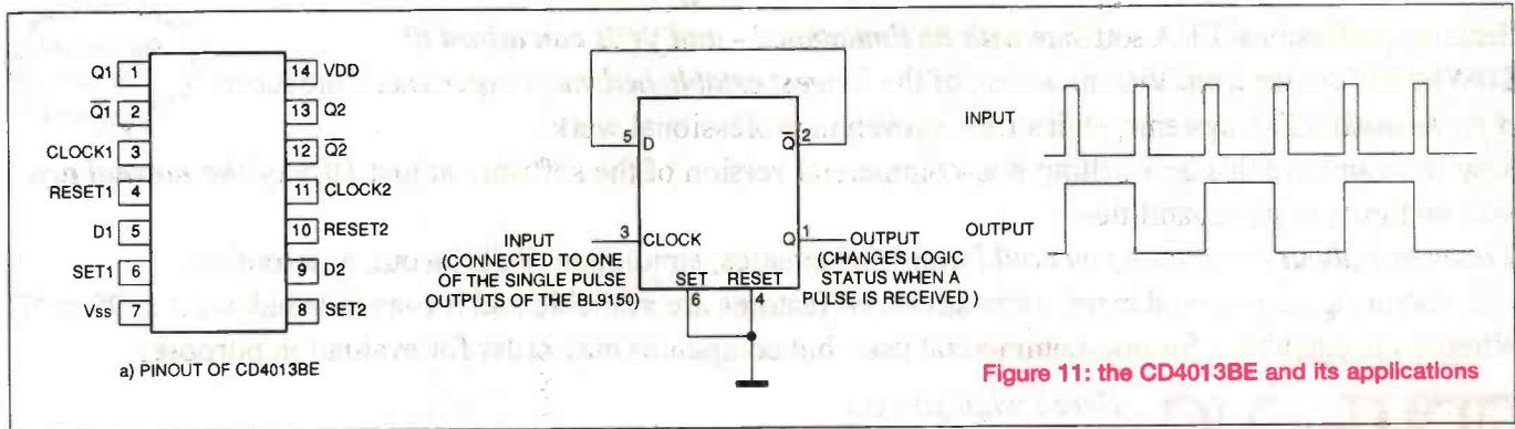
Figure 11: the CD4013BE and its applications
