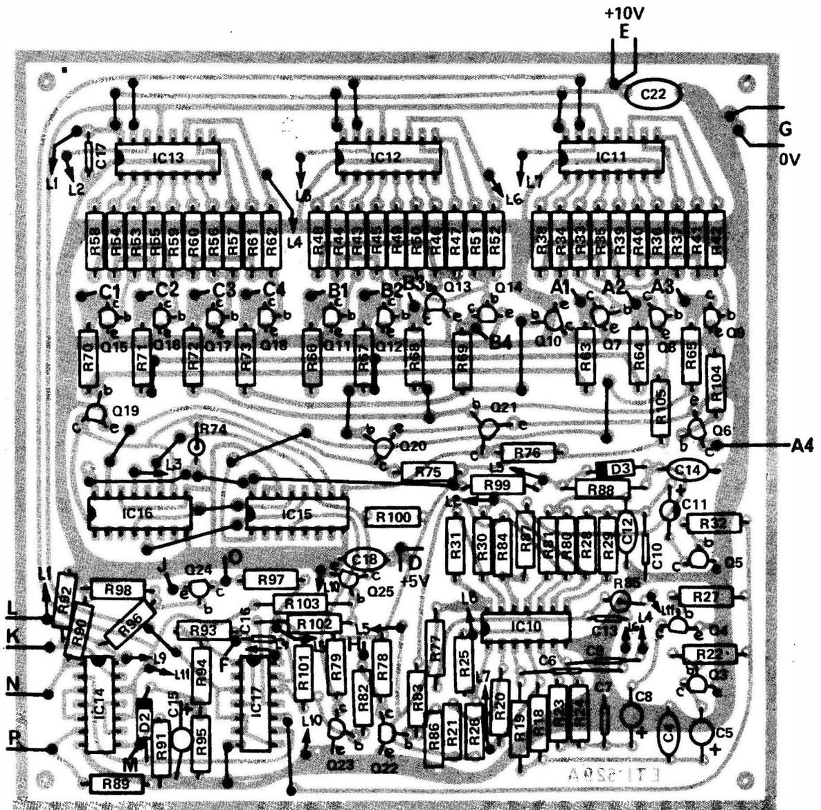
Fig. 5. Component overlay for the logic board.
