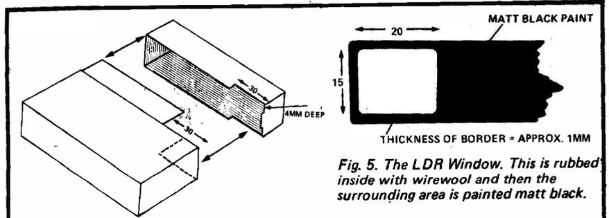
Fig. 4. The work required to modify the transparency case.
