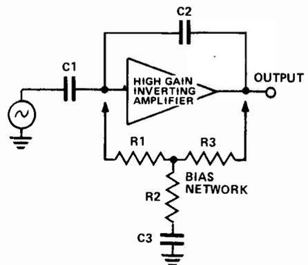
Fig. 6. Basic charge amplifier with bias and filter network. Gain control elements are capacitors. Bias network R1, 2, 3 and C3 are required for dc stability and to roll off bass response.
