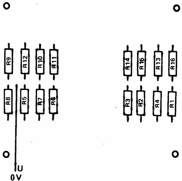
Fig. 3. Component overlay for the copper side of board ETI-123b.
