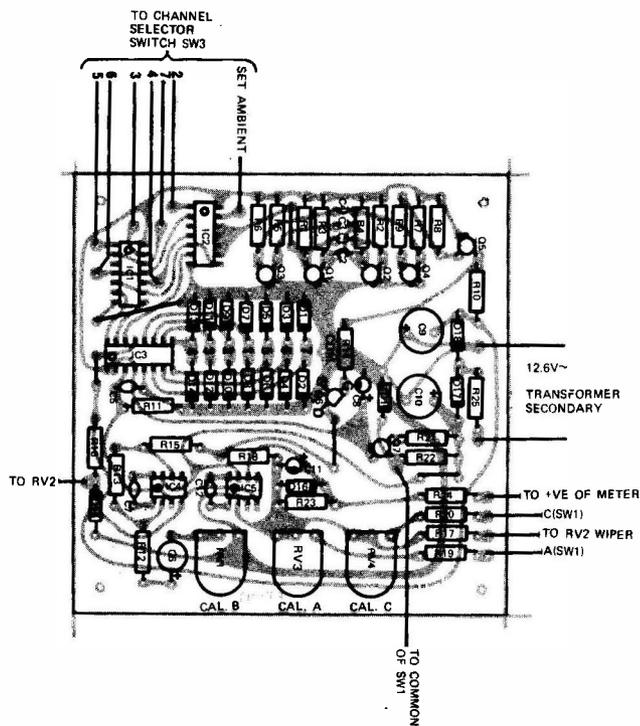
Fig. 3. Component overlay.
