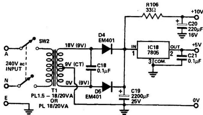
Fig. 4. Circuit diagram of the power supply.
