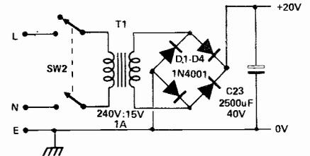
Fig. 2. Circuit of the power supply for Sweet Sixteen.
