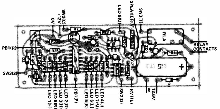
Fig. 2. Component overlay.
