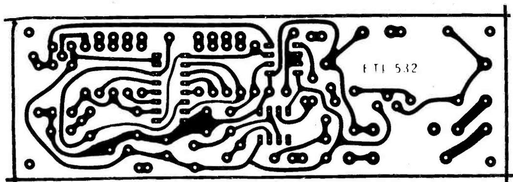
Fig. 4. Printed circuit layout. Full size 133 x 44 mm.
