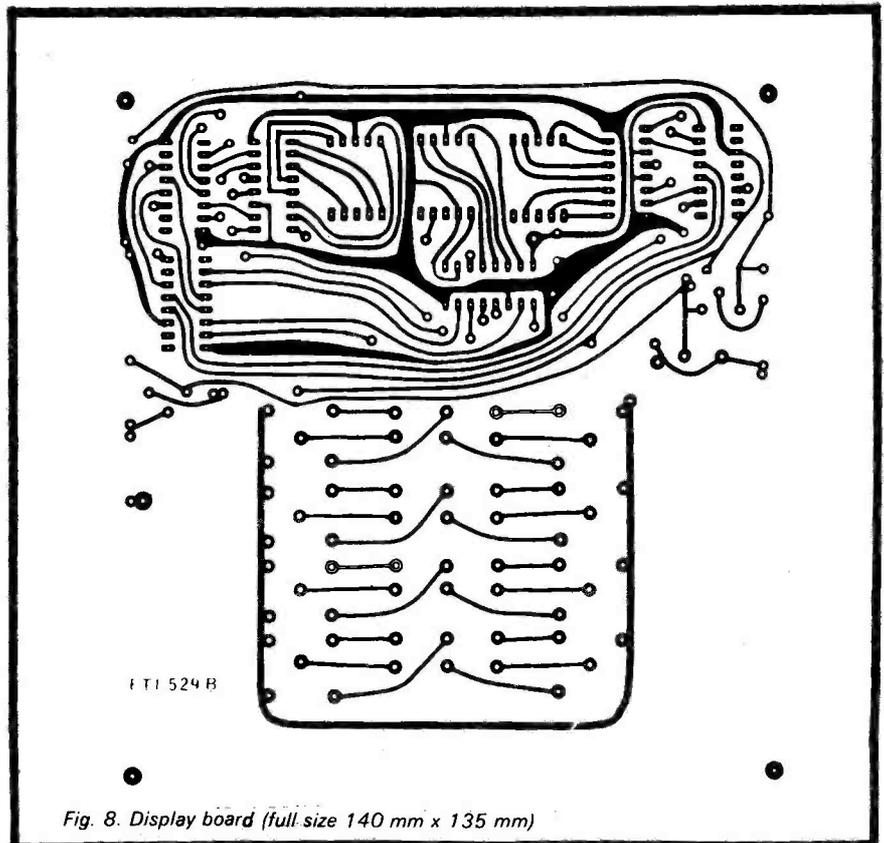
Fig. 8. Display board (full size 140 mm x 135 mm)
