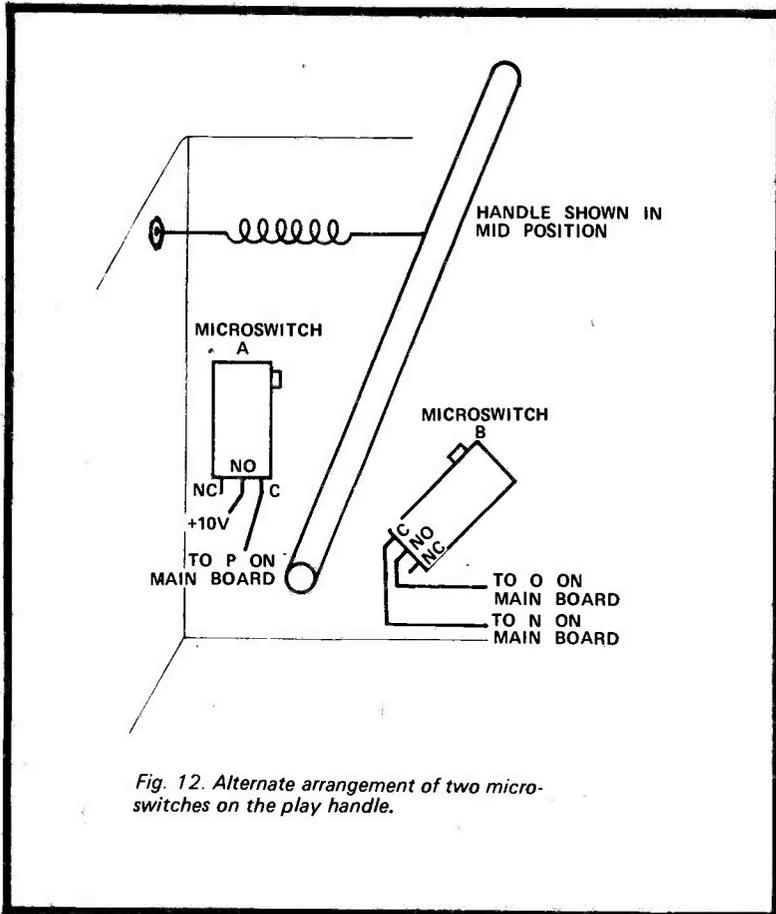
Fig. 12. Alternate arrangement of two microswitches on the play handle.
