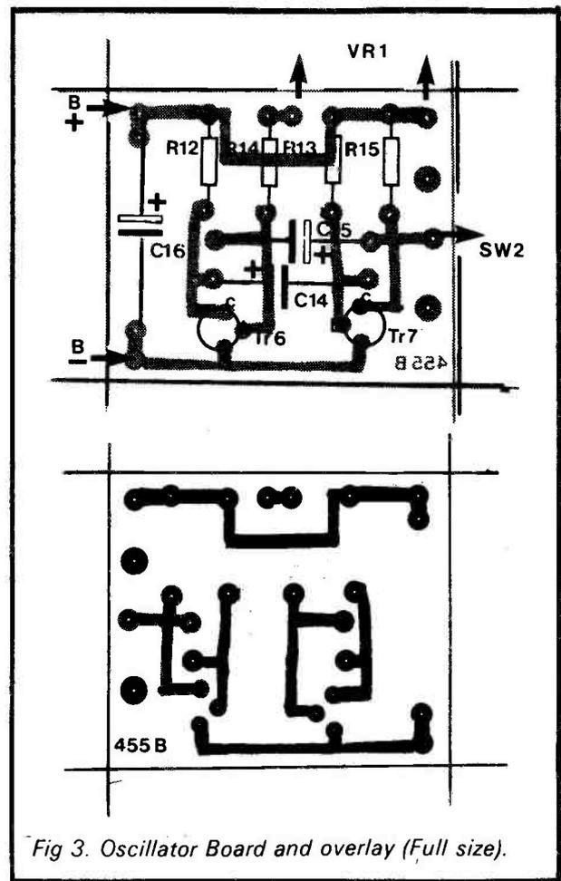
Fig 3. Oscillator Board and overlay (Full size).
