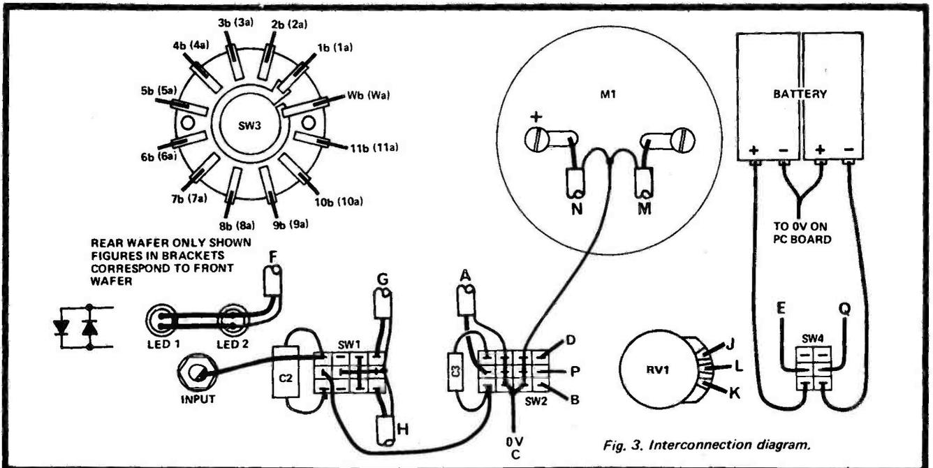
Fig. 3. Interconnection diagram.
