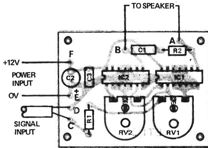
Fig. 3. Component overlay.
