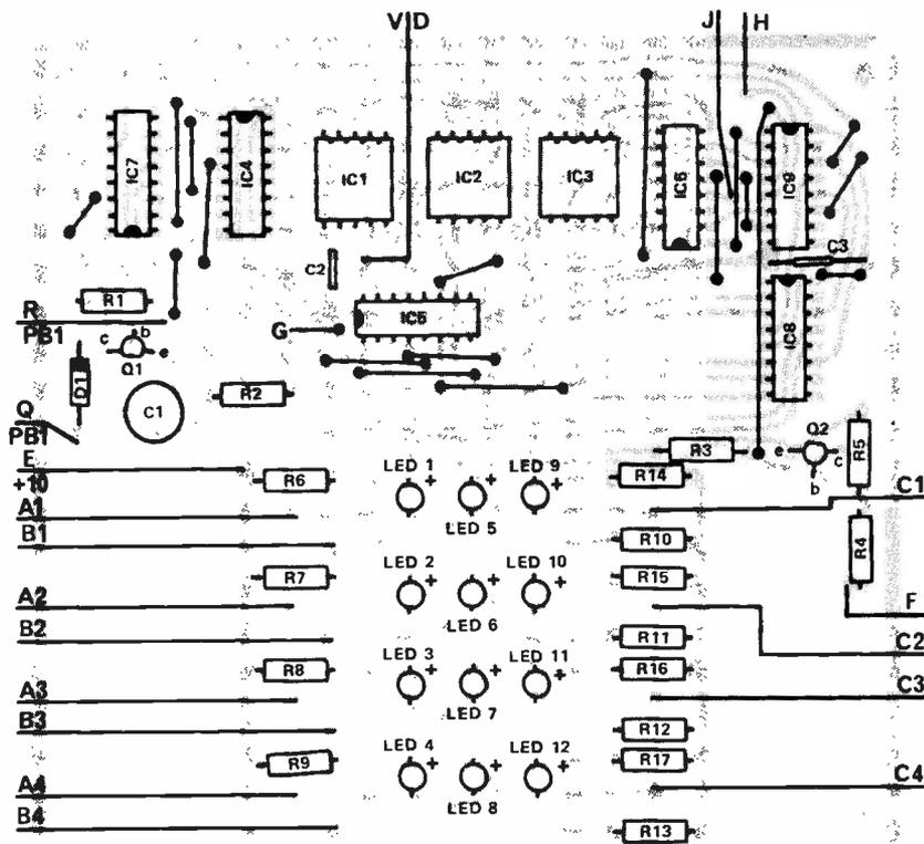
Fig. 9. Component overlay for display board.
