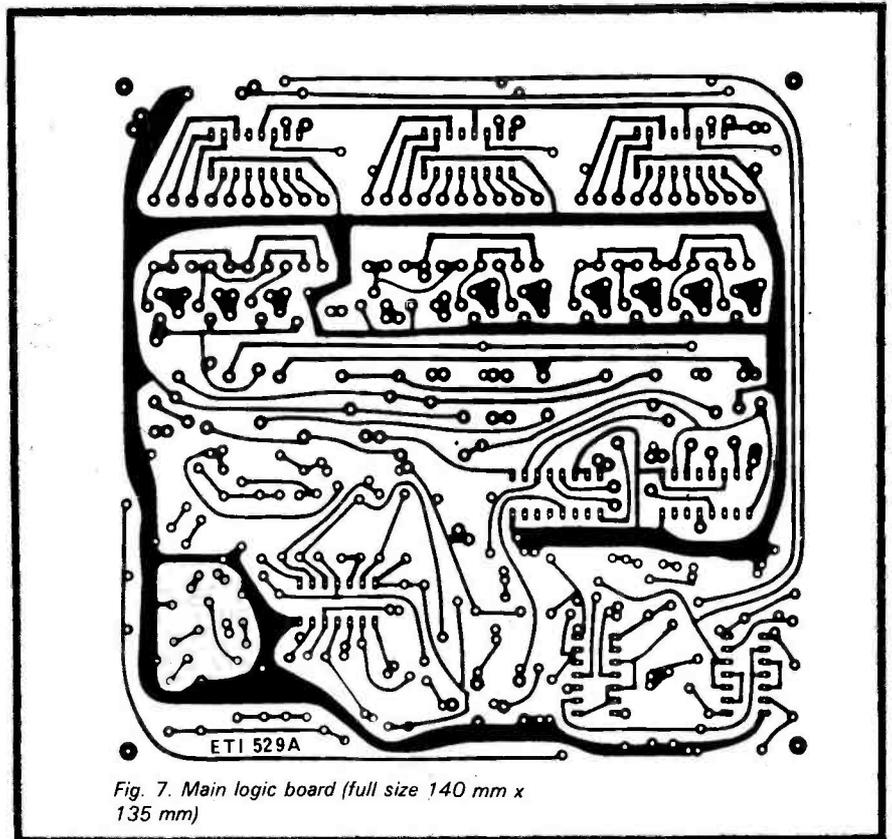
Fig. 7. Main logic board (full size 140 mm x 135 mm)
