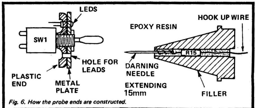
Fig. 6. How the probe ends are constructed.
