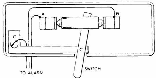
Fig. 3. (Right) Guide to the interior light connections.
