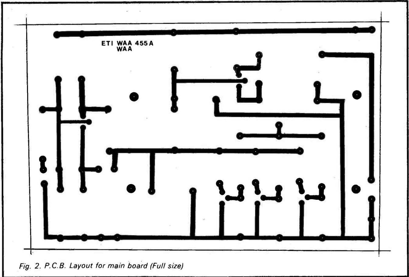
Fig. 2. P.C.B. Layout for main board (Full size)
