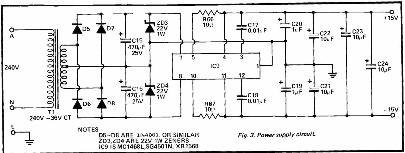
Fig. 3. Power supply circuit.
