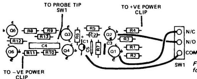
Fig. 3. Component overlay for the pulser.
