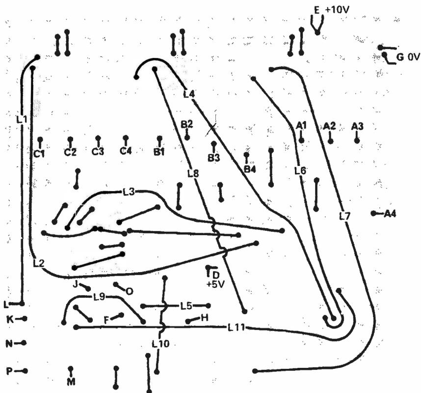
Fig. 10. Linking diagram for the logic board.
