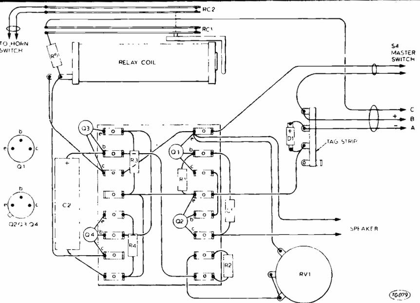
Fig. 2. (Above) The component wiring.
