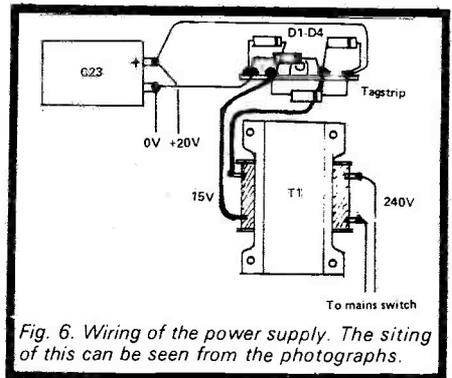
Fig. 6. Wiring of the power supply. The siting of this can be seen from the photographs.
