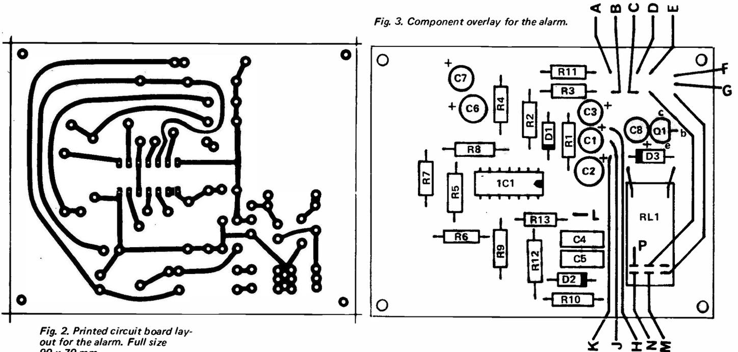
Fig. 2. Printed circuit board layout for the alarm. Full size 90 x 70 mm.
