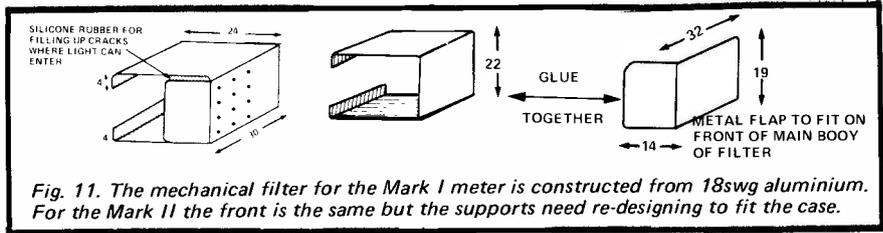
Fig. 11. The mechanical filter for the Mark I meter is constructed from 18swg aluminium. For the Mark II the front is the same but the supports need re-designing to fit the case.
