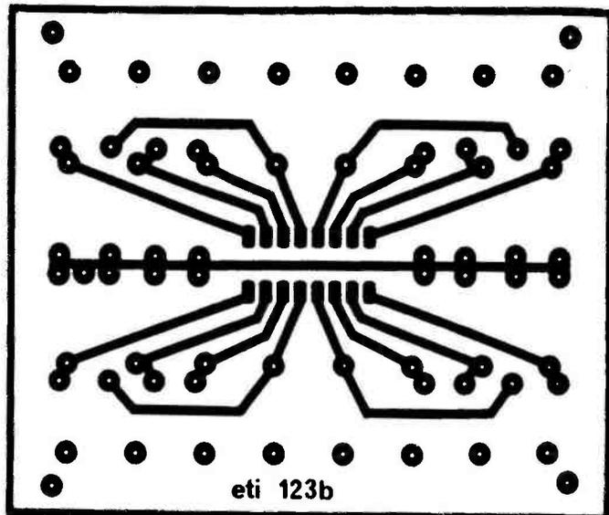
Fig. 6. Printed-circuit board layout – ETI 123a. Full size 88 x 63 mm. Fig. 7. Printed-circuit board layout – ETI 123b. Full size 88 x 71 mm.
