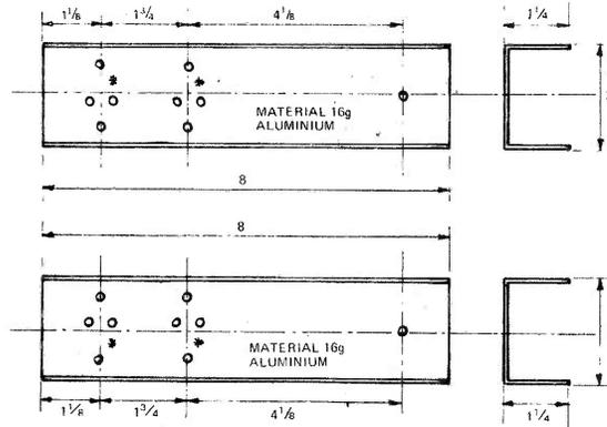
Drilling details of ITT box lid and associated heat sinks
