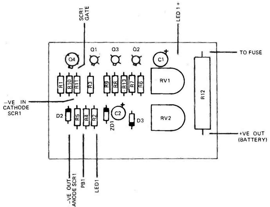
Fig. 3. Component overlay.
