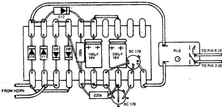
Fig. 7. Constructional details of circuit shown in Fig. 6.
