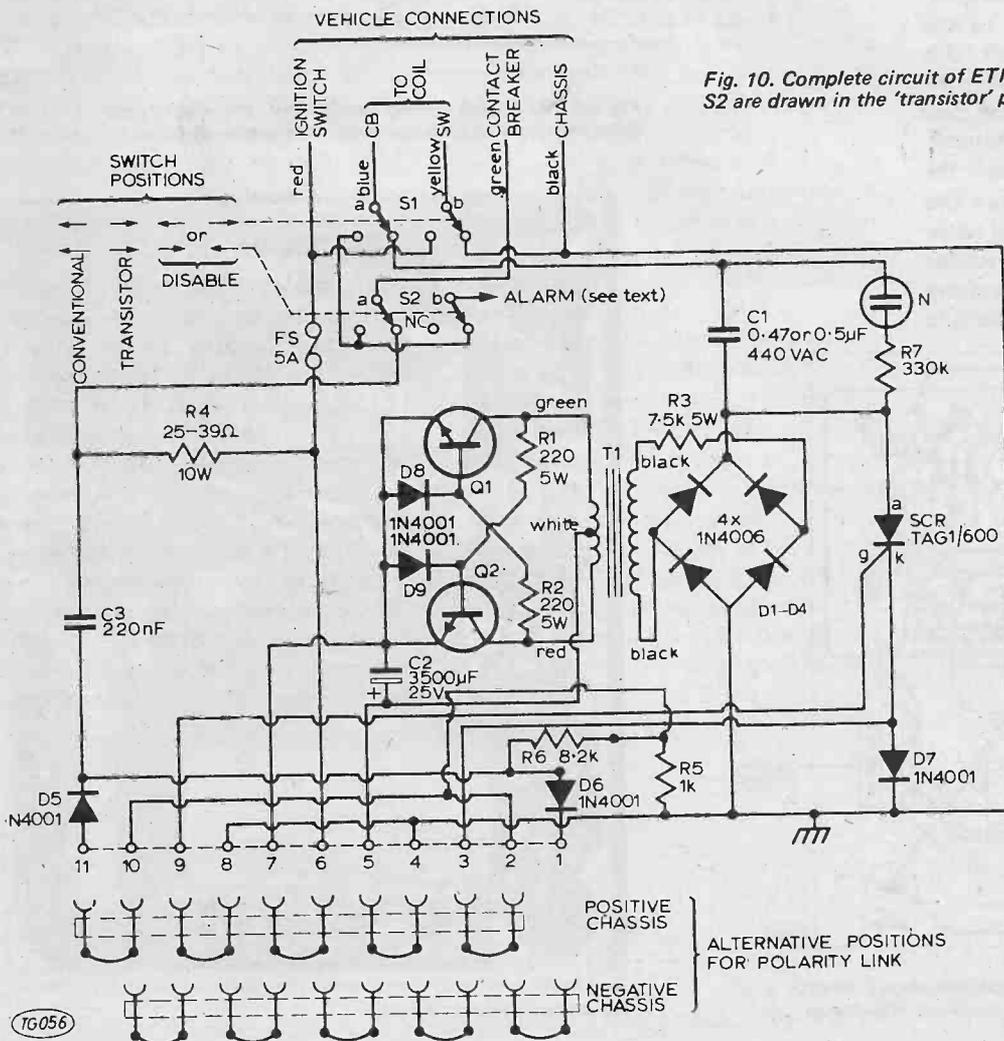
Fig. 10. Complete circuit of ETI Transistor Ignition. S1 and S2 are drawn in the 'transistor' position.
