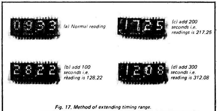
Fig. 17. Method of extending timing range.
