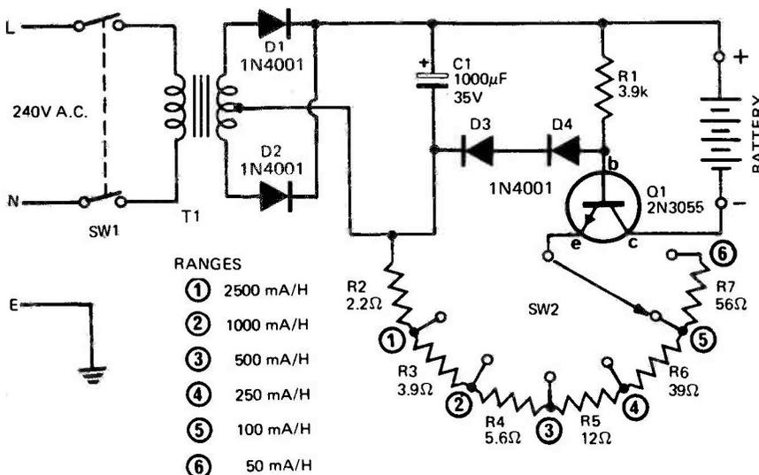
Fig. 1. Circuit diagram of the Nickel-Cadmium Battery Charger.
