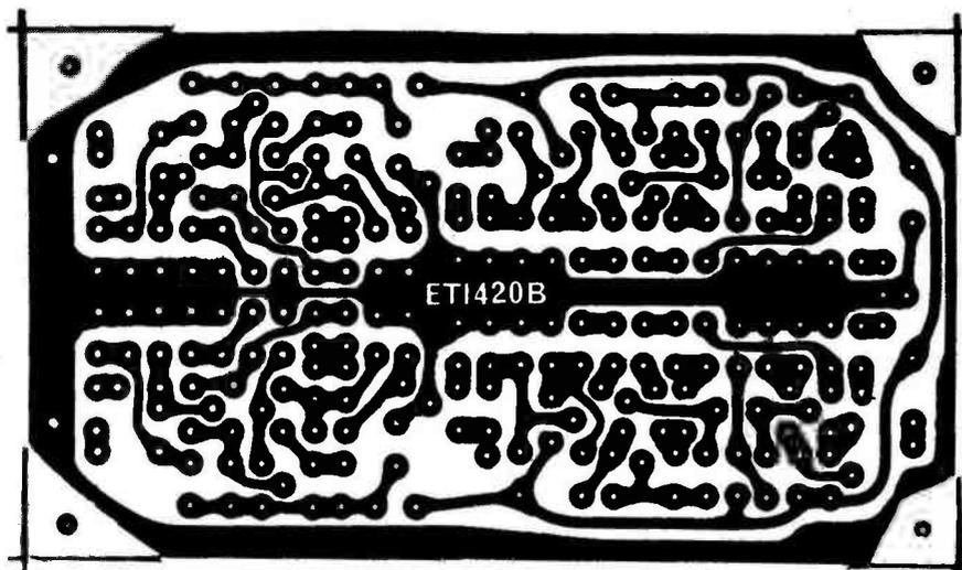
Fig.2. Printed circuit board pattern for the preamplifier.
