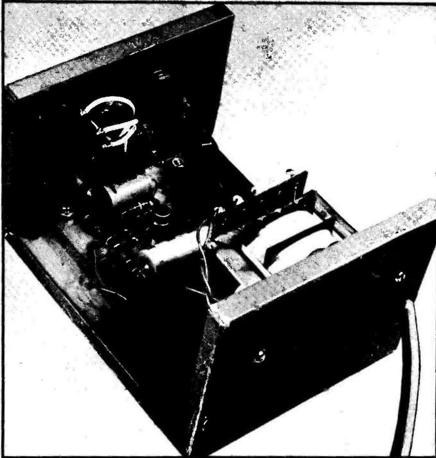
THIS PROJECT builds into a versatile power supply capable of delivering 1 amp up to 10 volts and ½ amp up to 15 volts.
