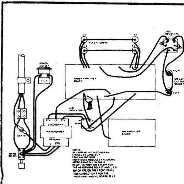
Fig. 9. Power wiring diagram of the complete amplifier.
