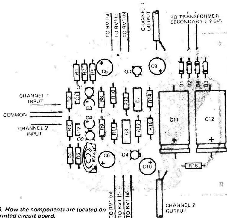
Fig. 3. How the components are located on the printed circuit board.
