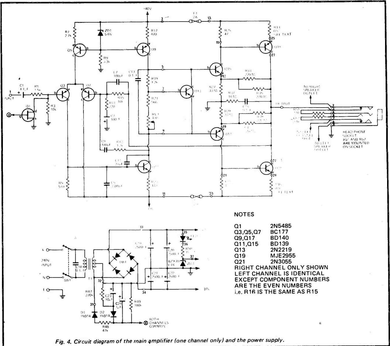
Fig. 4. Circuit diagram of the main amplifier (one channel only) and the power supply.
