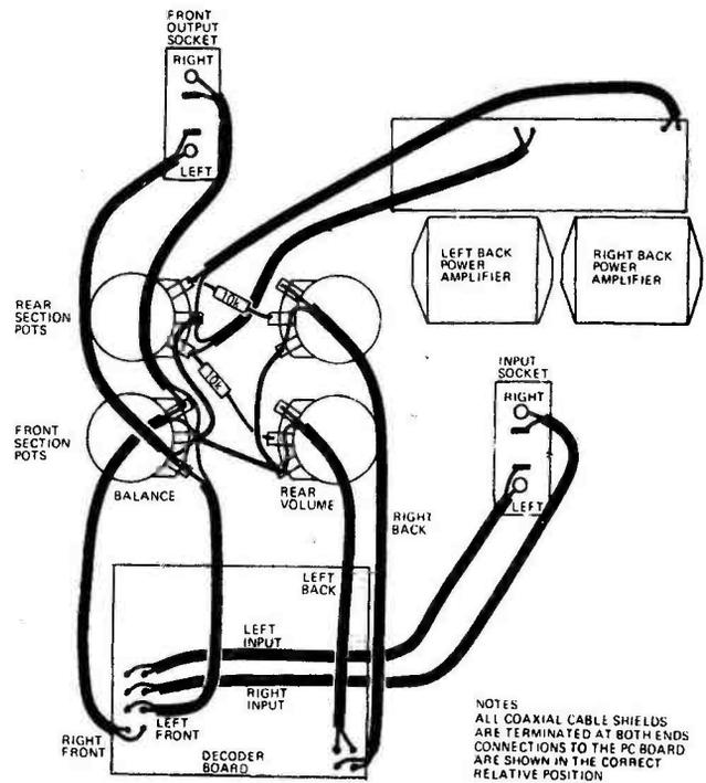
Fig. 9. Interconnections - signal wiring.
