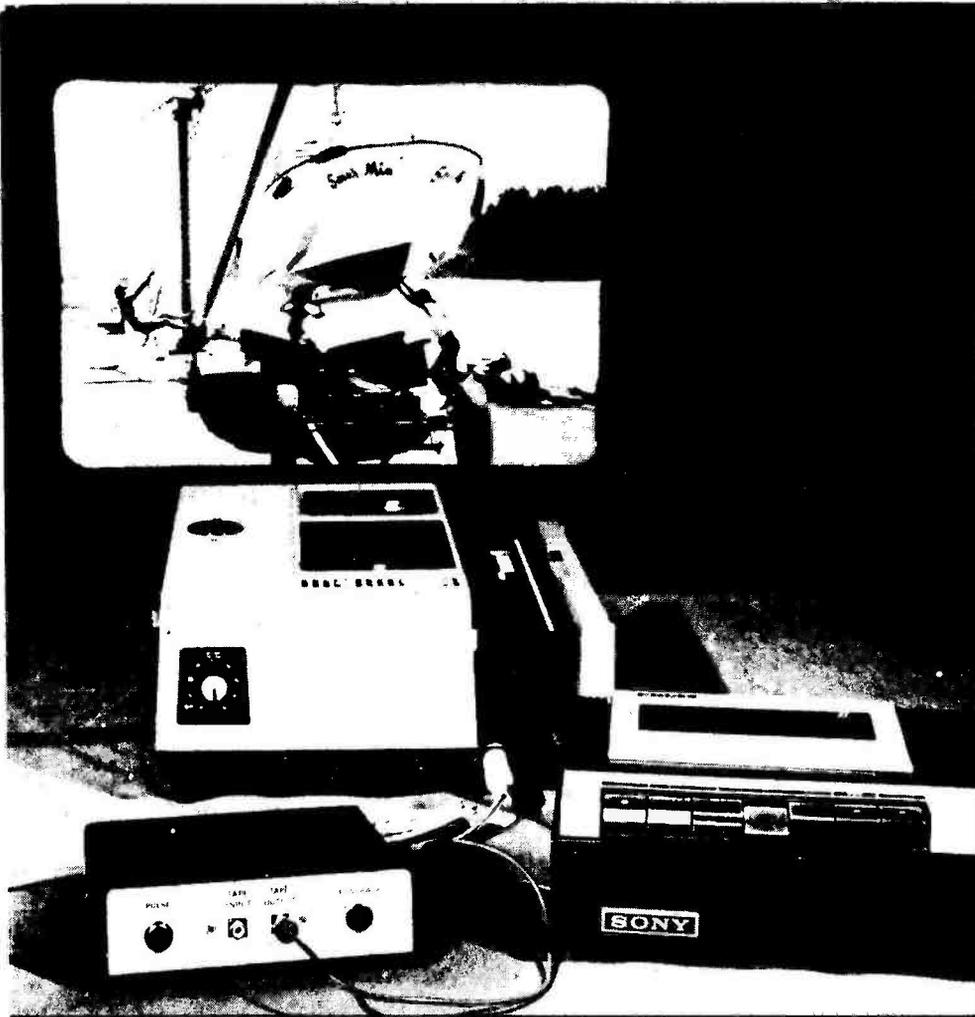
This unit automatically changes slides on an automatic projector. It does this at predetermined times, synchronizing with the commentary prerecorded on a two-channel, cassette or reel-to-reel tape recorder.
