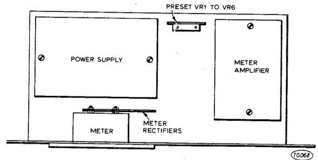
Fig. 9. Layout of circuit boards on the chassis.
