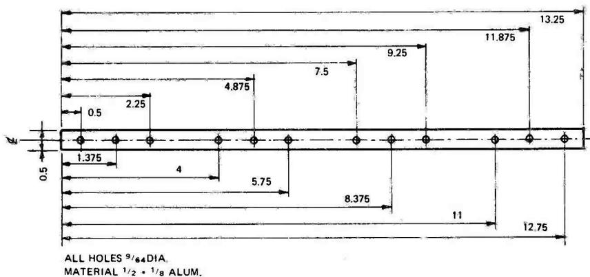
Fig. 13. Slide potentiometer support bars (two required)
