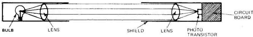
Fig. 15. Arrangement of light beam transmitter and receiver.
