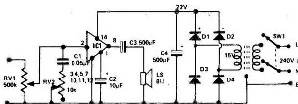
Fig. 5. Circuit of the record-player amplifier.
