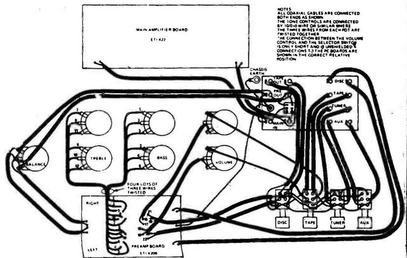
Fig. 10. Signal wiring diagram of the complete amplifier.
