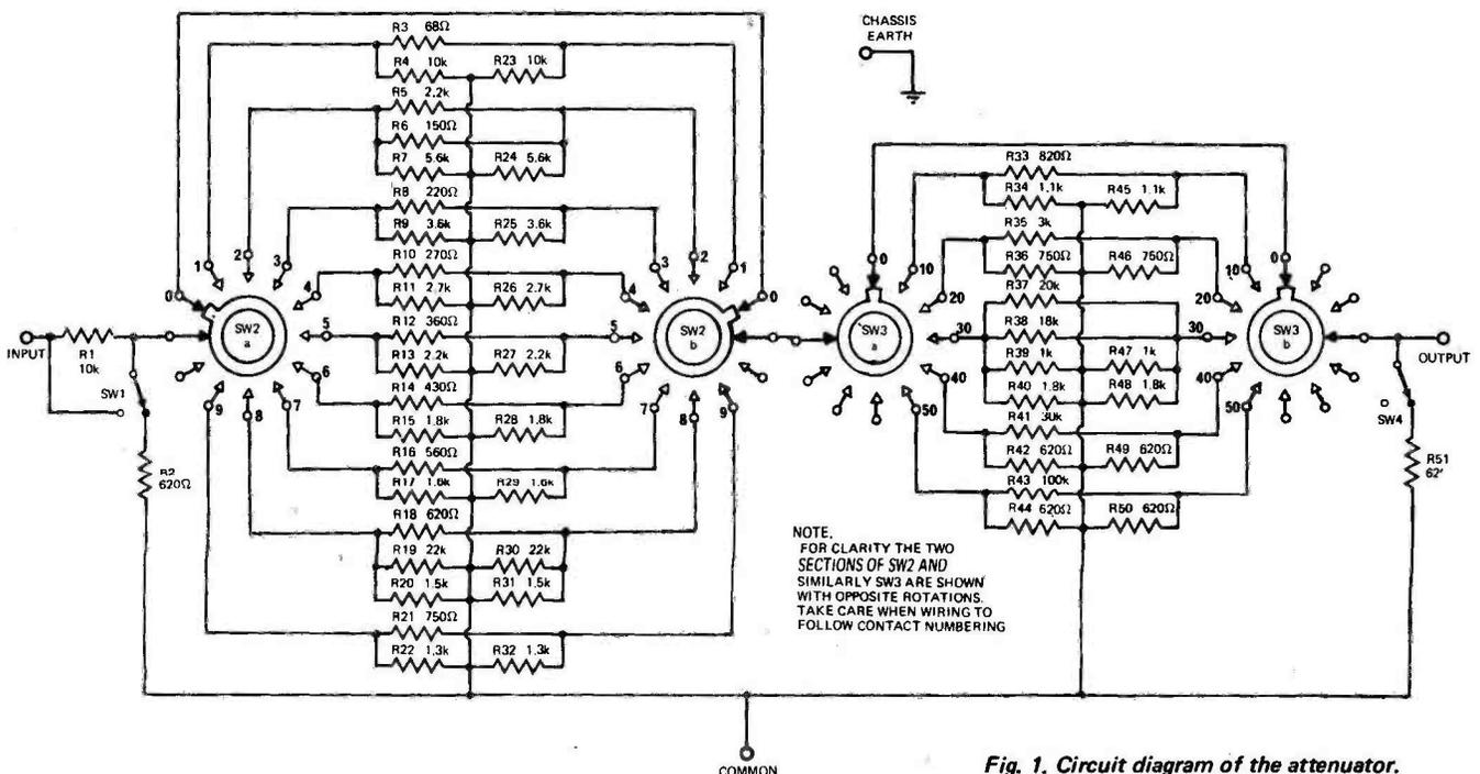
Fig. 1. Circuit diagram of the attenuator.
