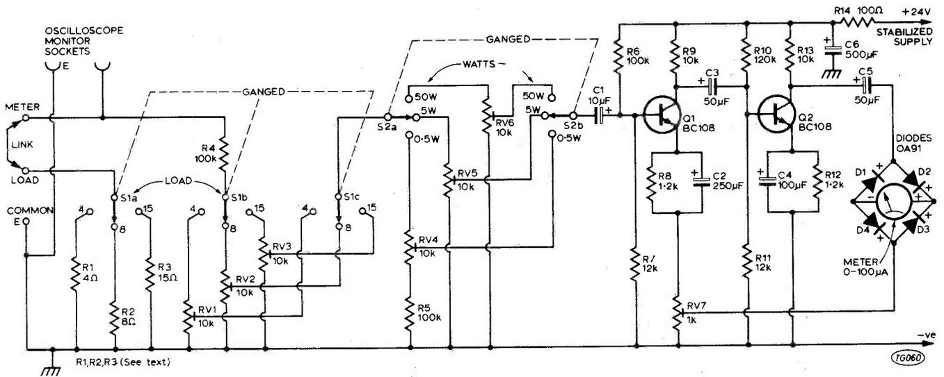
Fig. 1. Complete circuit of the Audio Wattmeter.
