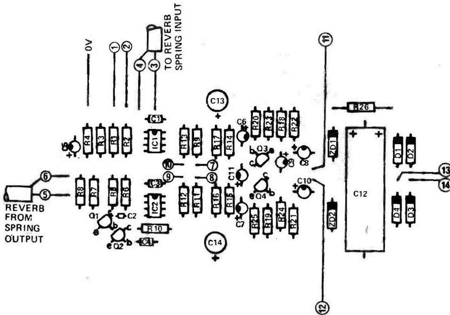
Fig. 3. Component overlay.
