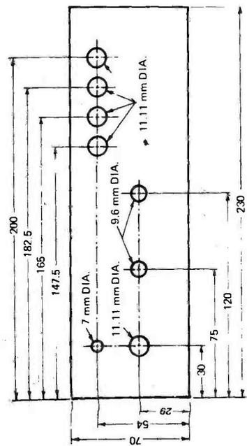
Fig. 14. Front panel escutcheon dimensions and drilling details
