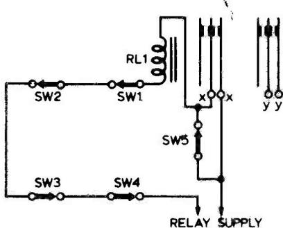
Fig. 4. (right) Closed circuit system.
