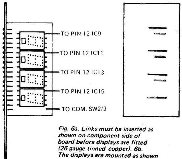
Fig. 6a. Links must be inserted as shown on component side of board before displays are fitted (26 gauge tinned copper). 6b. The displays are mounted as shown with the chip towards bottom of board.
