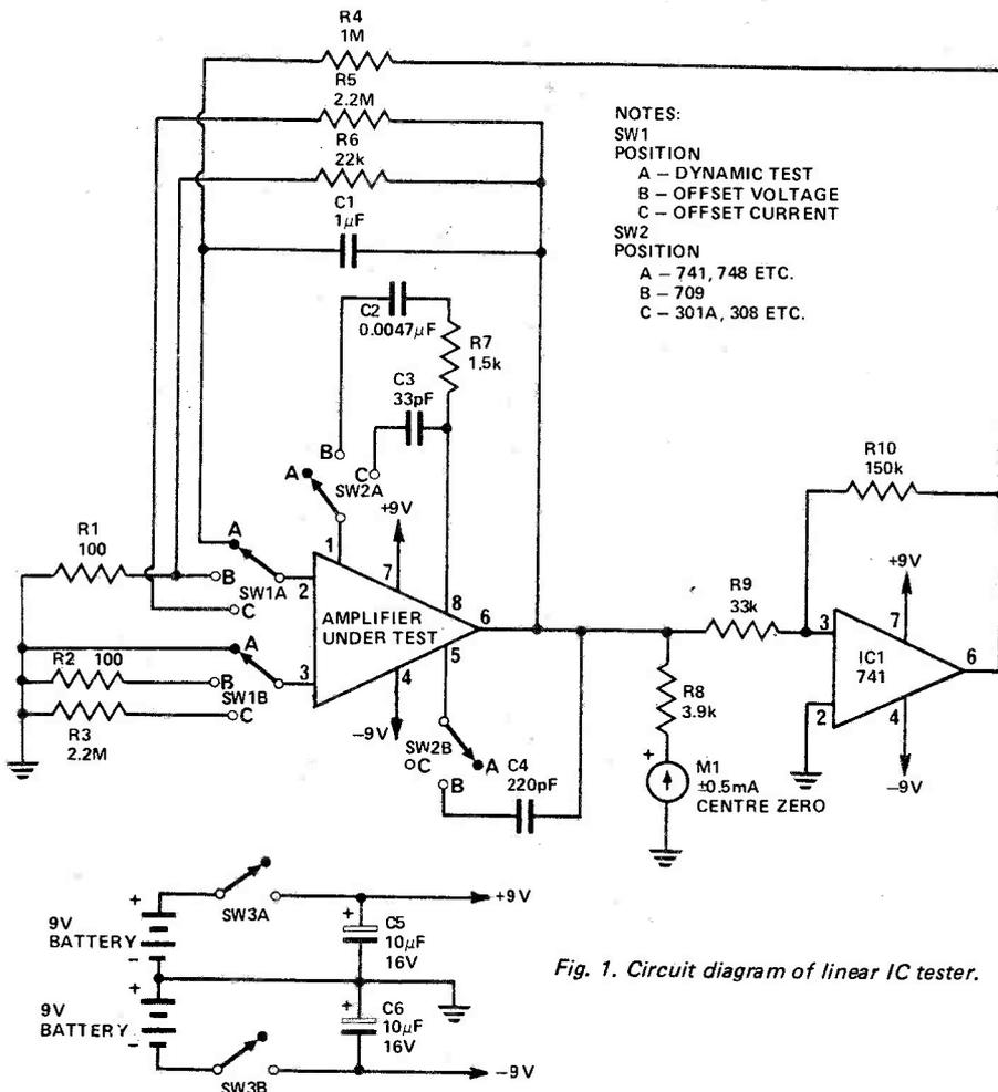
Fig. 1. Circuit diagram of linear IC tester.
