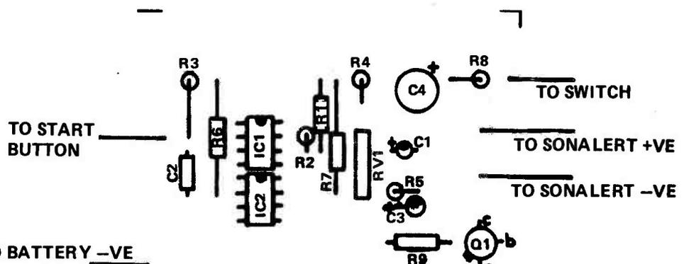
Fig. 4. Component overlay.
