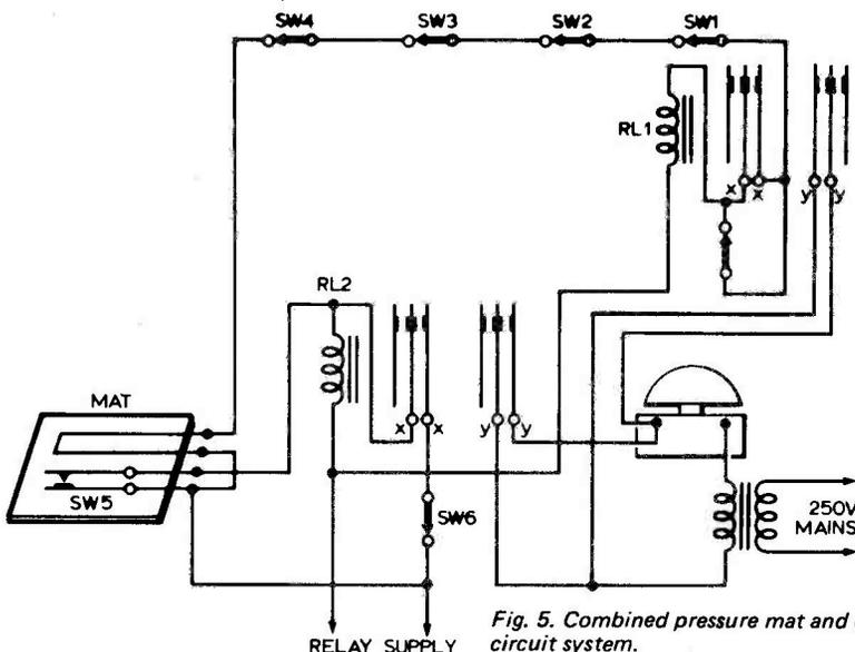
Fig. 5. Combined pressure mat and closed circuit system.
