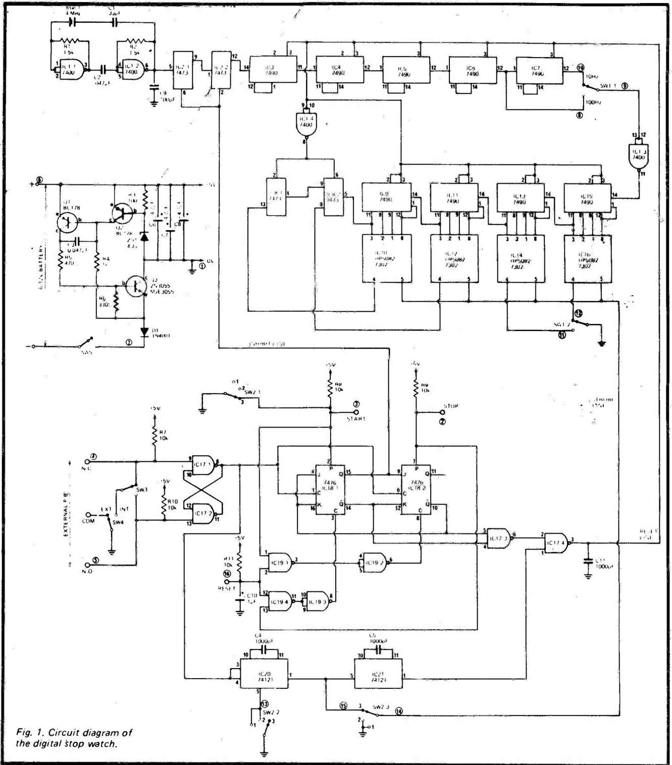
Fig. 1. Circuit diagram of the digital stop watch.
