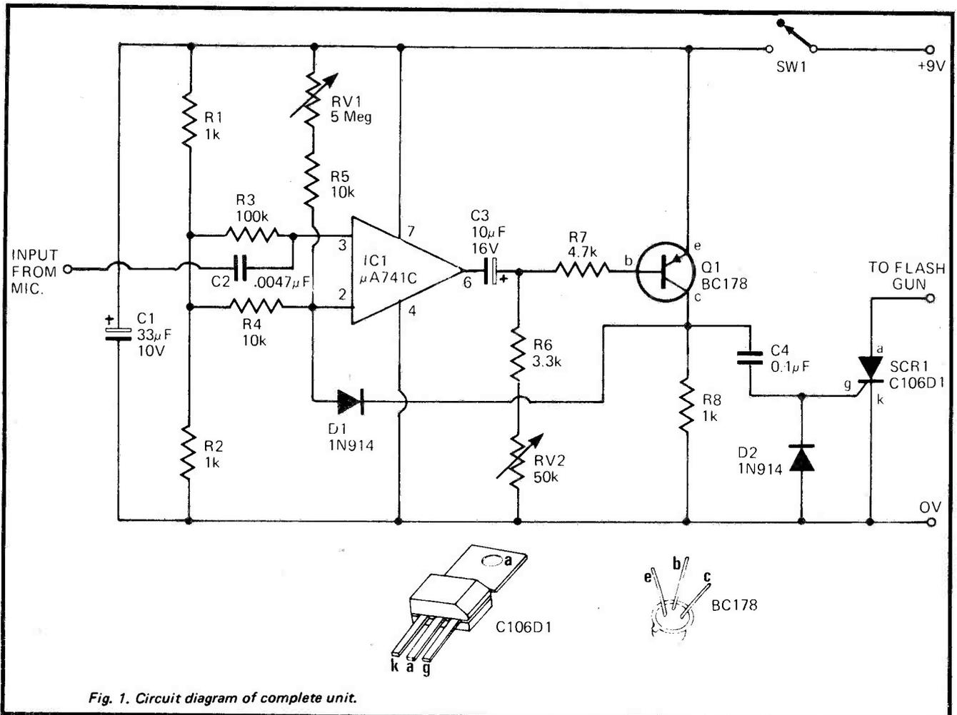
Fig. 1. Circuit diagram of complete unit.
