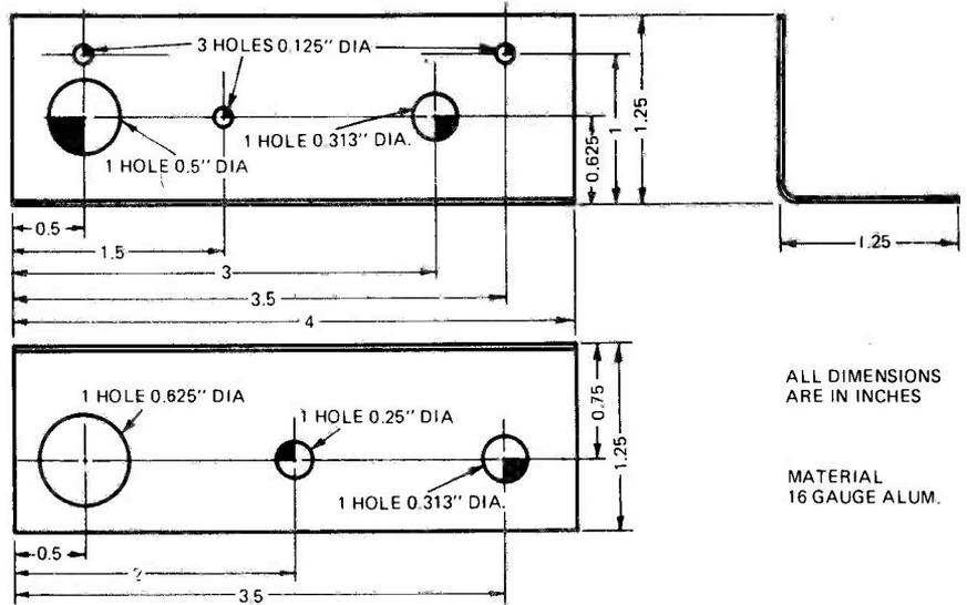
Fig. 5. Mounting bracket for printed circuit board.
