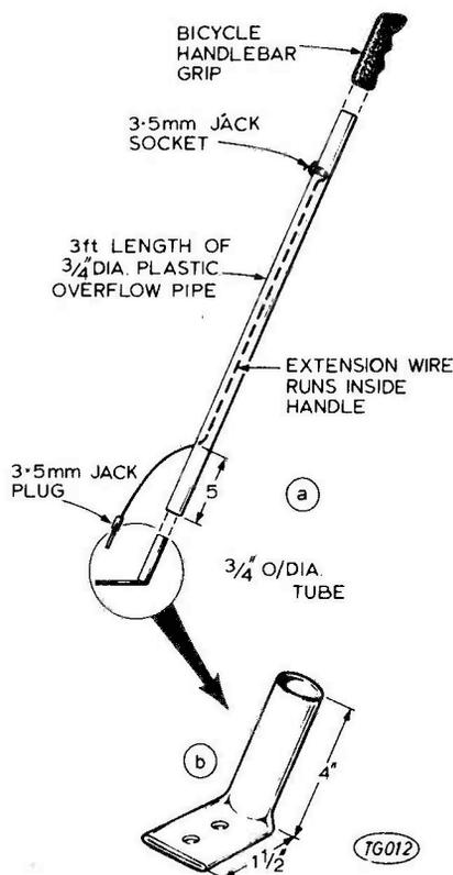
Fig. 2 Details of the long handle and bracket
