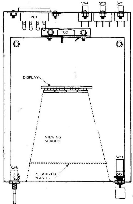
Fig. 5. Positioning of major components on the chassis.
