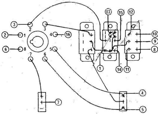
Fig. 7. Wiring to switches and power/control socket.
