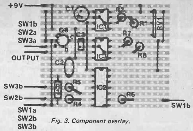
Fig. 3. Component overlay.
