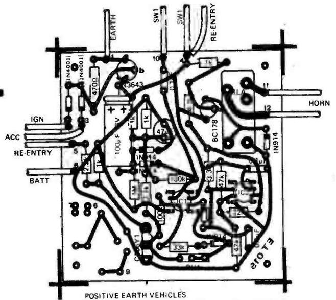
Fig. 2. Component layout (positive earth vehicles).
