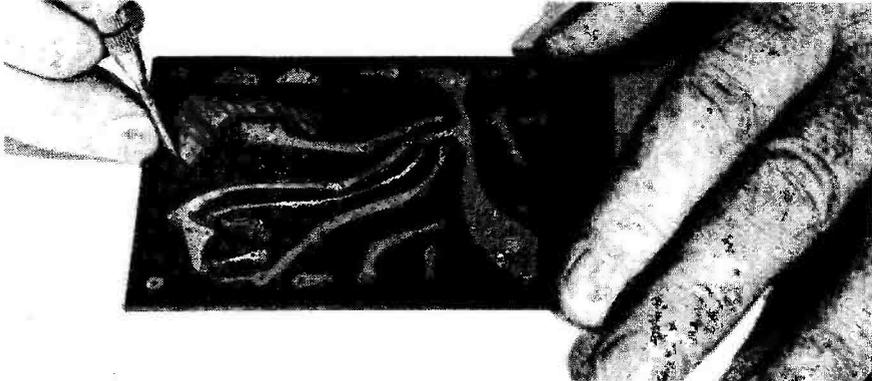
*Fig. 9. After etching away all unwanted copper, mark hole positions with a scribe.*
