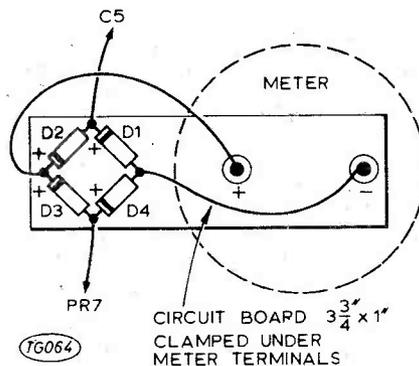
Fig. 5 (above). D1-D4 are fitted to a board which mounts on the meter terminals.
