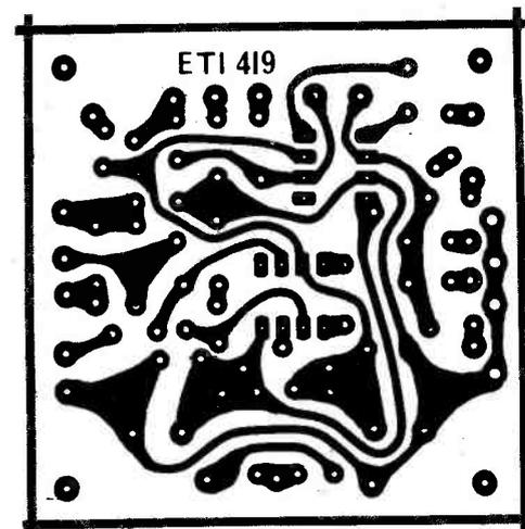
Fig. 4. PC board layout (both versions).
