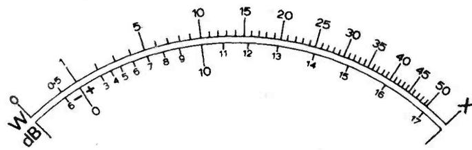
Fig. 12. Meter scale shown actual size. This will only fit the Anders KMI18.
