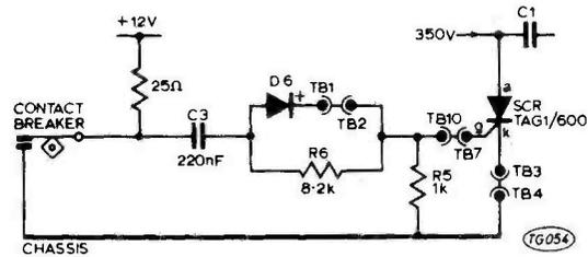
Fig. 8. Trigger circuit for negative chassis vehicles.
