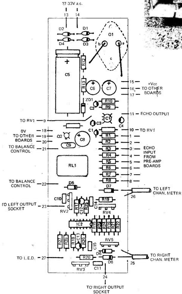
Fig. 3. Component overlay of power supply board.
