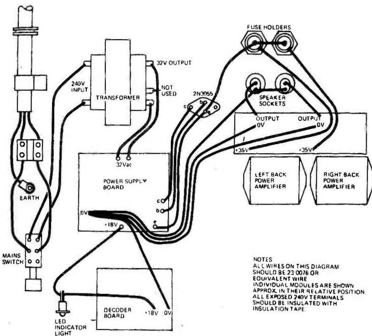
Fig. 8. Interconnections - power wiring.
