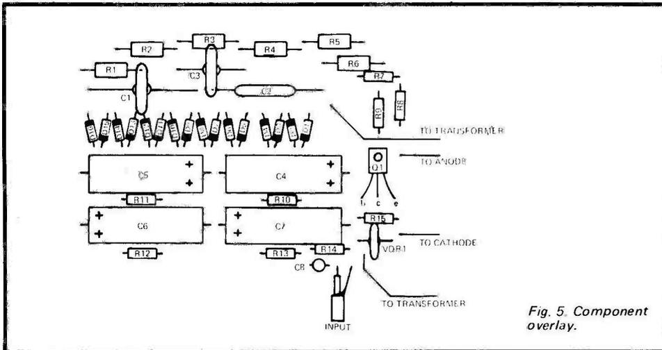
Fig. 5. Component overlay.
