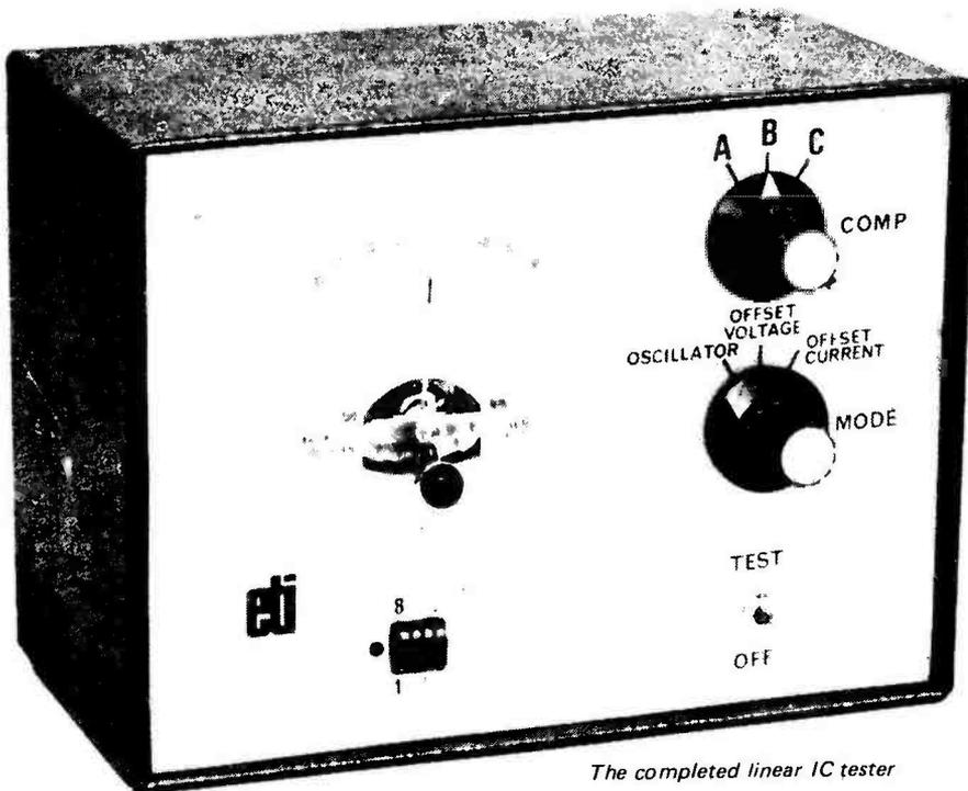
The completed linear IC tester
