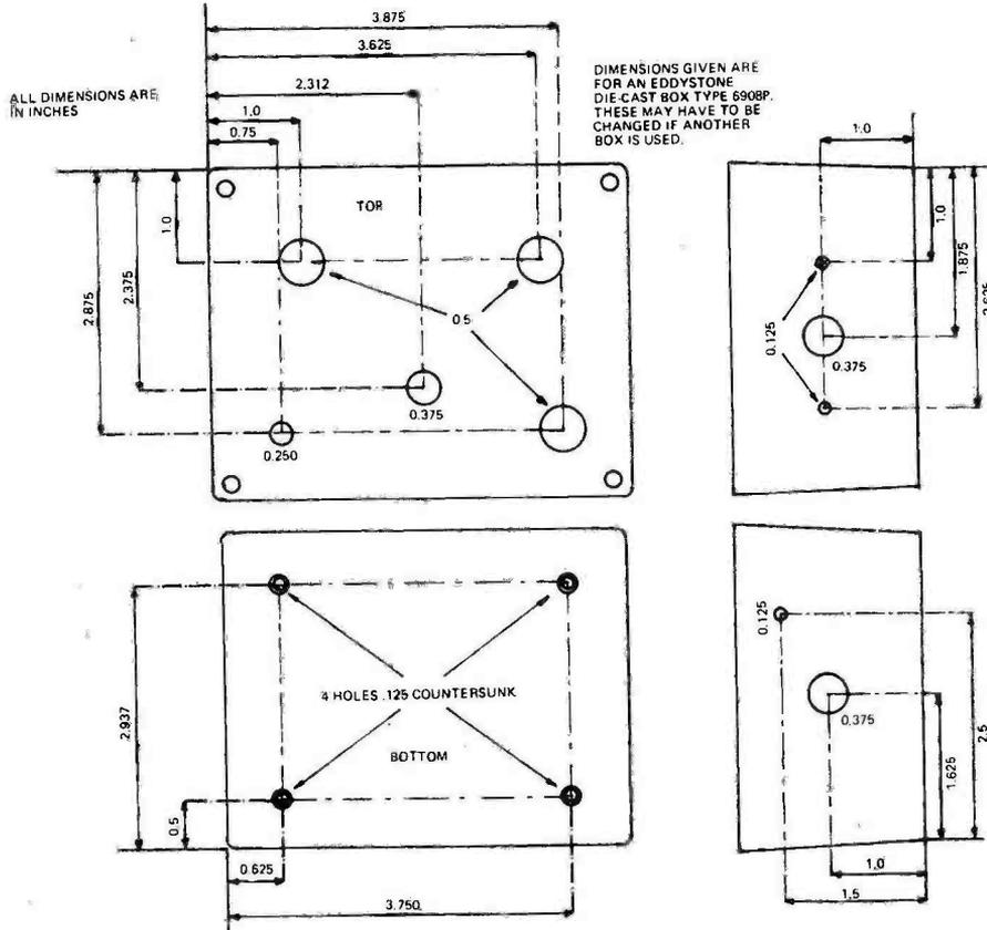
Fig. 4. Drilling details for cast aluminium box.
