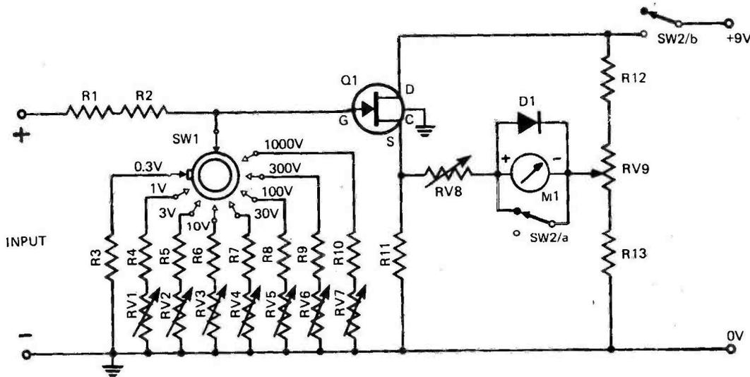
This cheap and easily constructed dc voltmeter has 10 Megohm input resistance.
