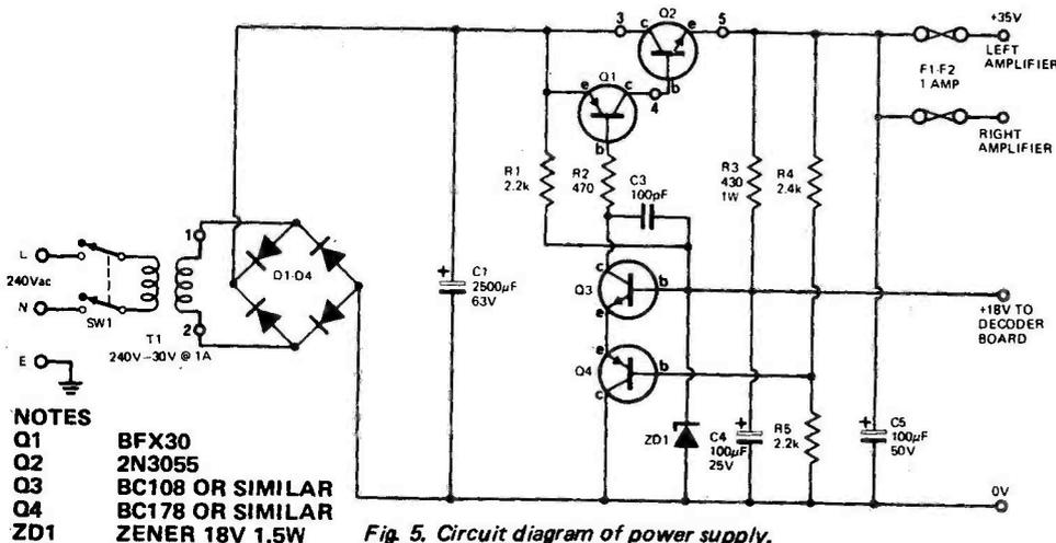
Fig. 5. Circuit diagram of power supply.
