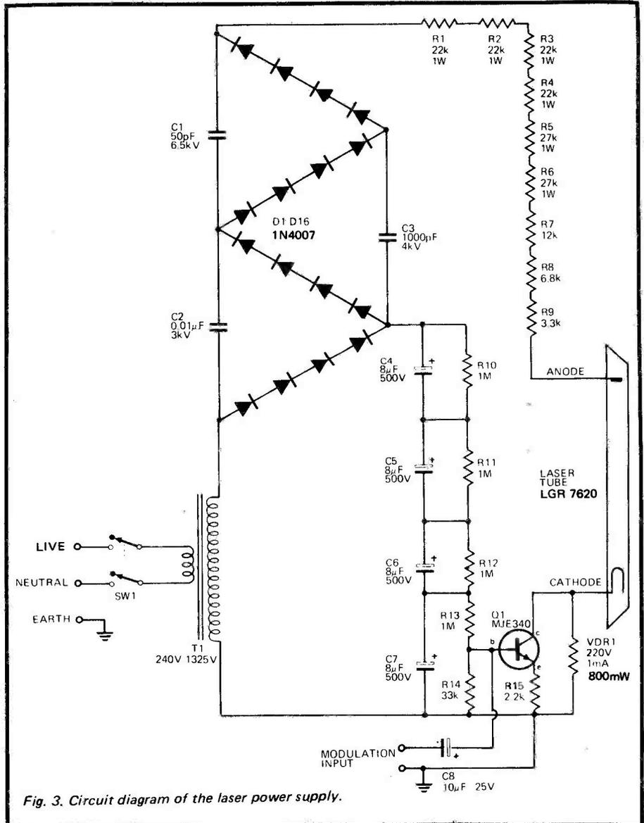
Fig. 3. Circuit diagram of the laser power supply.
