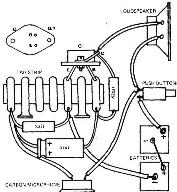
FIG. 2 COMPONENT CONNECTIONS
