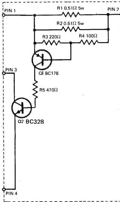
Fig. 1. Circuit diagram of the basic unit.
