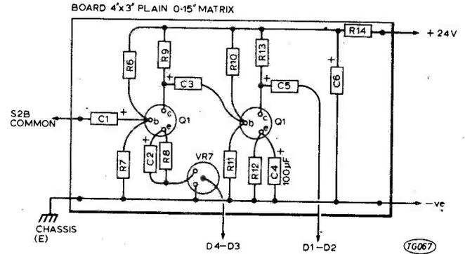
Fig. 8. Layout and wiring of the meter amplifier.
