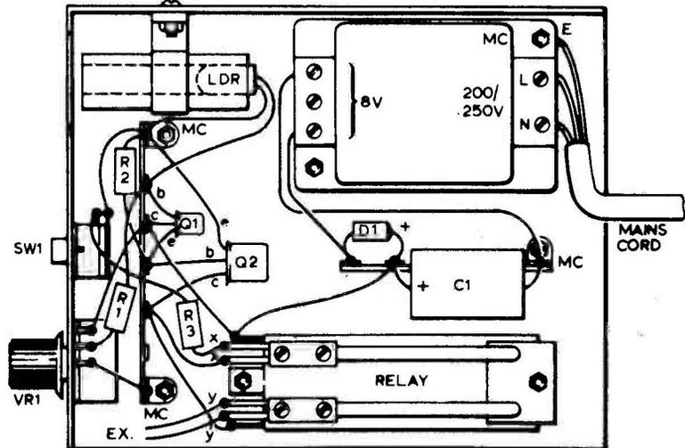
Fig. 8. Wiring of the light beam receiver.
