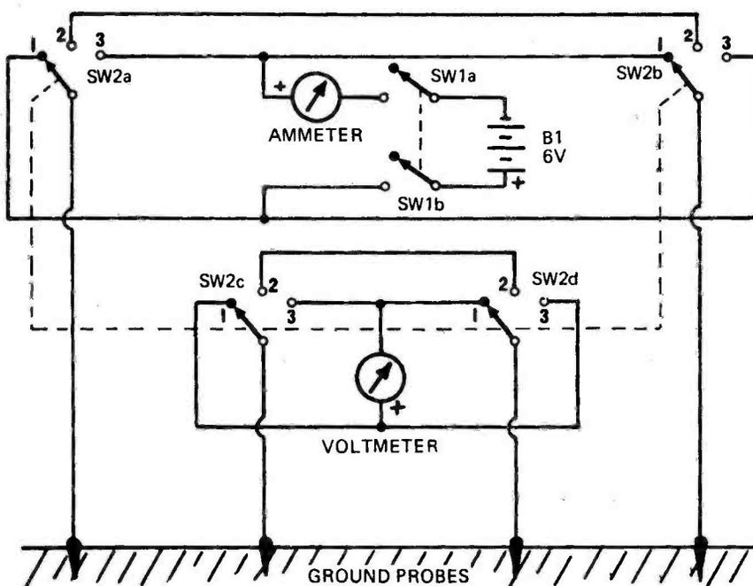
Fig. 1. Circuit diagram of resistivity meter.
