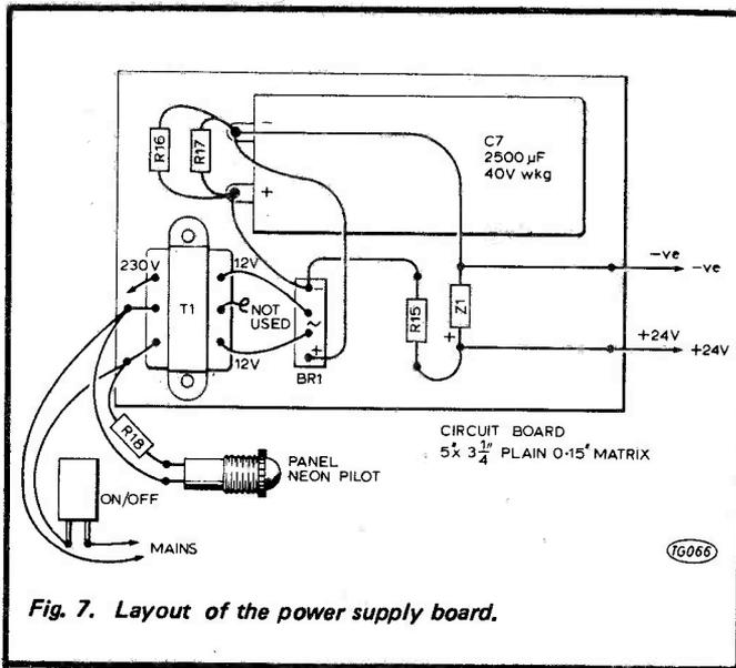
Fig. 7. Layout of the power supply board.
