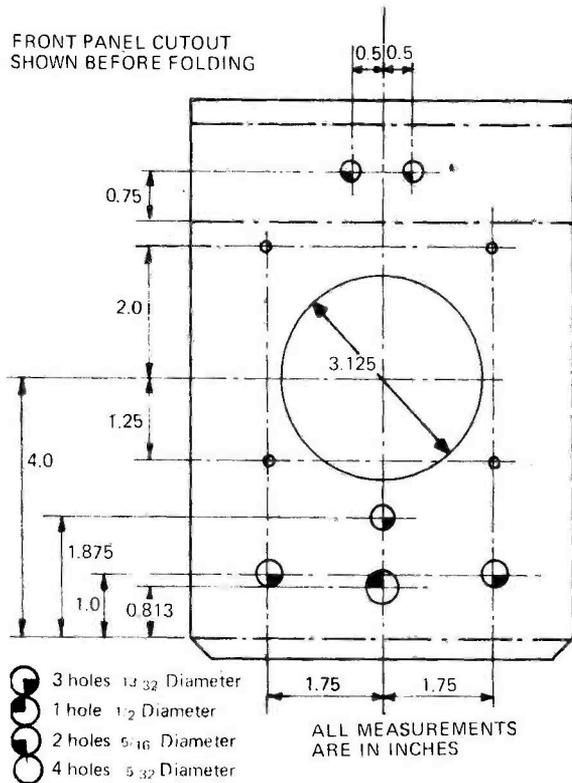
Fig. 4. Constructional details of the meter case.
