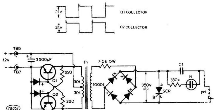
Fig. 7. The Inverter circuit.
