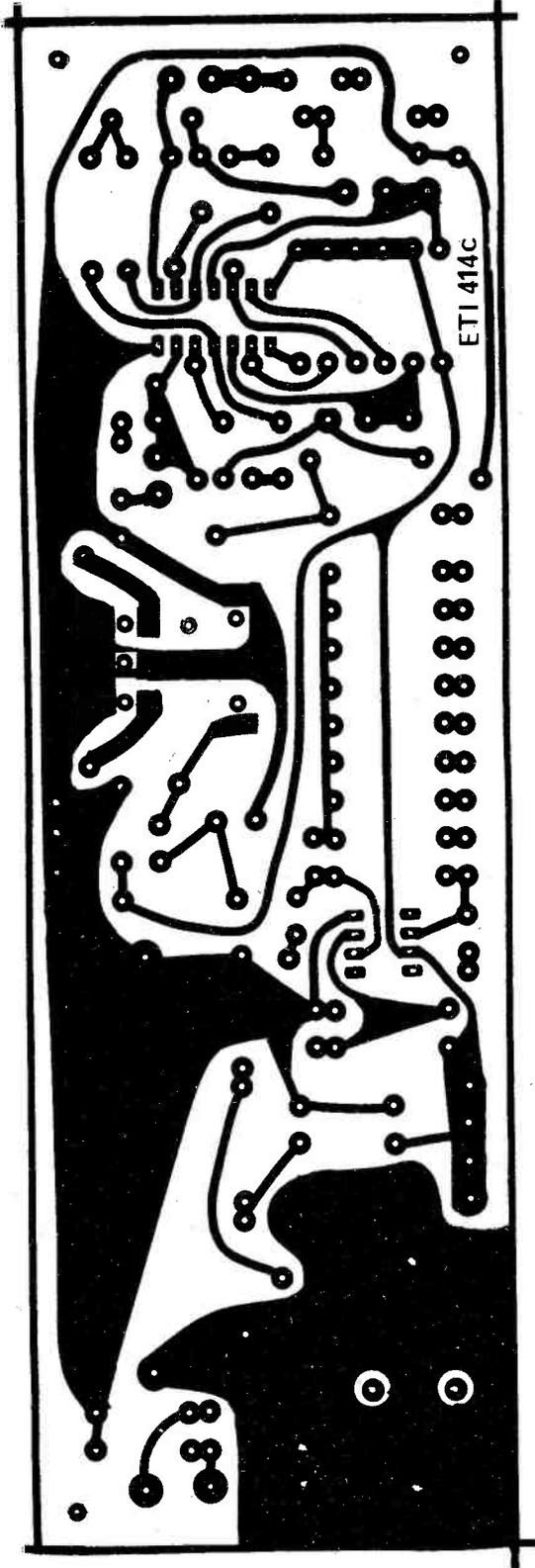
Fig. 2. Foil pattern for power supply board
