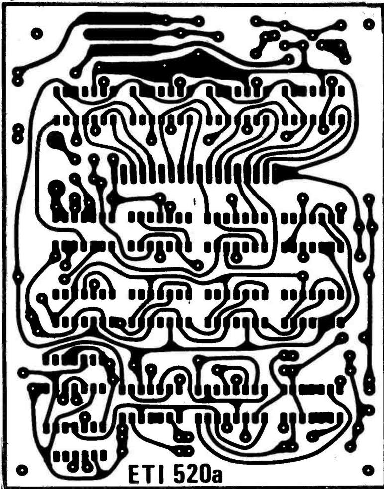
Fig. 2. Main PC board layout for the stopwatch.
