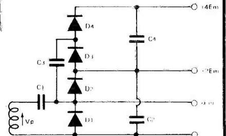
Fig. 2. The basic Cockcroft-Walton voltage quadrupler circuit.
