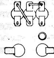
Relay connections. Holes should be drilled through the veroboard large enough to accommodate the twin tags. The tags are then bent over and soldered as shown.
