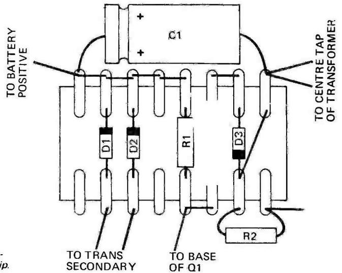
Fig. 2. Layout of components on the tag-strip.
