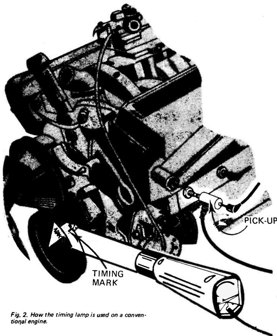
Fig. 2. How the timing lamp is used on a conventional engine.
