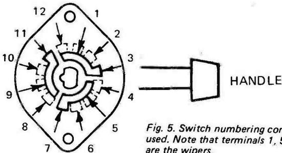
Fig. 5. Switch numbering convention used. Note that terminals 1, 5 and 9 are the wipers.
