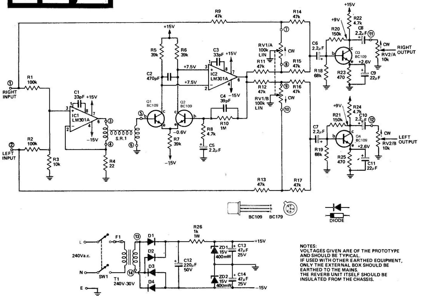
Fig. 1. Circuit diagram of the spring reverberation unit.
