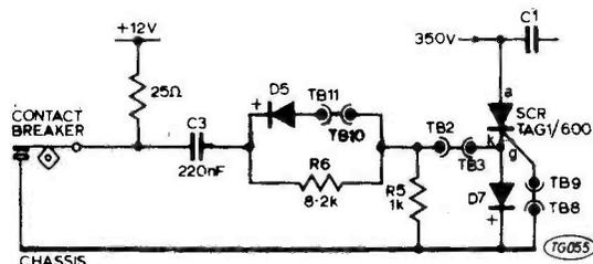
Fig. 9. Trigger circuit for positive chassis vehicles.
