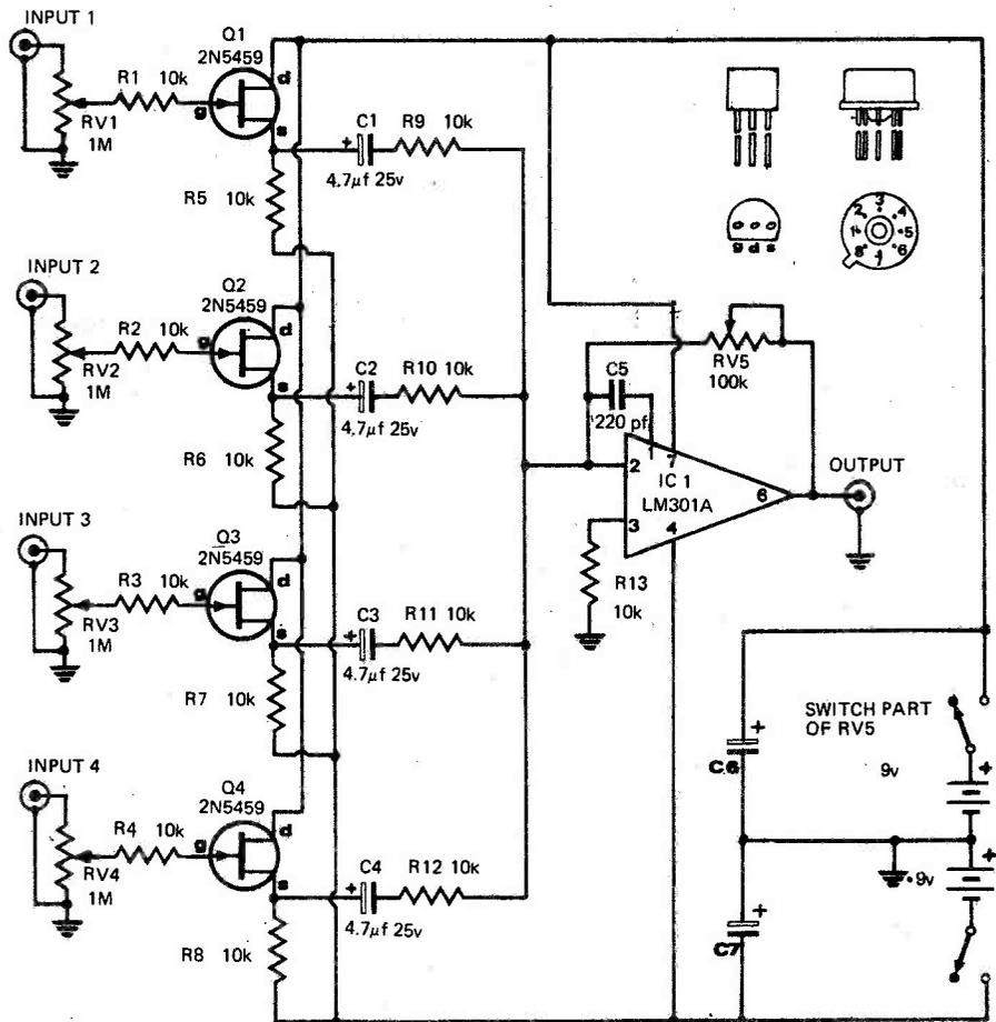
Fig. 2, Circuit diagram of complete unit
