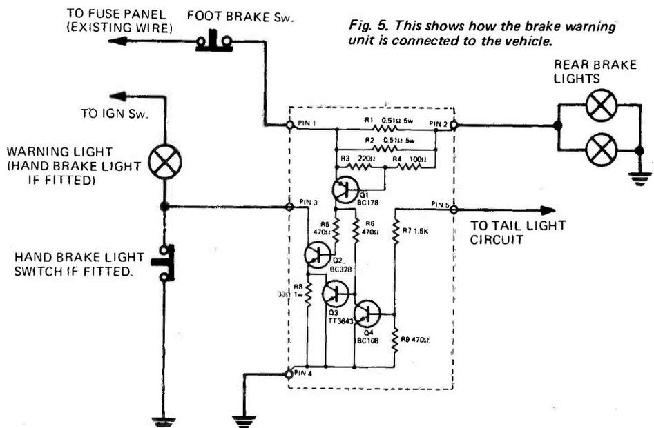
Fig. 5. This shows how the brake warning unit is connected to the vehicle.
