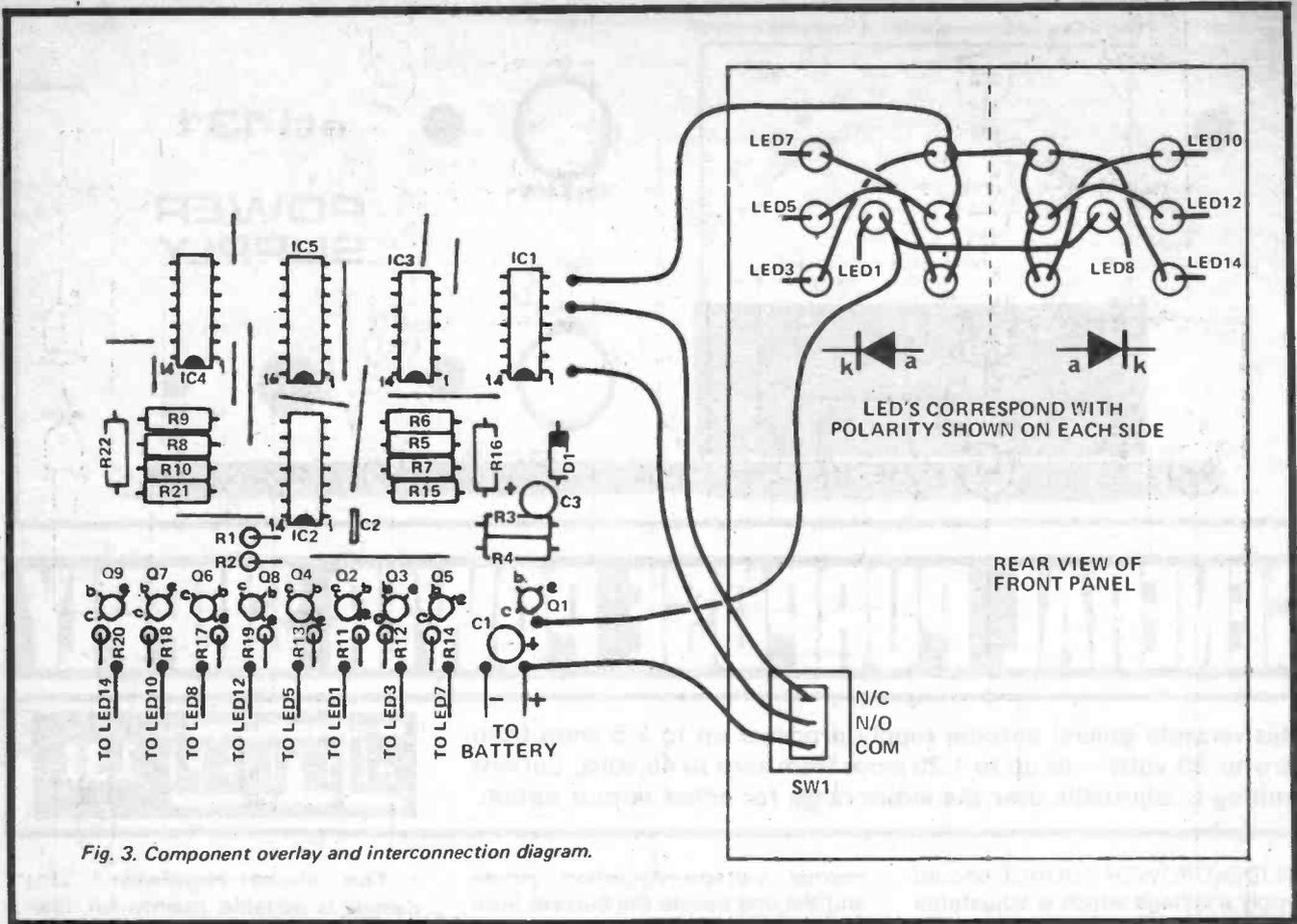
Fig. 3. Component overlay and interconnection diagram.
