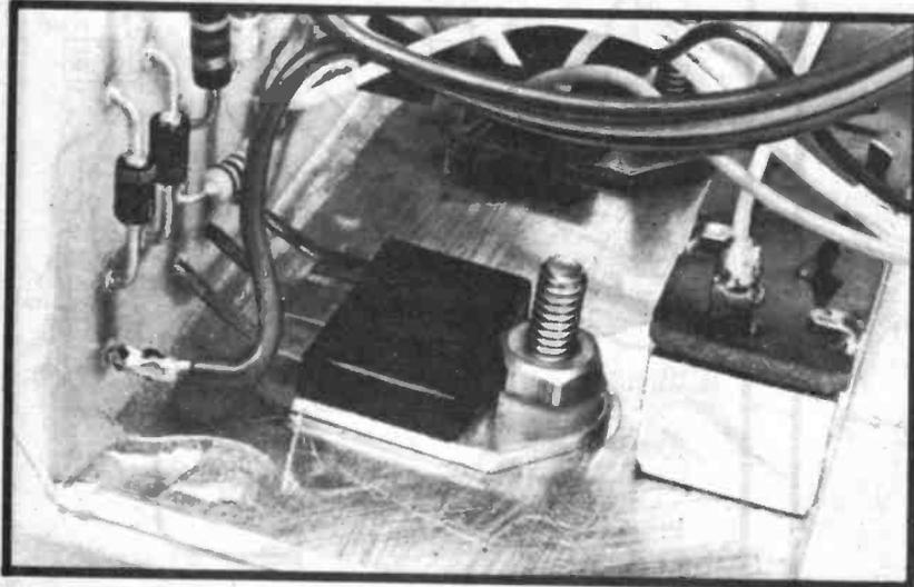
The power transistors are mounted to a bracket with countersink bolts. They can, if desired, be mounted directly on the front panel. Note how the pcb is mounted - by epoxying to the bracket.
