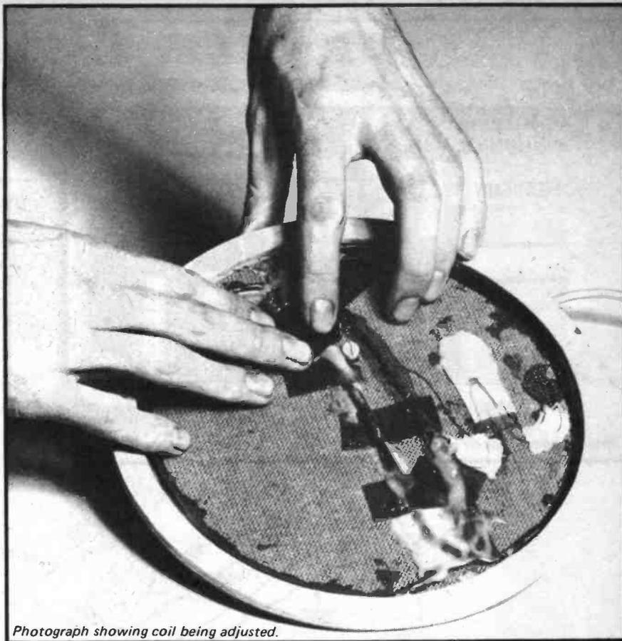
Photograph showing coil being adjusted.
