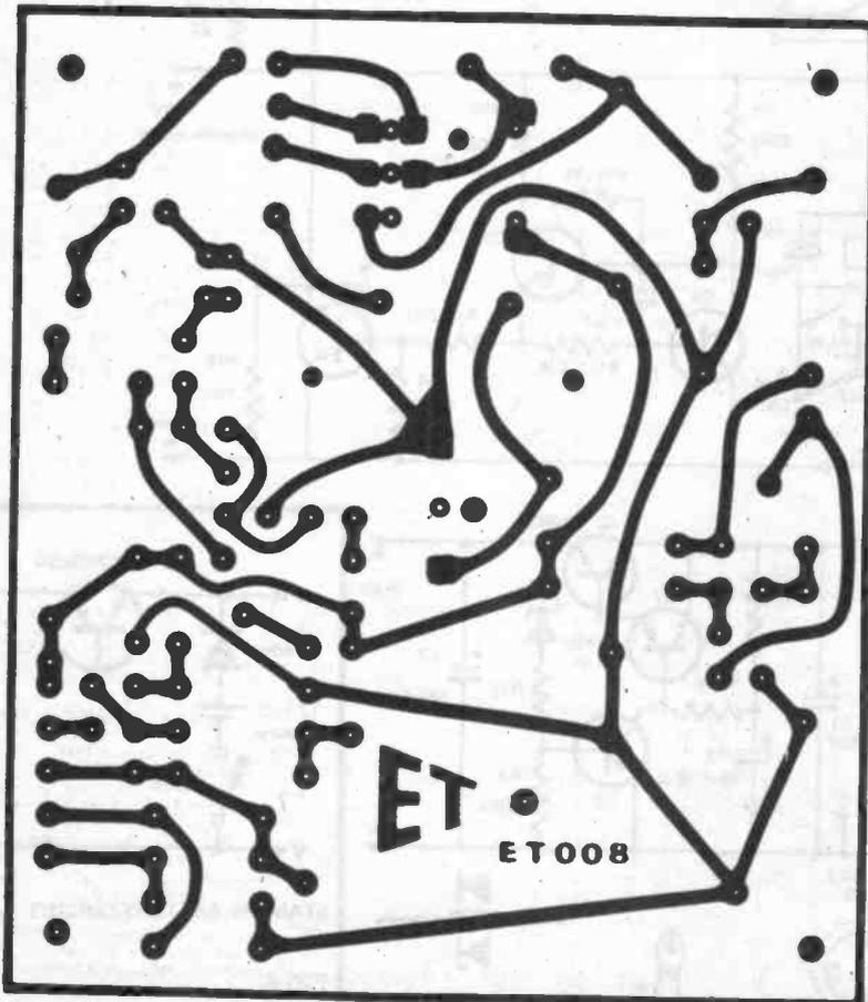
Fig. 5. Foil pattern for printed circuit board - full size.
