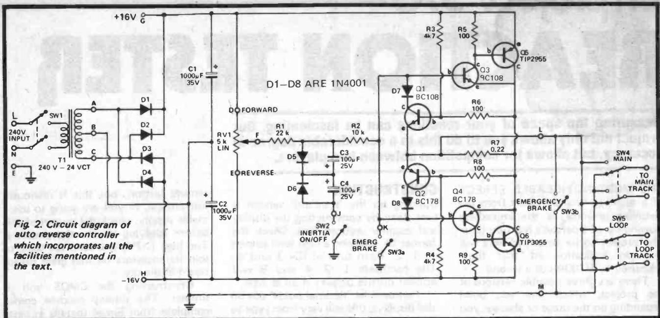
Fig. 2. Circuit diagram of auto reverse controller which incorporates all the facilities mentioned in the text.
