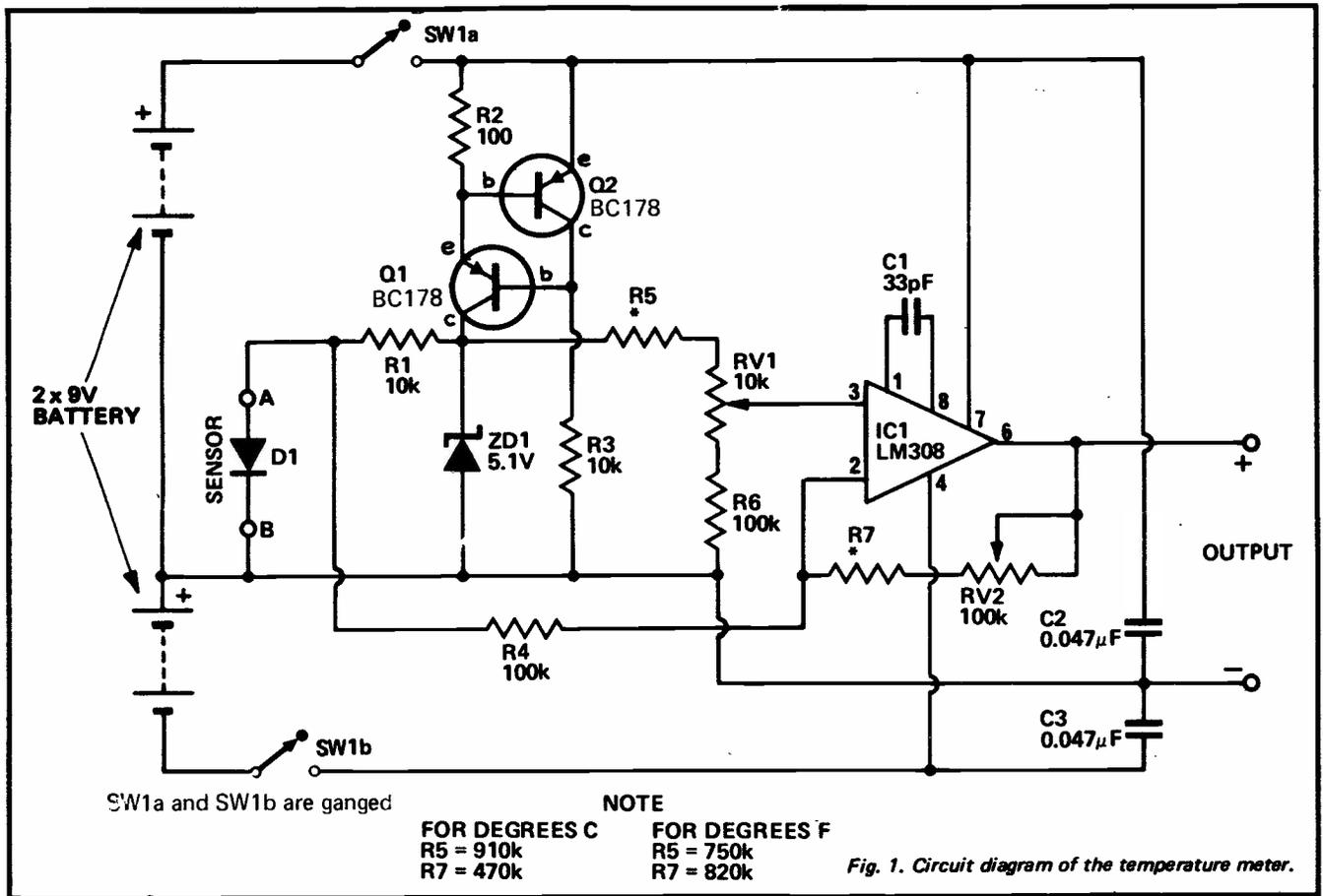
1. Place the sensor and thermometer into the cool solution, allow a little time for stabilisation, and then measure the voltage from the converter and the temperature. Record these two readings.
