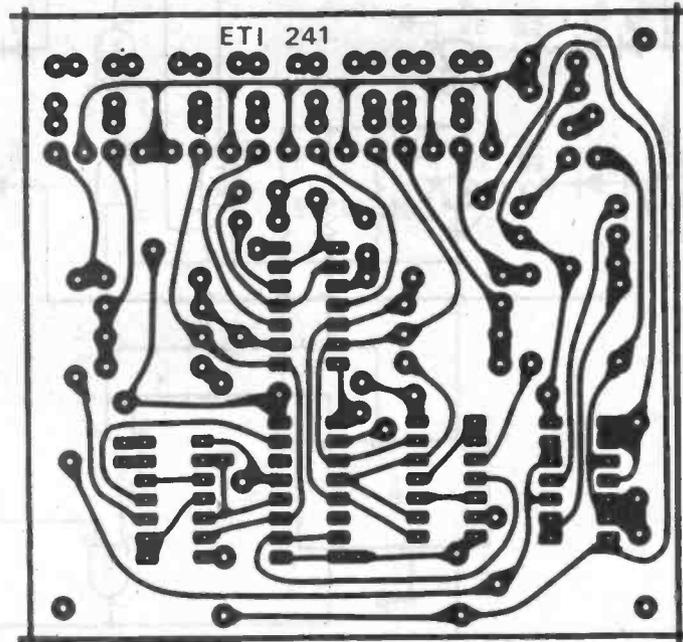
Fig. 1. Printed circuit layout for the double dice. Full size 84 x 81mm.
