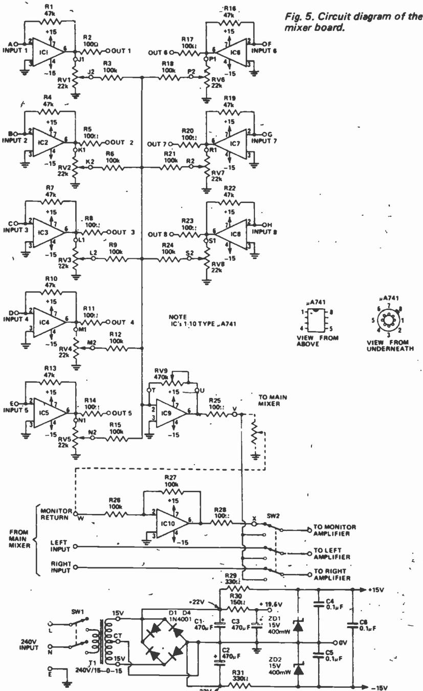
Fig. 5. Circuit diagram of the mixer board.
