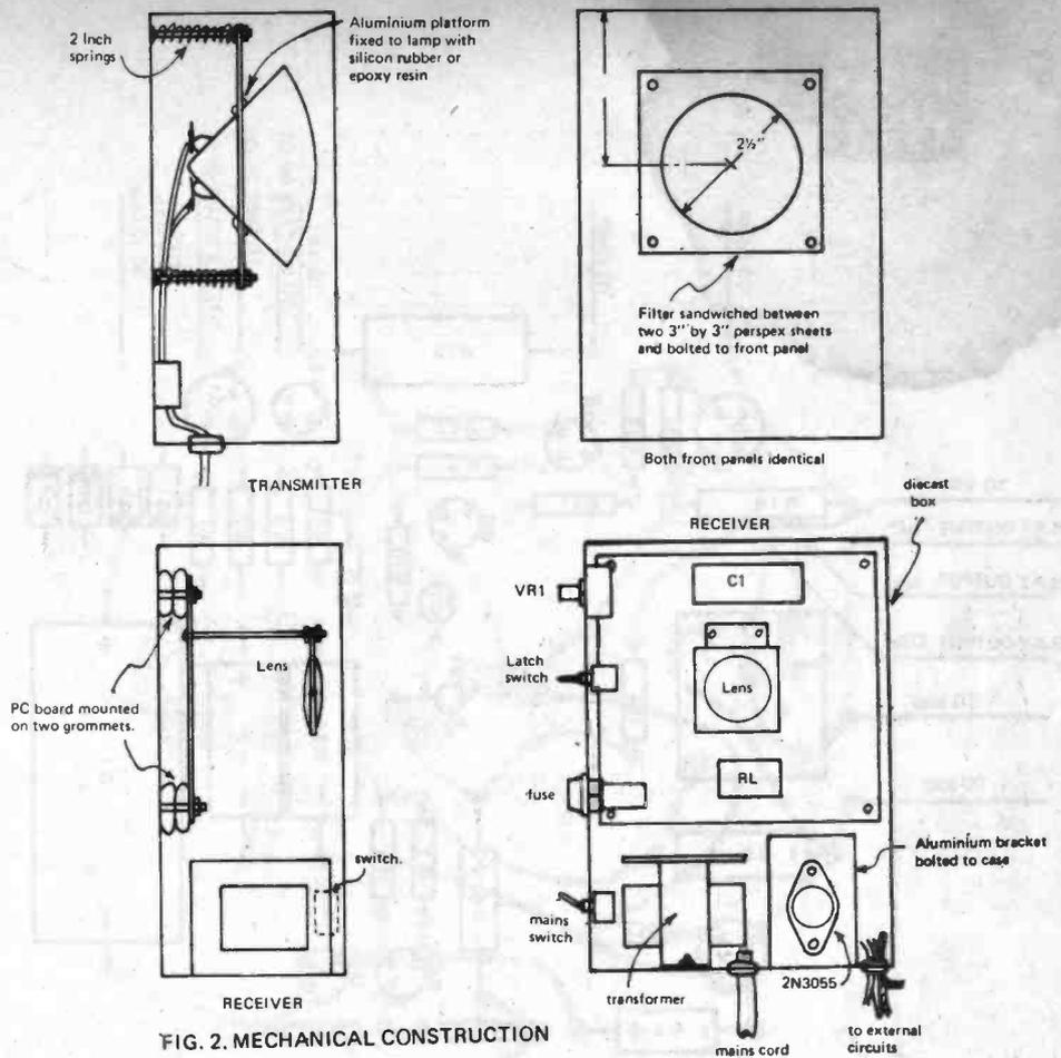
FIG. 2. MECHANICAL CONSTRUCTION
