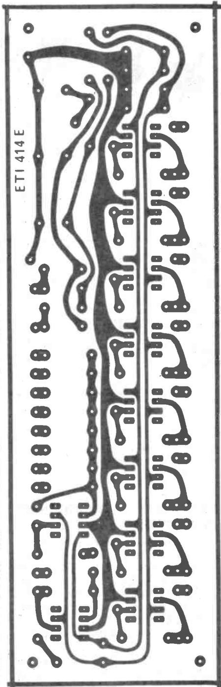
Fig. 6. Printed circuit layout for the mixer/power-supply board. Full size 182 x 57 mm.
