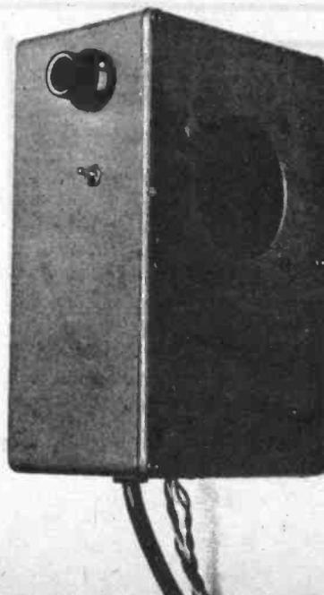
switched off when the beam is not required to be in use. The recommended batteries are two Eveready type 731 in series.
