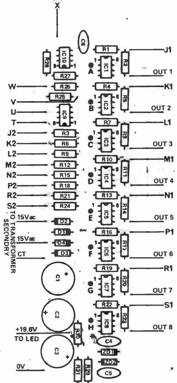
Fig. 7. Component overlay for the mixer/power-supply board.
