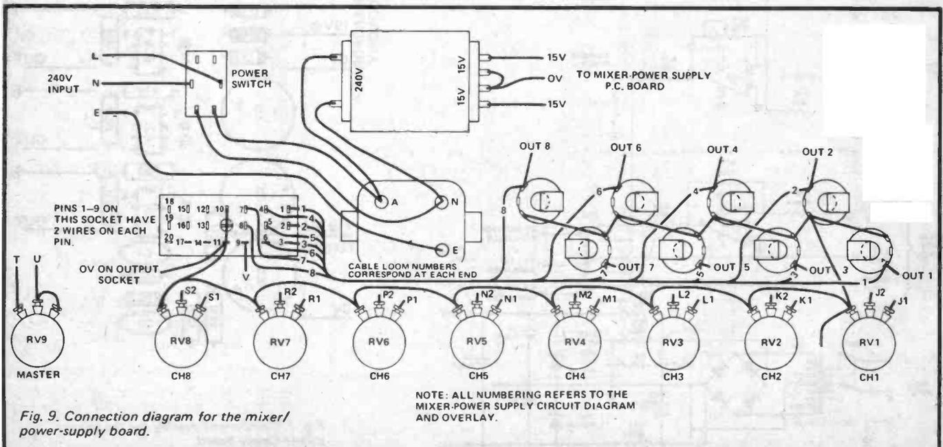
Fig. 9. Connection diagram for the mixer/power-supply board.
