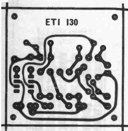
Fig. 4. Printed circuit pattern. Full size 63 x 63 mm.
