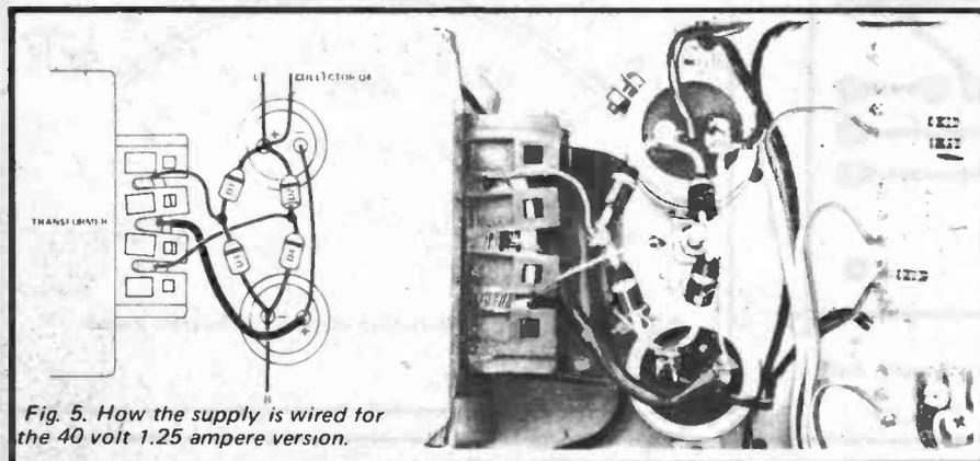
Fig. 5. How the supply is wired for the 40 volt 1.25 ampere version.
