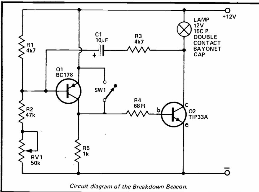
Circuit diagram of the Breakdown Beacon.
