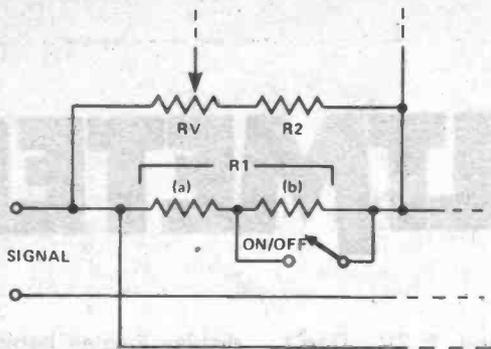
Fig. 2. Circuit modification allowing for two differing load impedances.
