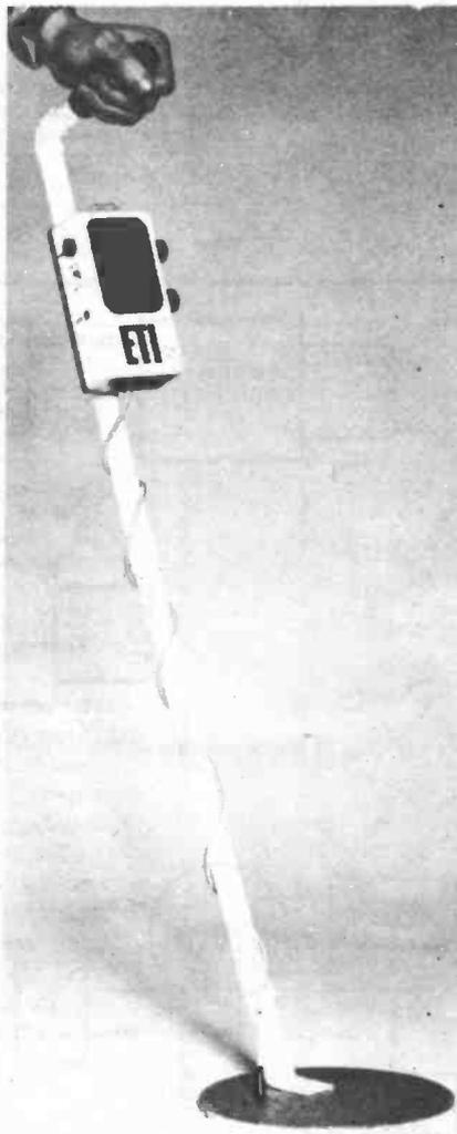
between 100-150kHz. A second internal oscillator operating on the same frequency is included and a tiny part of each signal is taken to a mixer and a beat note is produced. When the search coil is brought near metal, the inductance of the coil is
