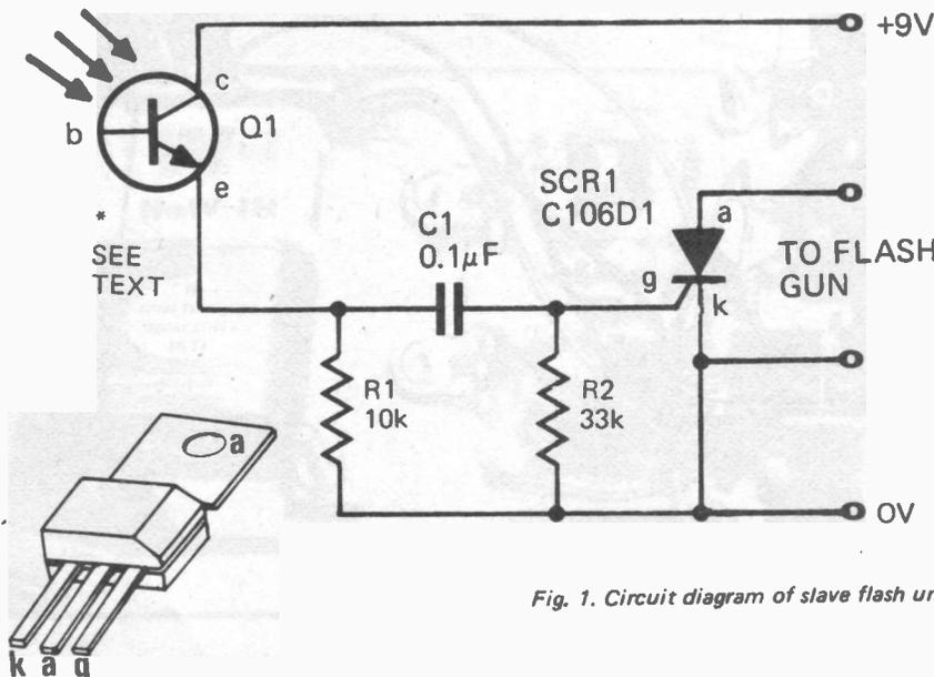
Fig. 1. Circuit diagram of slave flash unit.
