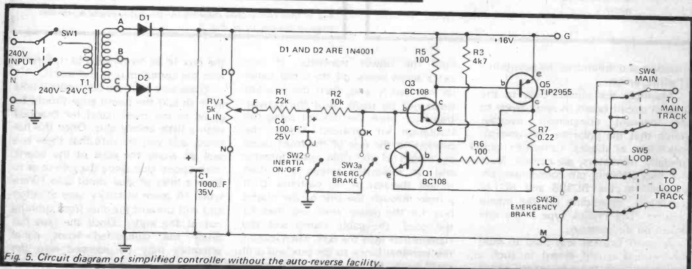
Fig. 5. Circuit diagram of simplified controller without the auto-reverse facility.
