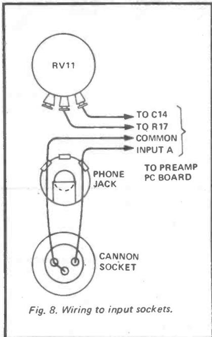
Fig. 8. Wiring to input sockets.
