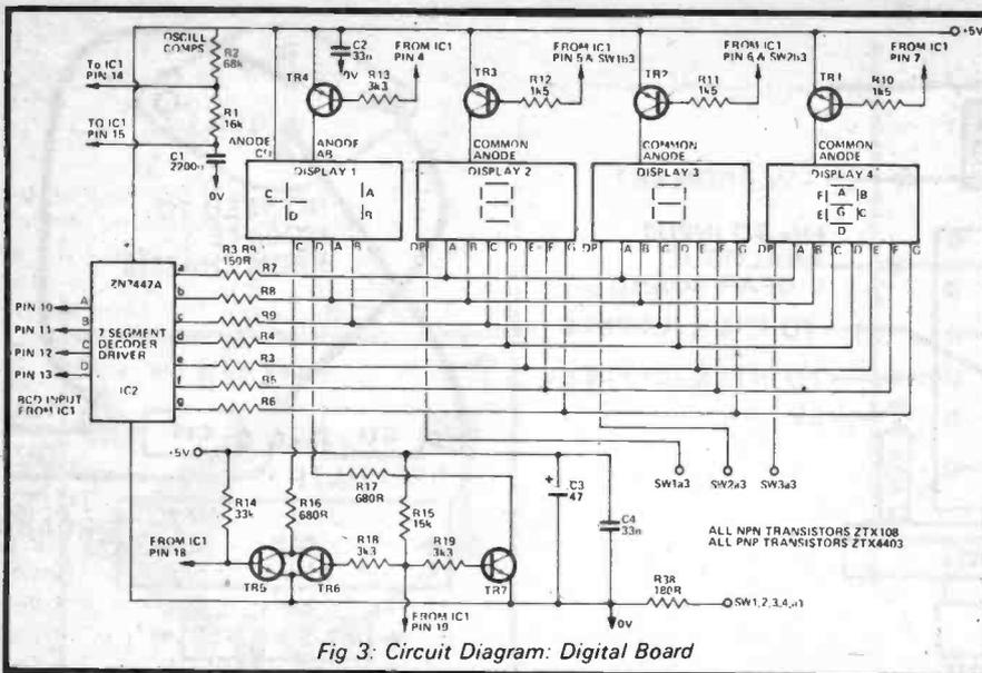
Fig 3: Circuit Diagram: Digital Board
