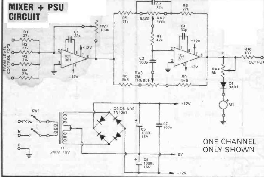
The inputs from the turntables, tape recorders microphones, etc. must be amplified, and if necessary equalized, by a preamplifier before any of the controls can handle them. The output of each of these preamps adjustable, by means of a volume control or fader, before being mixed in IC1. The overall gain of the mixer stage is adjusted by means of RV1. If different preamps have widely differing output voltages the value of R1-R4 can be changed to make them match.
