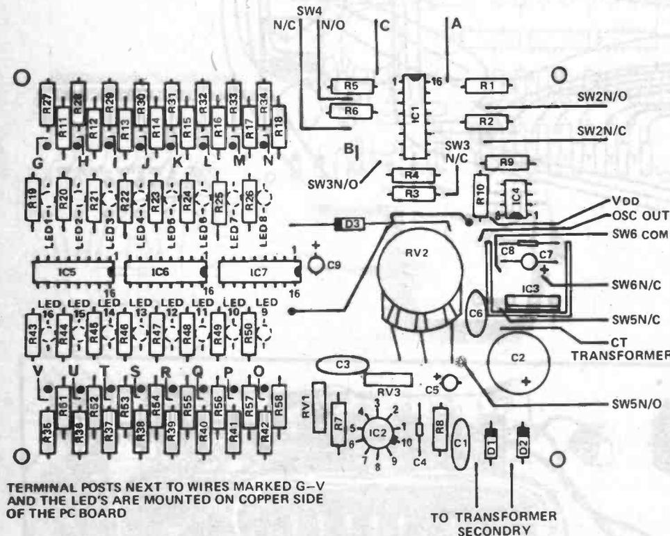
TERMINAL POSTS NEXT TO WIRES MARKED G-V AND THE LED'S ARE MOUNTED ON COPPER SIDE OF THE PC BOARD
