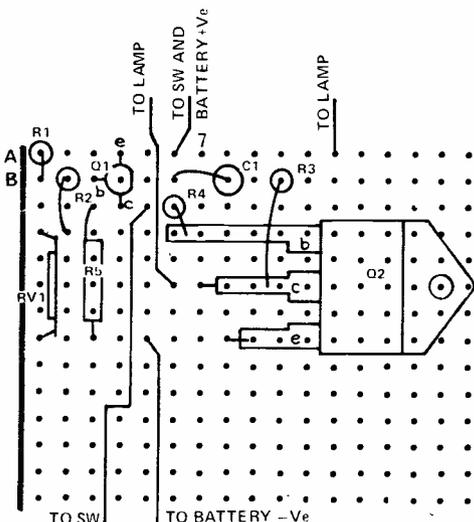
Veroboard layout for the beacon circuit. The copper strips run from left to right across the board. Only one break is required and this is at: B7
