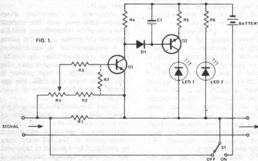
Fig. 1. Circuit of Power Indicator.
