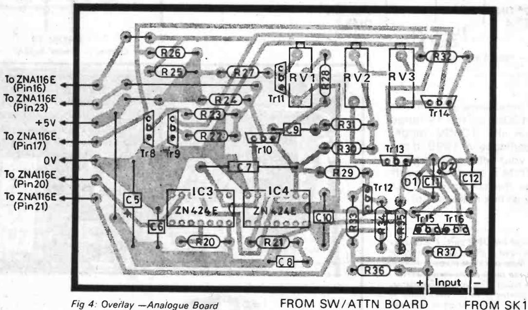
Fig 4: Overlay - Analogue Board
