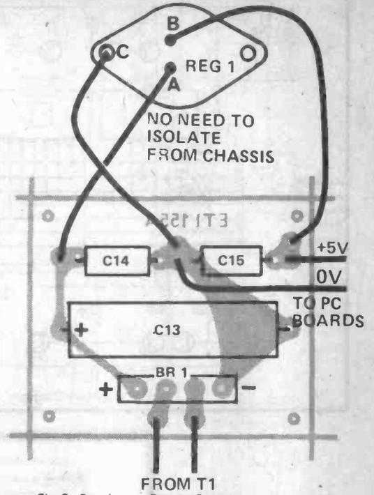
Fig 8: Overlay — Power Supply
