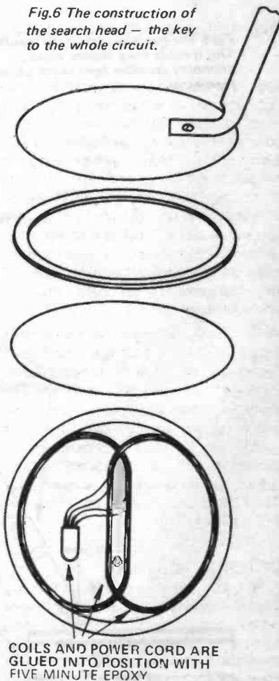
COILS AND POWER CORD ARE GLUED INTO POSITION WITH FIVE MINUTE EPOXY
