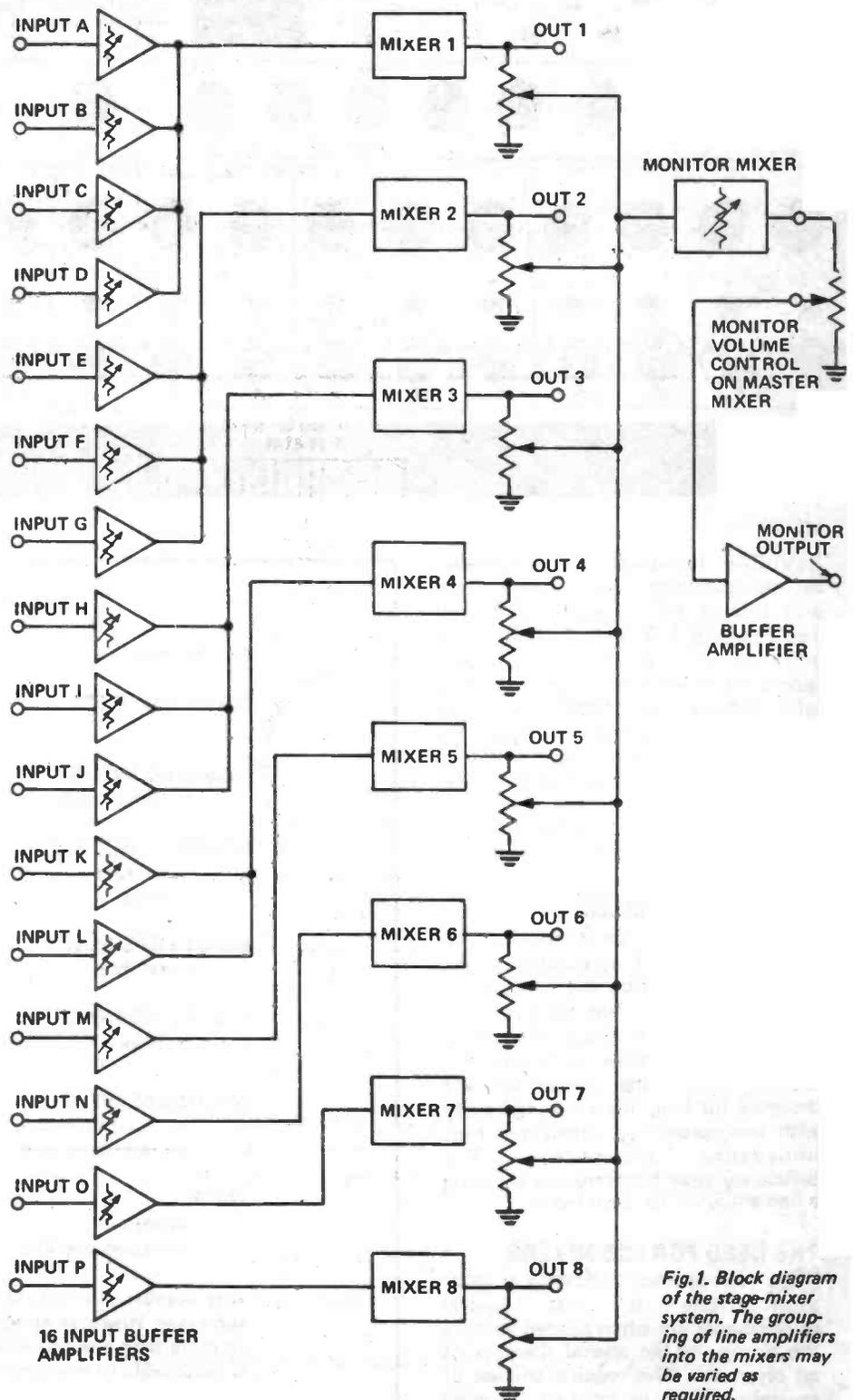
*Fig. 1. Block diagram of the stage-mixer system. The grouping of line amplifiers into the mixers may be varied as required.*
