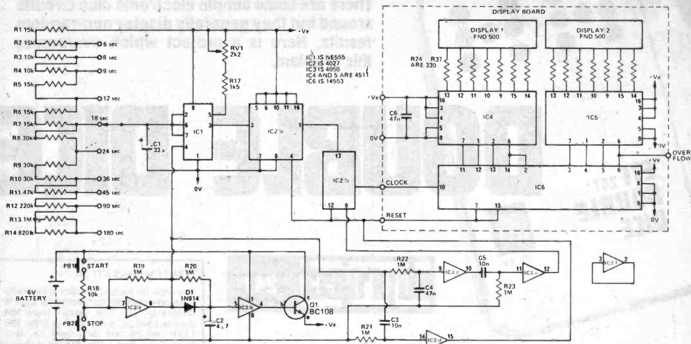
Fig.1 Circuit diagram of the STD timer unit
