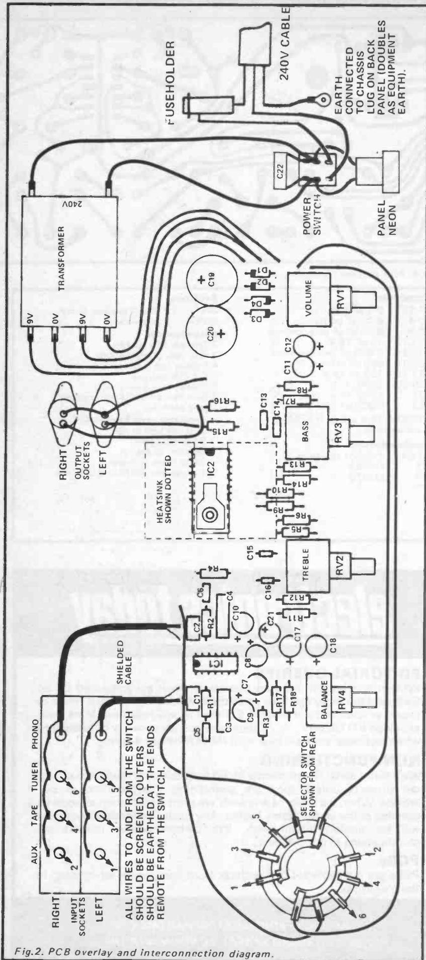
Fig.2. PCB overlay and interconnection diagram.
