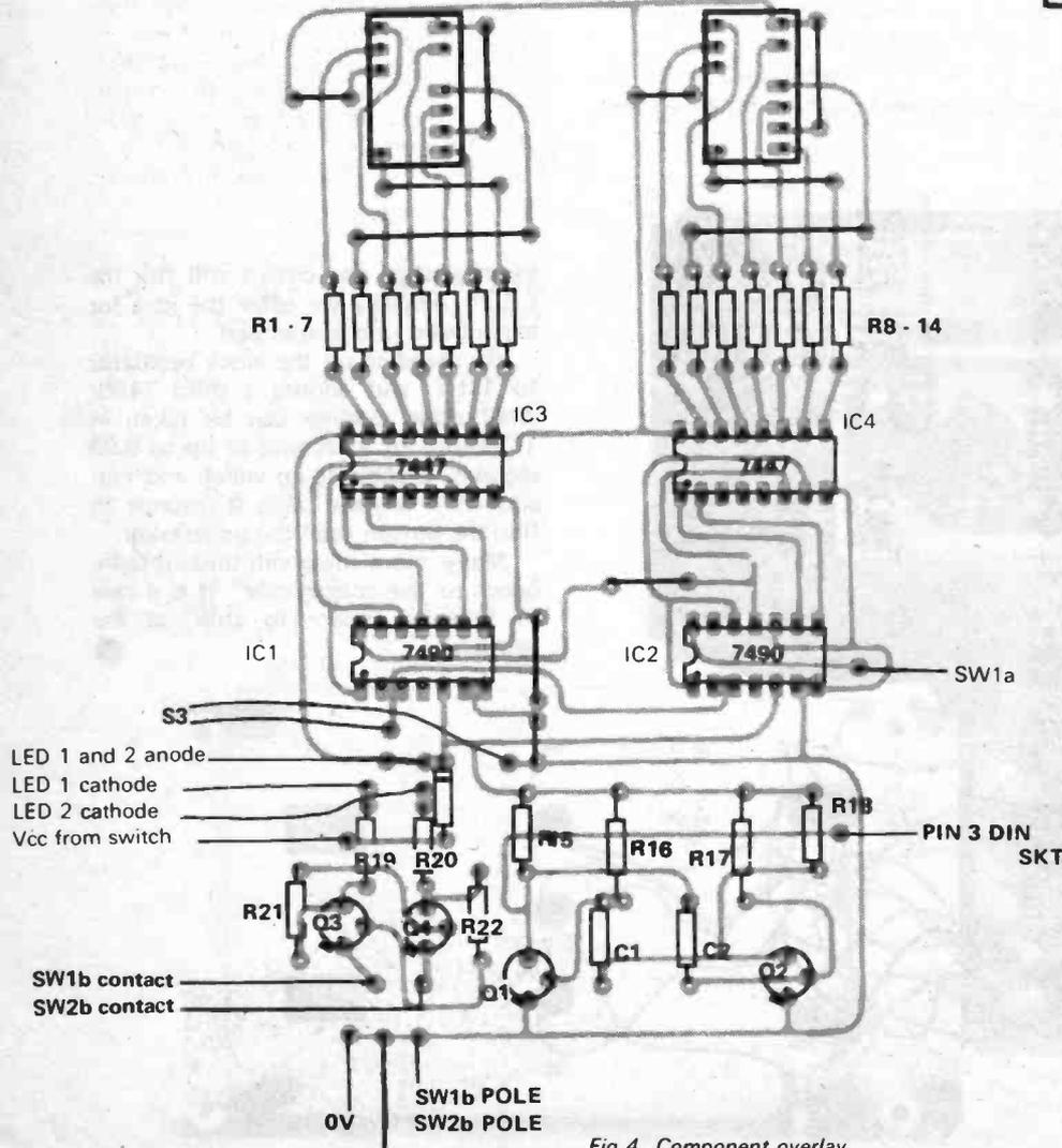
Fig 4. Component overlay.
