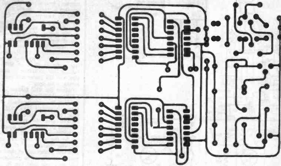
Fig. 2: PCB foil pattern — full size.
