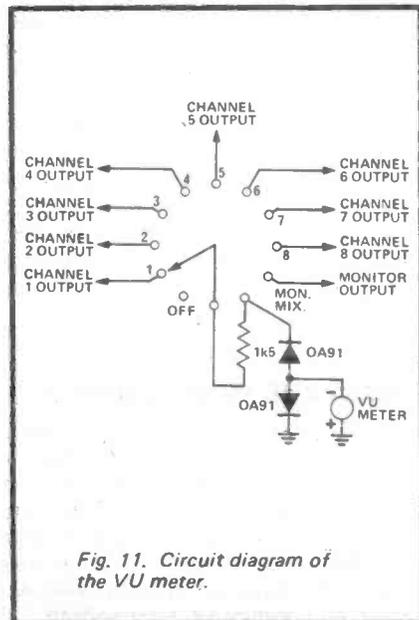
Fig. 11. Circuit diagram of the VU meter.
