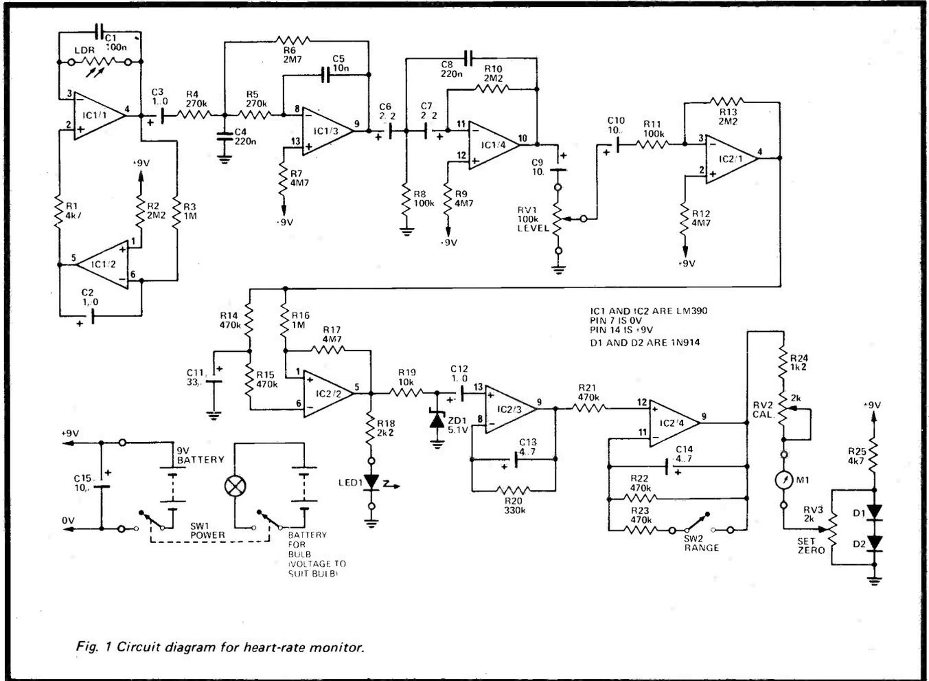
Fig. 1 Circuit diagram for heart-rate monitor.
