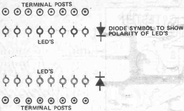
Fig. 4. Positioning of LEDs and terminal posts on the copper side of the printed-circuit board.
