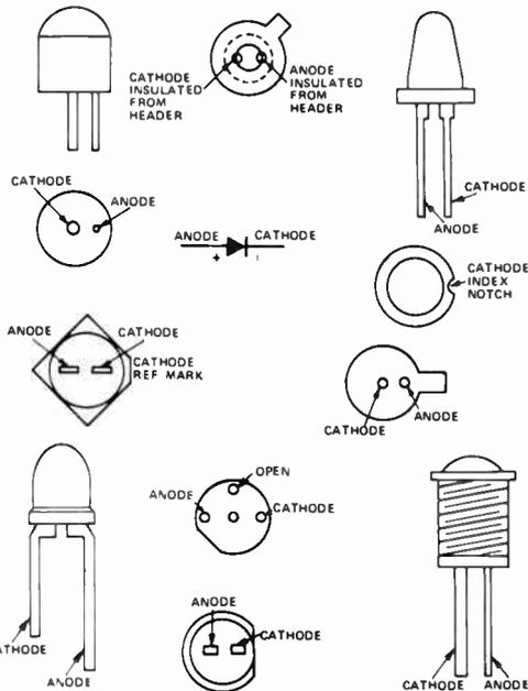
Fig. 12. Common lead connections for LED indicator lamps.
