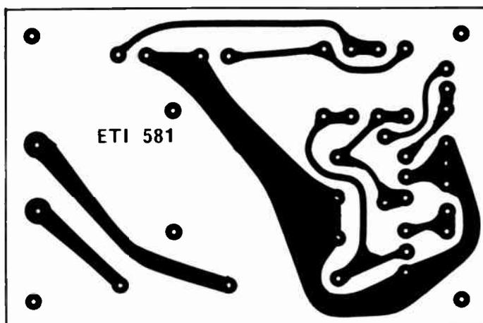
Fig. 1. Printed circuit layout.
