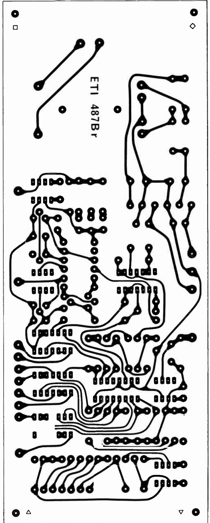
Fig. 9. Both sides of the ET1 487B board shown full size.
