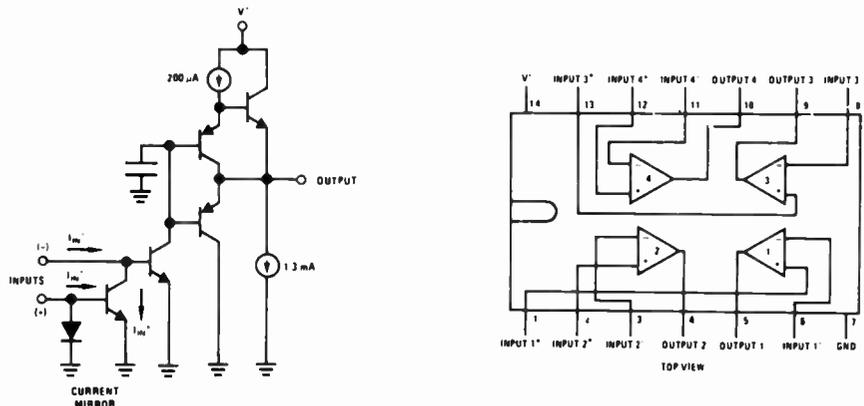
Fig. 4. Internal circuitry and pin connections of the LM3900 IC.
