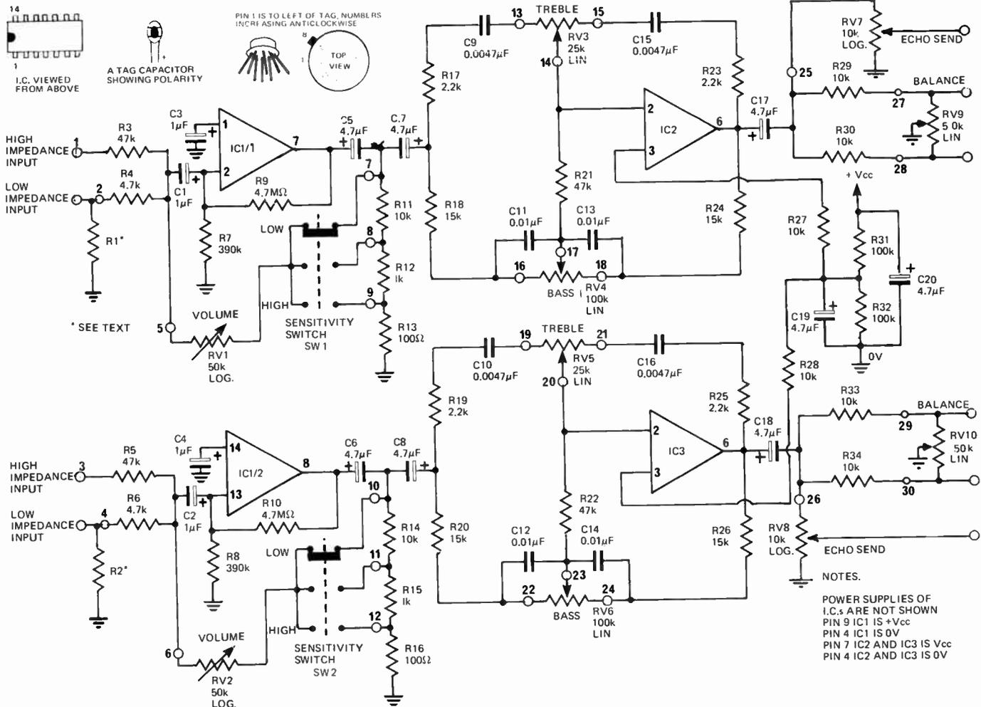
The circuit diagram of one of four identical preamplifier boards. I.C. 1/1 and I.C. 1/2 are in the same package.
