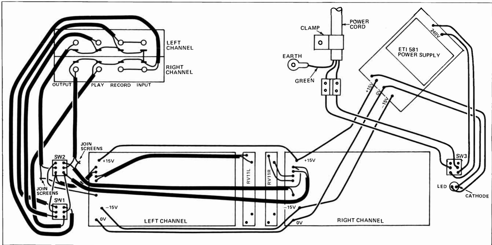
Fig. 6. Interconnection diagram for the unit.
