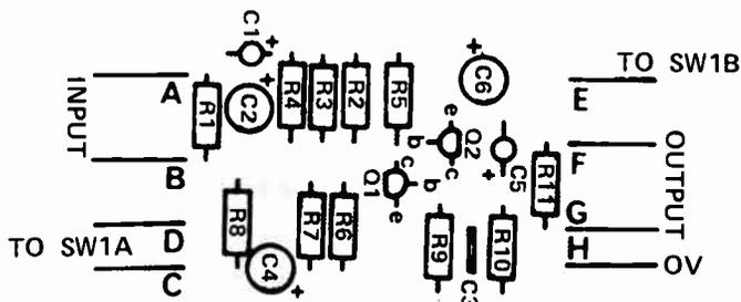
Fig.3. Component overlay. Note particularly the orientation of the transistors and electrolytic capacitors.
