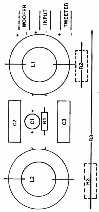
Fig. 6. Component overlay shows how to assemble the crossover network.
