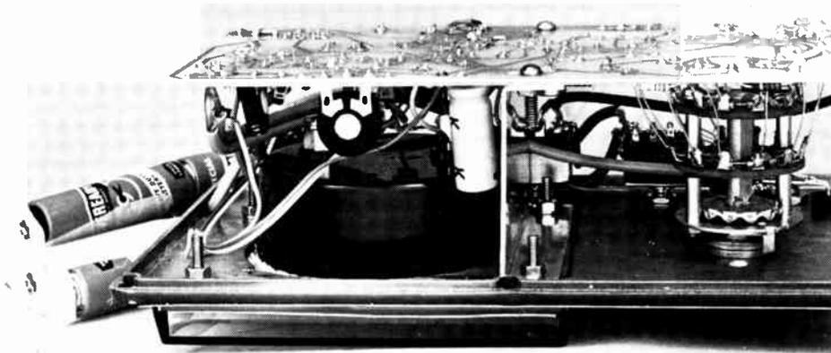
This internal view of the meter shows on the right, how the range switch is wired to the printed-circuit board. Note also the shield.
