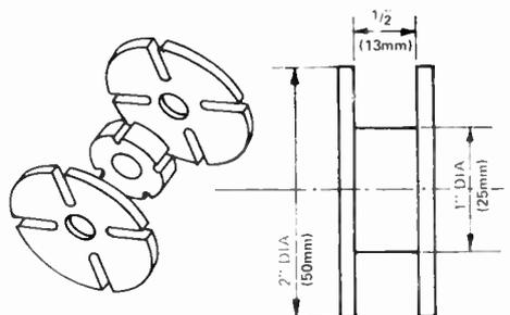
Fig. 4. Former for winding chokes L1 and L2. Chokes may readily be wound by hand, try and keep wire in uniform layers but a little jumbling will not appreciably affect the final value of inductance.
