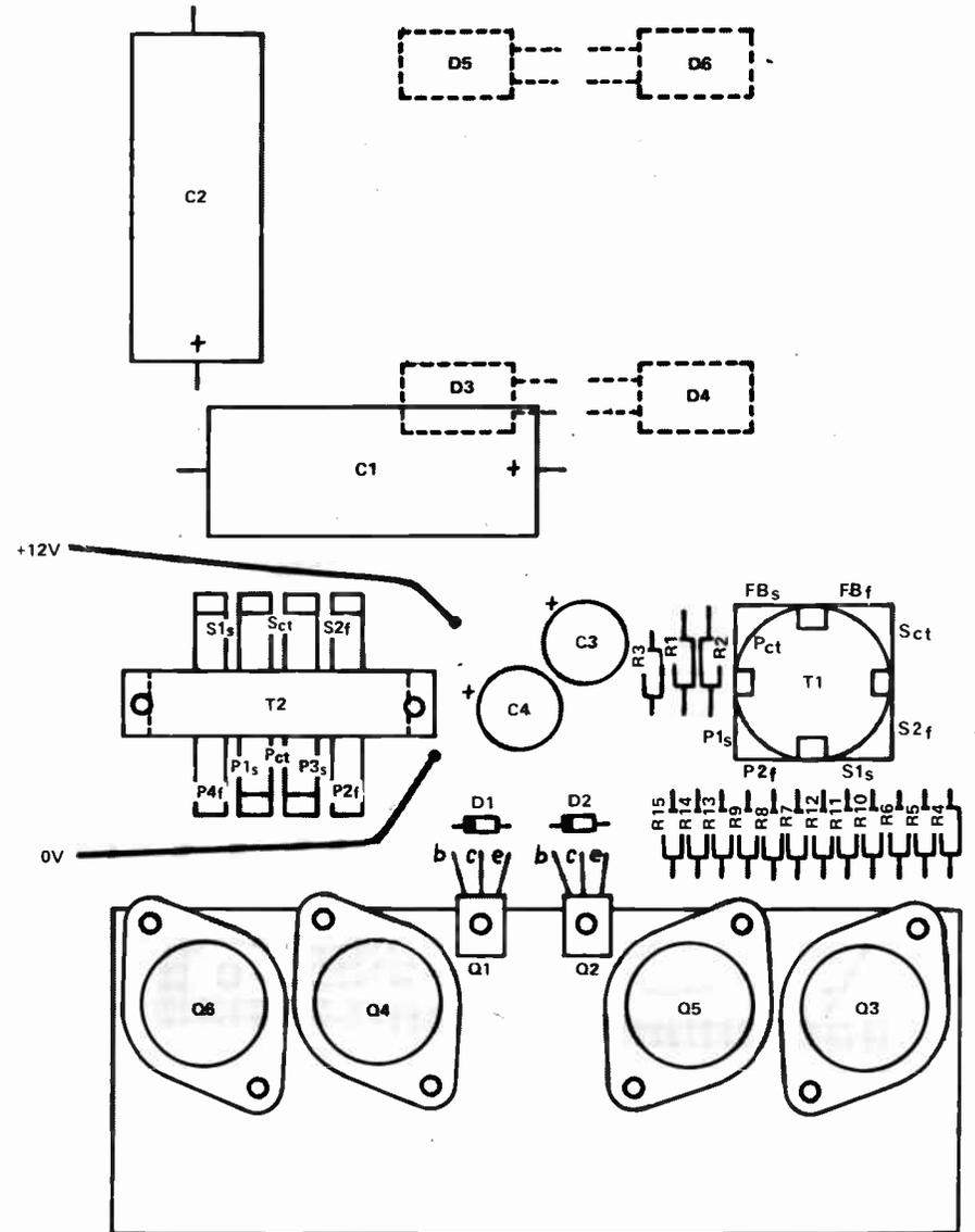
Fig. 4. Component overlay.
