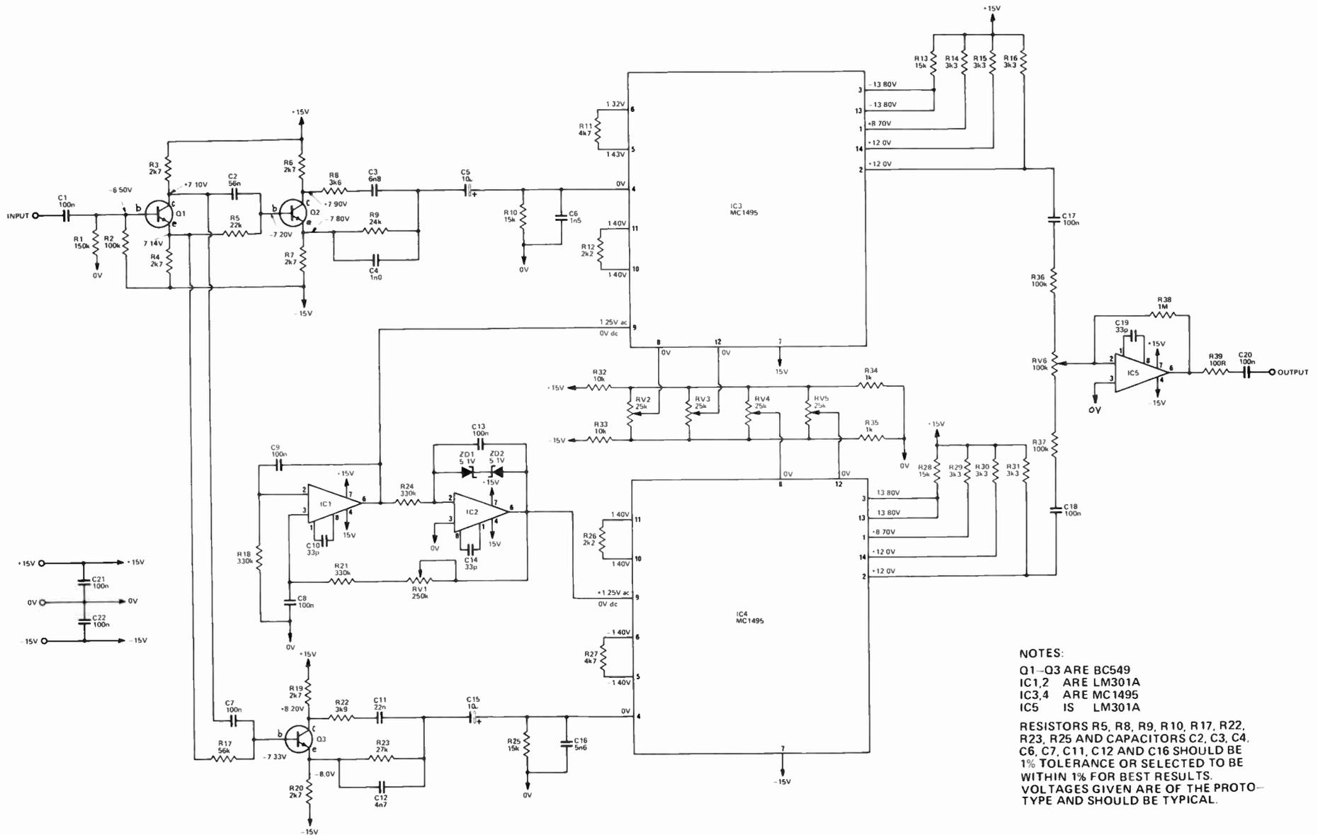
Fig. 1. The circuit diagram of the phase shifter. For the power supply see ETI Project 581 — page 89.
