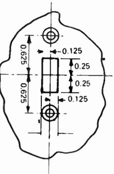
Fig. 11. Cutouts for meters and sensitivity switches.
