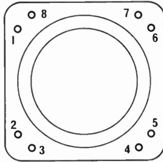
Fig. 5. The pin numbering sequence for T1.
