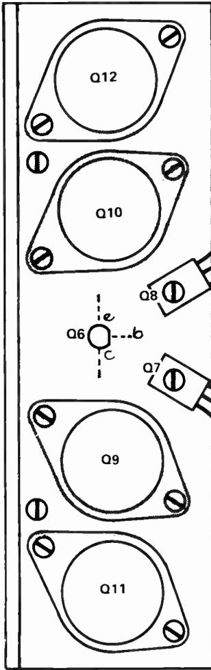
Fig. 5. Component overlay of the 100 W module. For the 50 W version delete Q11 and Q12.
