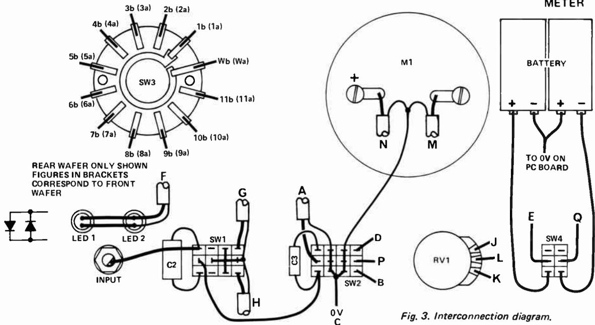
Fig. 3. Interconnection diagram.
