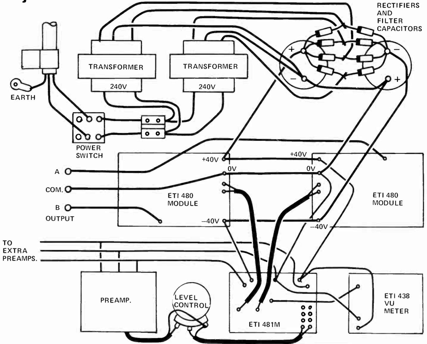
Fig. 4. Wiring diagram for the 200W bridge amplifier.
