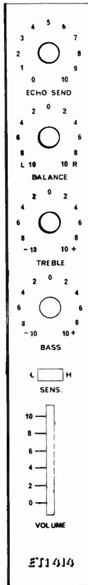
Fig. 4. Escutcheon for preamplifier (actual size 12" x 1 3/4").
