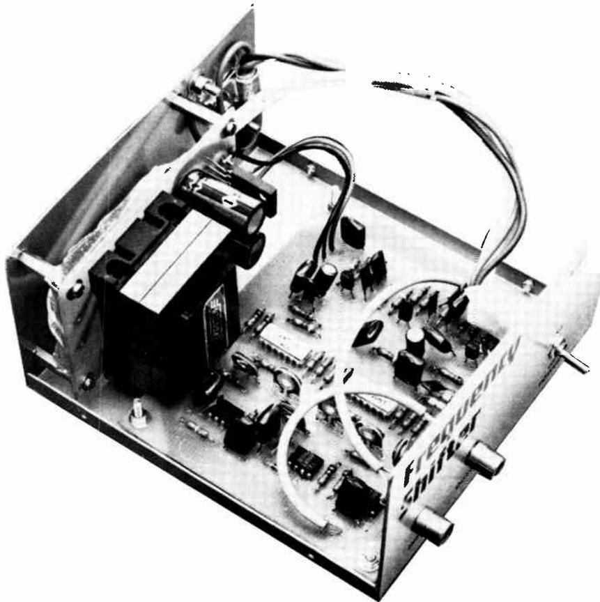
5. With no input signal, measure the output of IC3 (or the junction...) and adjust RV2 for minimum output.
