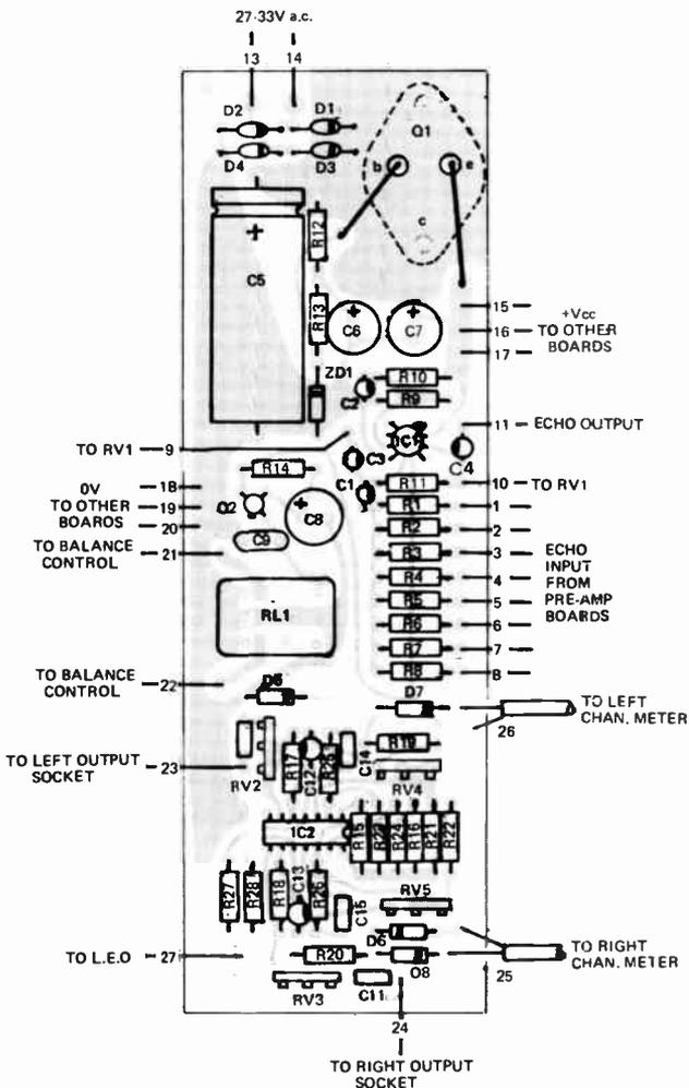
Fig. 3. Component overlay of power supply board.
