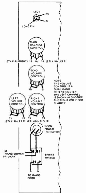
Fig. 7. Wiring to rear of main control panel.
