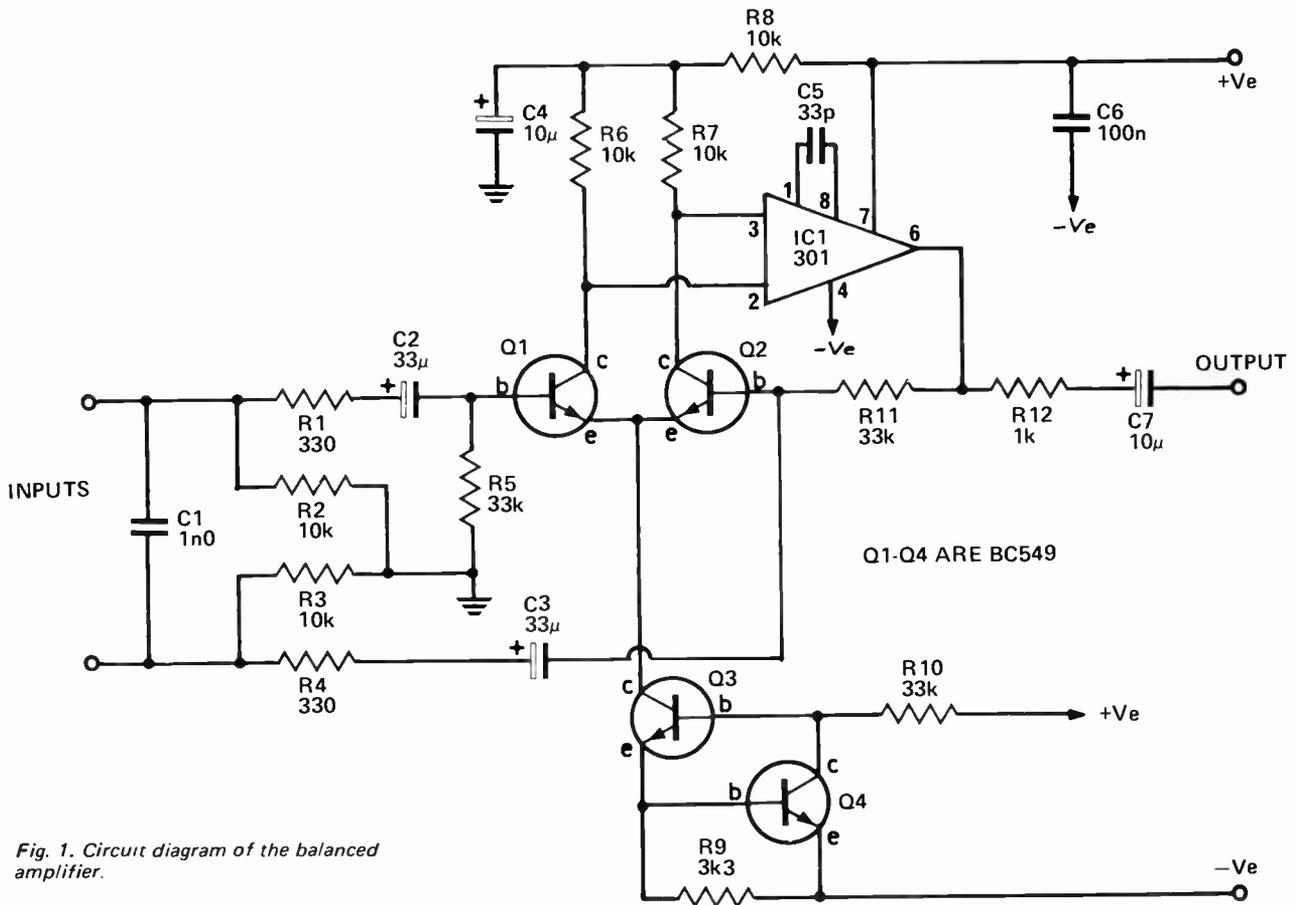
Fig. 1. Circuit diagram of the balanced amplifier.
