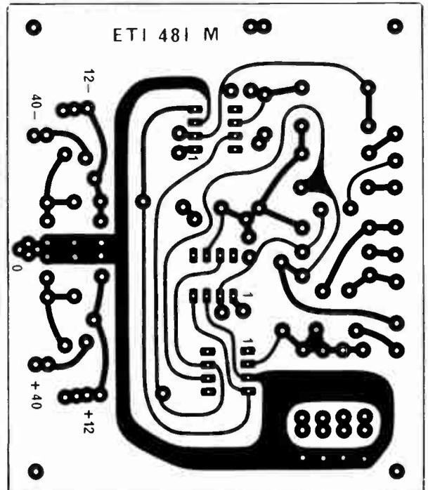
Fig. 5. Printed circuit layout. Full size 92 x 78 mm.
