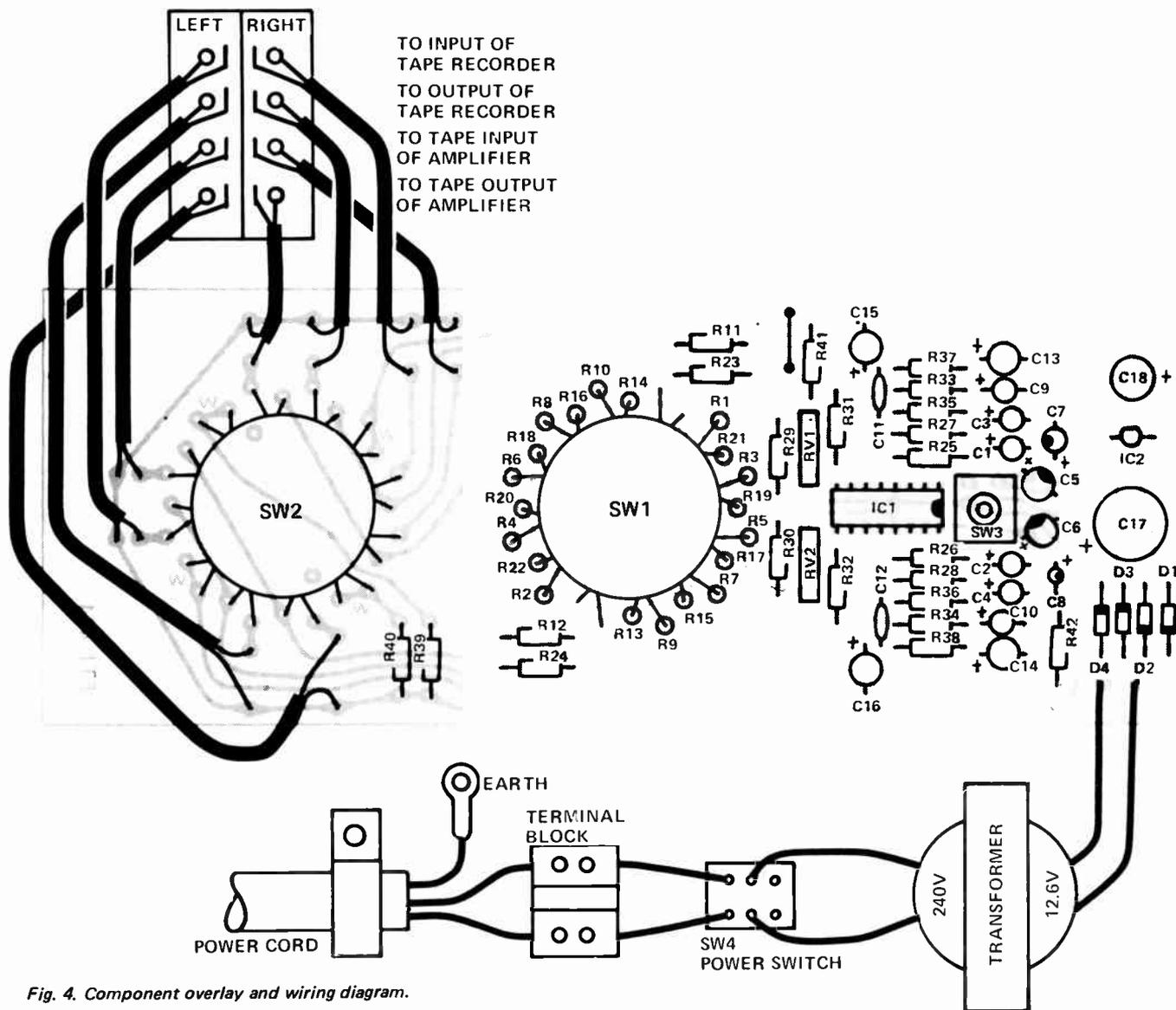
Fig. 4. Component overlay and wiring diagram.
