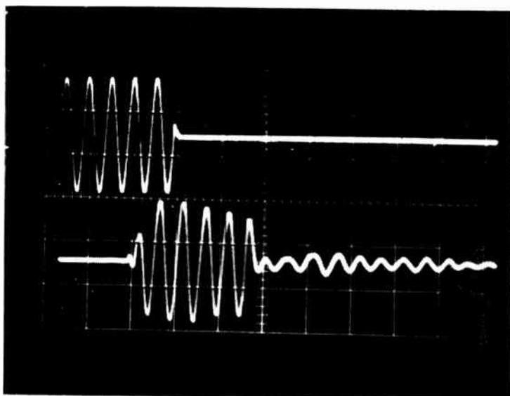
Fig.5 (a) Top trace – the input tone burst of five cycles. (original design).
