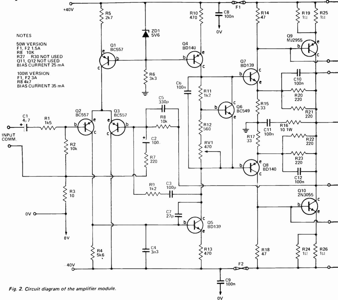
Fig. 2. Circuit diagram of the amplifier module.
