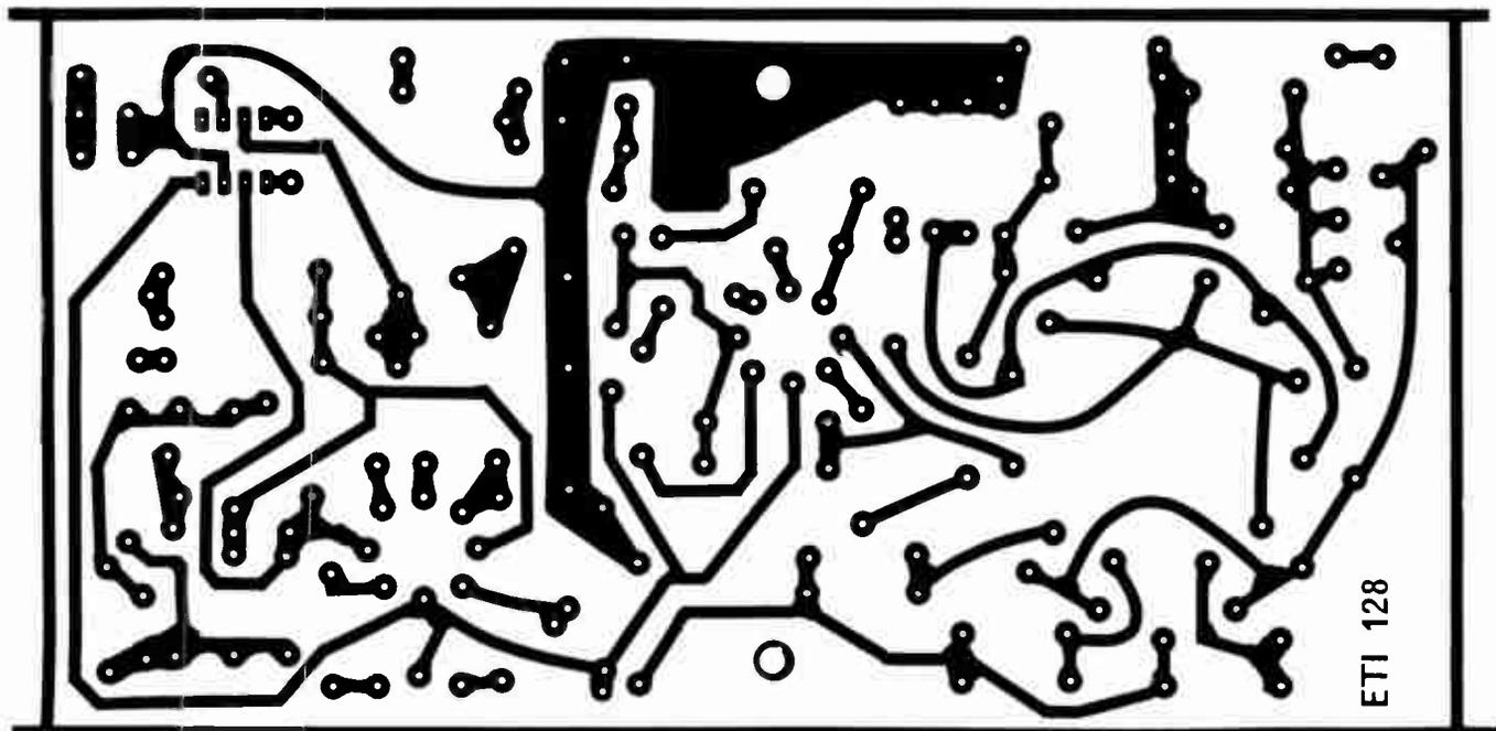
Fig. 5. Printed circuit layout. Full size 170 x 87 mm.
