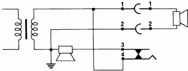
Fig. 1a. Example of using the type 05 connector inserted in position A. Both speakers are operational.
