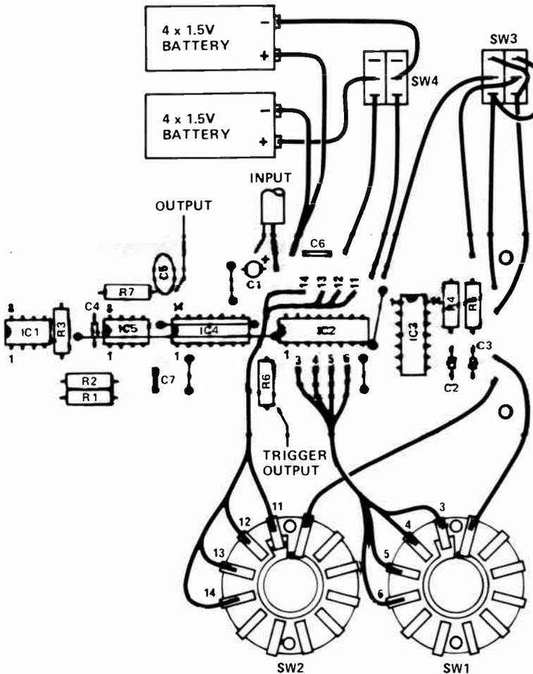
Fig. 2. Component overlay and interconnection diagram. Note that there are six links on the board, including two under IC4, which should be installed first.
