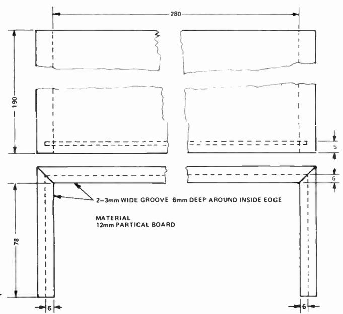
Fig. 8. Cover used on the unit.
