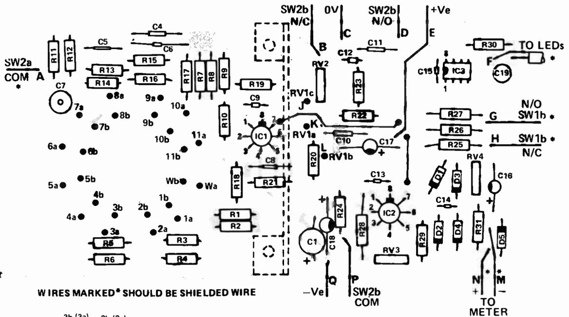
Fig. 2. Component overlay.
