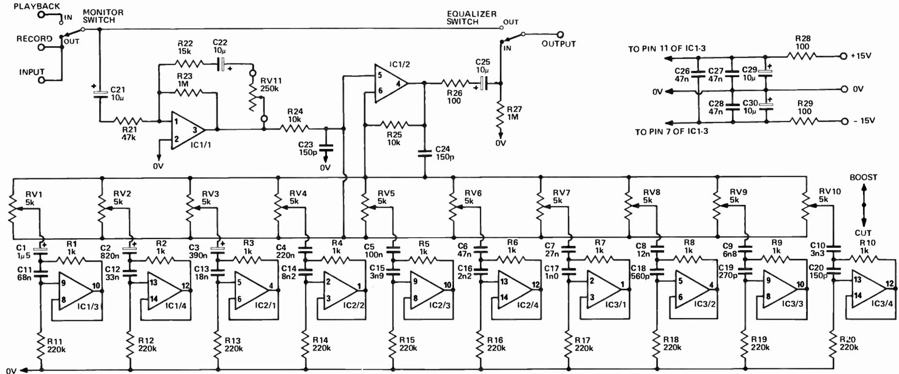
Fig. 1. Circuit diagram of one channel of the equalizer.
