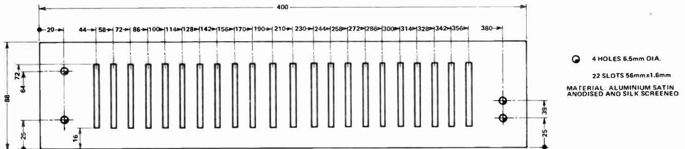
Fig. 8. Metalwork details of the front panel.
