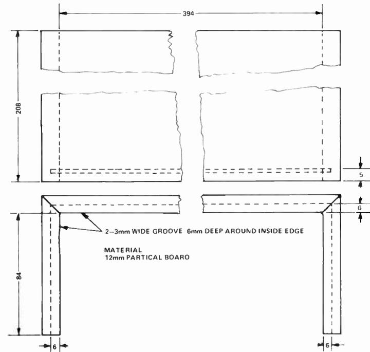
Fig. 4. Constructional details of the cover.
