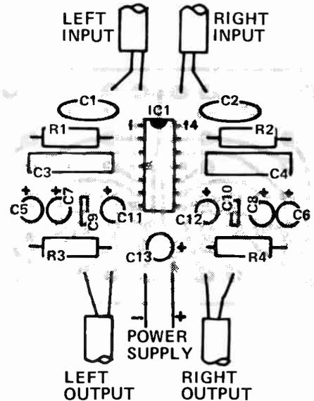
Fig. 4. Component overlay.
