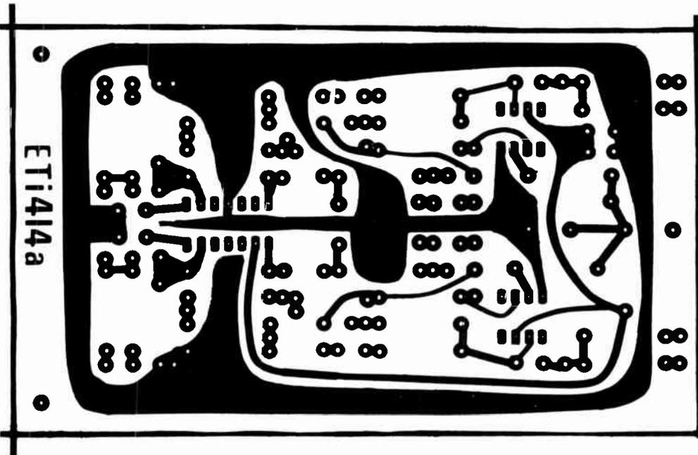
The printed circuit board pattern for the pre-amplifier sections — shown full size.
