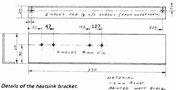
Fig. 10. Details of the heatsink bracket.
