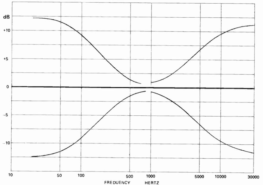
Fig. 6. Tone control characteristics of the amplifier.
