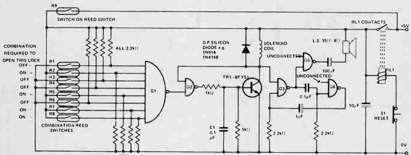
NOTE G1 - SN7430 8 INPUT NAND GATE I.C. G2,G3,G4,G5 - SN7400 QUAD 2 INPUT NAND GATE I.C.
