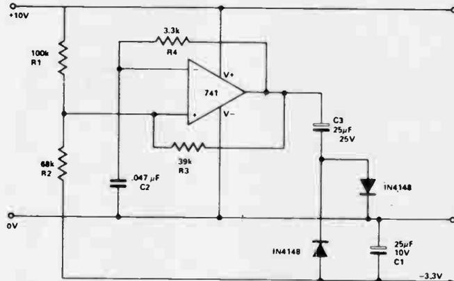
the operating range of the oscillator is pulled down until it is outside the operational range of the 741, and the charging ceases. This provides a form of switching regulation of the output voltage, roughly halving the output impedance. The output voltage can be
