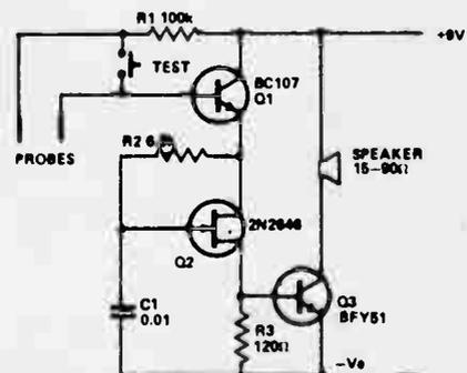
Almost any NPN silicon transistors can be used for Q1 and Q3 and almost any unijunction for Q2.
