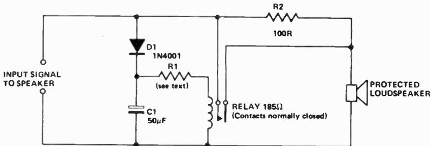
R1 is adjusted to give adequate protection at whatever power is being used. Resistor R1 value should be selected according to the power at which the speaker will need to be
