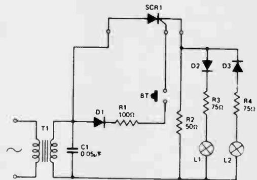
With a good SCR, lamp L1 (6.3 volt 0.25A) will come on, and stay on, only whilst push button BT is depressed. If Lamp L1 comes on before the push button is pressed the thyristor defective - most probably due to an internal short.
