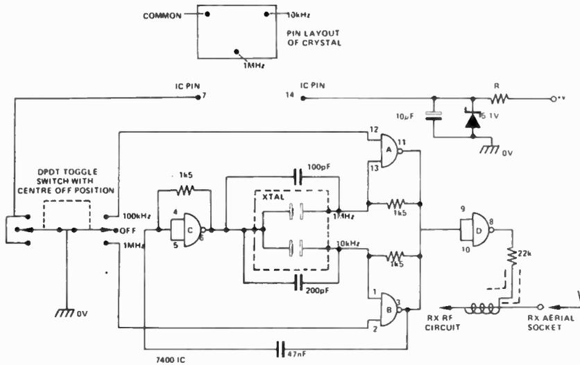
This circuit was designed to make use of an old 100kHz–1000kHz 10X, 3 pin twin crystal.
