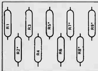
REED SWITCHES ARE SHOWN IN ONE ROW IN CIRCUIT DIAGRAM BUT SHOULD BE WIRED AS SHOWN ABOVE TO AVOID CROSS TRIGGERING BY CLOSE REED MAGNETS
