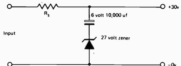
Electrolytics combining large capacity and high working voltage are bulky, expensive, and frequently difficult to obtain.
