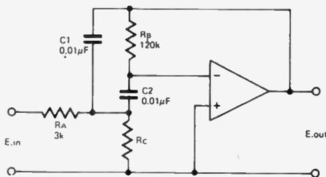
A simple bandpass filter may be constructed using an op-amp and a few discrete components. The circuit shown has a constant gain and bandwidth, and the centre frequency may be adjusted from 1.6 kHz to 2.4 kHz by changing  $R_c$  from 1100 ohms to 400 ohms. Gain is 26dB at centre frequency and bandwidth is 775 Hz at 10dB down.
