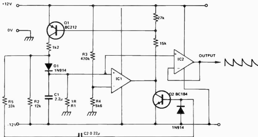
IC1 - An open-collector O/P comparator, eq LM339. IC2 - 741 or similar.
