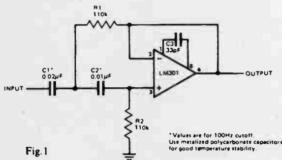
ACTIVE RC filters using operational amplifiers are increasingly being used to supplant LC filters because of the small size and ever-decreasing cost of integrated circuit operational amplifiers. Here are two useful general purpose circuits which may be readily incorporated into other circuitry where needed.
