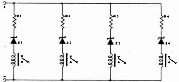
This circuit provides sequential closing of a relay series by appropriately increasing an applied voltage.
