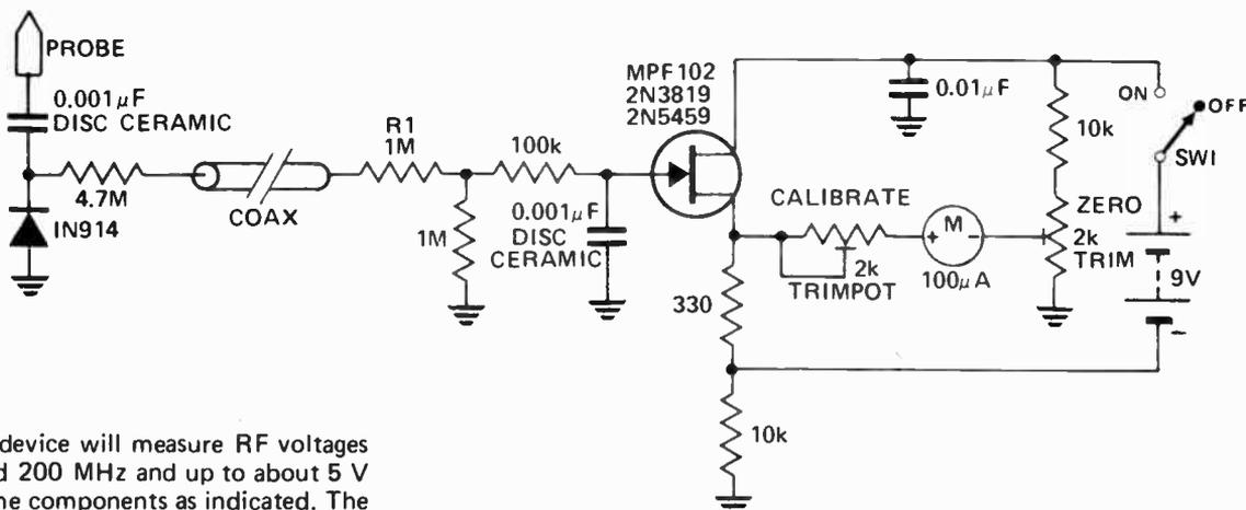
This device will measure RF voltages beyond 200 MHz and up to about 5 V with the components as indicated. The diode etc should be mounted in a remote probe, close to the probe tip. Sensitivity is excellent and voltages less than 1 V peak can be easily measured. The unit can be calibrated by connecting input to a known level
