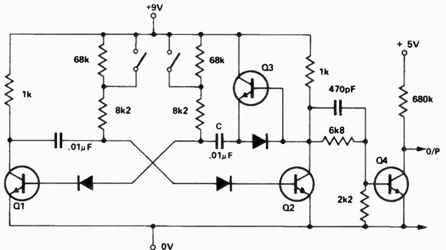
output is used for driving TTL the collector load must be returned to a voltage no greater than +5V.
