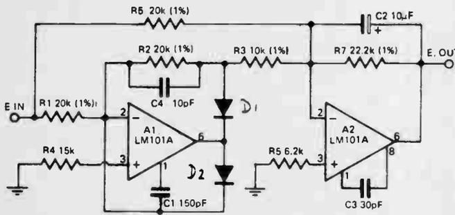
The circuit shown provides better than 1% conversion accuracy of ac signals up to 100 kHz. The output is calibrated to read the rms value of the sine-wave input with less than 1% ripple at 20 Hz.
