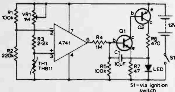
The figure shows a general purpose 741 op amp acting as a sensitive level amplifier of the voltage across the points X and Y of the bridge circuit. Resistors R1 and R2 set the inverting terminal (2) of the op amp at about 6V with respect to ground. The voltage at the non-
