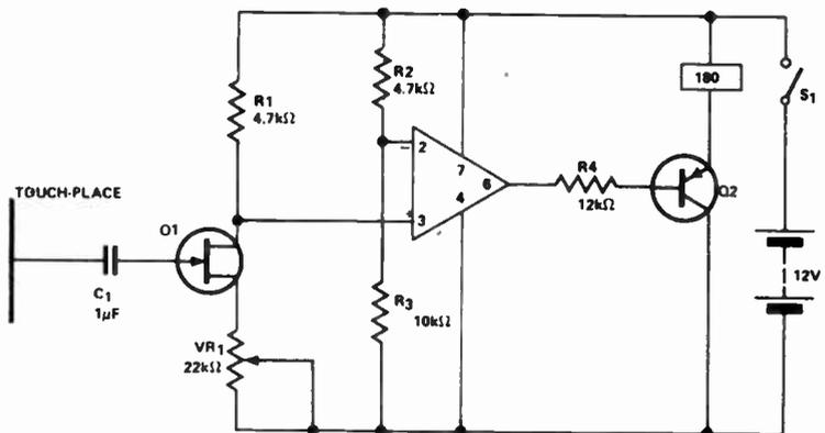
voltage drop across R1 lowers the voltage at pin 3 below that at pin 2. The voltage at pin 6 falls and switches on the relay via Q2. Resistor R4 may need to be selected to ensure that the relay is held off since a small positive voltage at the output remains even though the voltage at pin 3 is lower than that at pin 2 in the quiescent state. This problem can be overcome by using dual power supply for the op-amp in the more usual mode of
