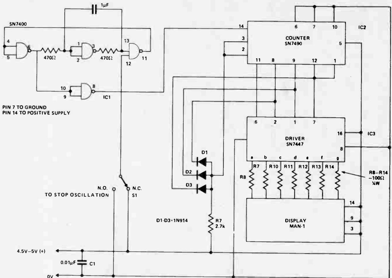
This device is based on a multivibrator (IC1) which has a frequency of about 1kHz. Oscillation continues as long as the input to pin 12 is high; as soon as the input is taken low or connected to earth it stops the cycle. This is used as
