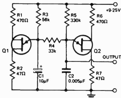
This circuit will produce a continuous sequence of increasing frequencies (in steps) until the highest is reached. The system then resets itself and starts again. Two unijunction relaxation oscillators are cross-coupled together. On switching on capacitors C1 and C2 start to charge up through R3 and R5. The time constant C2-R5 is shorter; Q2 fires first and discharges C2. As C2
