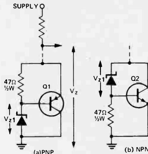
$$V_{z1} = V_z - V_{be}$$
