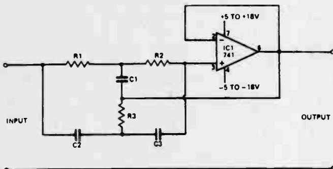
This narrowband filter using the 741 operational amplifier can provide up to 60 dB of rejection. Setting resistors equal to 100 k and capacitors equal to 320 pF the circuit will reject 50Hz.
