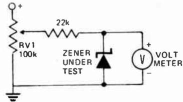
Unmarked Zener diodes may be tested using this simple circuit.
