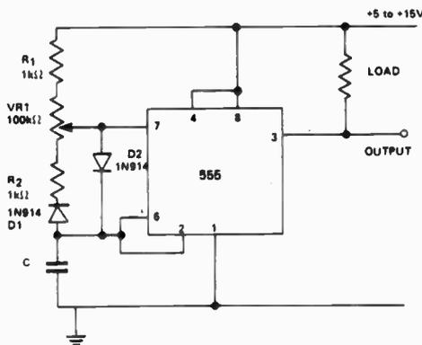
The circuit shown enables a rectangular wave output to be obtained with a duty cycle which can be varied over a wide range by the setting of the potentiometer VR1.
