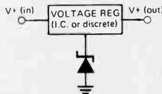
In this circuit the zener diode raises all voltages - with respect to earth - by the zener voltage, i.e.
