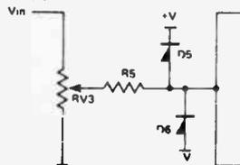
rails  $D_5$ ,  $D_6$  and  $R_5$  should be added to prevent damage to IC1.
