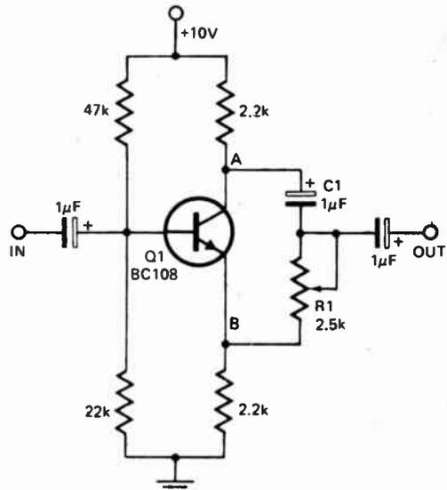
The circuit shown provides a simple means of obtaining phase shifts between zero and 170°. The transistor operates merely as a phase splitter, the output at point A being 180° out of phase with the input. Point B is in phase with the input phase. Adjusting  $R_1$  provides the sum of various proportions of these and hence a continuously variable phase shift is provided.
