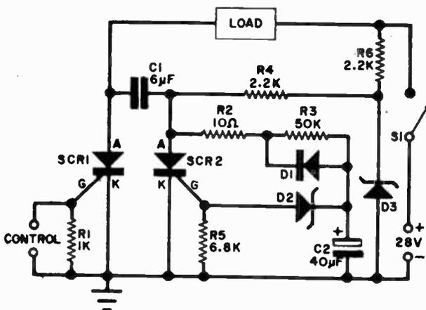
Originally developed by the Unitorde Corporation, this circuit will supply up to four Amps for a period of one second when triggered by an external positive going pulse.
