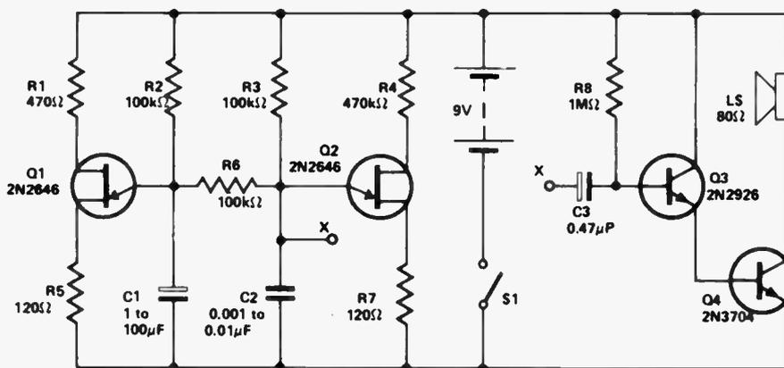
Interesting sound effects are produced by the circuit shown in the figure. The sounds generated by the speaker LS arise from the coupling of two unijunction transistor oscillators by
