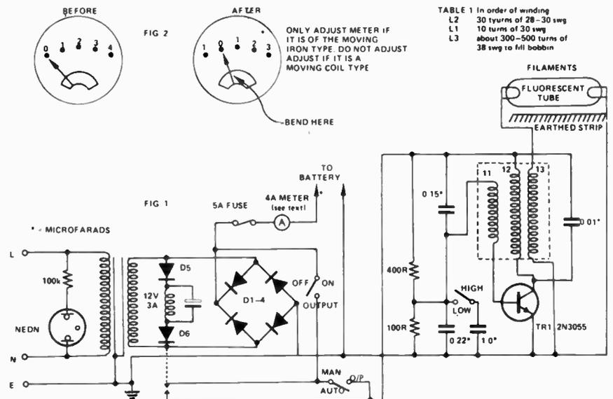
voltage divider for the biasing of C2, 3. With C3 in circuit the inverter in fact becomes more efficient, but has a lower output. Using a 2N3055 enables the inverter to be modified to give higher output and also guards against thermal runaway when used for long periods. A heatsink is advisable.
