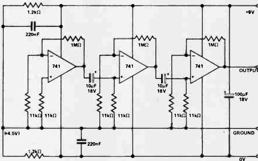
must be laid out as closely as possible to the schematic diagram, and carefully screened, because the input stage is very sensitive to extraneous signals and could pick up hum or oscillate due to capacitive coupling with the output. The prototype is run from a PP9 battery, mounted inside the case, to further reduce any possibility of hum pick-up.
