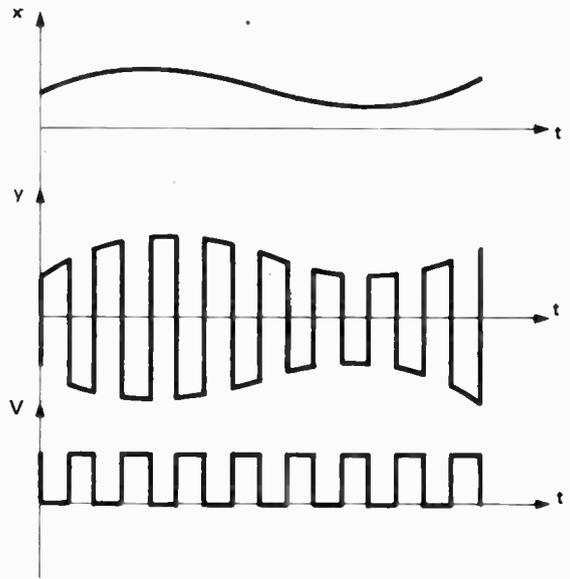
The circuit shown is a simple amplifier, the gain of which can be switched between two precisely controlled values by the application of a signal voltage:  $V$ . If  $V$  is such that Q1 is saturated, then the voltage gain of the circuit is simply  $-\frac{R_2}{R_1}$ . If the transistor is cut off, then the voltage gain be-
