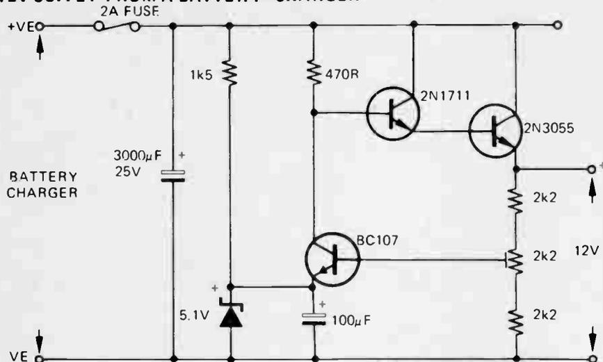
This 12V regulator unit was designed to enable bench testing of mobile equipment (radios, tapes, C-D units, etc.) using a battery charger, thus avoiding the expense of a complete bench supply and the inconvenience of a car battery.
