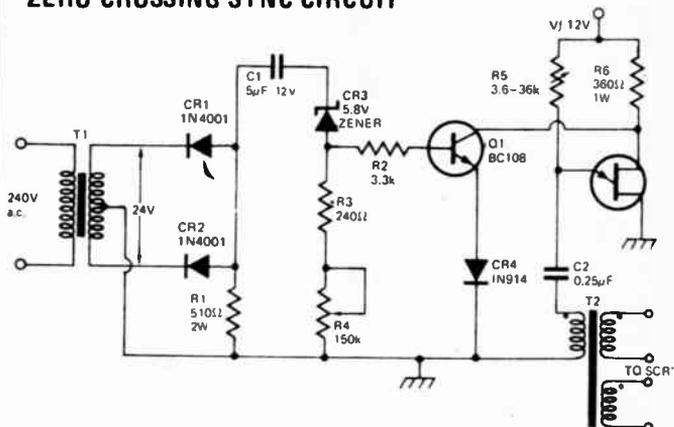
Zero crossing control of SCRs or Triacs is preferable to phase control because less RFI is generated. The circuit shown was developed for a temperature control system and effectively maintained temperature at any set point from ambient to 100°C. Resistor R5 may be a potentiometer, a thermistor or any type of sensing device. R4 is adjusted so that the breakover point of CR3 is at the peak of the reference voltage (zero crossing point of ac wave).
