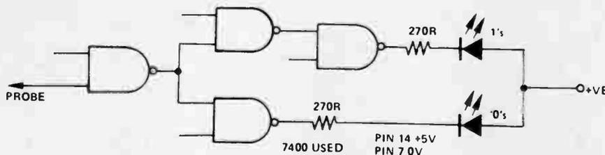
The logic probe automatically goes to logic 1 when not in use and uses the power supply of the circuit under test.
