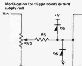
rails D5, D6 and R5 should be added to prevent damage to IC1.
