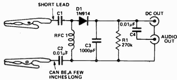
choke down to 470  $\mu\text{H}$  (i.e. Aegis C13, UPC560 or VPC470). In the VHF range C1 can be a 2 to 10 pF capacitor or 0.8 to 7 pF trimmer. RFC1 can be between 47  $\mu\text{H}$  and 150  $\mu\text{H}$  (i.e. Aegis VPC 150, UPC120, VPC100, VPC82, VPC68, VPC56 or VPC47).
