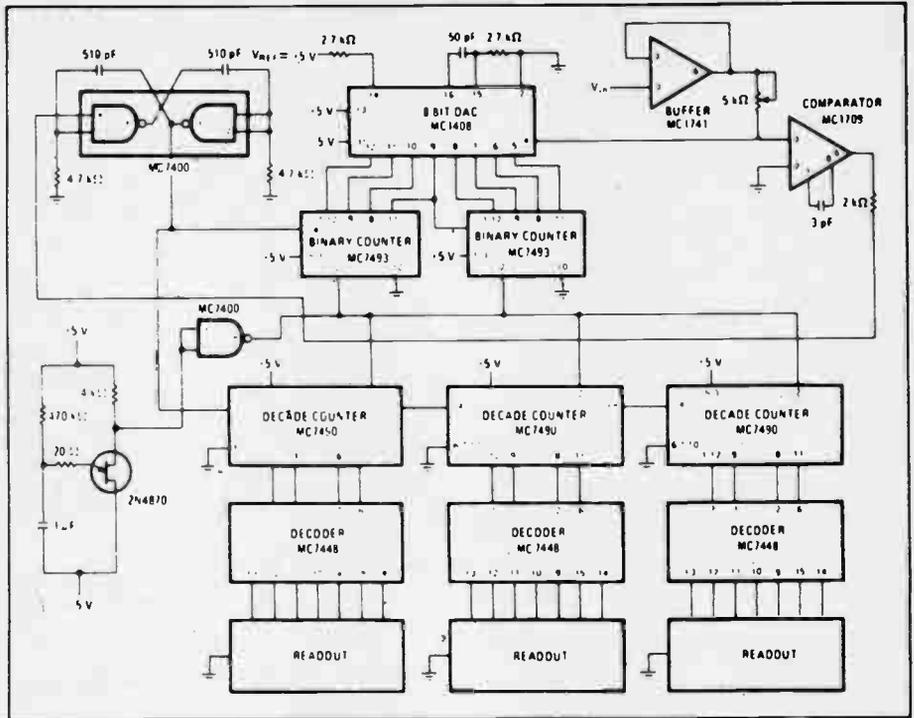
input buffer amplifier which, in addition to giving the meter a high input impedance, supplies an output current of up to 2 mA for comparison with the output of the converter.
