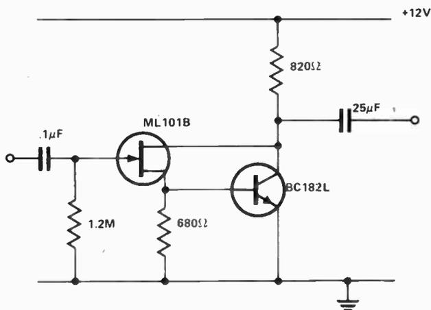
simple. The circuit employs a FET front end to obtain the high input impedance, but the transconductance
