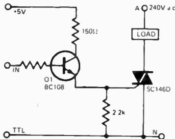
Here is a useful circuit for driven mains operated devices direct from TTL logic circuits. Although it works well, it has the inconvenience that the neutral line is connected to circuit ground.
