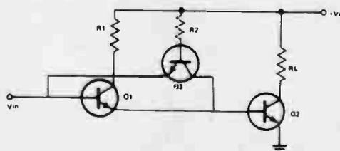
The useful properties of Darlington pairs are somewhat nullified when you need to get any speed out of them. The main drawback of the conventional Darlington in this respect is the long turn-off time, which results from the stored charge at the base of the output transistor.
