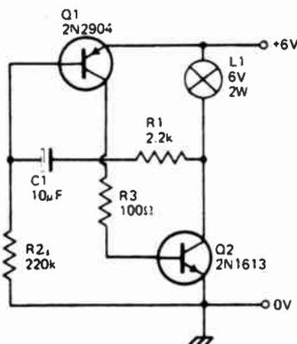
This simple circuit will flash a 6 volt lamp at a rate determined by the size of capacitor C1. It is most economical on power as it only draws current when the lamp is ON. When the lamp is OFF both transistors are biased OFF.
