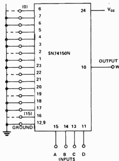
example implement a function to produce an output only if the binary number ABCD is exactly divisible by three.) If it is preferred, each input may be tied to a high level via its own resistor which may then be left in circuit even if required to short the input down to earth.
