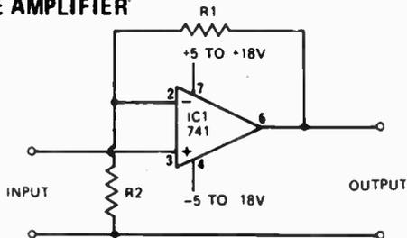
The circuit shown, using one op-amp and two resistors has a high input impedance (500 nanoamps input current) and a gain which may be programmed by R1 and R2.
