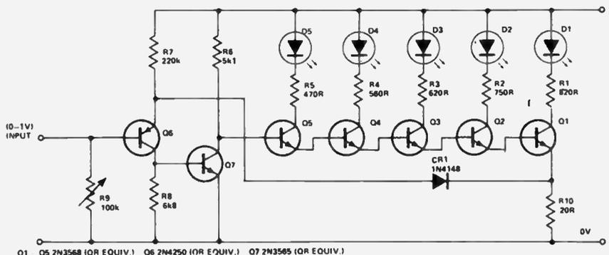
1V (for five LED's). Diode CR1 cancels the  $V_{BE}$  offset of Q6. Resistors R1 through R5 control the LED currents. The voltage across R3 for example is 10V minus 1.5V (two transistors  $V_{BE}$ 's) minus 0.6V (30mA
