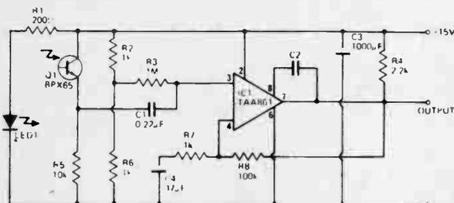
This circuit generates a fast rise time pulse each time the illumination of the BPX65 photo transistor by the LED is broken by a small object or rotating disc segment etc.
