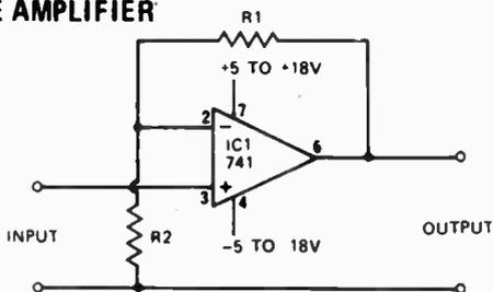
The circuit shown, using one op- amp and two resistors has a high input impedance (500 nanoamps input current) and a gain which may be programmed by R1 and R2.
