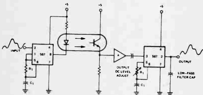
SOMETIMES it is necessary to transfer an analogue signal from one system to another without making any electrical connections.
