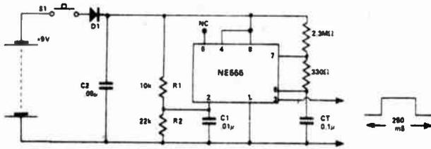
This circuit demonstrates a method of triggering a single time-period from a 555 timer supply by applying power to the circuit, thus eliminating the need for two switches or a two-pole push switch. The original application required that a single 250mSec pulse be produced when a push-button was operated, and the method shown allows the timer circuitry to be switched on and triggered simultaneously by a single MAKE contact. This also economises on battery power as there is no stand-by period.
