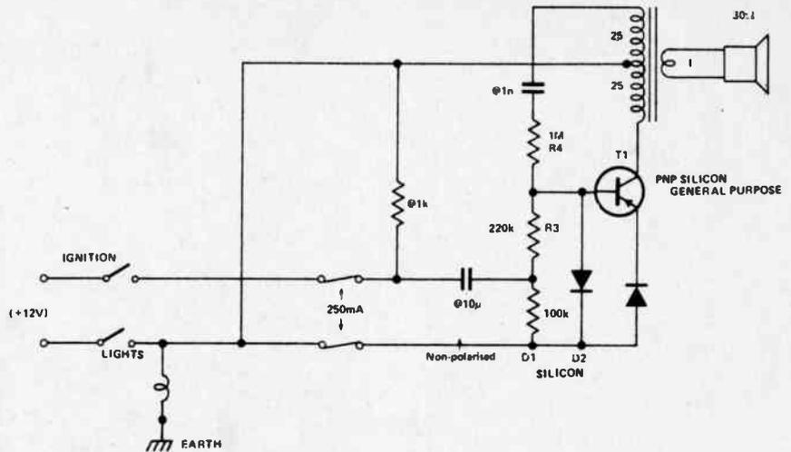
box. Basic requirements are that it should not be self-sustaining when the ignition switching transient in the base circuit has died away. The ratio R3/R4 was of course chosen to achieve
