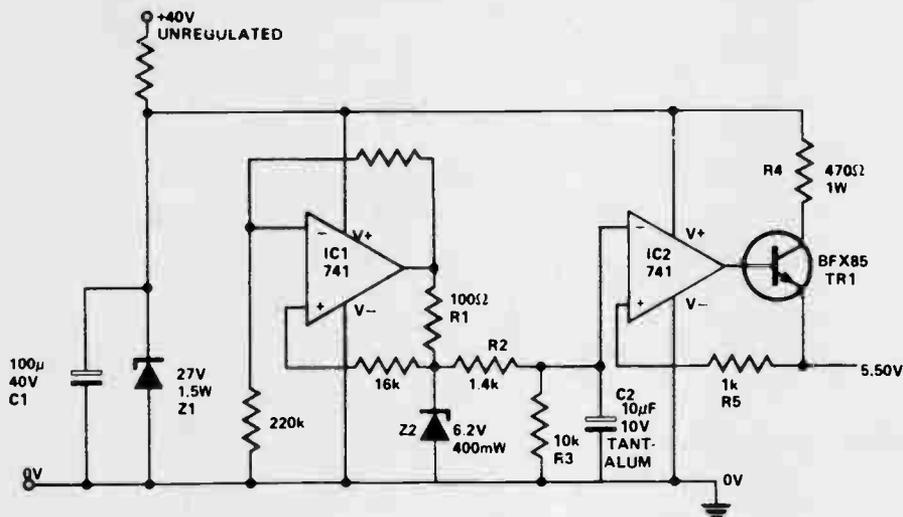
voltage-drop across R1. Z2 is a 6V zener since diodes of about this voltage have the lowest voltage/temperature coefficient.
