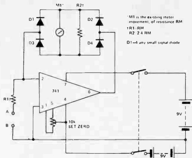
the DC ranges of the instrument. R1 and R2 should be close tolerance types for accuracy; the circuit is accurate up to 100kHz.
