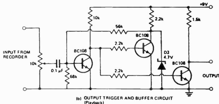
digital pulses which are then recorded. On playback the recorded pulses are fed into a Schmitt trigger whose output is then amplified restoring the
