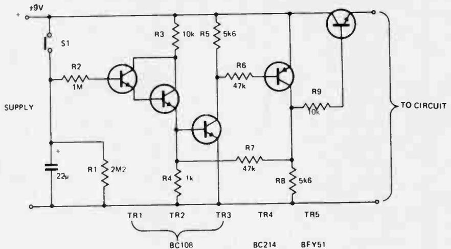
causing a sharp regenerative switching action to take place. TR5 is driven from TR4 collector and handles the supply current to the circuit being switched. R1 ensures C1 fully discharges since as long as any charge remains TR1 and TR2 continue to pass a small current (1mA).
