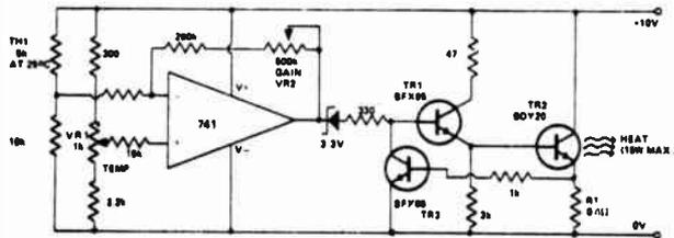
In electronics the need often arises to stabilise the temperature of critical sections of circuitry, such as master oscillators, log converters, and reference supplies. This circuit will control the temperature of a small mass of metal, such as a heat sink onto which critical components can be mounted, simply and efficiently.
