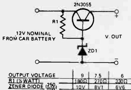
Many transistorised items such as radio, cassettes and other electrical items operate on batteries. Usually these are in the 6-12V range and sockets are provided for external power supply.
