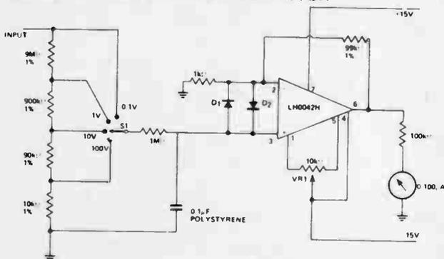
The circuit shown can be used as a high impedance voltmeter with ranges having full scale deflections of 0.1V, 1V, 10V and 100V. The range is selected by the input potential divider connected to S1.
