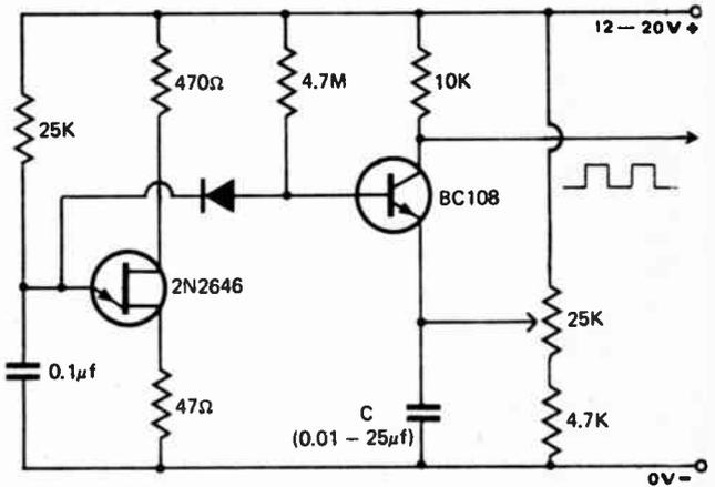
A variable duty cycle squarewave can be obtained from this unijunction circuit. The light loading imposed on the emitter timing circuit preserves frequency stability.
