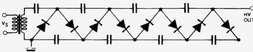
Sometimes a very high voltage is required for applications such as for ionisers or a CRT supply.
