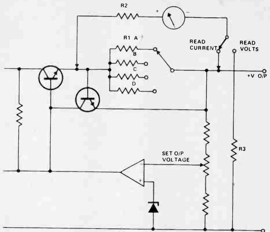
The addition of a single pole C/O switch as indicated will enable the meter to be used to set up the desired output voltage also, though it must be remembered that this will include the voltage drop across R1 if any
