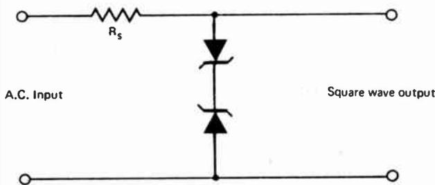
If a larger output is required, opposed zener diodes may be used to clip both halves of the input sine-wave.
