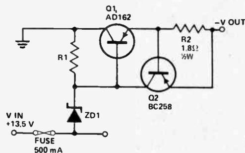
not rise above the 500 mV necessary to turn Q2 on and the circuit behaves as if there was only Q1 present.
