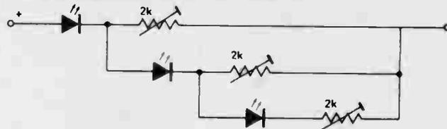
This device makes a very compact and robust level indicator where a meter would be impractical due to lack of space, or not justified due to cost.
