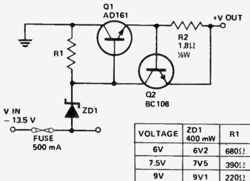
These short-circuit protected stabilisers give 6, 7.5 and 9 V from an automobile battery supply of 13.5 V nominal, however, they will function just as well if connected to a smoothed dc output from a transformer/rectifier circuit.
