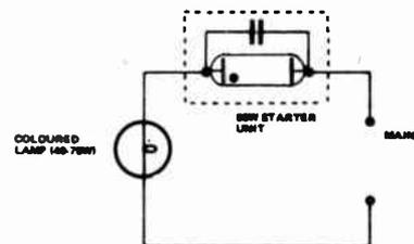
A cheap but effective way of flickering mains lamps suitable for discos etc.
