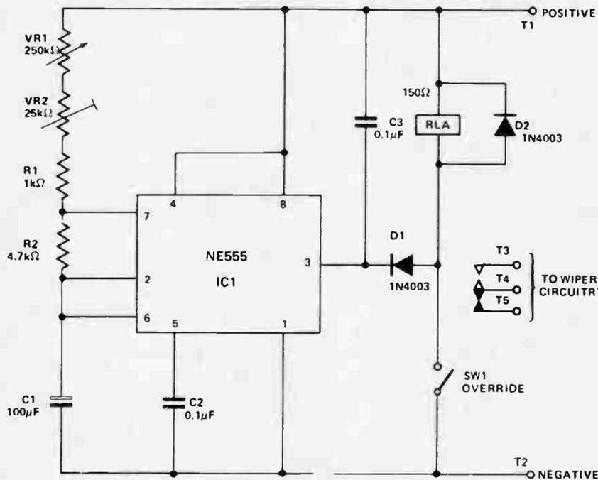
Fig. 1. Wiper Display Unit
