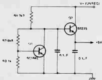
When it is necessary to power a few TTL packages, a simple zener diode — emitter follower stabiliser is often used. If a zener of the appropriate value is not available, then the circuit shown may be used instead. Q1 is a standard VBE-multiplier; the current through Q1 increases until its VBE-drop is established across R3. Hence about 8 times VBE is established across Q1, and this voltage is used as a reference for emitter follower Q2.
