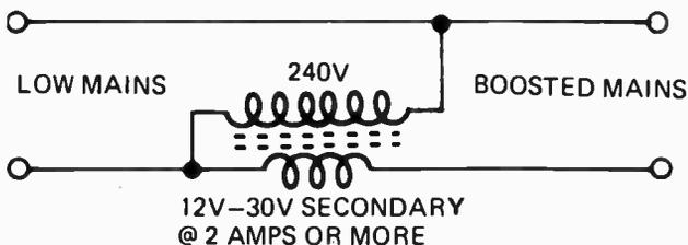
Mains voltage may be boosted by up to 10% by using a standard filament transformer connected as shown above.
