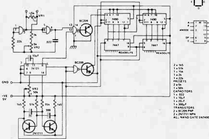
frequency of the multivibrator goes up and vice versa. Trimmer pot VR1 is used to adjust linearity.
