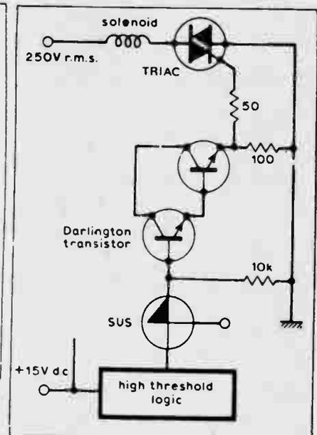
High-threshold logic, operating from a 15-V supply, produces a logic '0' output of 0 to 1.5 V and logic '1' output of 12.5 to 15 V. Noise amplitudes which increase the '0' level to 6.5 V and reduce the '1' level to 8.5 V can be tolerated.
