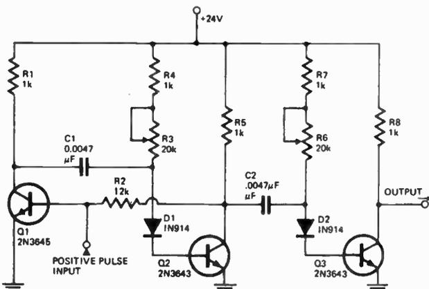
The circuit shown is of an economical pulse delay which utilizes only three transistors instead of the four normally required for a pair of one shots.
