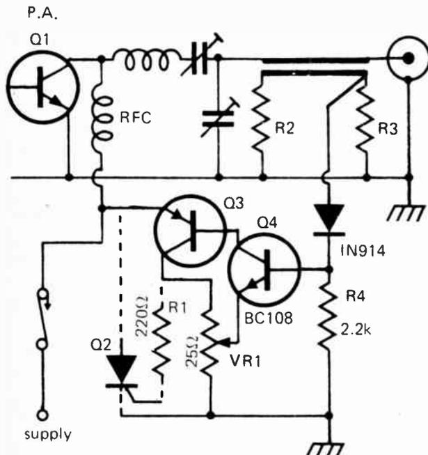
RF power amplifier output transistors may be destroyed by high standing wave ratio loads.
