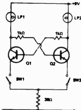
The circuit above can be used as an independent arbiter of which two people can throw a switch first. With both switches off the circuit is completely open and so neither bulb lights. If SW1 is made - even the tiniest fraction of a second before SW2 - Q1 will conduct and LP1, acting as the load, will light up. At the same time the voltage at the collector of Q1 falls meaning that even if SW2 is made there is insufficient bias current to drive Q2 on.
