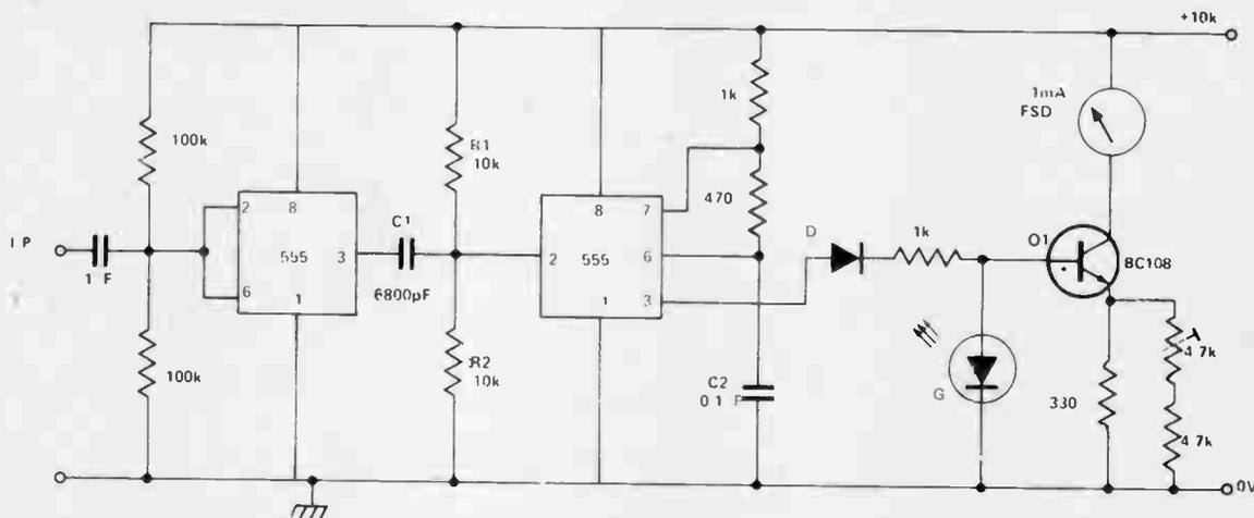
This circuit provides a meter deflection that is strictly proportional to the frequency of the input signal over the range 10Hz–300Hz. The first 555 timer IC is used as a Schmitt trigger, to convert the I/P signal to a fast-edge square wave. This is differentiated by the network C1, R1 and R2, and the resulting spikes used to trigger the
