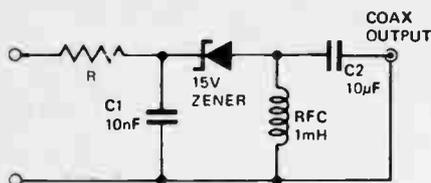
Zener diodes generate quite intense internal noise. This noise level is in the region of 30 dB above the inherent thermal noise and extends out to 150 MHz or so.
