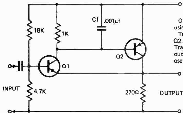
Output impedances as low as 0.05 ohm can be obtained by using this configuration.
