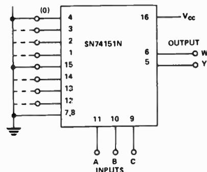
mounting dual-in-line switch which takes up little room. A typical application of this might be for adjusting clock rate timers. A similar arrangement is shown for a function of three variables using the SN74151 IC. In this case the output is available in both true (Y) and complement (W) forms. (In the example shown the majority function is produced. Output is high if two or more inputs are high, otherwise low.)
