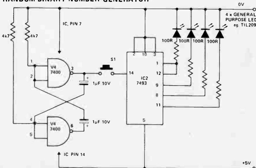
The circuit shown is a random indicator providing an output from one of 16 states.
