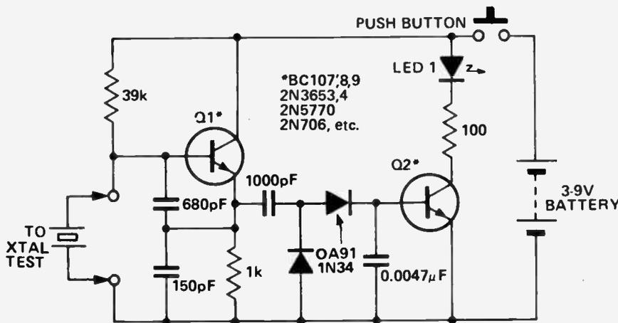
For checking fundamental HF crystals on a 'Go-No-Go' basis, the above circuit works quite well. An untuned Colpitts oscillator drives a voltage multiplier rectifier and a current amplifier. If the crystal oscillates, Q2 conducts and the LED lights. A 3 or 6V, 40mA bulb could be substituted for the LED.
