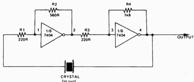
at fundamental frequency, whereas many crystals (particularly higher frequency ones) are stamped with the overtone frequencies. These will
