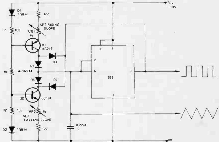
capacitor, and Q1 is allowed to linearly charge it up; when the capacitor voltage reaches  $2/3V_{CC}$  the 555 output goes low again, and the cycle
