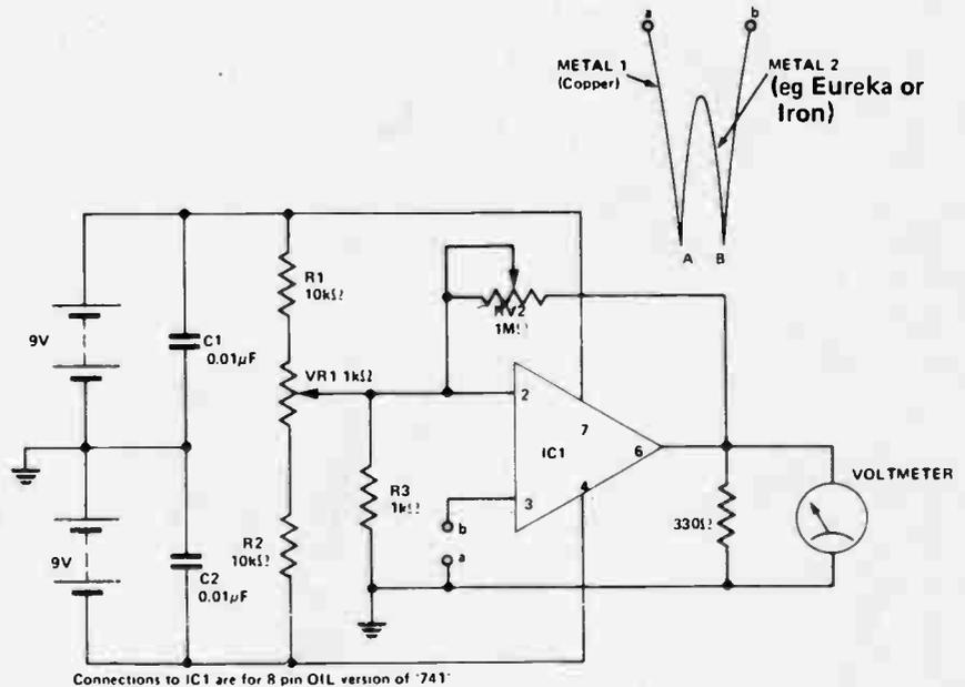
gain of the circuit is set high (at 1,000), electrical noise pick-up and drift become serious problems and it is advisable to assemble the circuit in a metal, earthed box and to ensure the unit is kept at constant temperature.
