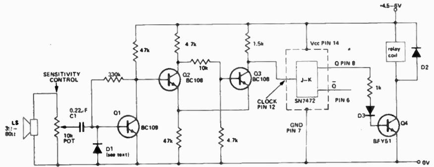
Schmitt trigger's output which is fed to the clock of the JK flip-flop causing it's output to change state. This is used to turn a relay on and off. Because the circuit is only sensitive to sharp noises it is generally unaffected by talking or sounds caused by movement. (The sensitivity control can be adjusted to prevent such noises triggering the circuit if this does arise). A moving coil loudspeaker is used as a microphone as it can respond to sounds from any direction. It was
