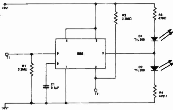
This circuit was devised as part of a touch controlled lighting system. It uses a 555 timer operated in the bistable mode.
