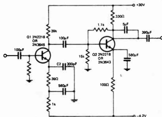
The amplifier shown has a frequency response of from 5Hz to 30MHz and is capable of giving a 10 volt output into a 100 ohm load. The circuit provides 26 dB gain and has excellent stability and linearity.
