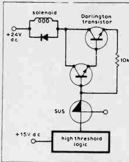
energisation of the solenoid; negative-going noise pulses occurring while the solenoid is on would have to reduce the input to the output amplifier to below 2 V, from between 12.5 and 15 V, for a spurious de-energisation.
