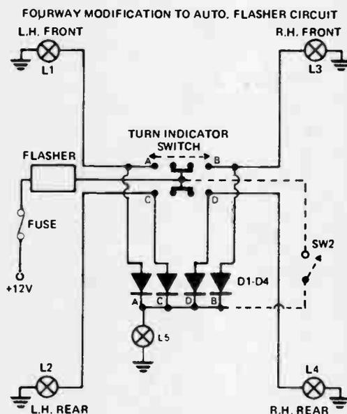
Many current model cars now incorporate a turn indicator switch position which causes all four indicator lights to flash simultaneously. This is a valuable safety device if stalled on the road – especially at night.
