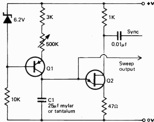
This circuit provides a linear time-base with a sweep time adjustable from a few milliseconds to over one minute. The constant-current effect of emitter follower Q1 causes C1 to be charged at a constant rate. The increasing voltage across C1 will be essentially linear (displacement error is less than 1%). The sweep is terminated when the increasing capacitor voltage reaches the peak valley point of unijunction Q2, when capacitor C1 will discharge through the current limiting resistor R1.
