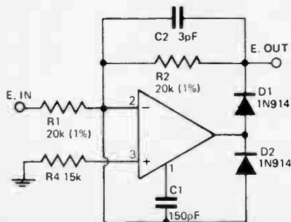
A precision half wave rectifier using an operational amplifier may be constructed as shown. This will have a rectification accuracy of 1% from dc to 100 kHz.
