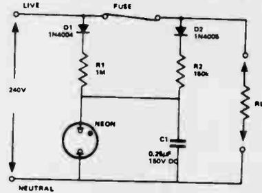
up to the striking voltage of the neon, diode D2 must have a PIV rating greater than peak mains plus this voltage. D1 can be rated at peak mains or greater. The types specified are suitable easily-obtained devices. Also, built-in resistors in certain types of neon indicator supplied for use at common supply voltages must either be removed or 'shorted'. The resistors should be 1/2W.
