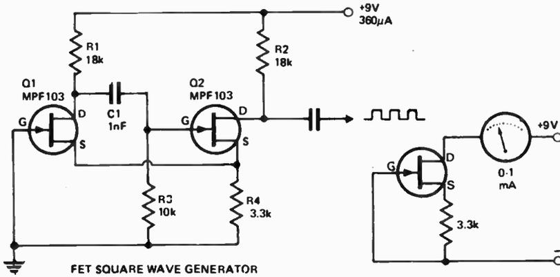
Field effect transistors lend themselves readily for use in astable multivibrator circuits.
