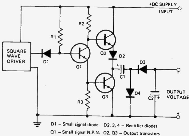
This transformerless inverter chops the dc supply voltage then rectifies the
