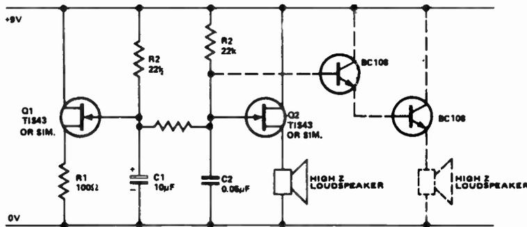
The circuit consists of two unijunction relaxation oscillators, Q1 for low frequency and Q2 for audio frequency. R3 couples the slow rising
