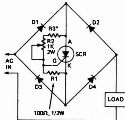
This circuit enables a single SCR to provide fullwave control of resistive loads.
