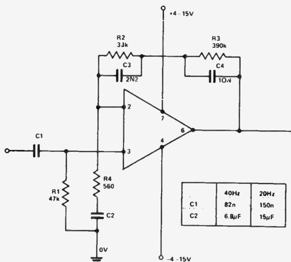
magnetic cartridge may be only about 5mV normally a musical peak may well force the cartridge output to 100mV. Clearly unless a large signal swing is possible the sound emanating from the speaker is not going to be Hi-Fi.
