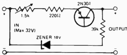
A series transistor is used as a variable resistor for this constant current supply.
