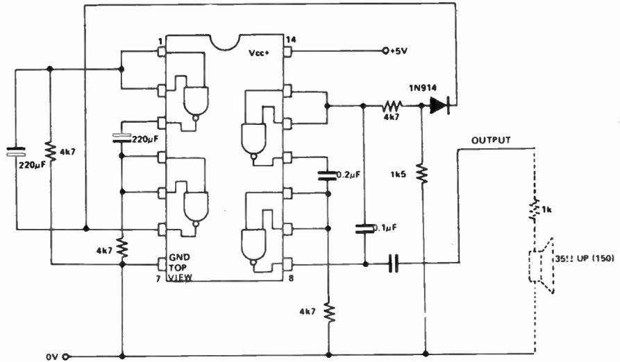
oscillator frequency altogether). DTL-7400s but they give a higher pitched note. 946s could be used instead of the
