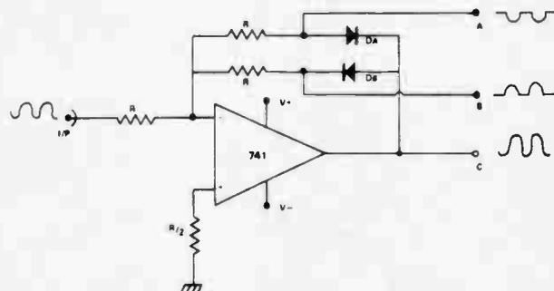
This circuit separates the positive and negative halves of an input waveform, and presents them (both phase-inverted) at separate output terminals. When the input swings positive, terminal A swings negative by an equal amount, terminal B remaining at zero voltage due to the reverse-biasing of DB and the virtual-earth action of the op-amp. For negative inputs, terminal B swings positive by an equal amount, terminal A remaining at zero due to the reverse-biasing of DA.
