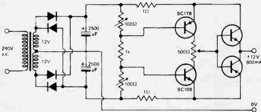
A variable power supply using complementary output transistors is capable of swinging the voltage at the output from +12 V through zero to -12 V.
