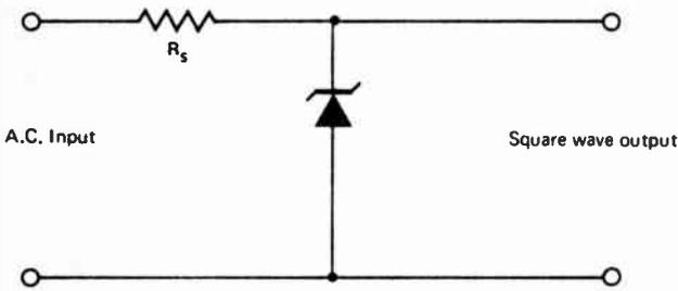
A zener diode clips one half-cycle of the input sine-wave in this simple square-wave generator. The zener voltage must be a small fraction of the input voltage for acceptable results.
