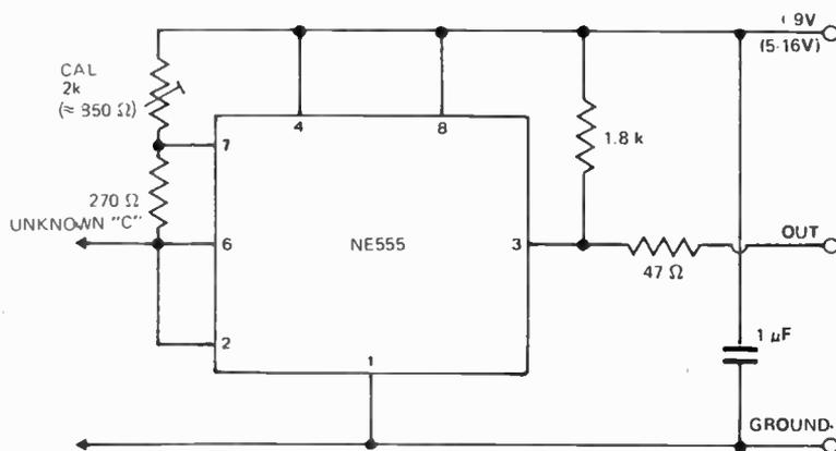
The prototype unit accurately measured a 50 000  $\mu\text{F}$  capacitor and a 2  $\mu\text{F}$  could still be measured
