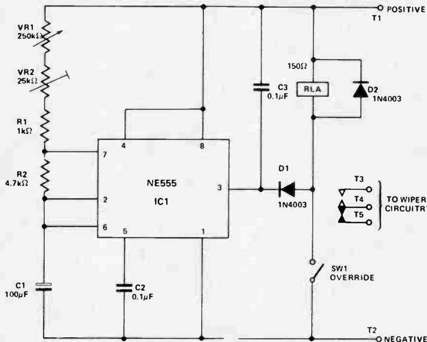
Fig. 1. Wiper Display Unit
