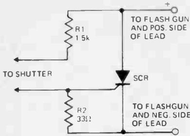
This three component device will keep sparks out of your camera shutter, when using a flash gun, by letting an SCR carry the firing current.
