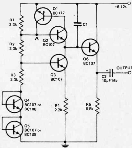
In this circuit two transistors Q1 and Q2 are connected so that they operate as a unijunction transistor.
