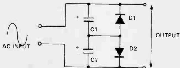
Quite often, especially when constructing operational amplifier circuits, capacitors of several  $\mu$ Farad values are required and they must be of the non polarised type (non elect-
