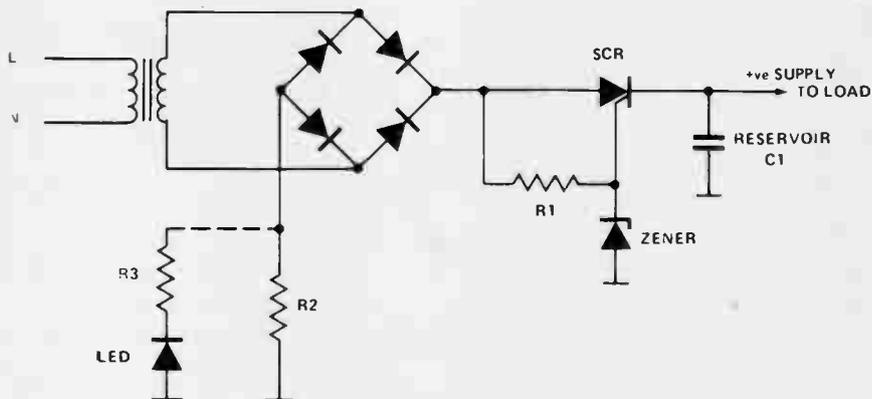
charge via the load, whatever power is being supplied, until the gate is once more positive, when the SCR will fire again. One or more half cycles are sufficient to raise the reservoir voltage sufficiently to prevent further firing.
