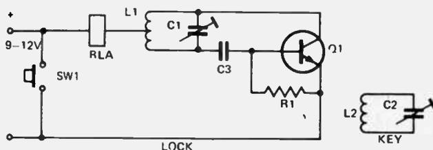
Operation is very simple, when the key is brought near the lock, providing L1-C1 have the same resonant frequency as L2-C2, the reed relay will open as the key absorbs energy from
