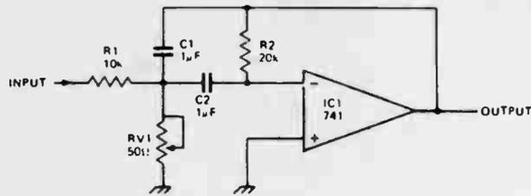
This active filter has a gain of unity (0 dB) and is useful over the range 0.01 Hz to 3 kHz. The centre frequency of the passband is set by potentiometer RV1 and the bandwidth is determined by the values of R1, C1 and C2. The values shown in the circuit provide a bandwidth of about 15 Hz. With RV1 set to mid-position the centre frequency is approximately 220 Hz.
