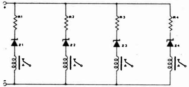
This circuit provides sequential closing of a relay series by appropriately increasing an applied voltage.
