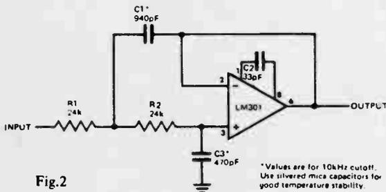
ACTIVE RC filters using operational amplifiers are increasingly being used to supplant LC filters because of the small size and ever-decreasing cost of integrated circuit operational amplifiers. Here are two useful general purpose circuits which may be readily incorporated into other circuitry where needed.
