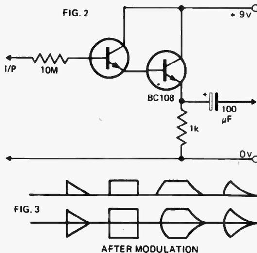
an add-on circuit which should be used if a low impedance output is required.
