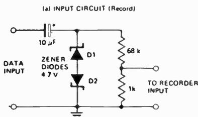
The two circuits shown allow digital data to be recorded and replayed on an ordinary domestic recorder. The input circuitry differentiates the
