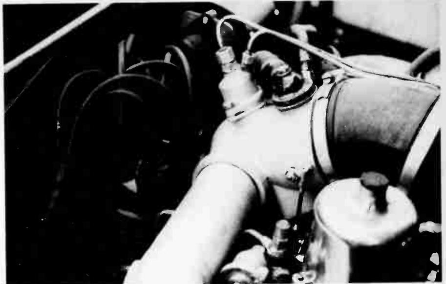
*The distributor on an engine is most often the culprit in severe ignition interference problems.*
