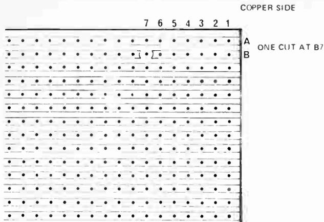
Only one break in the Veroboard copper pattern is required – as shown in this diagram.
