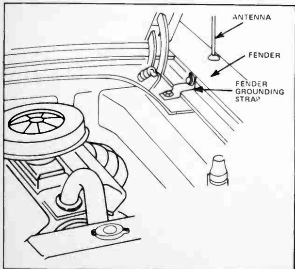
Figure 6. It is essential that the body panel on which the antenna is mounted is properly bonded to the vehicle's general chassis. This won't be necessary on vehicles having welded body panels. This precaution not only aids noise reduction but ensures proper antenna operation.
