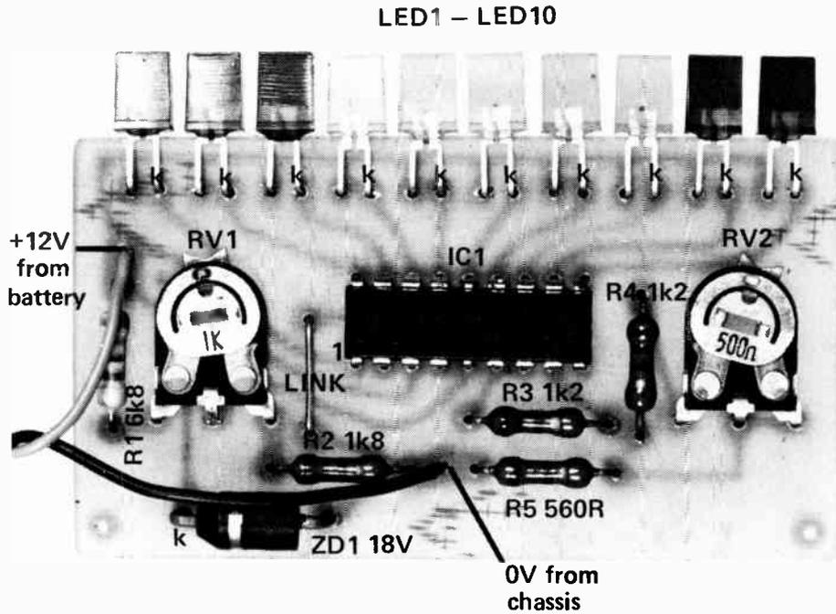
ing the reading (such as in the headlight wiring). The chassis connection can be made to the car body under the dash, wherever convenient, or taken to a chassis connection point in the engine bay.
