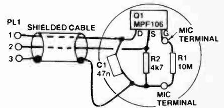
General construction for the buffer, mounted on the rear of a mic insert.
