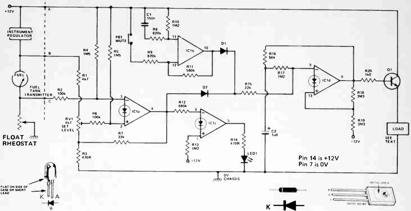
most cars will have to be removed and the wires to the fuel gauge identified and tapped. This can take the best part of a day, so give yourself plenty of time. Some cars use a printed circuit dash instead of a wiring loom and the connections can be soldered onto the back of the pc board, taking care not to damage it.
