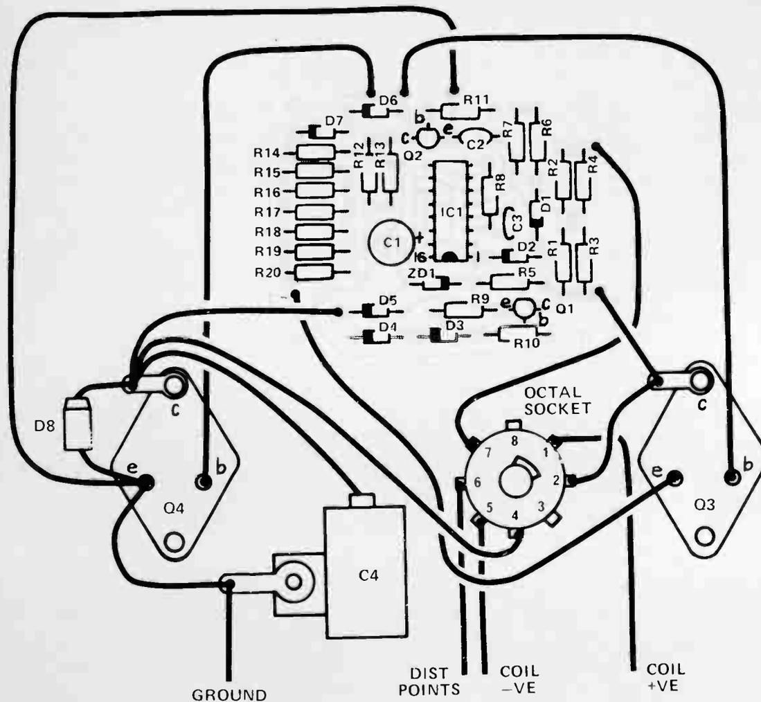
Fig. 2. Overlay and wiring diagram.
