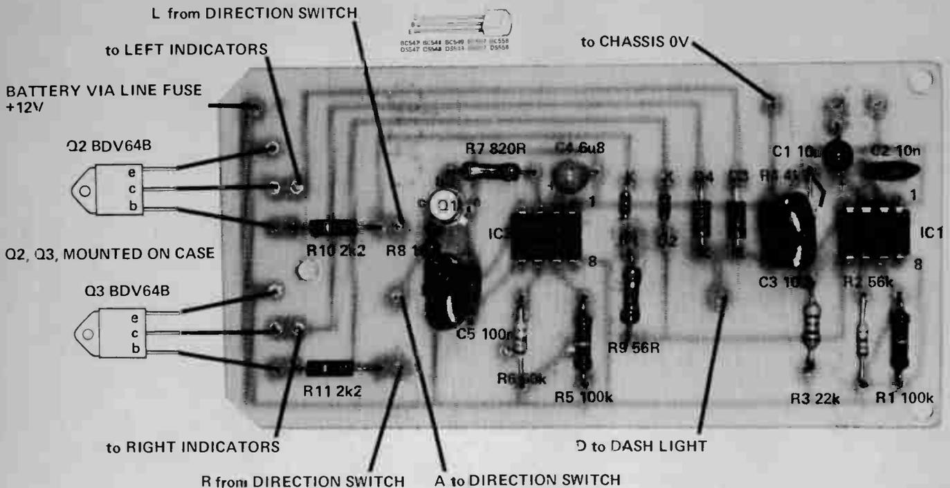
Component overlay and external component connections.
