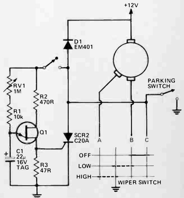
Fig. 3. Simplified ETI 319A Vari-Wiper for use with wound field coil motors. The right circuit is for use with negative earth vehicles, and the left for positive earth. Both share the same PCB.
