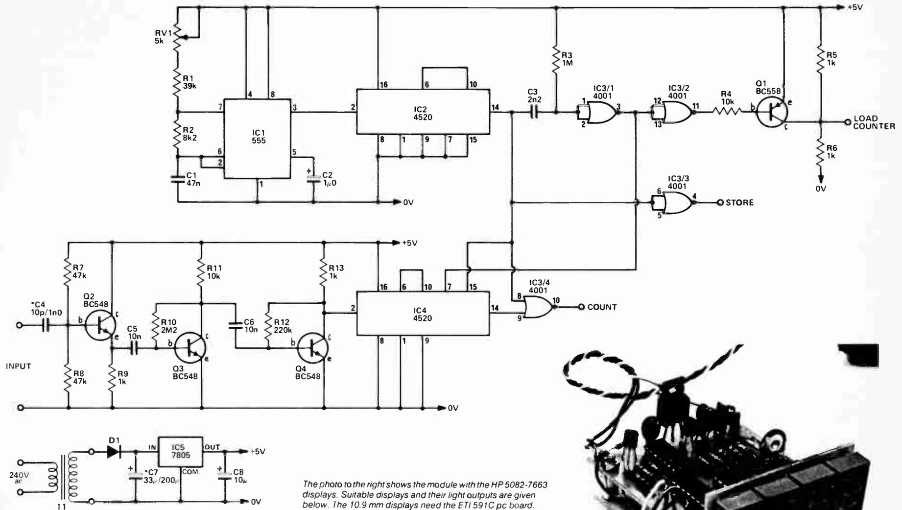
Fig. 3. The circuit diagram of the control logic.
