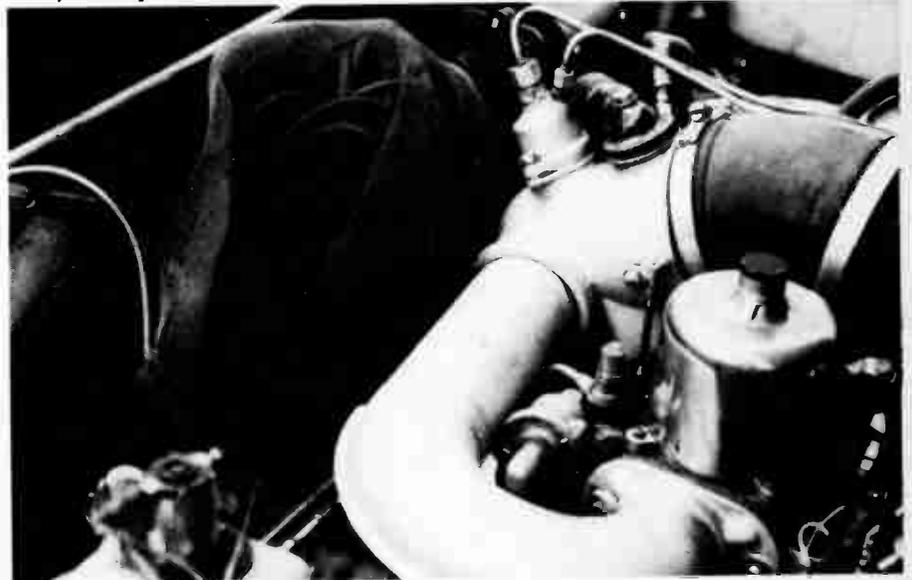
*An often completely effective method to get rid of the problem is to screen the distributor with ordinary fly-screen mesh as illustrated.*
