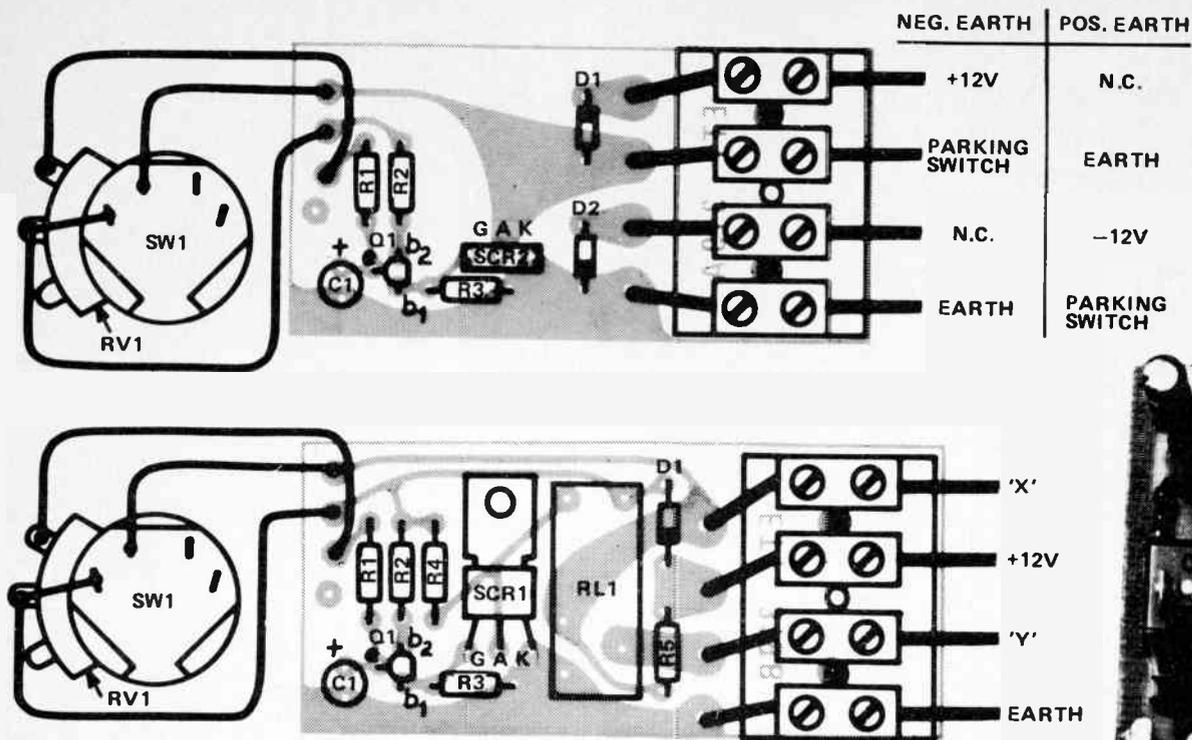
Fig. 5. Component overlays. Note that the same PCB is used for both earth polarities on the ETI 319A. (The PCB pattern is on page 34).
