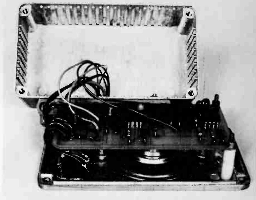
Our unit was assembled into a diecast box using standoff pillars to support the pc board. If you use an 8 ohm or 16 ohm speaker with a series resistor, the value of the resistor may be varied to alter the speaker volume. With a high impedance speaker, a suitable value resistor may be inserted in series to lower the volume. Try 100 ohms as a start.
