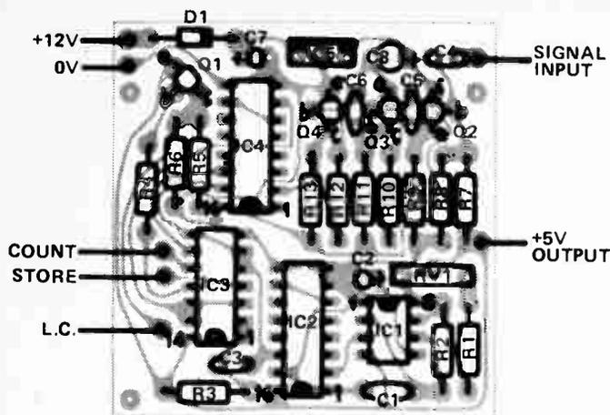
Fig. 1. The component overlay for the control card.
