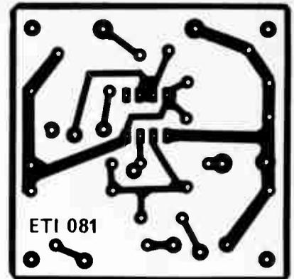
Fig. 2. Printed circuit layout. Full size 50 mm x 50 mm.
