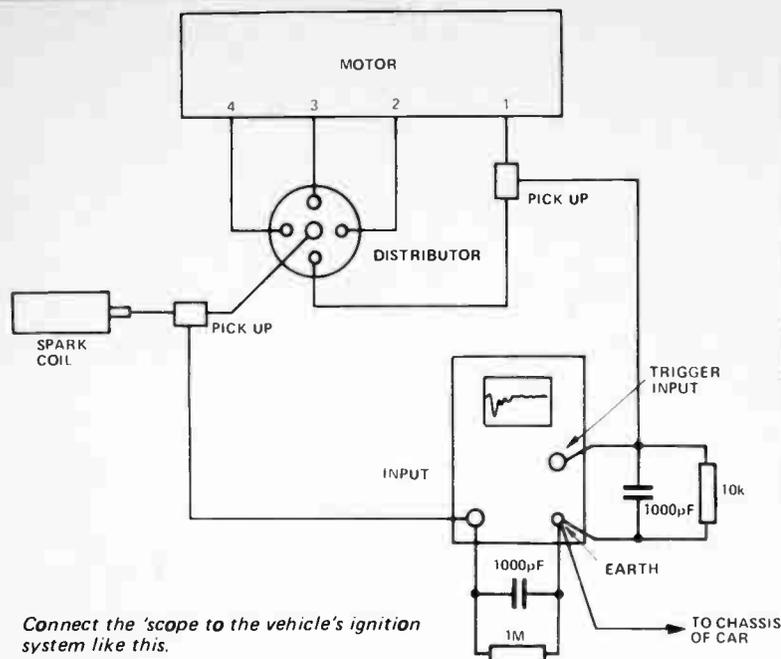
Connect the 'scope to the vehicle's ignition system like this.
