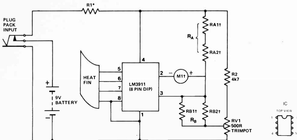
\*R1 = 470R (¼W or ½W) for 9 V operation; 1k8 for 12 V battery (11 - 15 V) operation.
