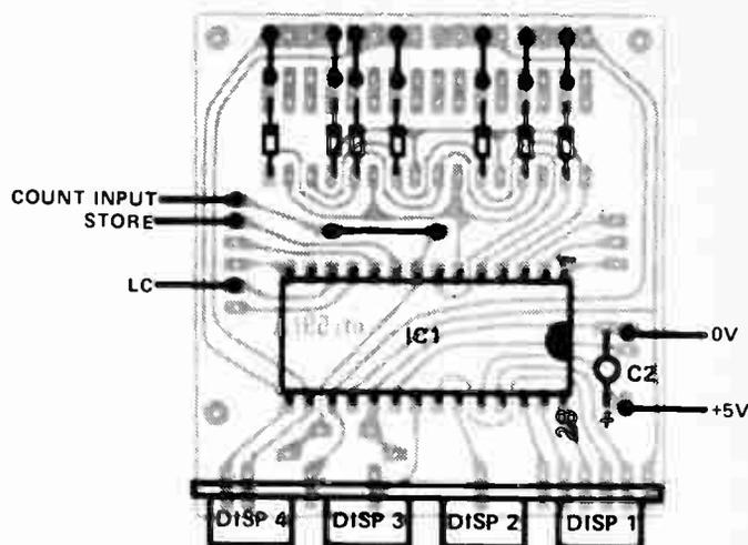
Fig. 2. The component overlay of the display module showing the diodes and links required.
