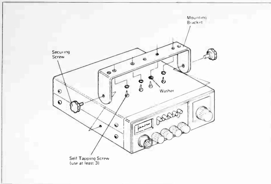
Figure 1. (Above) Typical installation arrangements for a mobile CB rig.
