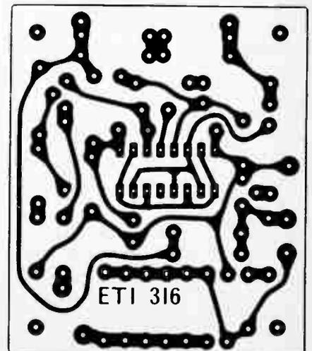
Fig. 3. Printed circuit board. Full size 65 x 55 mm.
