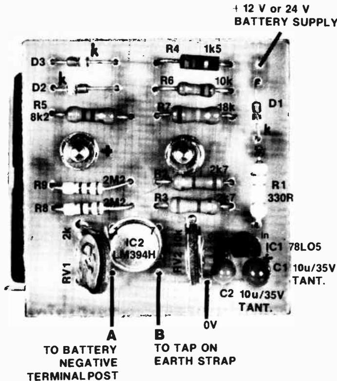
Component overlay for the pc board (pc board pattern is on page 74). Trimpot RV1 is for BALANCE while RV2 is for ZERO SET. The latter, along with R7, is left out if you use a centre-zero meter.
