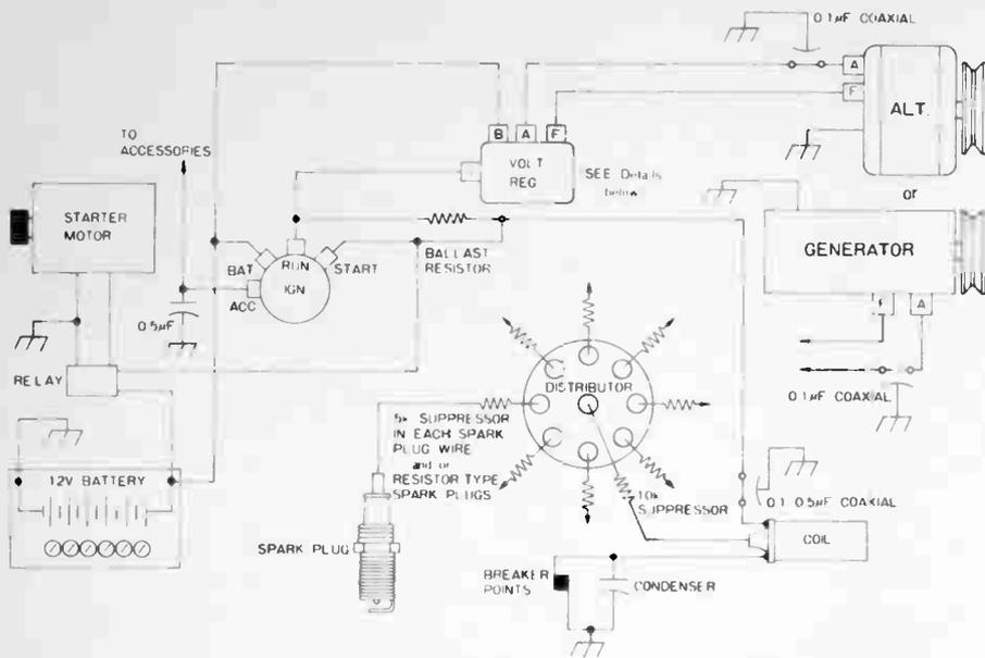
Figure 4. General circuit of a vehicle ignition and alternator/generator electrical system showing where suppression components are connected.
