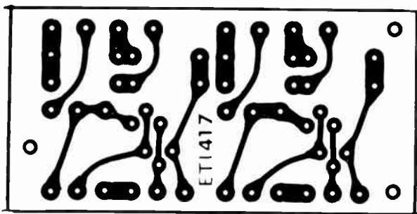
Printed circuit board layout — shown full size.
