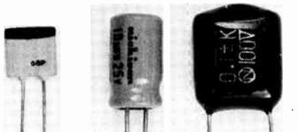
The second number of importance is the voltage rating. You must never use a capacitor rated at a lower voltage than specified but you can go upwards if you like. That is if the project calls for say a 10 uF 16 volt capacitor then you can
