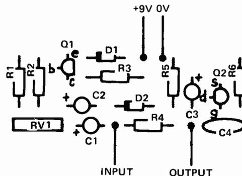
Component layout of printed circuit board version.
