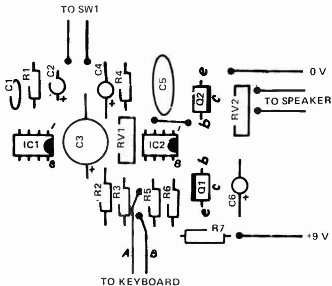
Component overlay for printed circuit board version.
