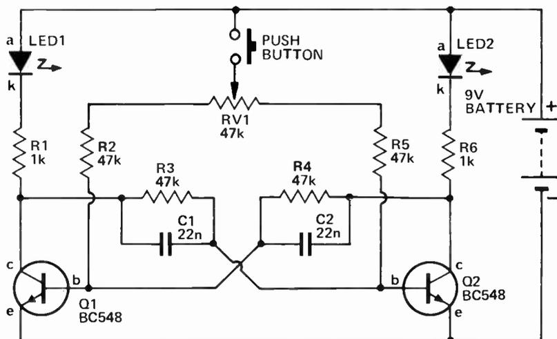
Fig. 3. Circuit diagram of the unit.
