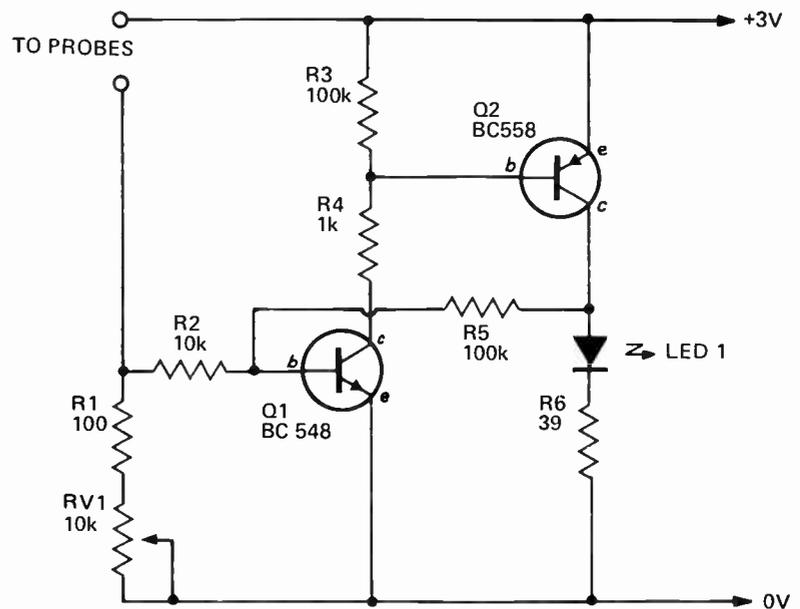
shown and replaced by a small 10 k rotary potentiometer mounted on the other end of the case. A pointer knob and calibrated scale could be added to enable the unit to be used to monitor plants with different moisture requirements.
