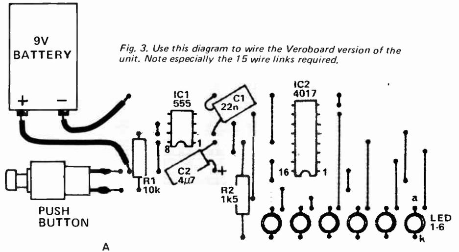
Fig. 3. Use this diagram to wire the Veroboard version of the unit. Note especially the 15 wire links required.
