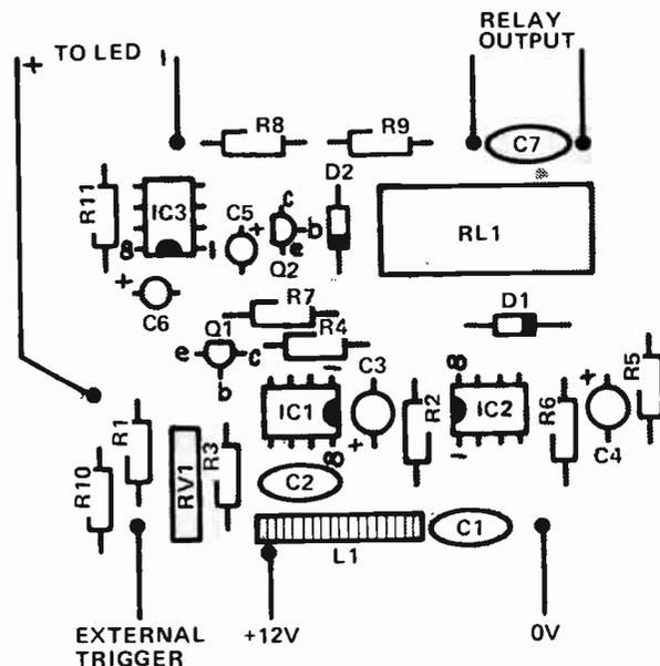
Component layout — printed circuit version.
