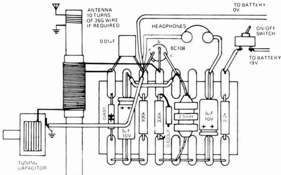
*Tag Strips – construction is quick, cheap and simple. However the method is only really suitable for small scale projects as inter-tag wiring will otherwise be extensive and tedious. The method also wastes space. (Circuit shown is of a single transistor reflex receiver first published in our December 1971 issue).*
