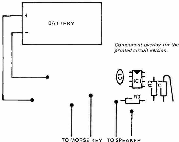
Component overlay for the printed circuit version.
