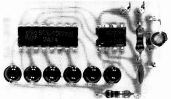
The completed printed-circuit board version of the LED dice.
