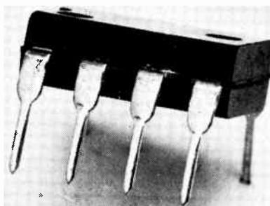
A typical 8 pin dual-in-line (DIL) integrated circuit.
