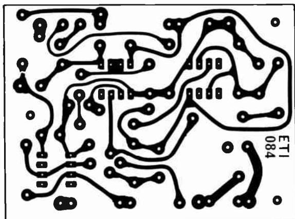
Printed circuit board pattern — shown here full size.
