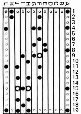
Drilling details for Veroboard of over-rev alarm. Dots mean solder points while hollow circle indicates a hole cutting the copper track.
