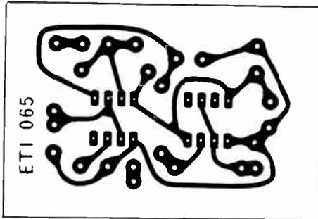
Printed circuit board full size 60 x 40 mm.
