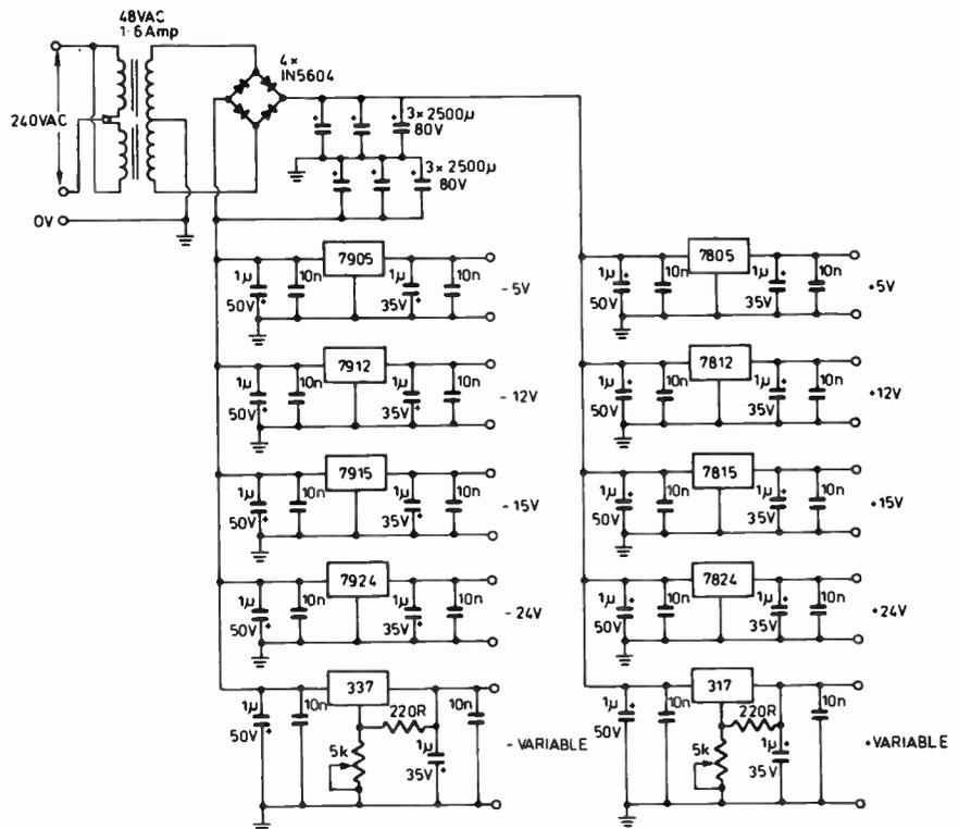
The variable regulators (LM317 and LM337) work by maintaining a constant 5 V between their output and Common pins. The voltage between output and ground can thus be controlled by devising a voltage divider with R1 and VR1. A constant current of  $(5/220) = 23 \text{ mA}$  flows through the 220R resistor, and a linear voltage drop will thus be created across VR1.
