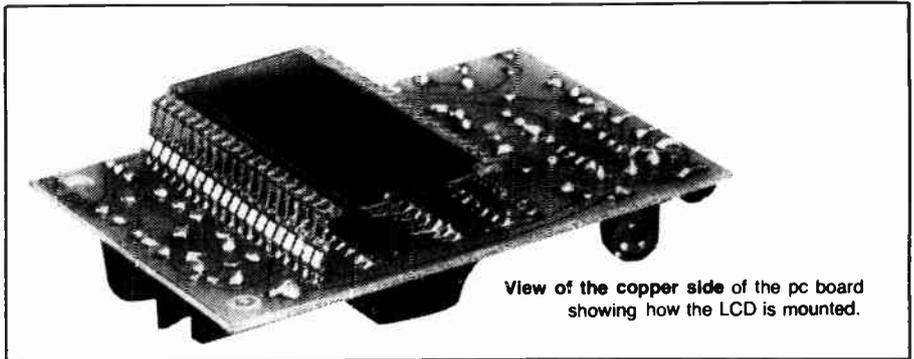
View of the copper side of the pc board showing how the LCD is mounted.
