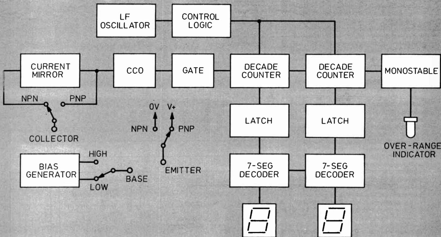
Figure 2: block diagram of the digital transistor tester.
