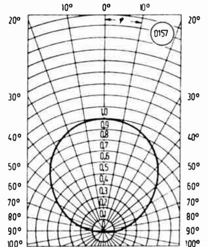
**Figure 1.** Silicon photodiode characteristics.
