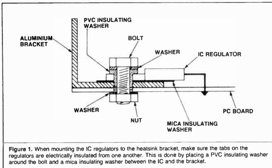
**Figure 1.** When mounting the IC regulators to the heatsink bracket, make sure the tabs on the regulators are electrically insulated from one another. This is done by placing a PVC insulating washer around the bolt and a mica insulating washer between the IC and the bracket.
