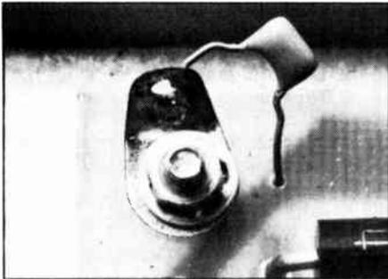
A solder lug should be used to bolt the 100n bypass cap to the chassis. This allows the case to act as an rf shield but still provides for a floating supply.
