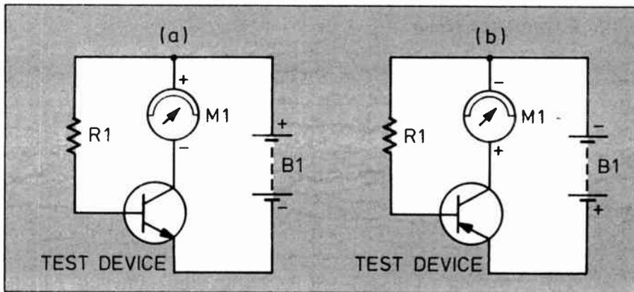
Figure 1: basic test circuits for NPN and PNP transistors.
