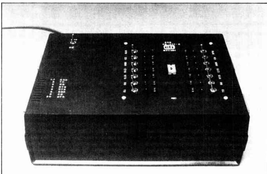
THE RS-232-C STANDARD greatly simplifies the interconnection of digital devices. When something goes wrong at an RS-232-C interface, the 25 signal lines and two equipment configurations — Data Terminal Equipment (DTE) and Data-circuit Terminating Equipment (DCE) — can easily confuse the trouble shooter. The RS-232-C BreakOut Box (BOB) is a piece of test equipment used to simplify RS-232-C trouble shooting.
