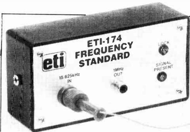
Get the equivalent of a rubidium frequency standard by draping a piece of wire over the back of your TV set!!!
