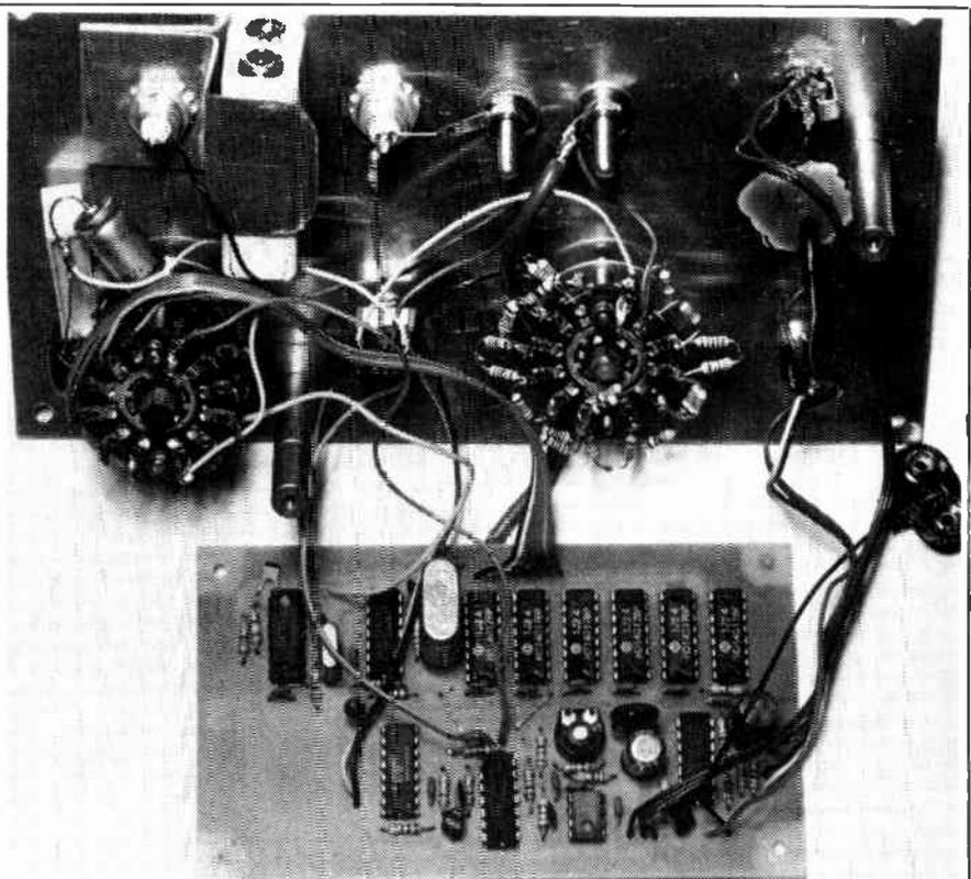
**Inside the case.** Apart from the ICs and other components mounted on the PCB there are few other components required and these are mounted directly on the switches. Note the battery clamp bracket, attached to the front panel by the 10 MHz output socket.
