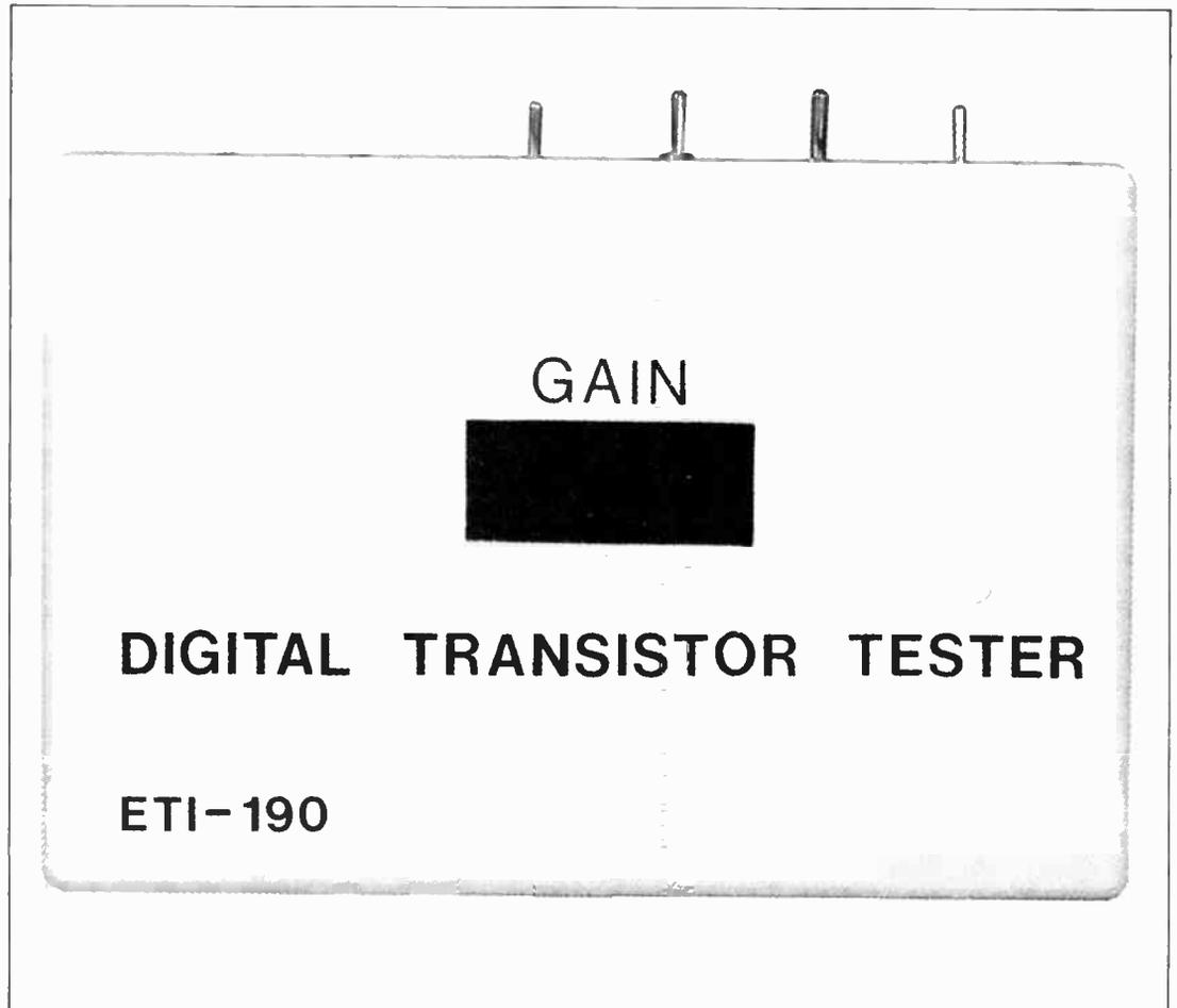
and PNP devices and has two gain ranges, 0-99 and 0-990. This enables reasonably accurate checks to be made on anything from low gain RF and switching devices through to very high gain audio devices.
