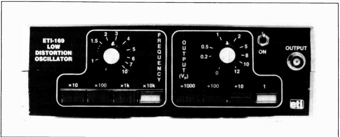
Amplifier distortions normally run from 0.1% or -60 dB (crummy) to 0.001% or -100 dB (so good it's very hard to measure and doesn't really matter!). This latter figure sets the required performance of an oscillator if it's to be used in thd testing. That is, the sum of all the harmonics that come out of the oscillator should be about -100 dB or 0.001% of the fundamental. This is a pretty tall order but it seems a good place to start.
