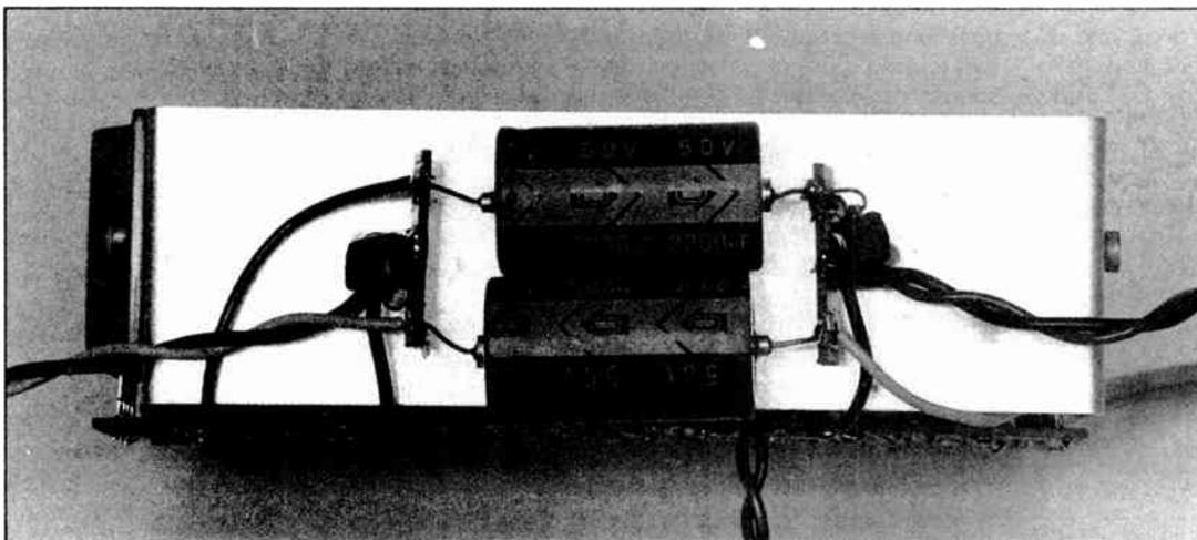
Left: A rear view of the module itself. The power modules are at either end of the aluminium strip, which serves as a heatsink, apart from carrying the power supply capacitors.
