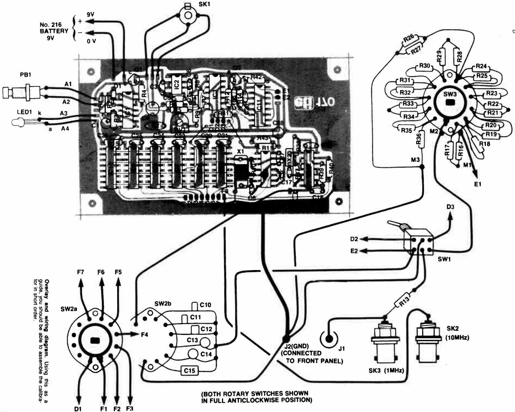
Overlay and wiring diagram. Using this as a guide, you should be able to assemble the calibrator in short order.
