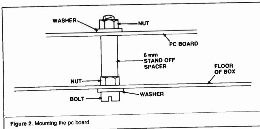
Figure 2. Mounting the pc board.
