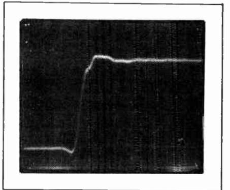
Figure 5. Tek 465 again, 20 mV/div and 10 ns/div, with the calibrator on 100 mV range.
