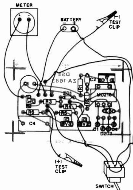
the 50V range and connect the 30V zener across the test clips. Adjust RV3 for a correct reading. This completes the setup procedure.
