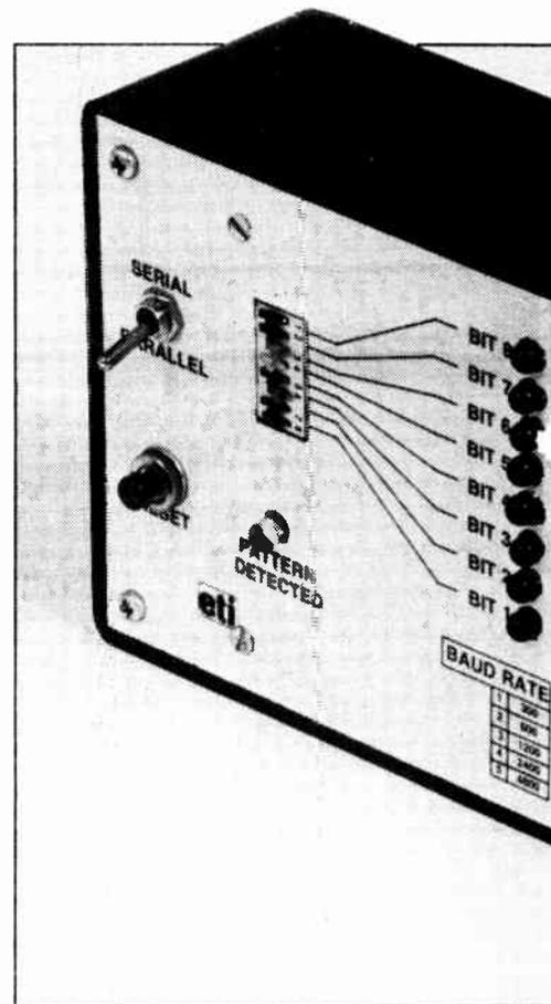
The buffered display shows the byte present on the data path on a row of LEDs. These LEDs are driven by non-inverting buffers to reduce loading.
