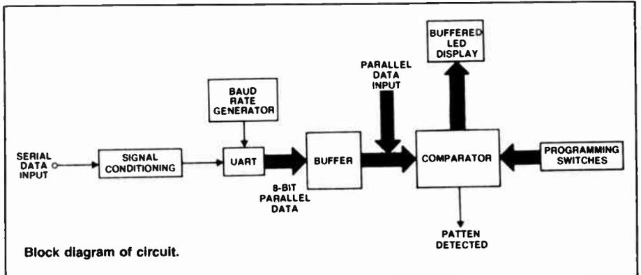
aligning this diagram over your front panel, it can be used as a drilling template. When you have it in position, lightly punch the centres of all holes. To make the centres more accurate it may help to have a hard surface under the front panel when you are punching it. The outlines for the DIP switches can be marked by cutting through the diagram with a sharp blade or scalpel. This will transfer all the required markings on to the metal.
