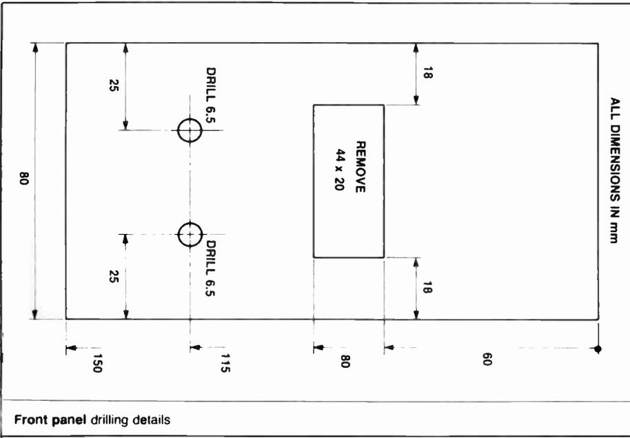
Front panel drilling details
