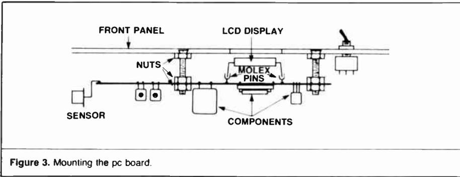
Figure 3. Mounting the pc board.
