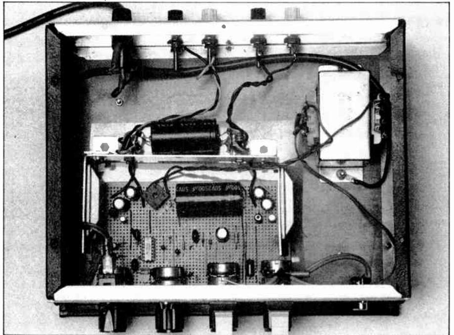
Above: The top view of the amplifier mounted in its case. The transformer is at the bottom left, along with output terminals.
