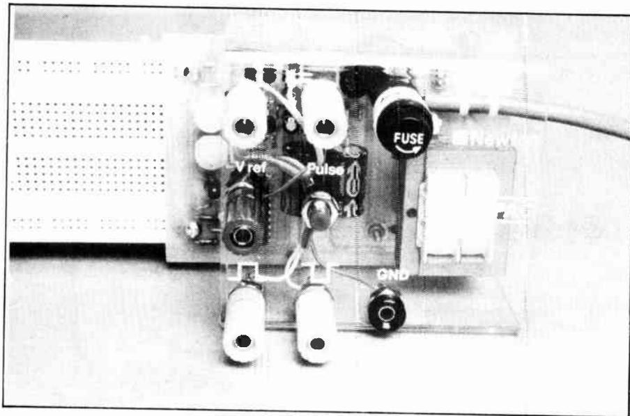
THE DEVELOPMENT AND testing of electronic circuits is usually a costly and time consuming business. Firstly, the system needs to be prototyped in one way or another, power supplies connected and test signals applied. Wires dangle around the test bench and connections to the circuit are often far from ideal. In order to simplify the prototyping stage of the design process this low cost protoboard system was developed.
