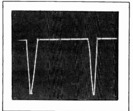
Figure 4. A BWD 511 of unguessable age. CRO calibrator set to 1μs timing pulses, CRO at 1 V/div and 0.2 μs/div. No graticule illumination available.
