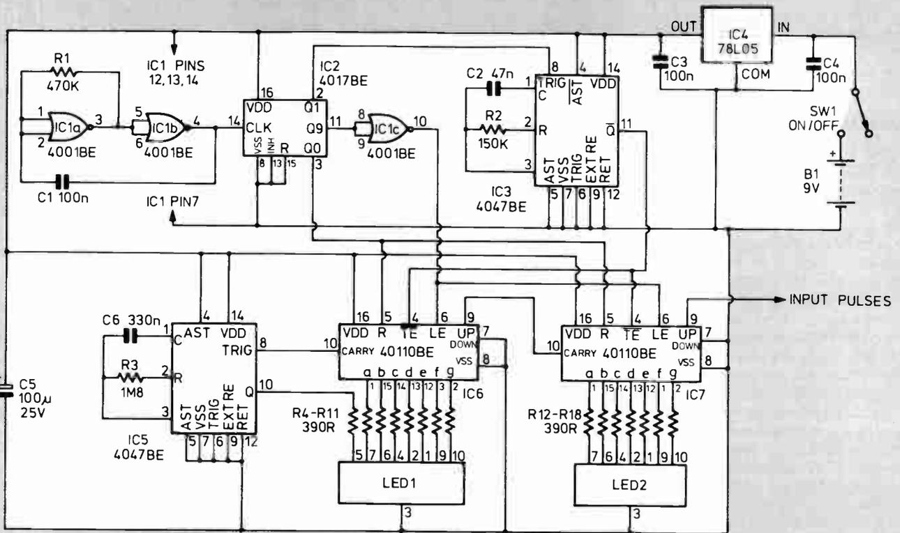
Figure 3: the circuit diagram of the display section.
