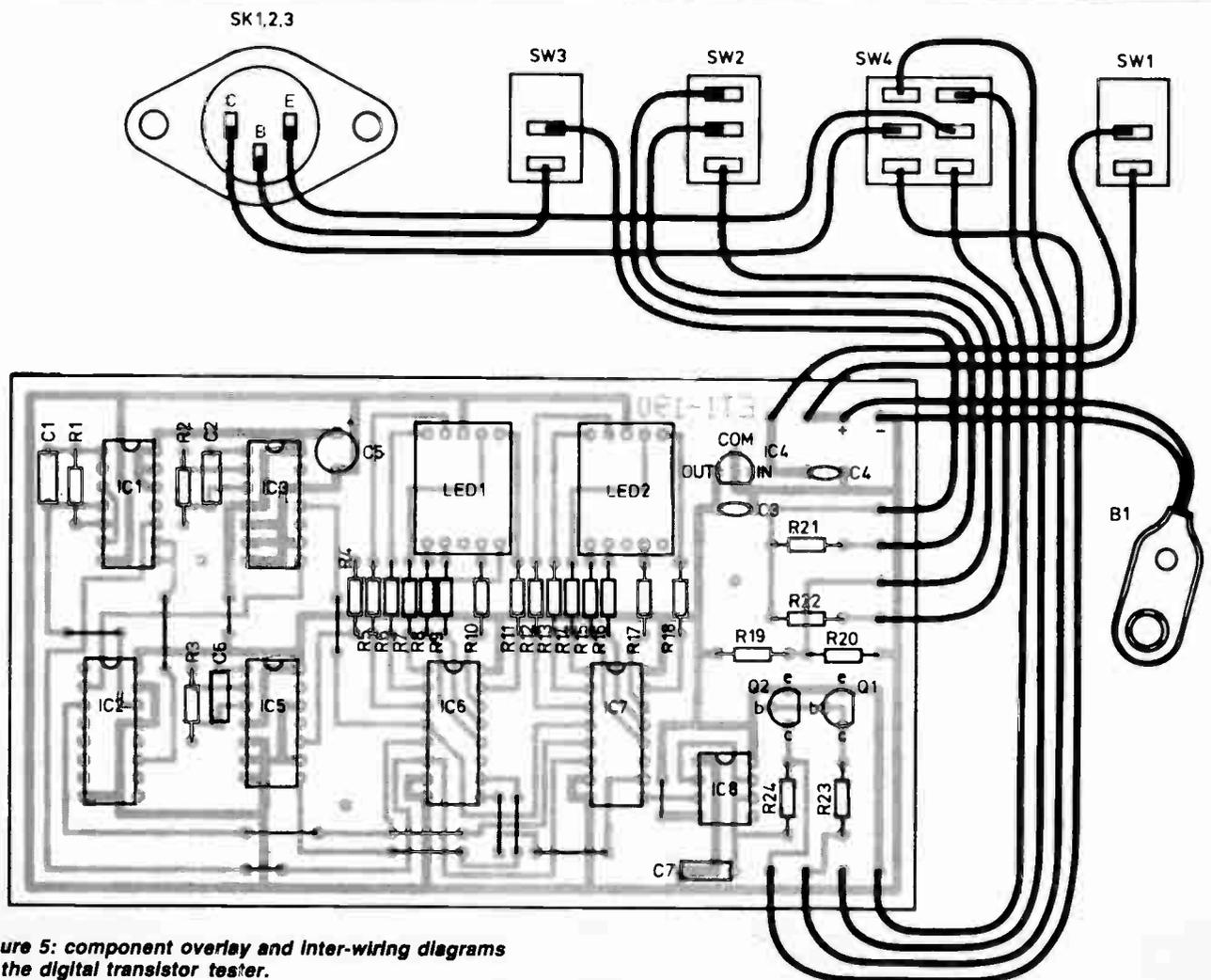
Figure 5: component overlay and inter-wiring diagrams for the digital transistor tester.
