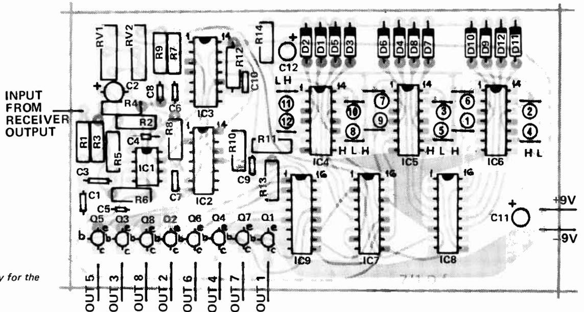
Fig. 7. Component overlay for the decoder.
