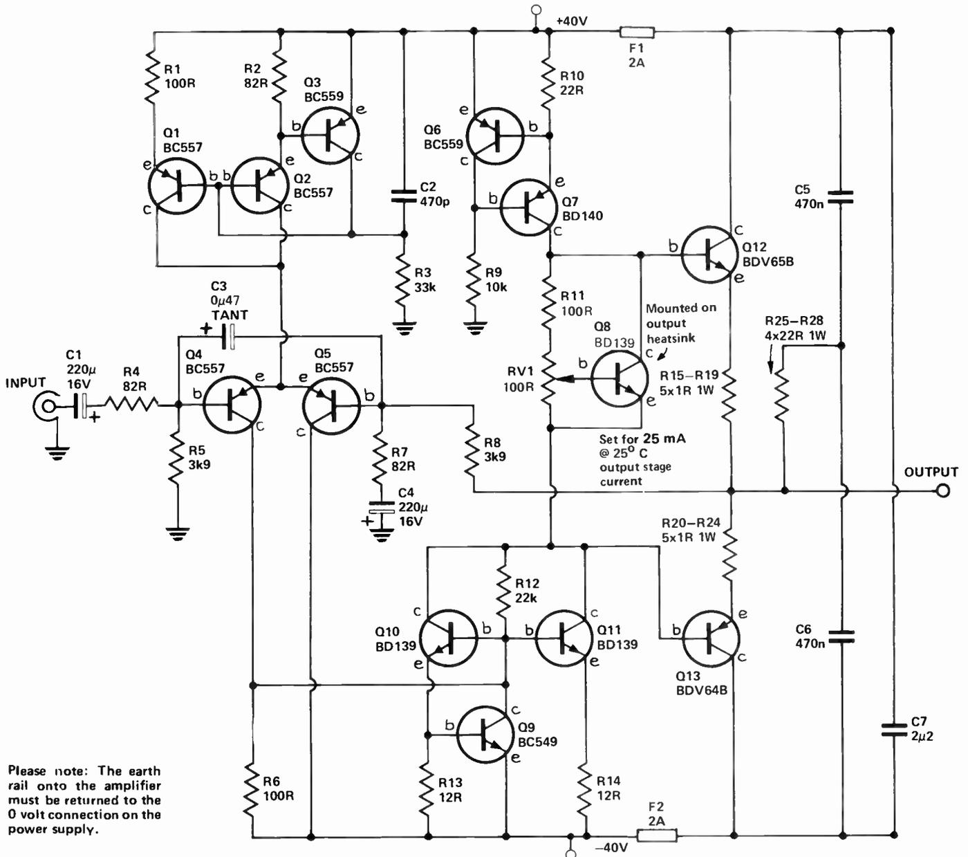
Please note: The earth rail onto the amplifier must be returned to the 0 volt connection on the power supply.
