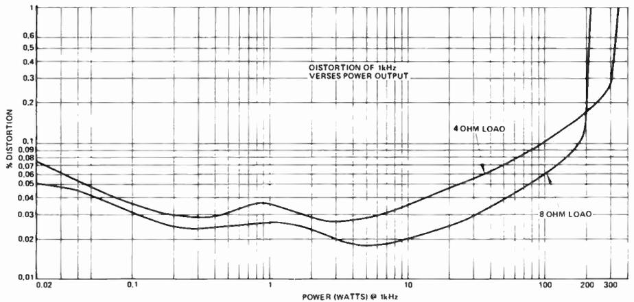
Total harmonic distortion versus power output at 1 kHz. The 'bump' at around 1 W is due to the output stage changing from Class A operation to Class AB operation.
