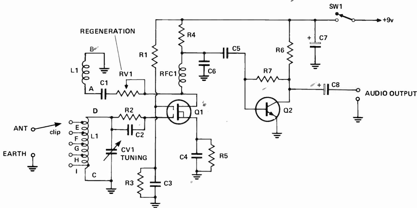
Fig. 1. Circuit diagram of the receiver.
