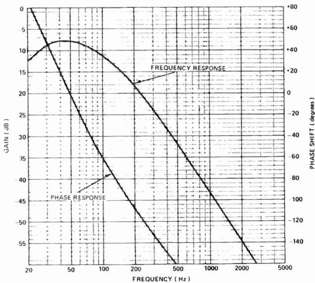
Fig. 6. The frequency and phase response of the control tone filter.
