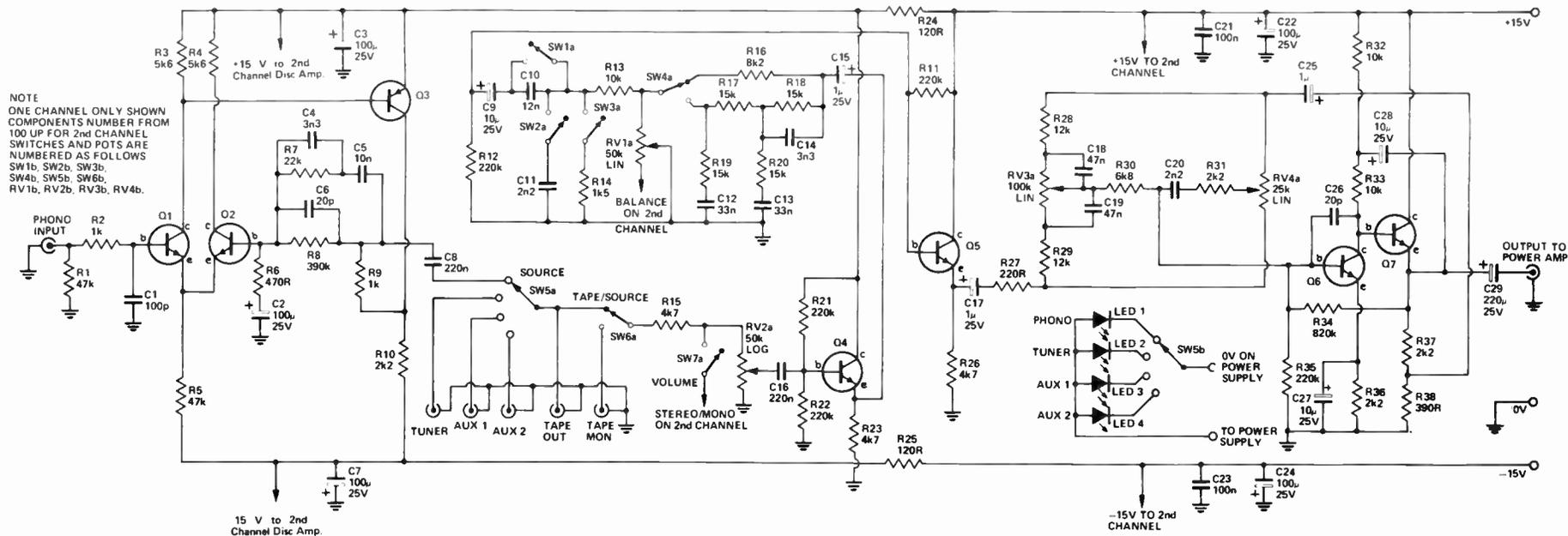
Fig. 1. Preamplifier circuit diagram. Only one channel has been shown for clarity. The component numbering of the other channel begins at 101.
