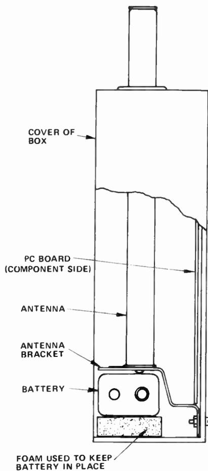
Fig. 4. Method of mounting the antenna and the battery by means of an aluminium bracket.
