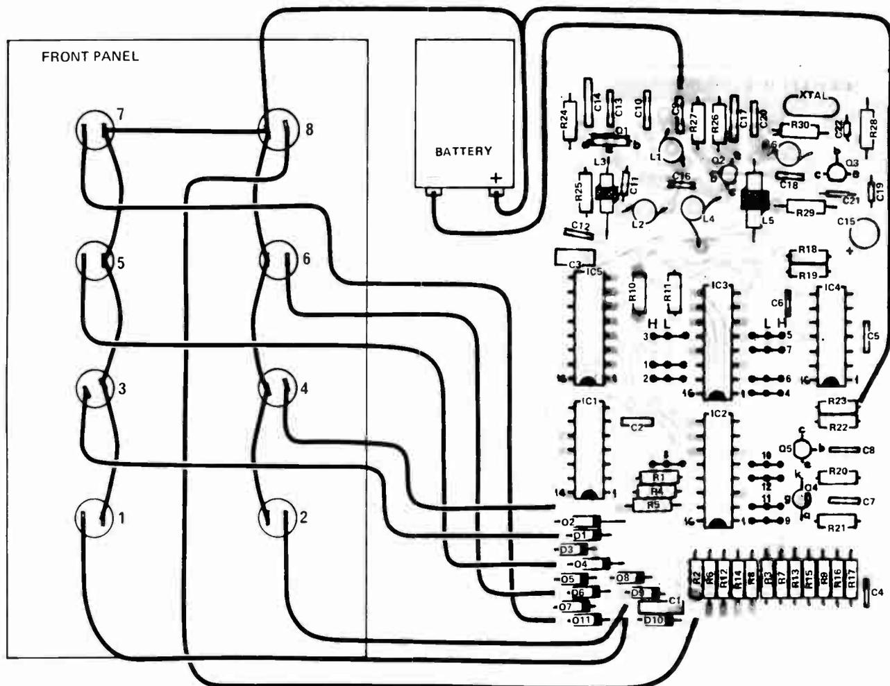
Fig. 7. Component overlay and wiring diagram. Note the links from IC2 and IC3 to the 'H' or 'L' lines. You must decide on the code word to be used and link to one or the other as detailed in the text. Overlay is shown larger than full size for clarity.
