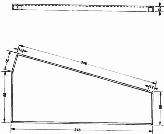
Fig. 4. The end pieces for the box. These should be fitted into the ends of the box as shown in Fig. 3. The two ends should be of opposite hands.
