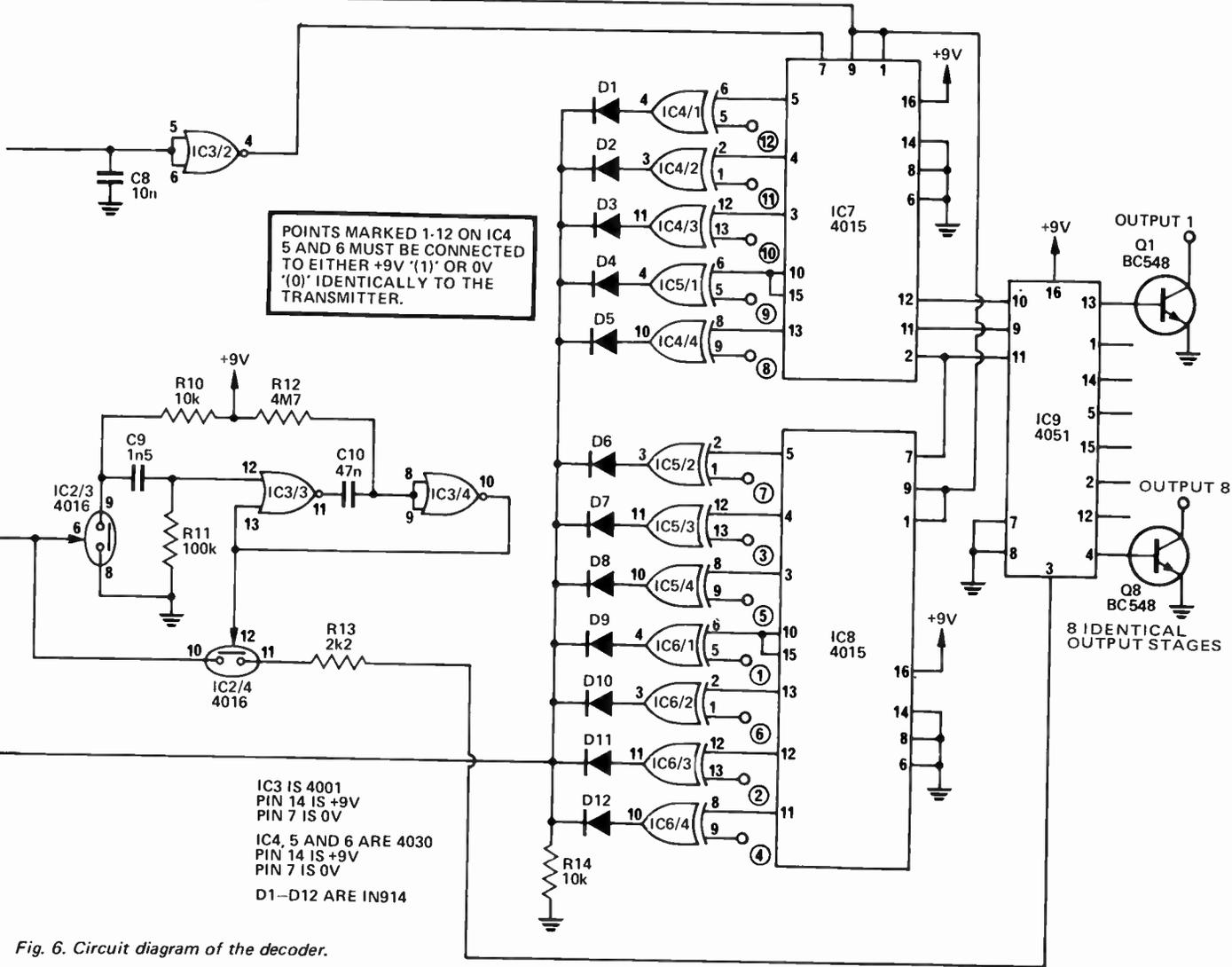
Fig. 6. Circuit diagram of the decoder.
