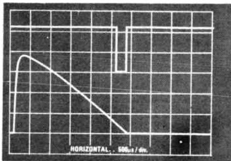
Fig. 3. Waveform showing relationship between the end of the half cycle and the sync pulse.
