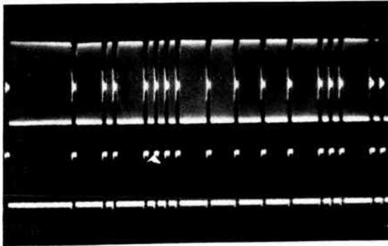
Fig. 2. One complete code word of 16 bits. At top is the gated CW as seen in the IF strip of the receiver whilst the bottom trace shows the output from the detector. The 4.8 millisecond sync pulse is at the left and is followed by the code word 101000111110010. The beginning of the next sync pulse can be seen on the right.
