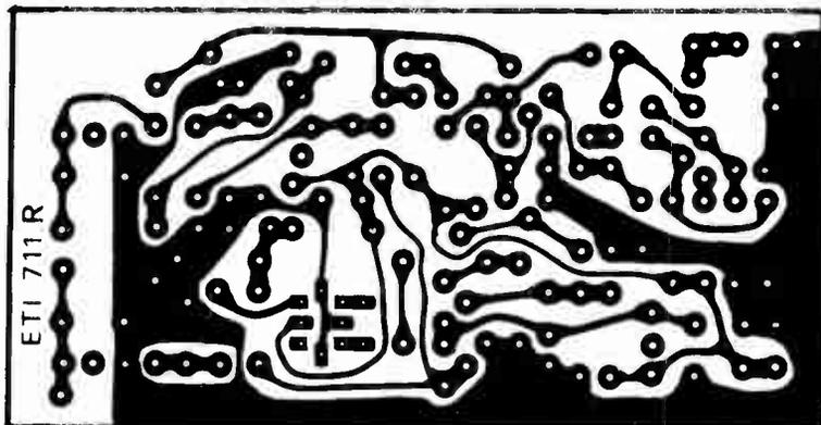
Fig. 5. Printed-circuit layout for the receiver.
