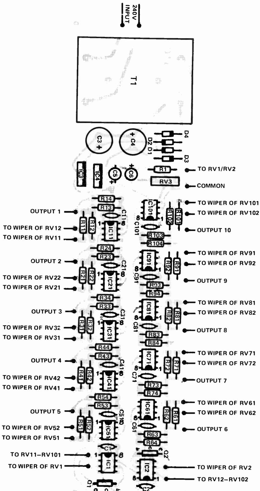
Fig. 2. Component overlay for the controller board, ETI588C.
