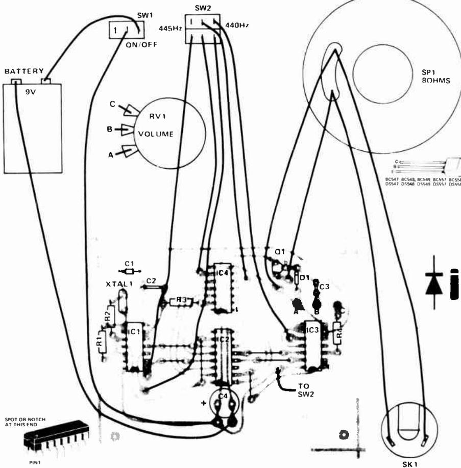
Component overlay. The pc board pattern is reproduced on page 158.
