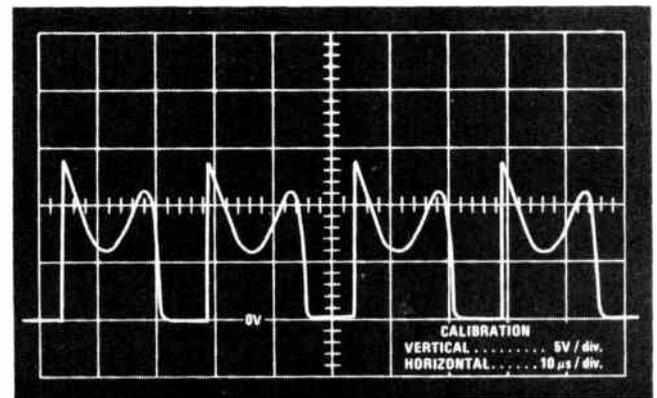
Fig. 3c. Voltage on the collector of Q2.
