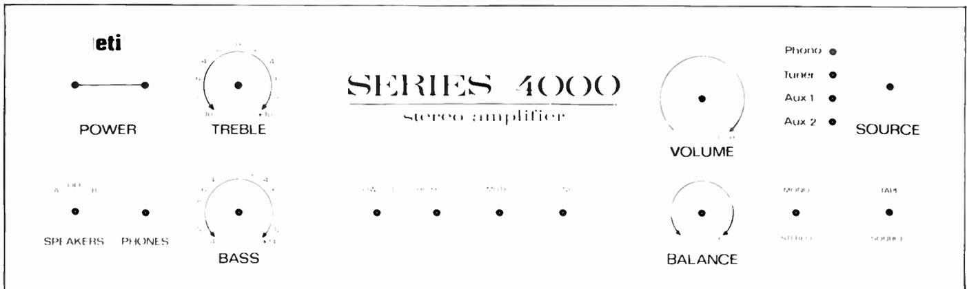
THIS stereo preamplifier is designed to drive two 60 watt, low distortion amplifier modules (FTI 470), described in the previous article.
