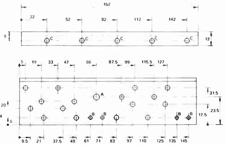
Drilling details for the heatsink bracket assembly. All dimensions are in millimetres. Suitable aluminium angle stock is available from Alcan Handyman stores.
