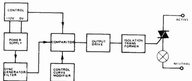
Fig. 4. Block diagram of the dimmer module.
