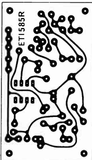
Fig. 6. Printed circuit board of receiver.
