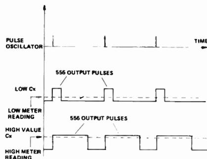
The unknown capacitance,  $C_x$ , determines the width of the output pulses from the 555 monostable. The meter integrates these pulses to produce a reading which is directly proportional to the unknown capacitor's value.
