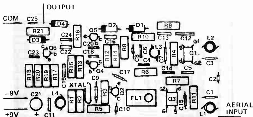
Fig. 4. Component overlay for the receiver.
