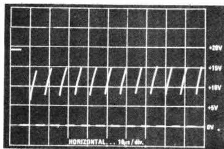
Fig. 4. An expanded view of the transformer drive waveform showing the collector voltage of Q1.
