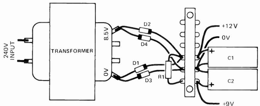
Fig. 8. Interconnection diagram for the power supply.
