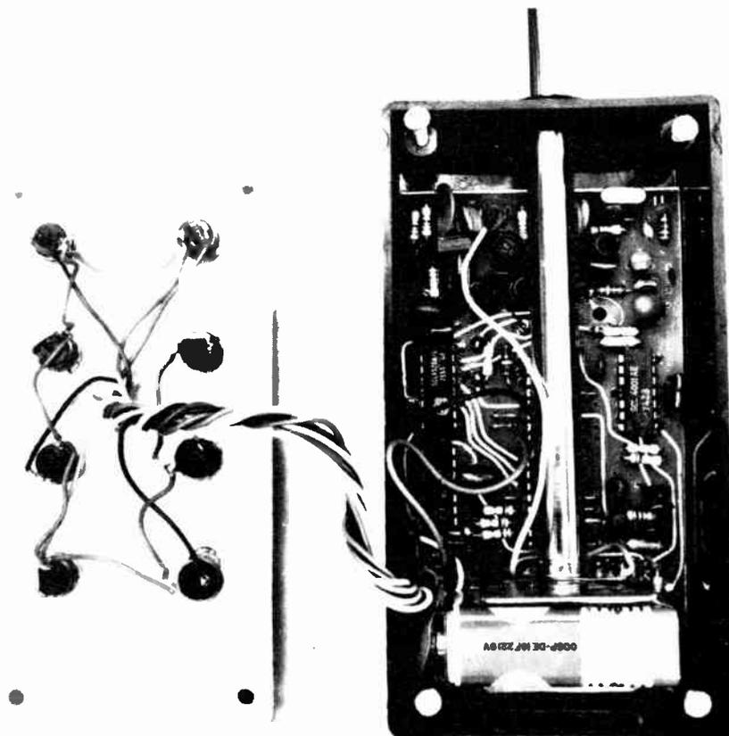
Fig. 6. The transmitter installed in the box. Note the method of mounting the antenna and the battery.
