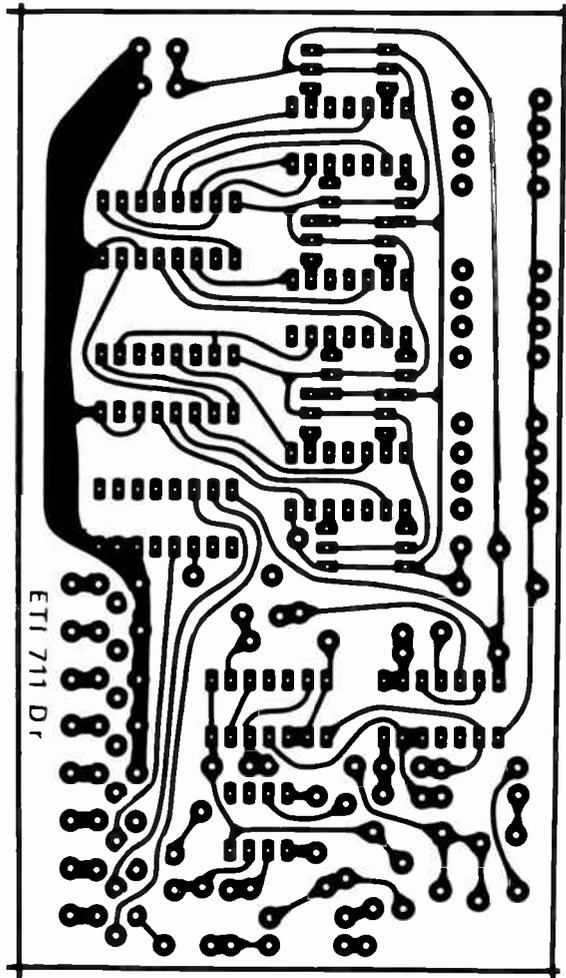
Fig. 8a. Non-component side of the decoder board. Full size 127 x 69 mm.
