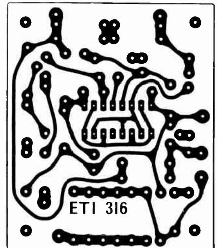
Fig. 3. Printed circuit board. Full size 65 x 55 mm.
