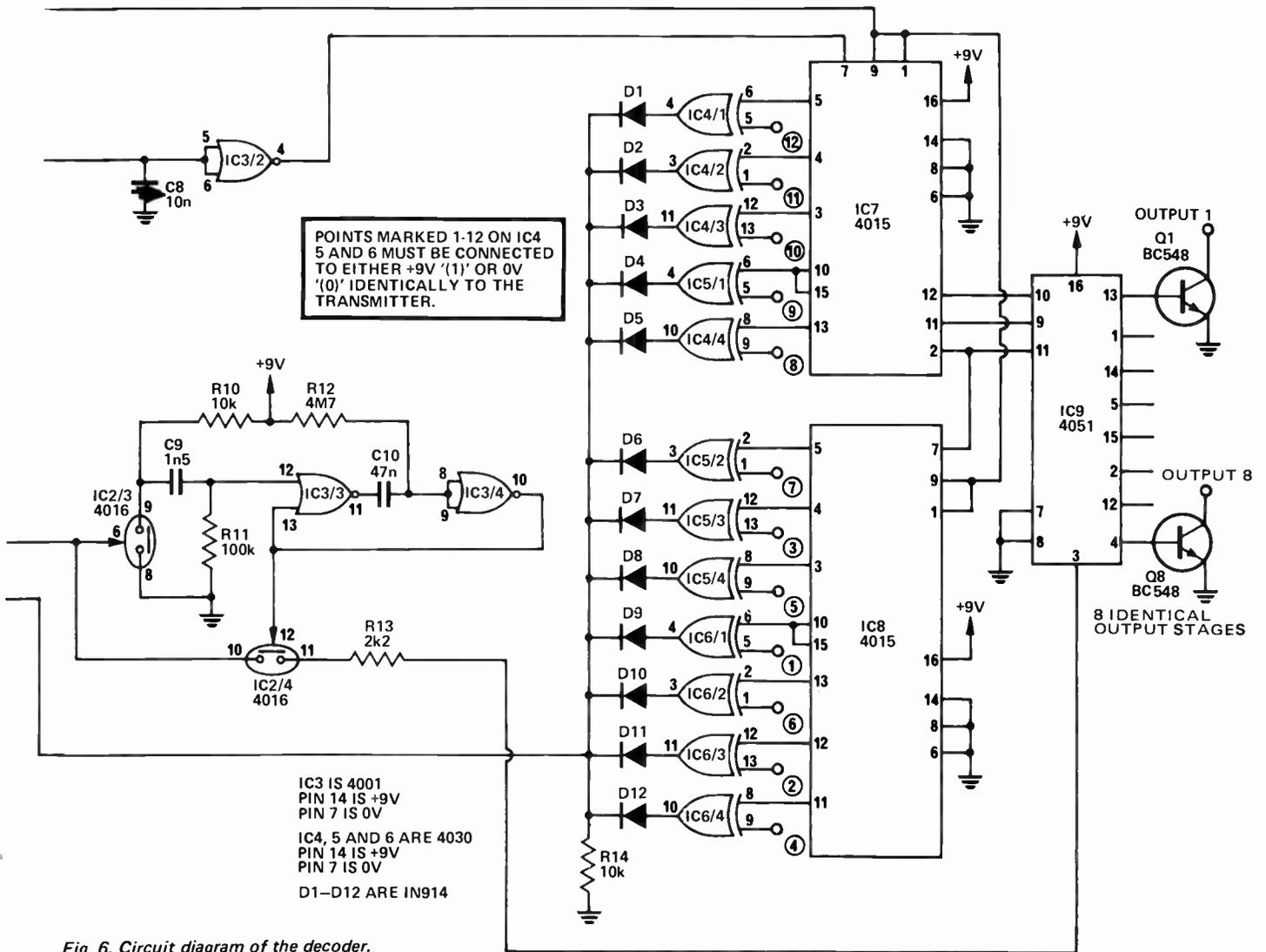
Fig. 6. Circuit diagram of the decoder.
