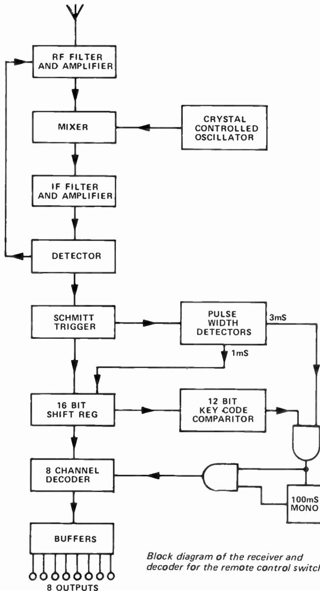
Block diagram of the receiver and decoder for the remote control switch
