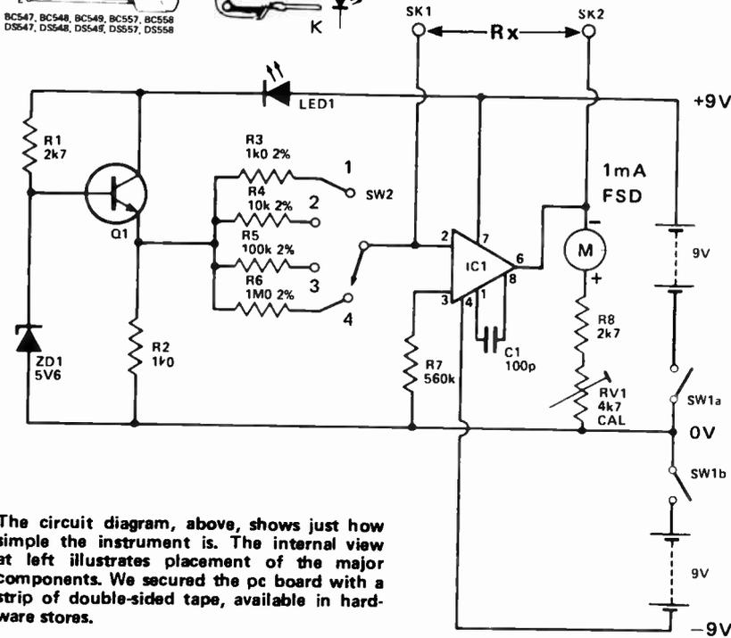
The circuit diagram, above, shows just how simple the instrument is. The internal view at left illustrates placement of the major components. We secured the pc board with a strip of double-sided tape, available in hardware stores.
