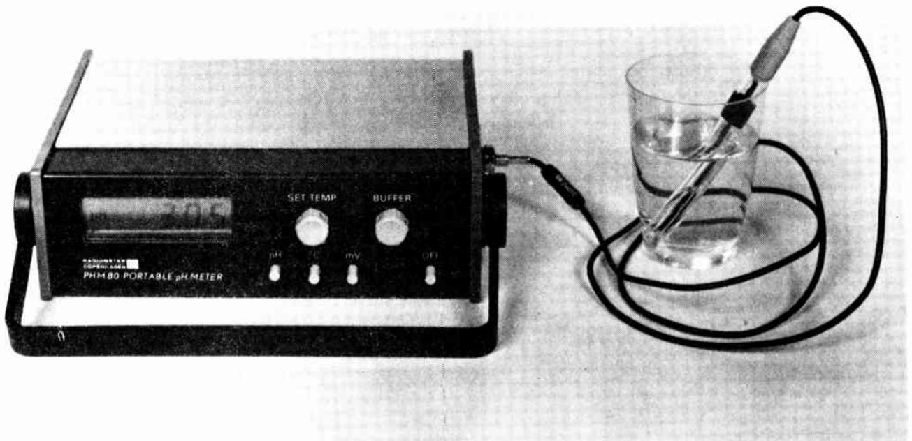
A high quality portable pH meter with a liquid crystal display that directly indicates the pH of the solution under test.
