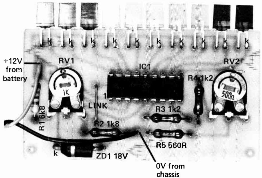
ing the reading (such as in the headlight wiring). The chassis connection can be made to the car body under the dash, wherever convenient, or taken to a chassis connection point in the engine bay.
