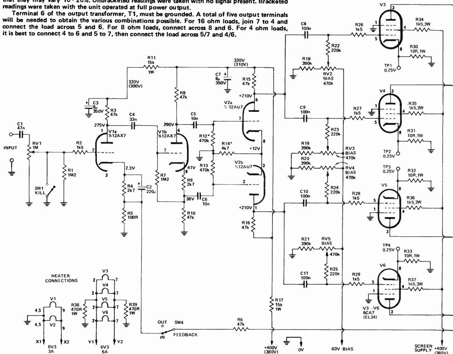
The amplifier has four separate stages: the input voltage amplifier, a phase-splitter, a push-pull driver stage and a push-pull power output stage.
