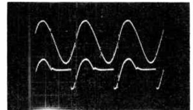
E) Same as pic (D) but with metal target near the search head. Note the increase in average dc level from the output of IC1b. The change in this signal is much larger for non-ferrous than for ferrous metals.
