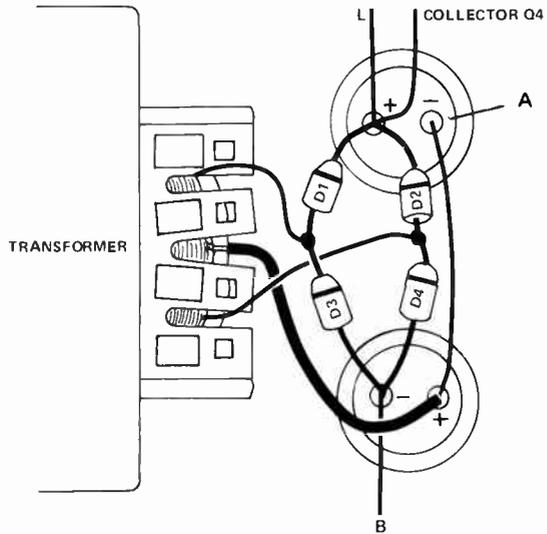
Fig. 5. How the supply is wired for the 40 volt 1.25 ampere version.
