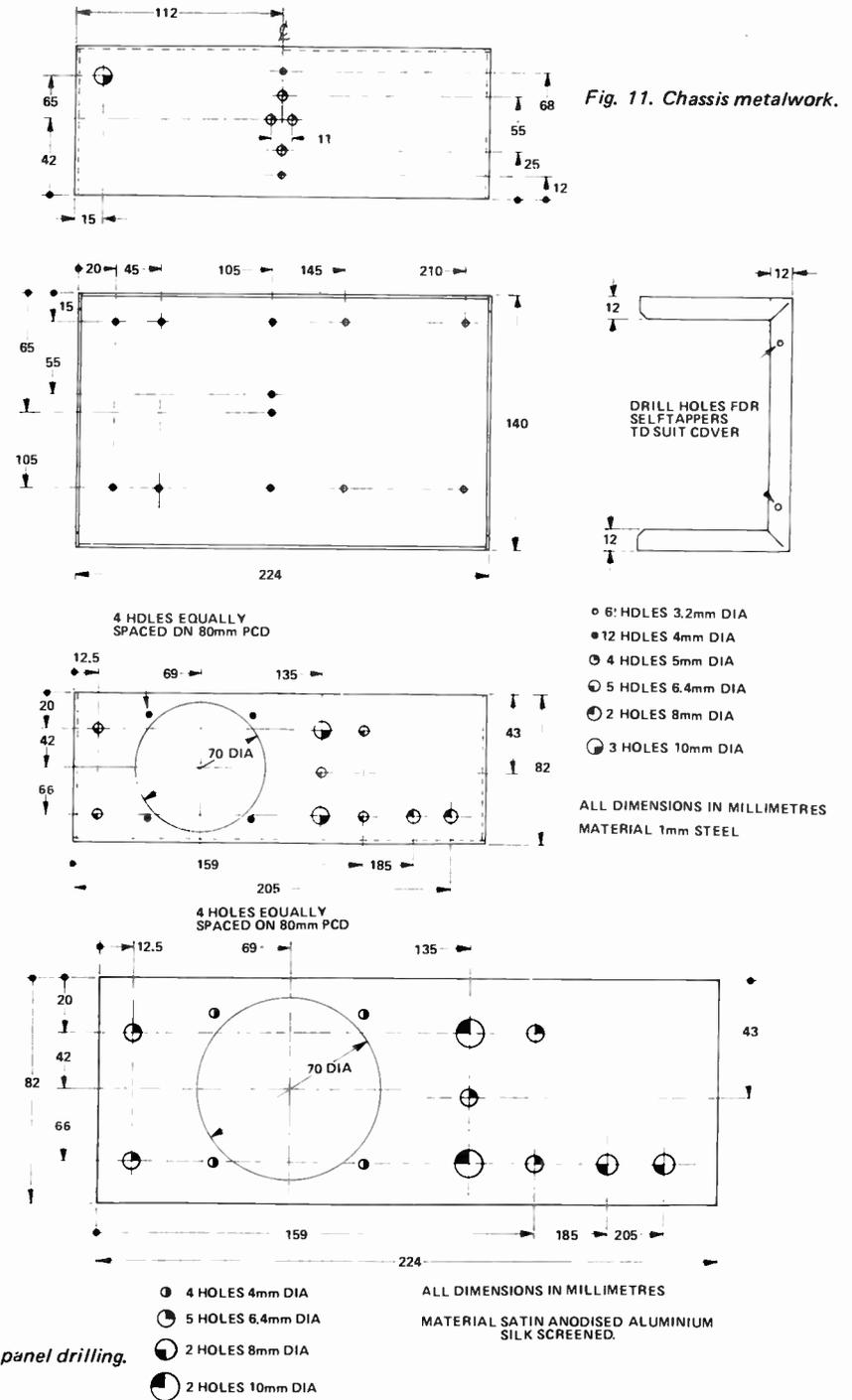
Fig. 12. Front panel drilling.
