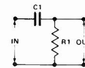
Figure 2 (a). Simple passive high-pass filter.
