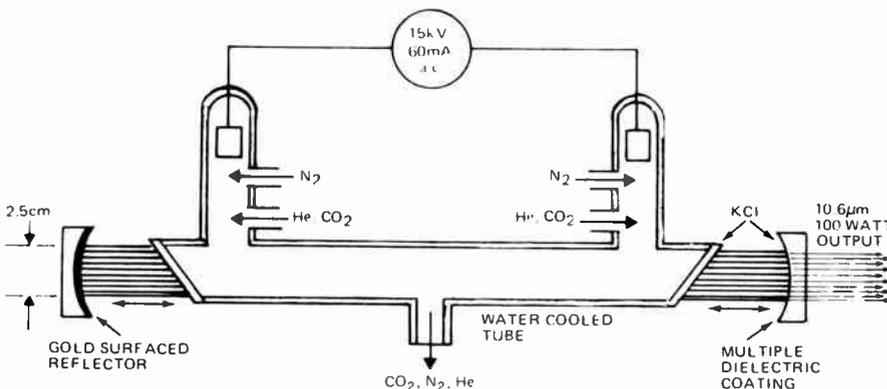
Some gas lasers can generate enormous output powers. This diagram illustrates the general construction of a carbon dioxide laser.
