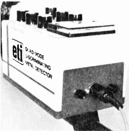
A view of the forward end of the case showing the two battery test pushbuttons and the DIN plug and socket connection to the search head. The Atek cabinet is two-tone grey plastic. The upper section is a lighter hue. Note the "GT" stripes!
