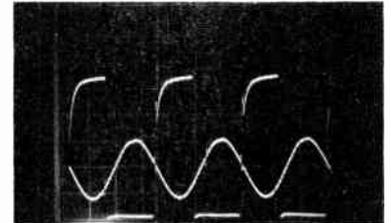
C) As per pic (B) but with aluminium target held near search head. Note the phase delay and change in amplitude of the received signal.
