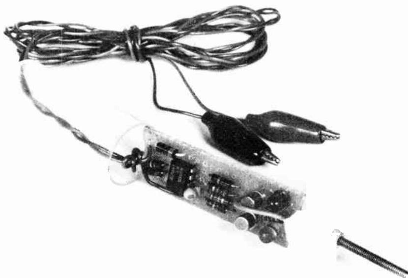
The Auto-probe is housed in a common pill bottle. You can construct it either on matrix board, as shown here, or on a printed circuit board (see over the page). It's an amazingly handy gadget!
