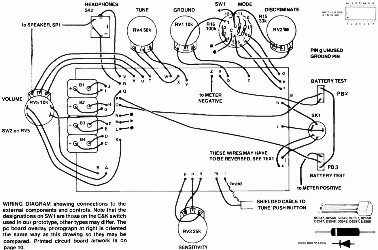
**WIRING DIAGRAM** showing connections to the external components and controls. Note that the designations on SW1 are those on the C&K switch used in our prototype, other types may differ. The pc board overlay photograph at right is oriented the same way as this drawing so they may be compared. Printed circuit board artwork is on page 10.
