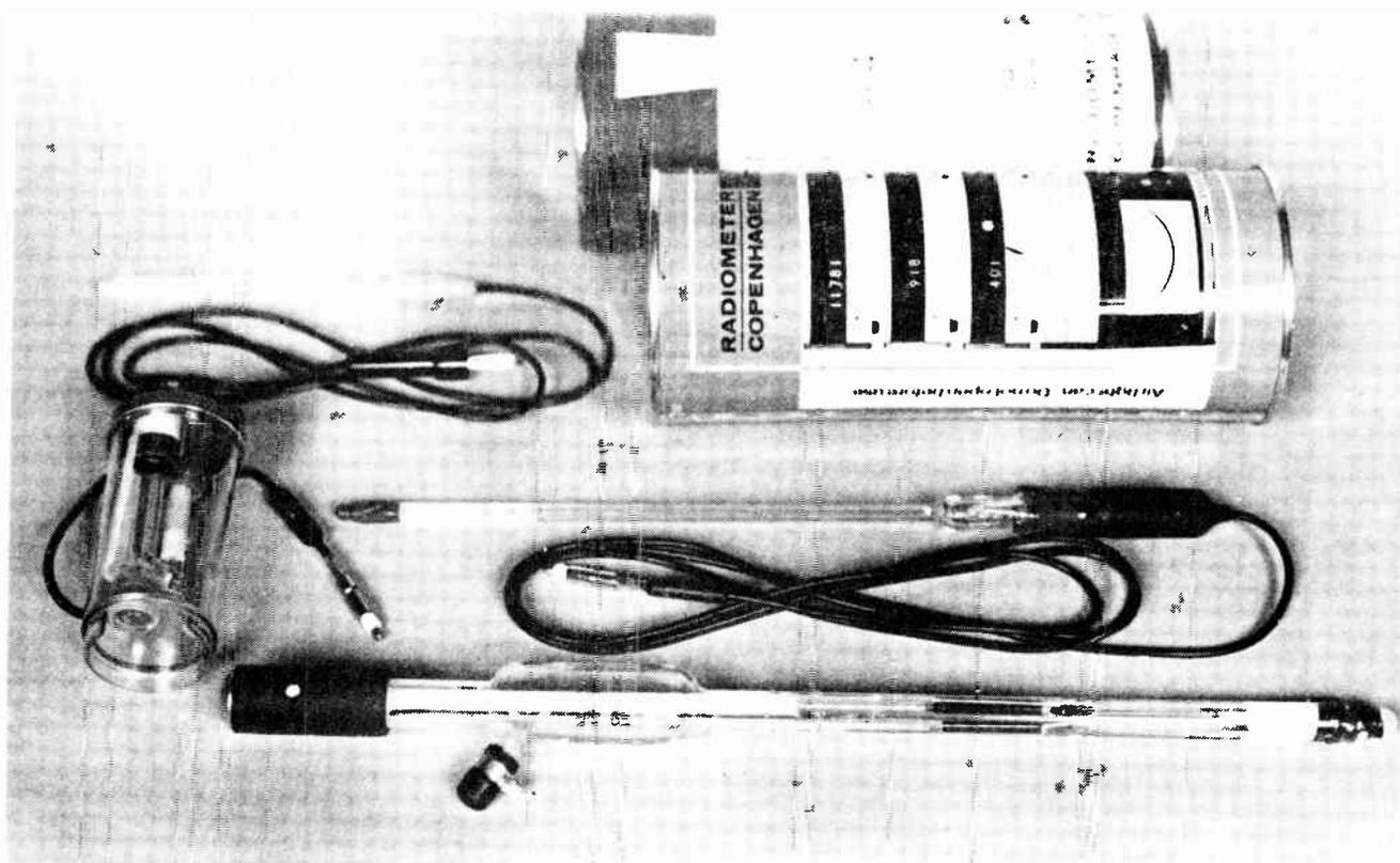
pH electrodes are made in a variety of shapes and sizes to suit different applications. at the rear of the picture are two cans of 'buffer solutions' — liquids whose pH does not change much when they are contaminated. Buffer solutions are used to calibrate pH electrodes.
