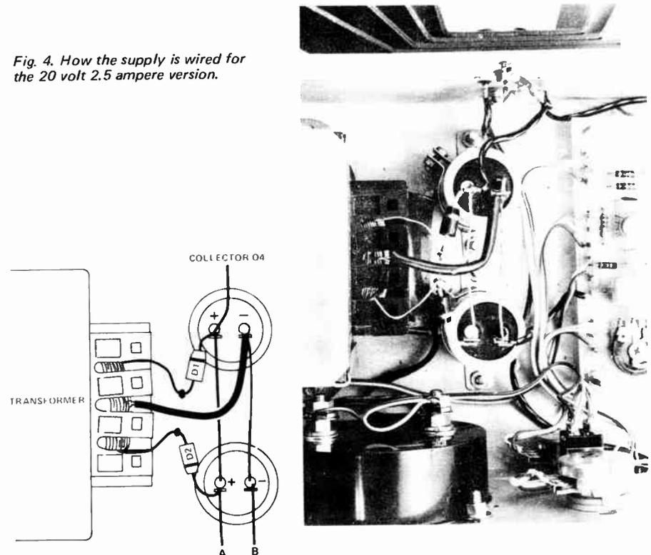
Fig. 4. How the supply is wired for the 20 volt 2.5 ampere version.
