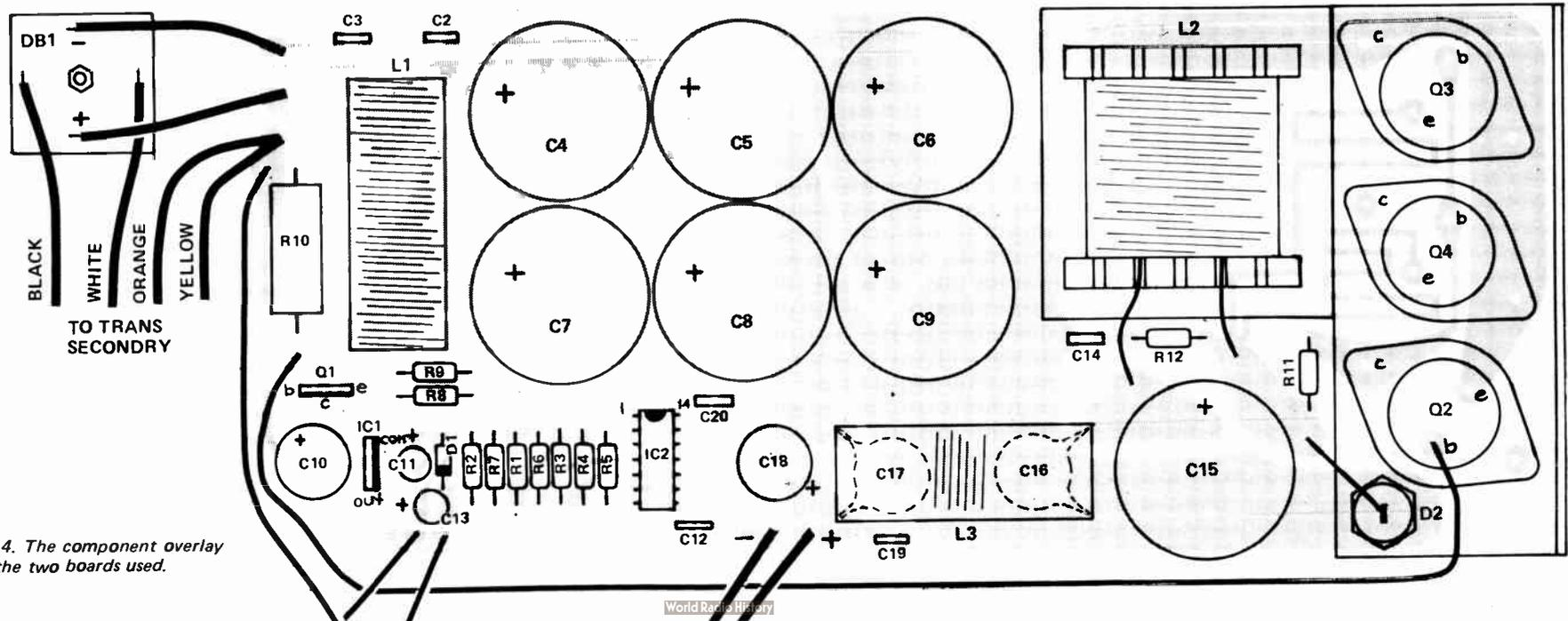
Fig. 4. The component overlay for the two boards used.
