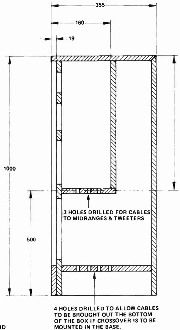
Complete cutting and assembly details for the four-way loudspeaker box. It is important that all joints be well sealed.
