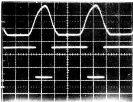
Waveforms around IC1. At top is the waveform on the input, bottom shows the output.
