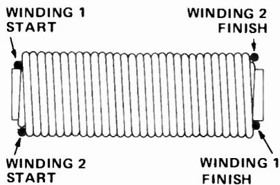
Fig. 2. L1, 3 with the first layer wound (top) and with both layers wound (lower).
