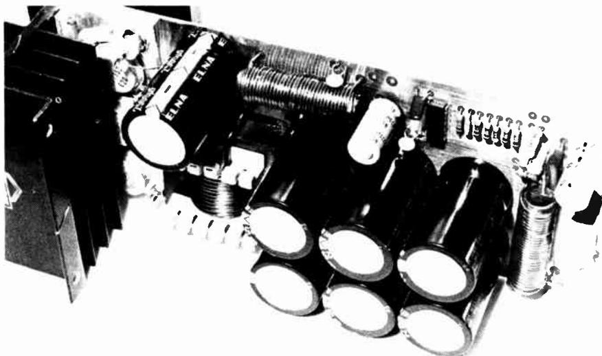
hookup wire about ½ meter long, baring one end and soldering them into the lower row of holes in the series regulator board. Add similar wires to the switching regulator board for the +40V and control input connections. To the output pads on this board, add about 200 mm of wire capable of handling 15A.
