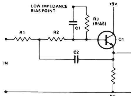
Figure 5 (a). Two-stage low-pass filter.
