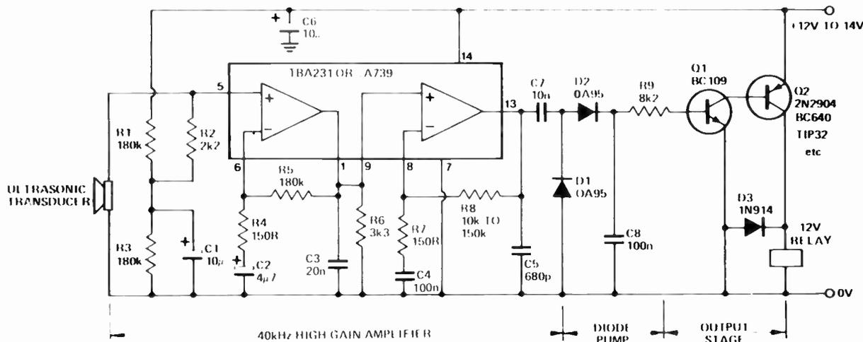
Figure 7. Receiver circuit using the TBA231 or uA739 as a high gain amplifier.
