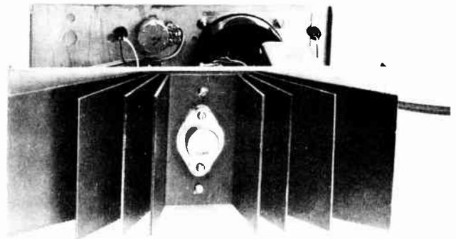
*Rear view of the heatsink showing how it and the transistor are mounted.*
