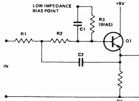
Figure 5 (a). Two-stage low-pass filter.
