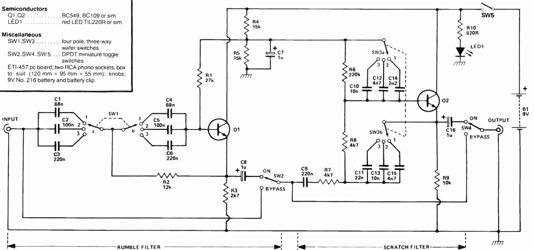
Figure 1 shows the block diagram of the mono version of the scratch and rumble filter. The input signal (from the turntable pick-up) is first fed through a high-pass filter, which rejects unwanted low-frequency rumble signals, and is then fed through a low-pass filter which rejects unwanted high-frequency scratch signals. Each filter can be bypassed via a simple switch if required, so the input signal can be passed through either one, both, or neither of the filters.
