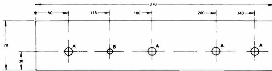
VALVE AMP CHASSIS FRONT LAYOUT DIMENSIONS
