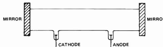
Figure 7. Basic construction of a gas laser. A glass cylinder, containing a gas at a low pressure, has two mirrors placed at either end — one is totally reflective, the other slightly transmissive. When current is passed through the gas, population inversions of the atoms occur and laser action results.
