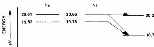
Figure 6. Energy level diagram for the helium-neon laser.
