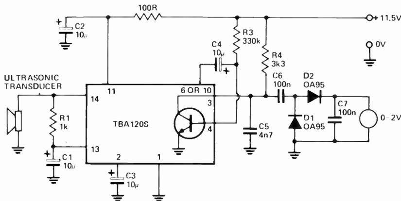
Figure 8. A receiver employing the TBA120S as an amplifier and featuring a meter display.
