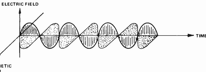
According to the electromagnetic wave theory, light is seen as a continuous wave of oscillating electric and magnetic fields.
