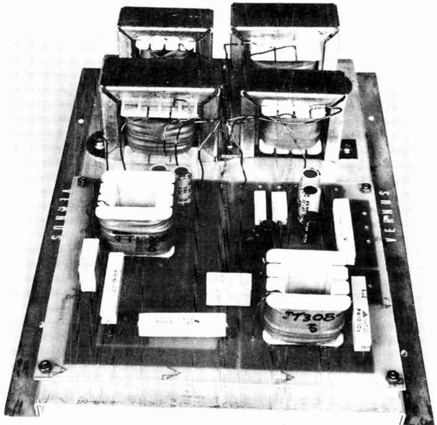
We mounted the crossover network assembly on an aluminium plate, bent as shown. The whole assembly was then screwed to the bottom of the loudspeaker and each driver connected as per the overlay.
