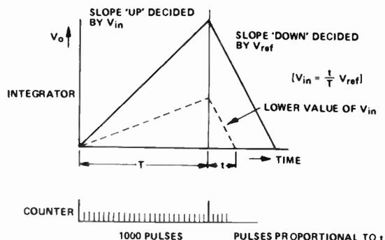
Timing diagram for the dual-slope A/D conversion technique.
