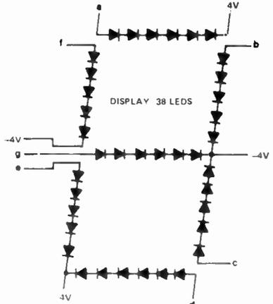
A total of 38 LEDs are used in each seven-segment display. Each of the vertical segments uses five LEDs, while the horizontal segments use six.
