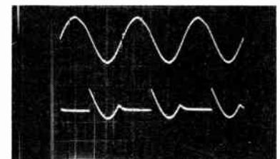
I) As per pic (G) but steel target held near search head. Note the decrease in average dc level of the signal at the output of IC1b, illustrating discrimination.
