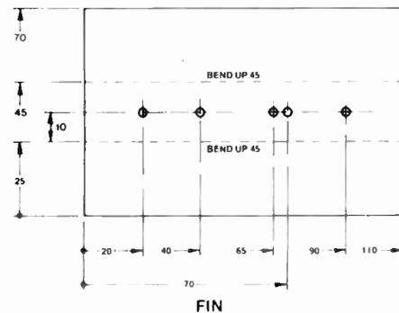
HEATSINK DIMENSIONS FOR 25 WATT UNIT
