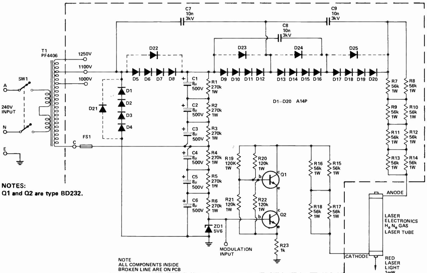
swamping resistance is determined from the particular tube's characteristics and, for this reason, laser tubes are supplied with details of the required minimum series anode resistance and our circuit adheres to the requirements of the tube supplied by Laser Electronics.
