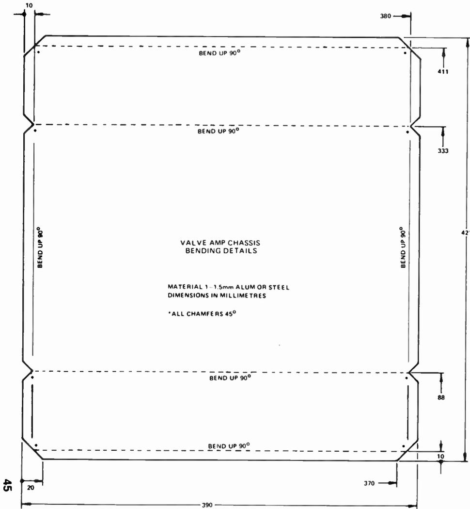
VALVE AMP CHASSIS BENDING DETAILS
