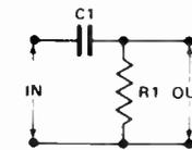
Figure 2 (a). Simple passive high-pass filter.
