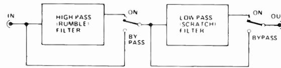
Figure 1. Block diagram, scratch and rumble filter.
