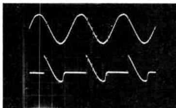
H) As per pic (G) but brass target held near search head. Note the increase in the average dc level of the signal at the output of IC1b.
