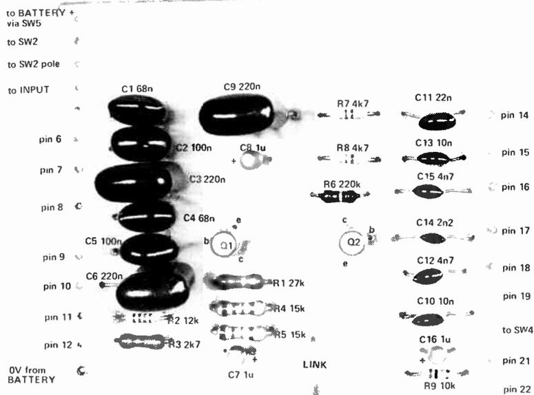
Component overlay for the pc board. Note that pin numbers 1 to 5, plus 13 and 20, are not used. Resistor R10 and the indicator LED1 are mounted off the pc board (we have not used these).
