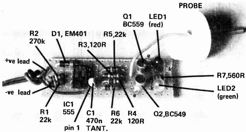
Matrix board construction showing the component positioning and orientation. Note that we used the metal-can type transistors (BC109 etc) in this prototype. R3 and R4 are ½W GLP types.
