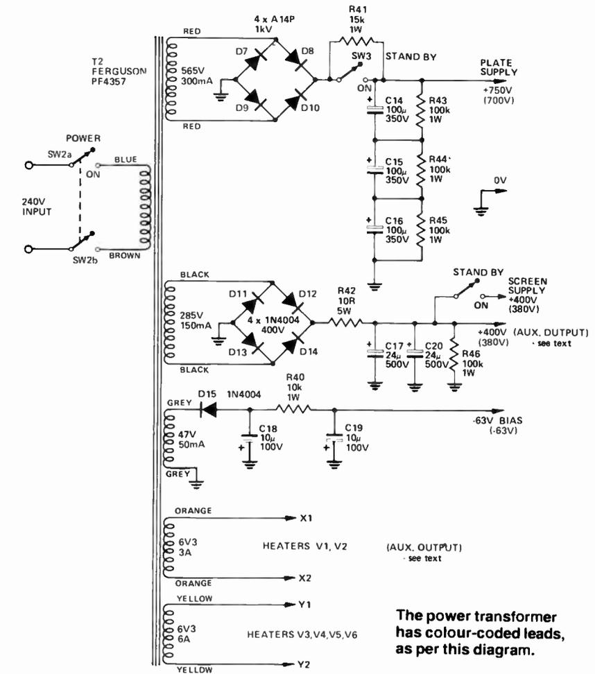
**The power transformer has colour-coded leads, as per this diagram.**
