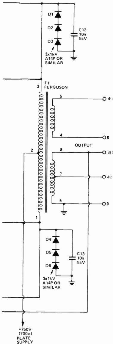
capable of driving four, eight or sixteen ohm loads, or two four ohm loads simultaneously.
