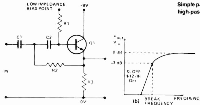
Figure 3 (a). Two-stage active high-pass filter. Figure 3 (b). Frequency response.
