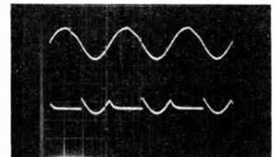
G) Top trace: received signal on emitter of Q2. Bottom trace: output of IC1b showing composite waveform of received signal 'mixed' with a dc level. Detector set to TR1 mode, discriminate control to 9. (Both traces 2 V/div, ac-coupled; time base 20 us/div).
