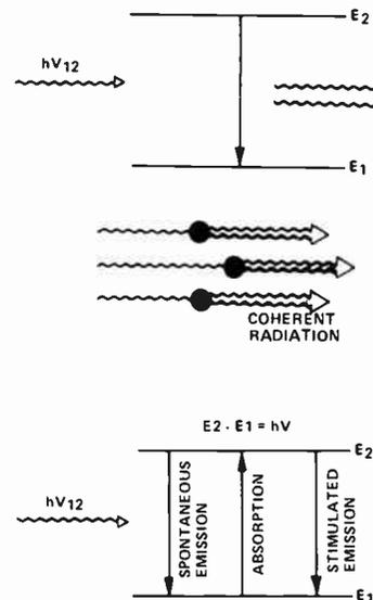
Figure 5. Energy level diagram for the process of stimulated emission.
