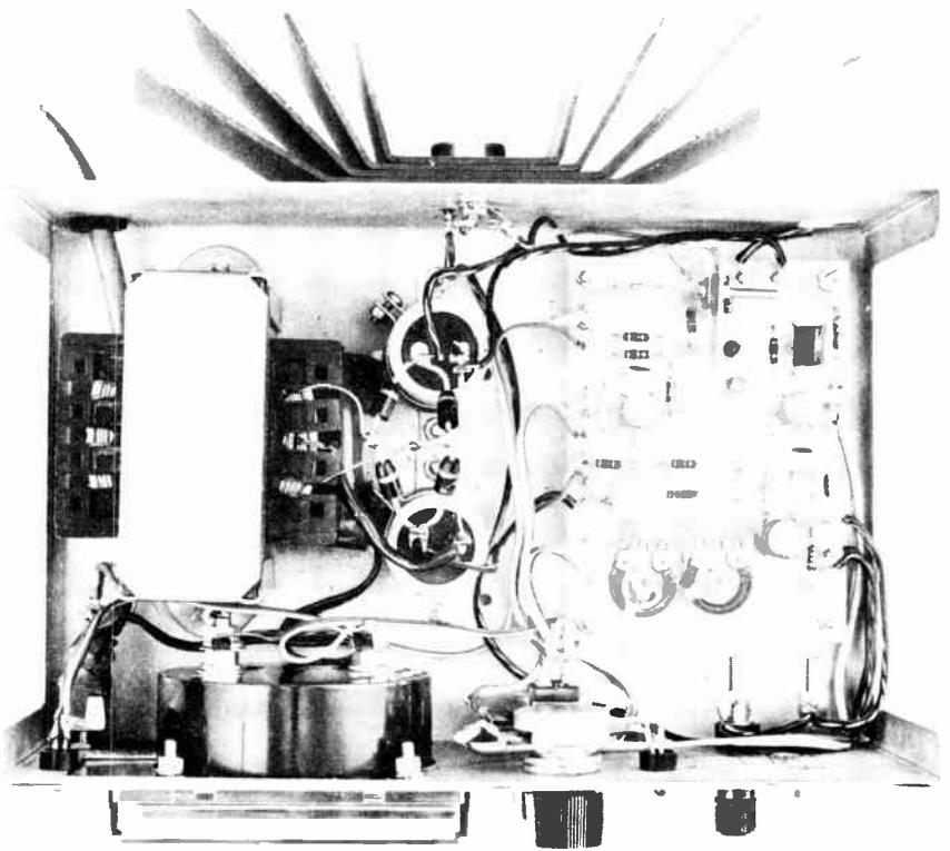
*Inside view of the completed 40 volt power supply. Note how the heatsink is mounted to the rear of the unit.*
