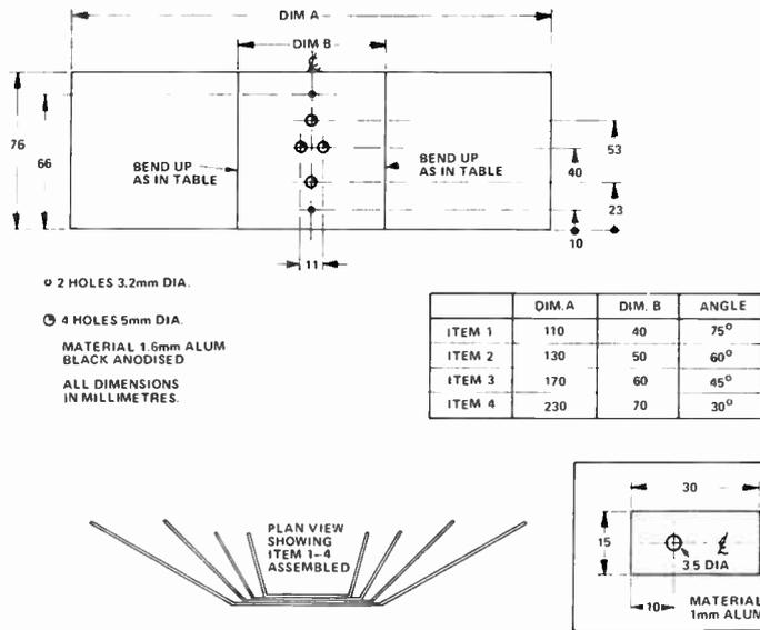
Fig. 10. Heatsink detail.
