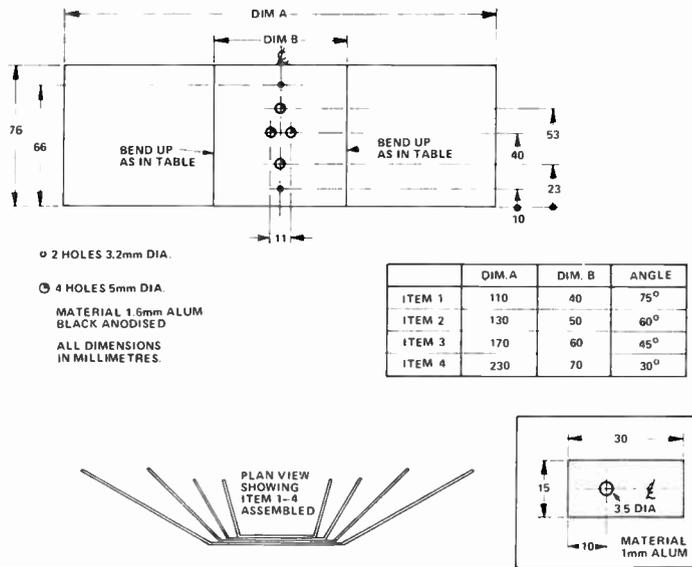
Fig. 10. Heatsink detail.
