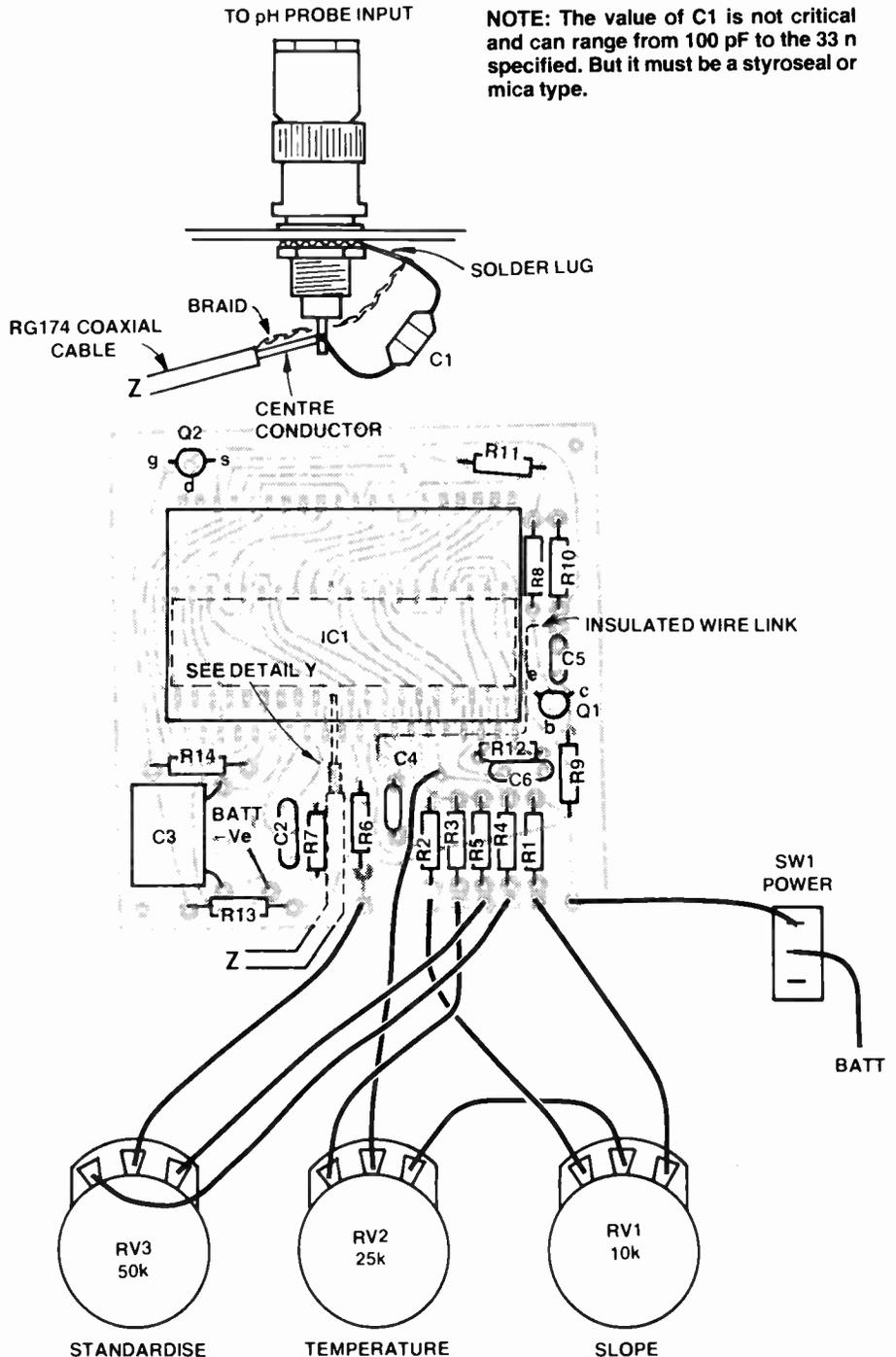
**NOTE:** The value of C1 is not critical and can range from 100 pF to the 33 n specified. But it must be a styroseal or mica type.
