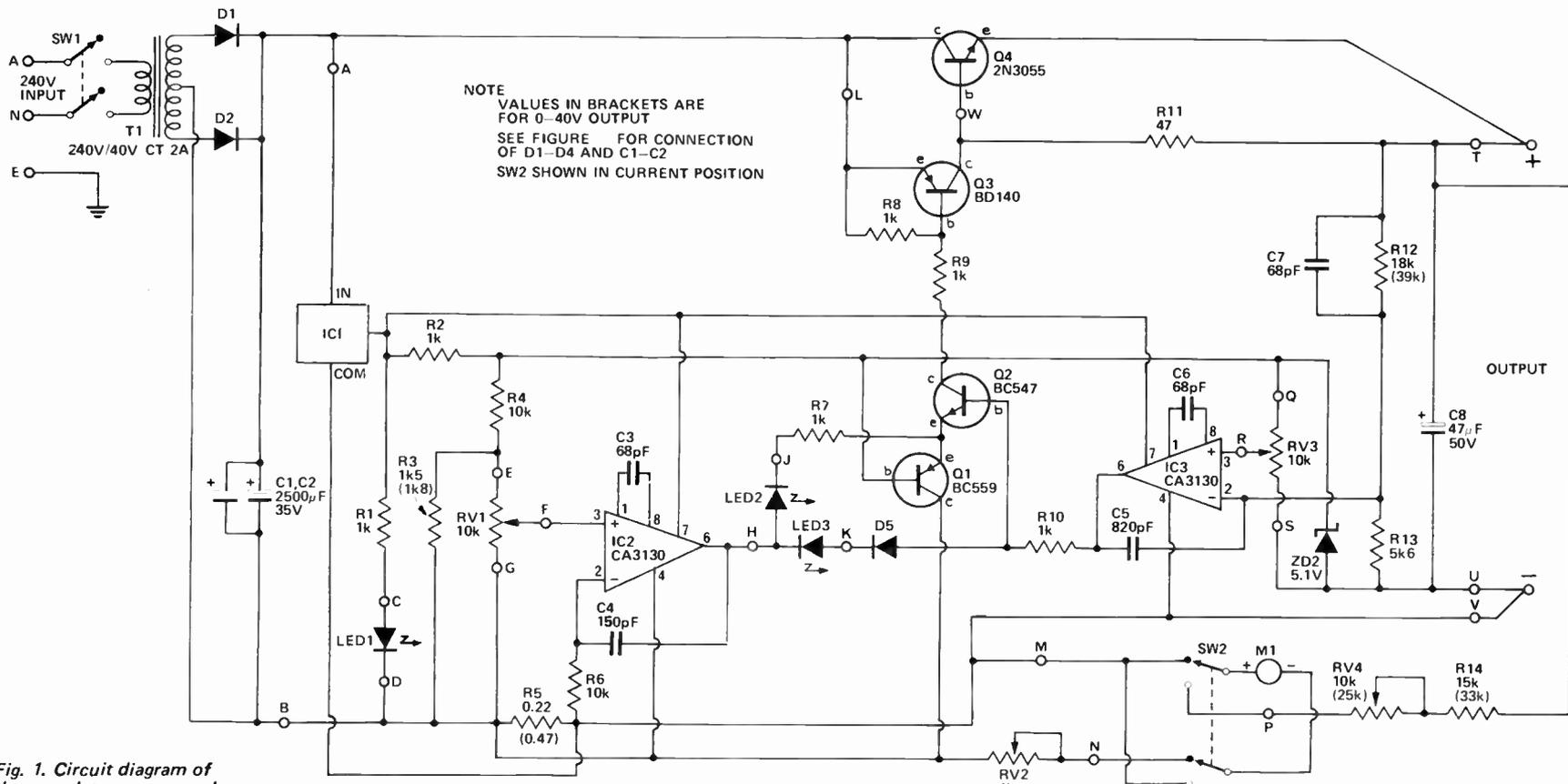
Fig. 1. Circuit diagram of the complete power supply 20 volt 2.5 ampere version.
