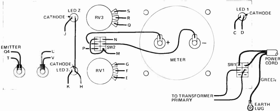
Fig. 6. Front panel wiring diagram.
