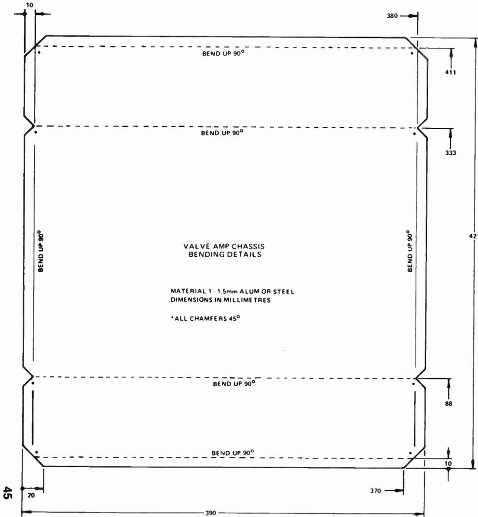
VALVE AMP CHASSIS BENDING DETAILS
