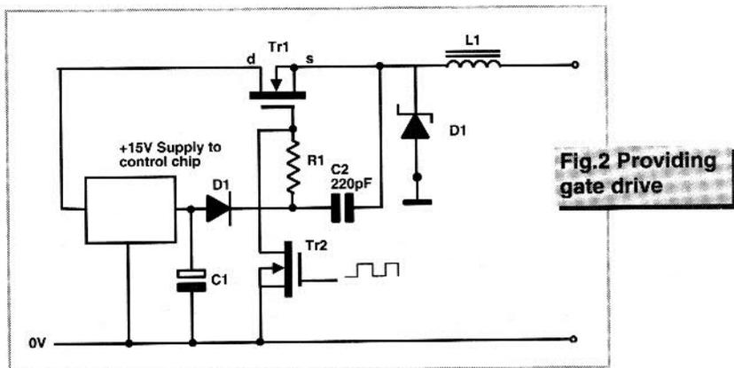
**Fig.2 Providing gate drive**
