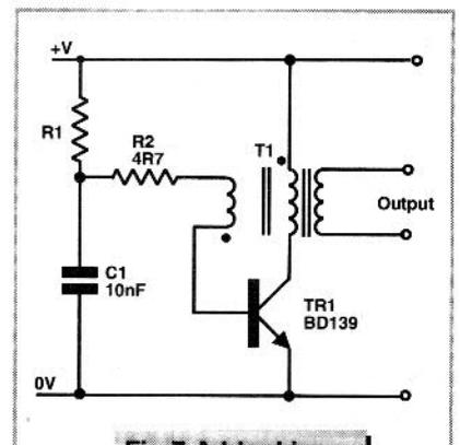
**Fig.7 A blocking oscillator design**
