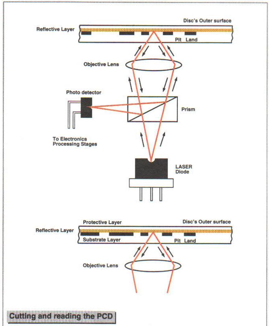
Cutting and reading the PCD
