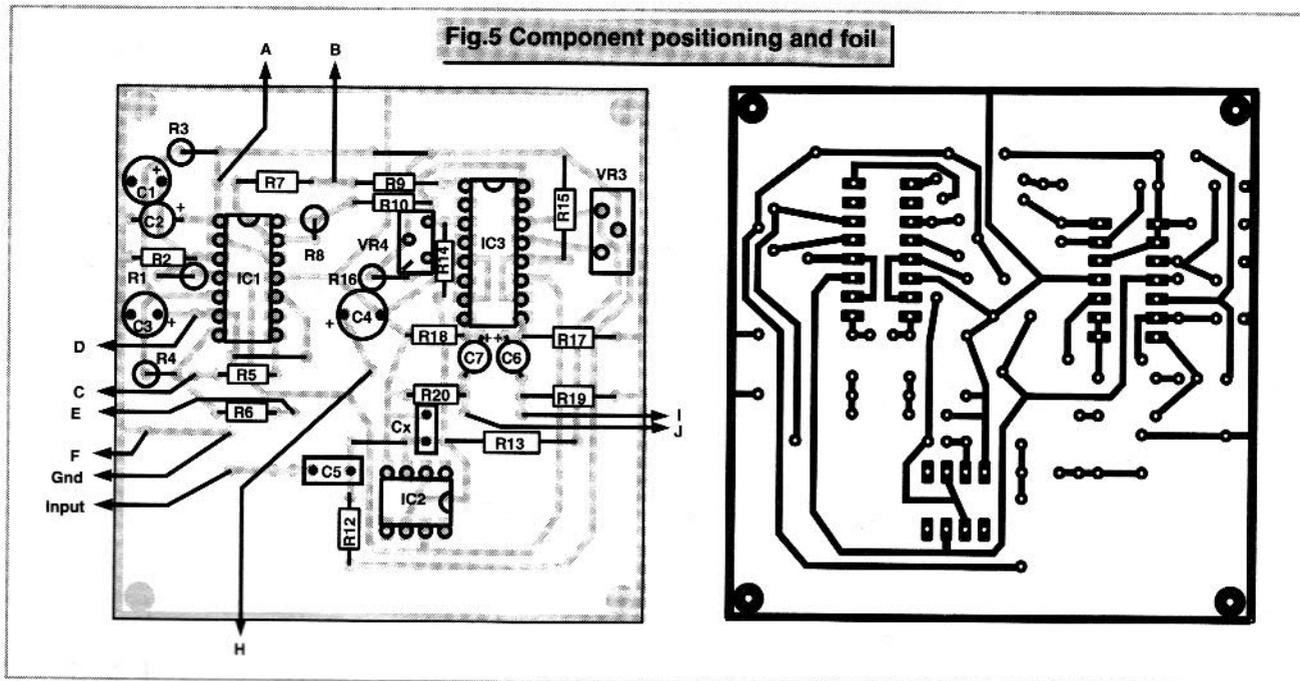
If this problem arises, try using a polystyrene capacitor of around 470pF. If this fails, increase the value until the RF is eradicated, but remember that too high a value may cause treble loss with high impedance sources - experimentation is the best way to solve this!
