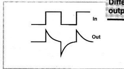
**Fig.5 Differentiated output drive**
