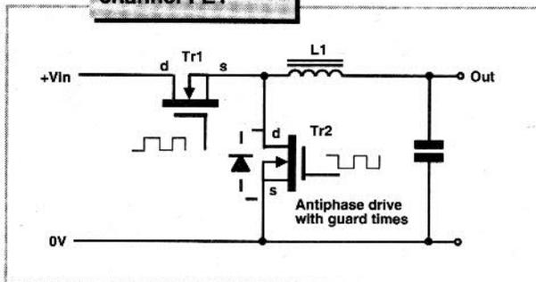
voltages in the range 10-20V, and becomes increasingly inefficient at higher voltages. At input voltages lower than 10, the on-resistance of TR1 will be slightly higher, with serious inefficiency setting in at around 6V. If a lower input voltage must be used, then a special logic level FET may be used for TR1. This type of FET is more expensive than run of the mill MOSFETs, because its processing is optimised to make it switch on fully with gate drives of less than 5V.
