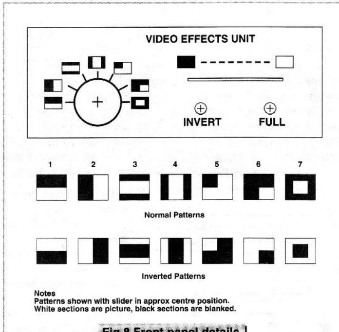
Fig.8 Front panel details
