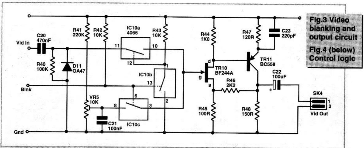
**Fig.3 Video blanking and output circuit**
