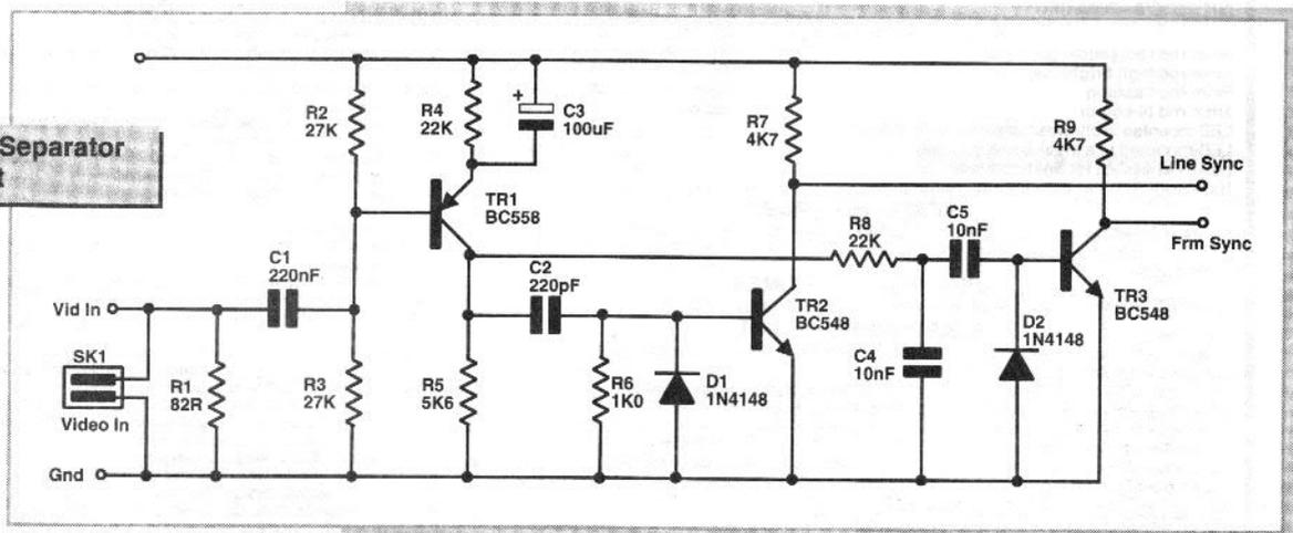
**Fig.1 Sync Separator circuit**
