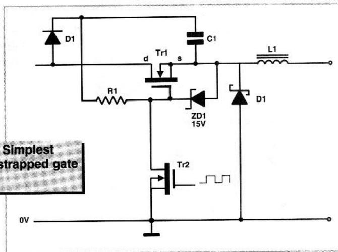
**Fig.3 Simplest bootstrapped gate drive**
