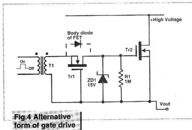
**Fig.4 Alternative form of gate drive**
