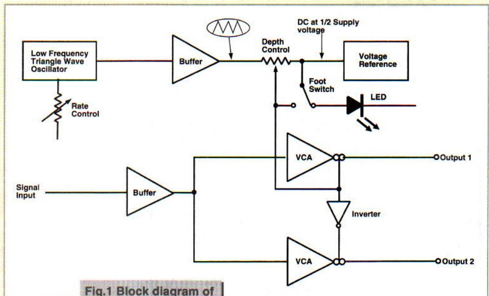
Fig.1 Block diagram of the stereo tremolo unit
