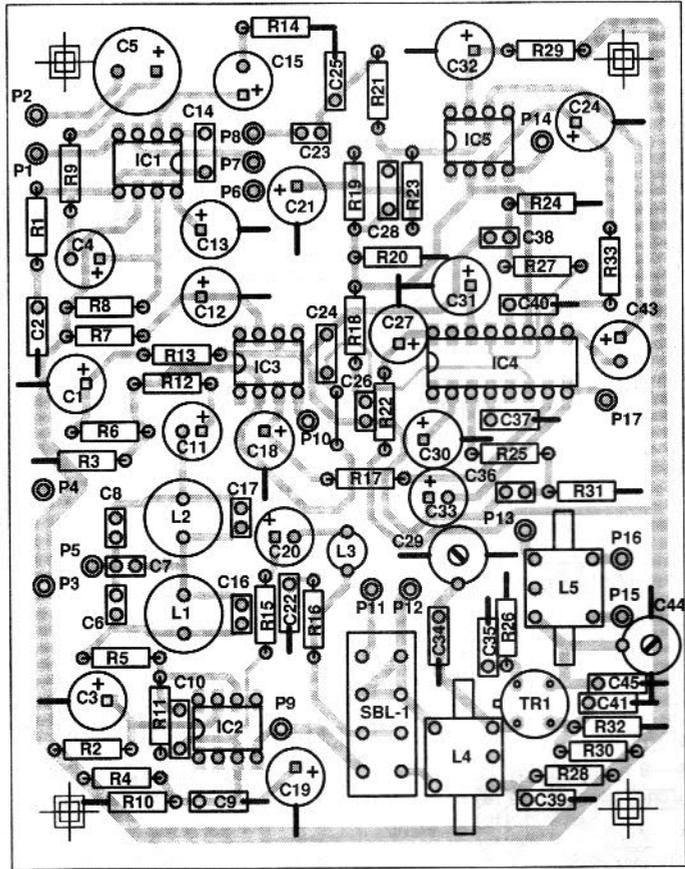
Fig.6 Main board component overlay and foil
