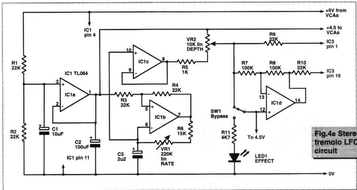
**Fig.4a Stereo tremolo LFO circuit**
