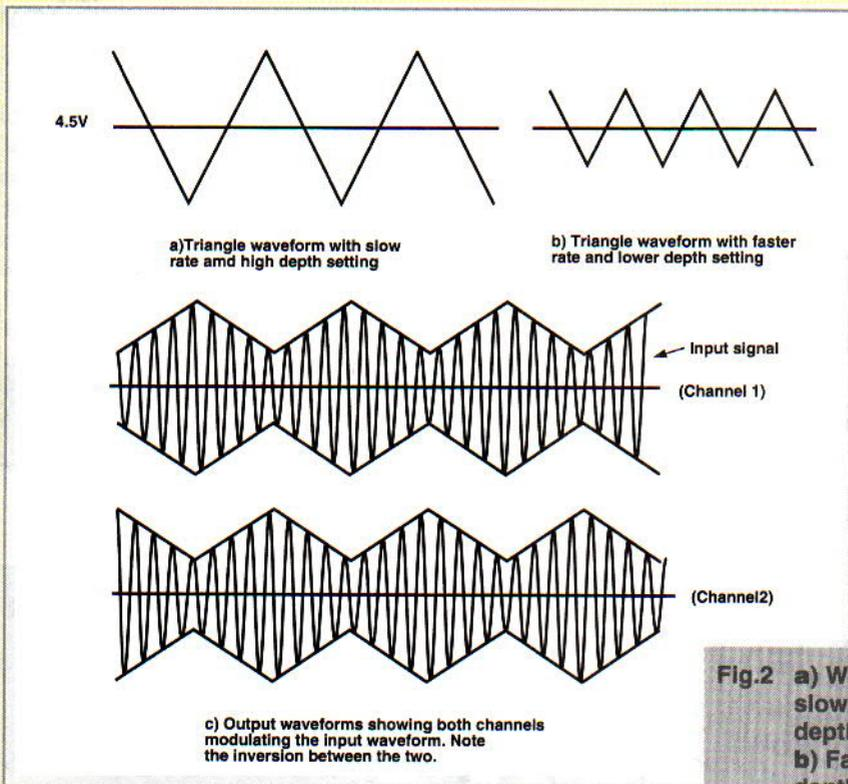
**Fig.2** a) Waveform with slow rate and high depth setting
