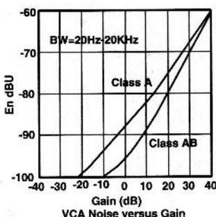
**Fig.6 Noise graph showing differences in characteristics of class A & AB operation**
