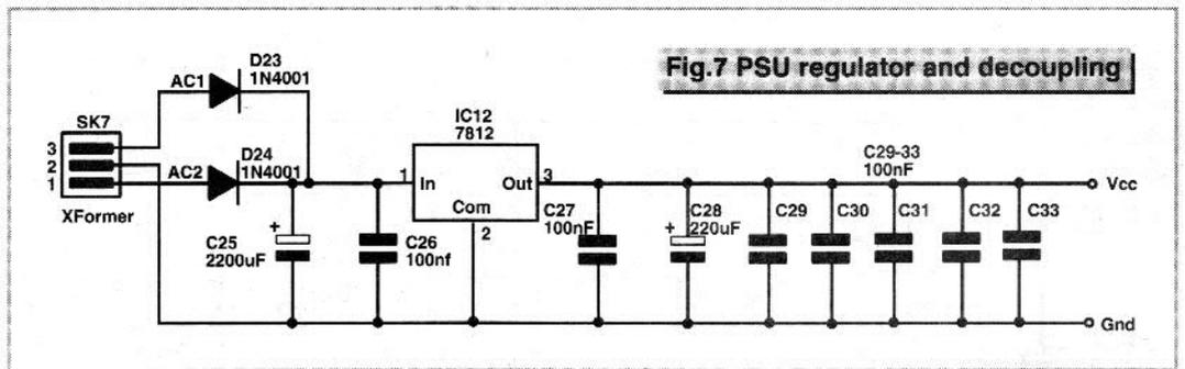
Fig.7 PSU regulator and decoupling
