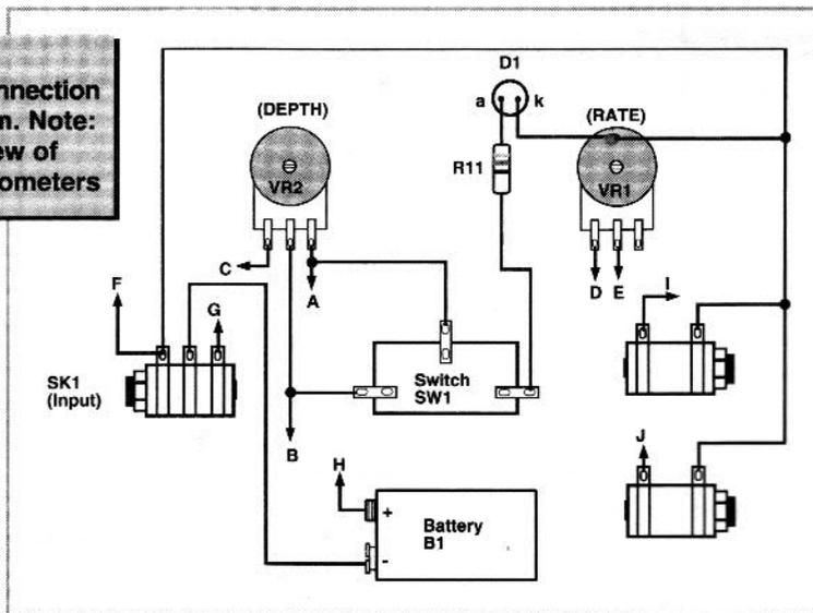
pot could be used instead, with the opposite track connection used to provide smoother rate control, albeit back-to-front. This appears to be counter-intuitive, but is worth consideration. If you only intend to use the tremolo in mono (one amplifier) then change the value of the rate pot to 100K. A 220K pot is specified to accommodate lower rates for stereo 'panning' effects, and would be worth changing to improve its 'sweep'.
