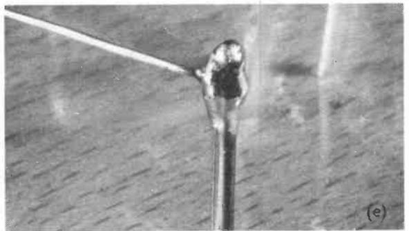
either copper, tin, gold or silver coated wires and components, and for these materials the most common solder contains 60 per cent tin and 40 per cent lead.
