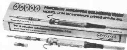
**CCN.240** New model 15 watt 240 volts miniature soldering iron with ceramic shaft to ensure perfect insulation (4,000 v A.C.). Will solder live transistors in perfect safety, fitted with 3/32" iron coated bit. Spare bits 1/8", 3/16" and 1/4" available. Can also be supplied for 220 volts. Price **£1.80**
