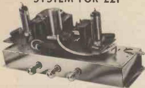
Stereo amplifier with double wound mains transformer (200-250v. a.c.); 2 x ECL82 valves giving 2 x 2½W; printed circuit (10" x 3½") mounted on metal chassis. Ganged tone controls, sep. vol. controls; on-off switch; excellent channel separation. Output trans. for 3-ohm speakers. For crystal, ceramic cartridges or radio tuner. Only £6.25 (post 40p).
