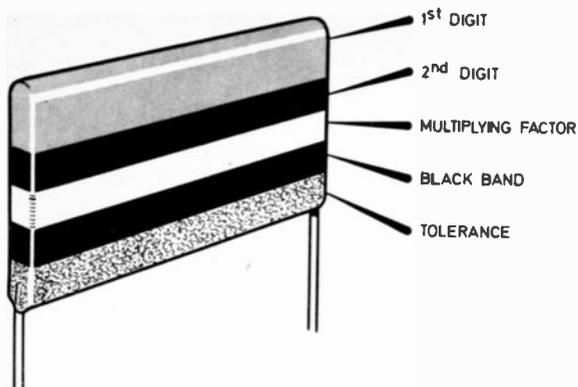
Fig. 5. An example of the capacitor colour code.
