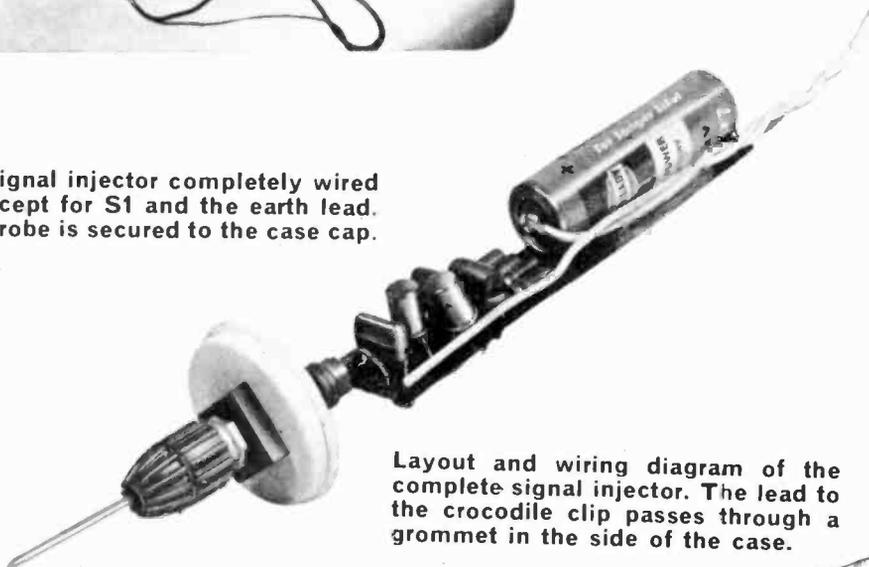
Layout and wiring diagram of the complete signal injector. The lead to the crocodile clip passes through a grommet in the side of the case.
