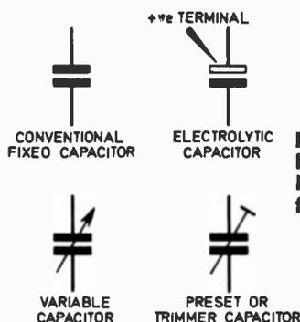
Fig. 3. Circuit symbols used for different kinds of capacitors fixed and variable.
