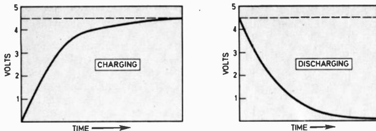
Fig. 7. Typical charge and discharge curves for a capacitor. Similar curves should be obtained from the results of experiment 1.
