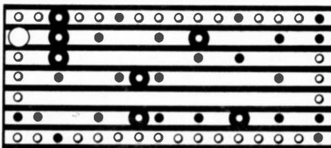
Compare the photograph with the drawing and identify the strips of copper, soldered connections and breaks in the strips.
