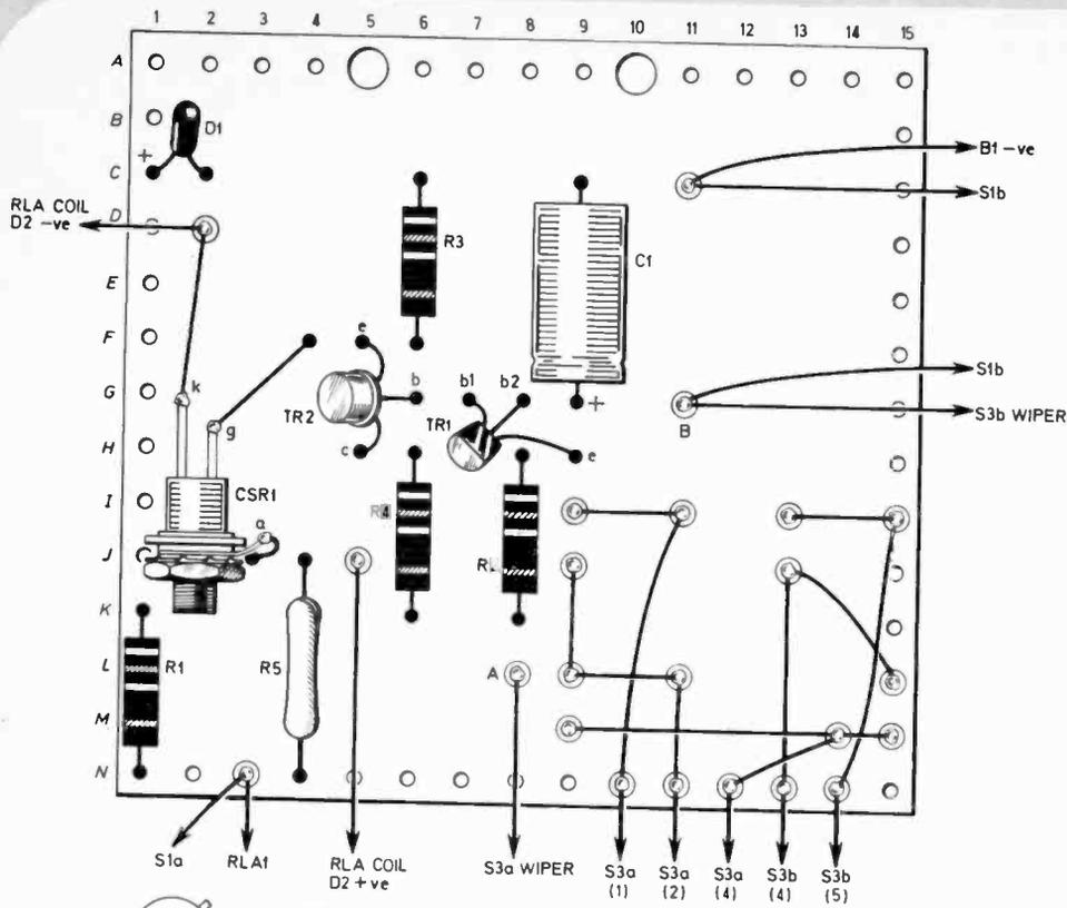
Fig. 3. Layout and wiring of the components mounted on the board. The preset potentiometers are mounted on the underside of the board (shown below) so that they can easily be adjusted.
