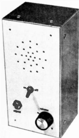
Fig. 5. A completed case of a small amplifier showing holes drilled for loudspeaker
