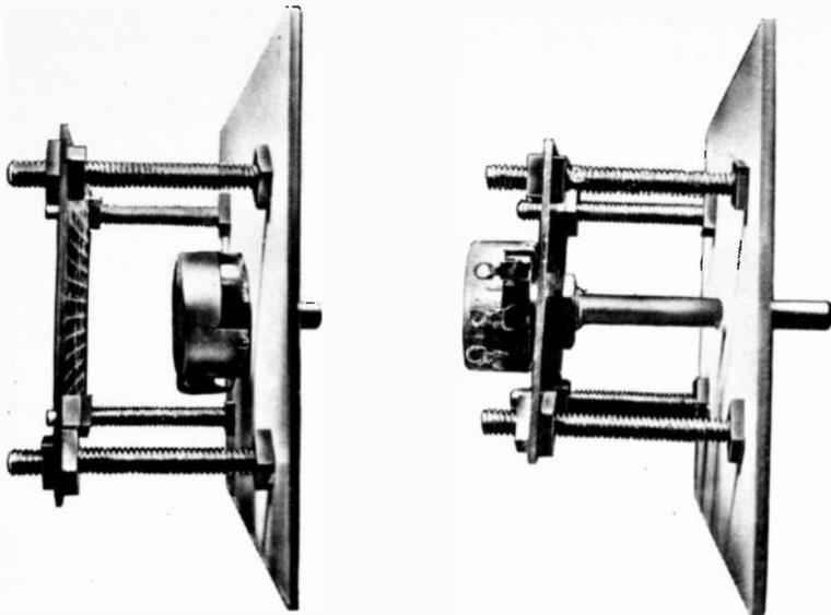
Fig. 3 (a) (left) Fixing the potentiometer to the front panel if there is not enough space on the component board.
