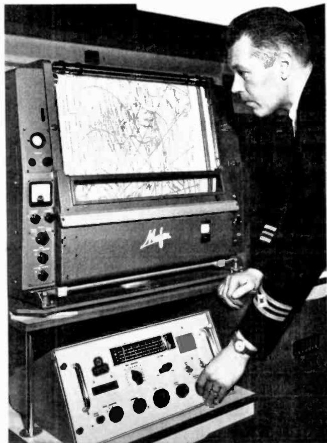
South Poles, and broadcasting signals which announce their position every two minutes. The special shipborne observation equipment comprises a receiver, a data handler and a teleprinter. The system operates by measuring the Doppler effect variations in the broadcast frequency received from each satellite as it passes, but the shipboard installation is costly and cumbersome and the system is at present in use on only one or two high-prestige ships.
