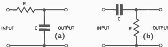
Fig. 9 (a) Integrator and (b) differentiator circuits.
