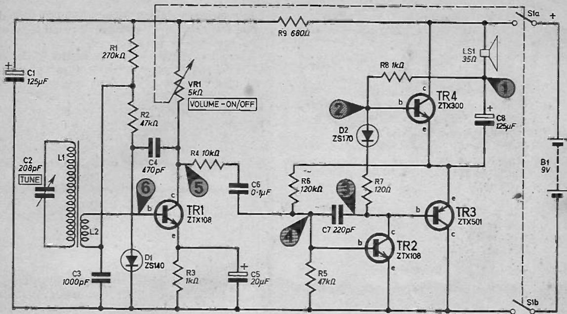
Fig. 4 The circuit diagram of the Astron receiver with the test points indicated for fault location and checks.
