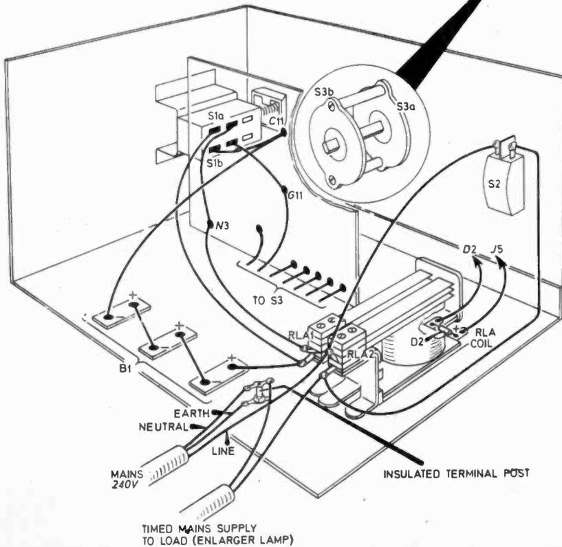
Fig. 4. Layout and wiring of the components mounted in the case; the board has been cut away to show S3 and S1. The board is held by a bracket fixed to S1. Switch S3 has also been shown separately, as it would appear when dismantled, for clarity. The batteries are not shown but their clips are wired up in the approximate positions of the batteries.
