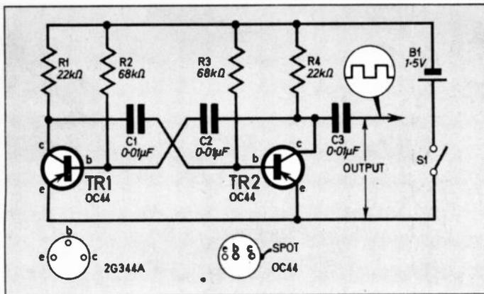
Fig. 1. The complete circuit diagram of the signal injector. Output is taken from the collector of TR2, and is a "square" wave of basic frequency 11kHz.
