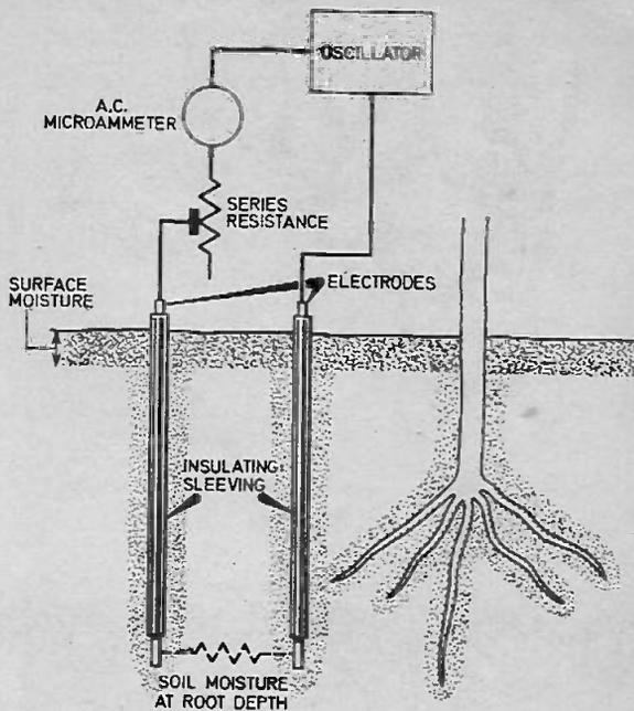
Fig. 1. Basic arrangement of the moisture meter.
