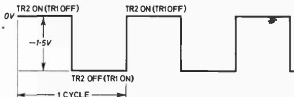
Fig. 2. The waveshape obtained at the output. This is made up from periods of TR2 conducting and non-conducting, the resultant effect being a square wave. A similar wave form is available at the collector of TR1.
