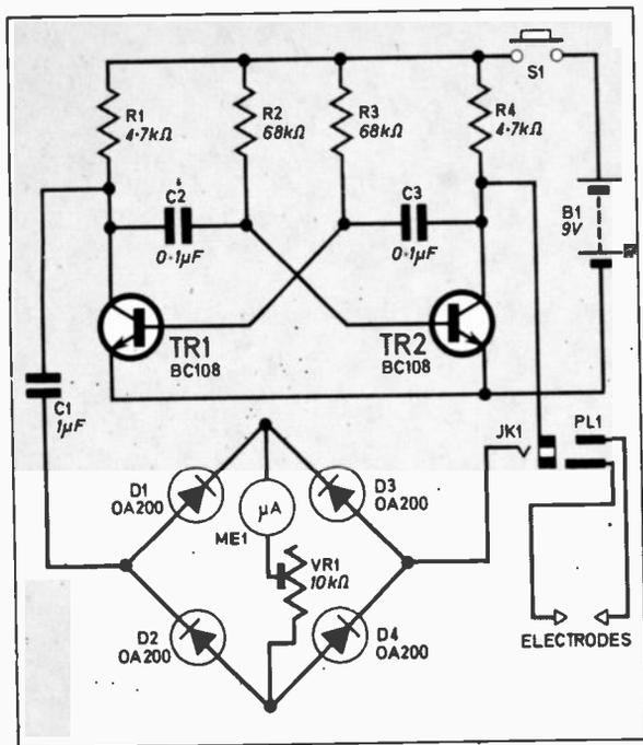
Fig. 2. Complete circuit diagram of the soil moisture meter.
