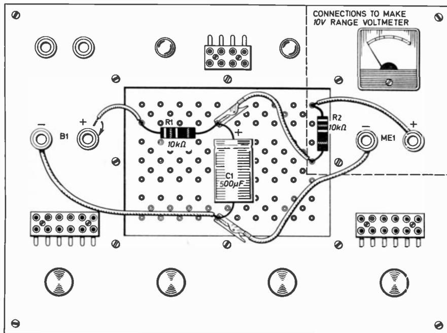
Fig. 6(a) (above). The circuit diagram for experiment 1.
