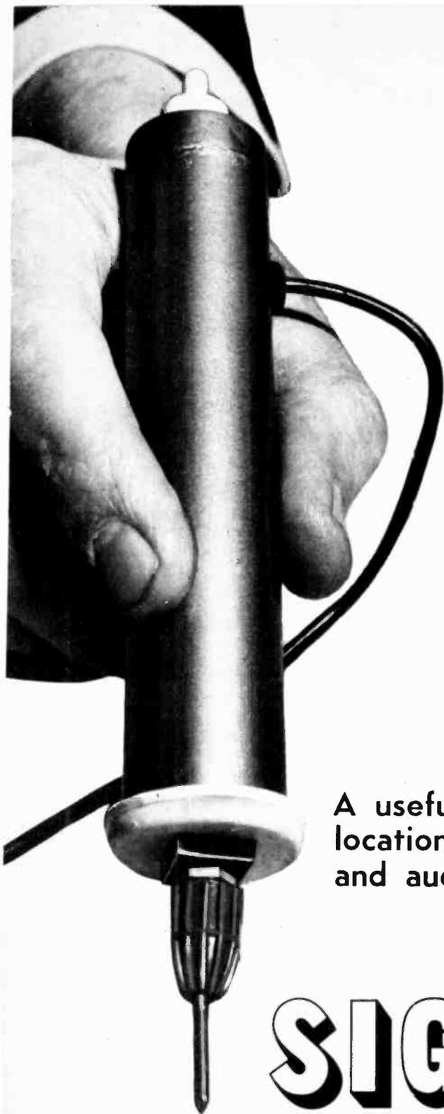
**A**LTHOUGH only a simple instrument in the field of radio servicing, the pocket signal injector is a most valuable and handy tool for both the amateur and professional.
