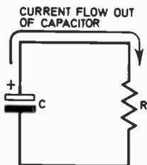
Fig. 2. Capacitor discharging through a resistor.
