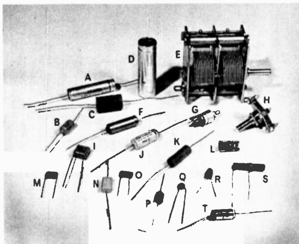
Fig. 4. Shown above is a variety of common capacitor types: A paper; B polyester; C tubular metallised polyester; D electrolytic can-type; E ganged variable; F electrolytic; G beehive trimmer (concentric); H variable; I metallised polyester; J paper dielectric; K tubular mixed dielectric; L trimmer (compression); M and N metallised polyester; O silver mica (printed circuit type), P silver mica; Q disc ceramic; R tantalum; S high voltage (pulse) ceramic; T polystyrene.
