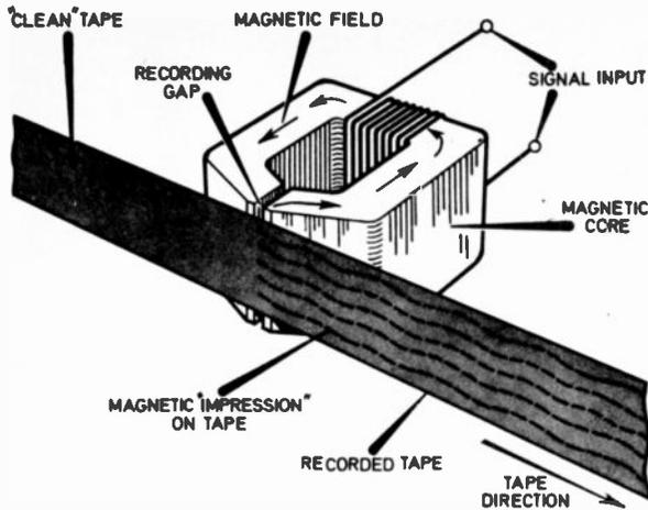
**Fig. 1. The basic method of creating a magnetic field on a recording tape.**
