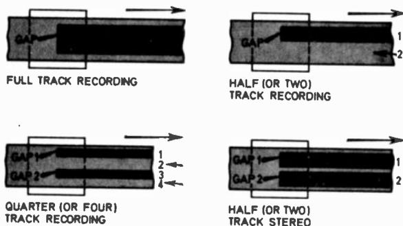
**Fig. 6. Various track arrangements.** In the four track system gap 1 records tracks 1 and 4, and gap 2 records tracks 2 and 3.
