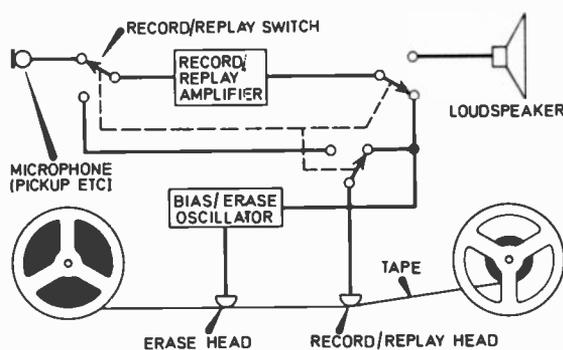
**Fig. 4. Block diagrams of two basic tape recorder systems. Left—the system using separate record and replay heads. Right—the system using a single record/replay head.**
