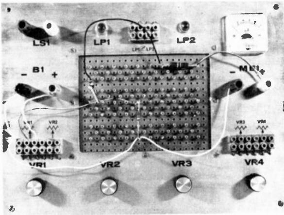
Photograph of the Demo Deck in use for measuring the characteristics of the IN4148 (silicon) diode.
