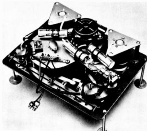
**The underside view of a Brenell tape deck.** This deck used three separate motors, one synchronous type for the capstan and the other two to drive each spool.
