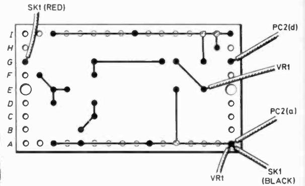
Fig. 2. (Above) Layout and wiring of the component mounting board.
