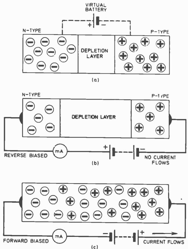
impurity atom added—this is known as “doping.” These extra electrons will be free to move about thus increasing the electrical conductivity. By “adding” electrons in this manner we say we are introducing “negative carriers” (of current) and the resultant material is called an “n-type” semiconductor.
