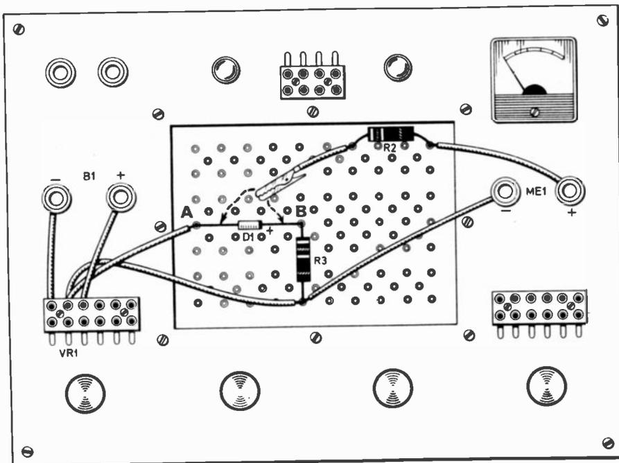
**Fig. 4(b) (left).** The circuit of Fig. 4(a) wired up on the Demo Deck.
