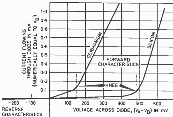
**Fig. 5. Forward and reverse characteristics for the OA91 (germanium) and IN4148 (silicon) diodes obtained using circuit of Fig. 4(a). The two curves would eventually become parallel straight lines if we were able to plot the characteristics to a higher voltage.**
