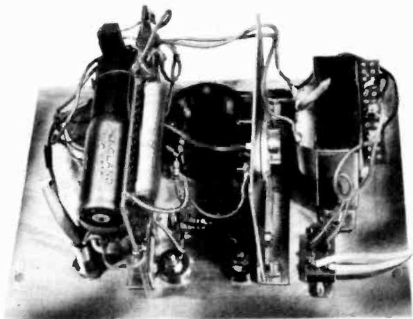
Fig. 5. Shows the positioning of all the components in the aluminium case and the flying lead connections to the component board. Ensure that TR1 is fully insulated from the heatsink by using a mica washer and plastic bushes.
