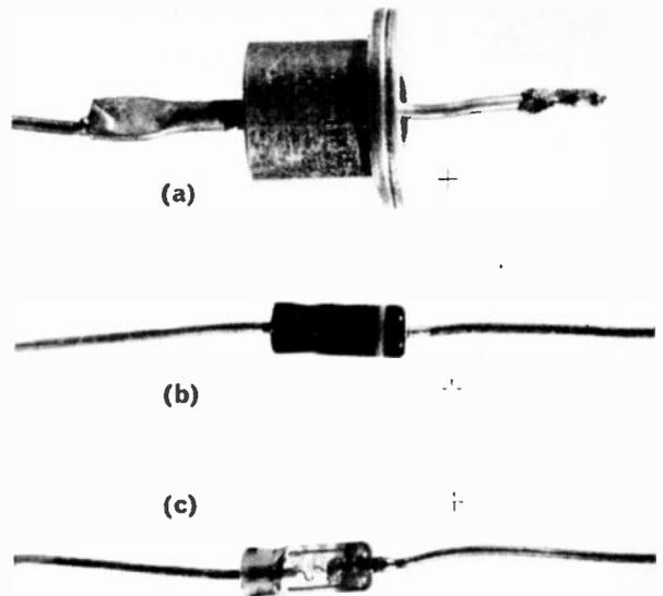
Three common diodes: (a) medium power rectifier, BY100 silicon (b) signal diode IN4148 silicon (c) signal diode OA91, glass encapsulated point-contact germanium (Magnified x 2½).
