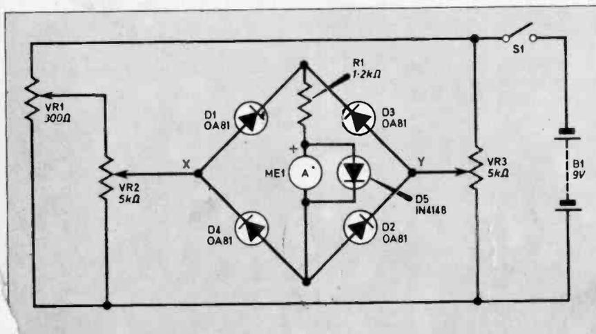
Fig. 1. Complete circuit diagram of the Simple Calculator.
