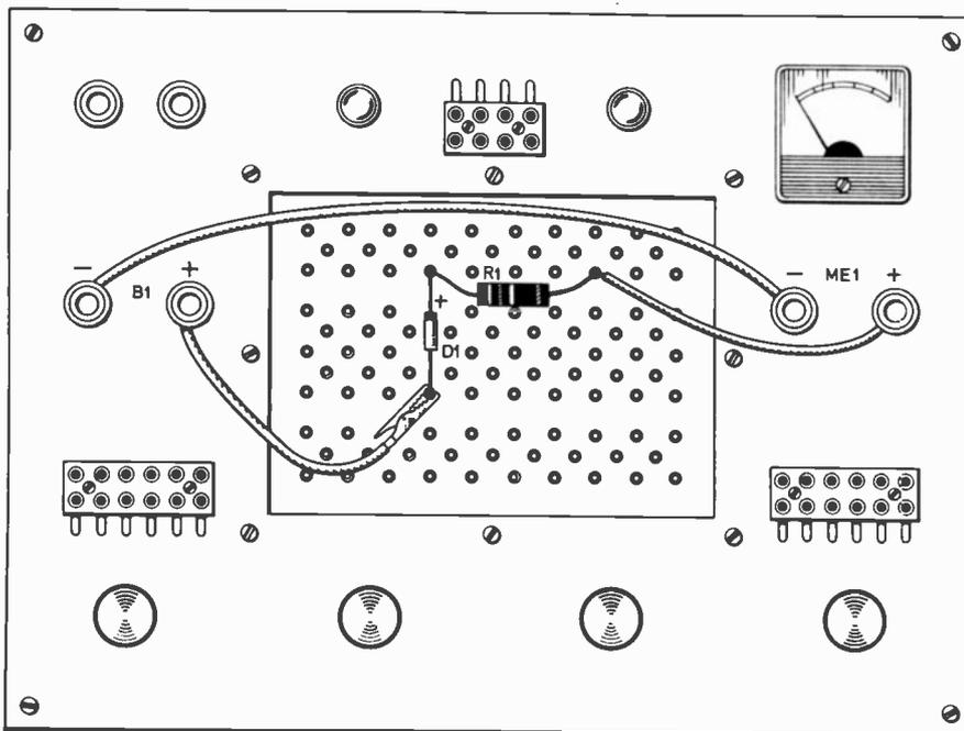
Fig. 3(a) (above). The circuit diagram for polarity test and demonstrating current flow in one direction only.
