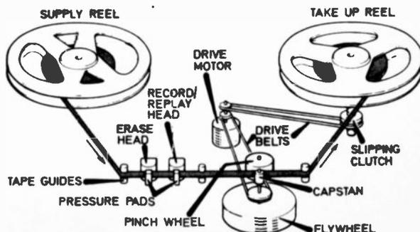
hindered passage of tape in either direction at fast speed. The mechanism lifting the tape clear of the heads also serves to protect the heads. The rate of wear under rewind conditions would soon render the heads useless.
