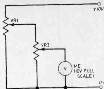
Fig. 2. Theoretical circuit to show the basic operation of the Simple Calculator.
