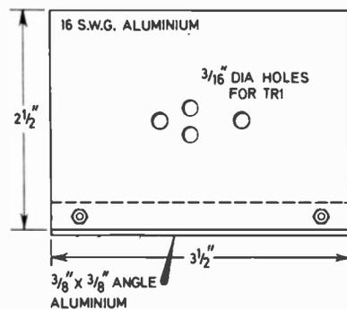
Fig. 3. (above) The dimensions of the heatsink for TR1.
