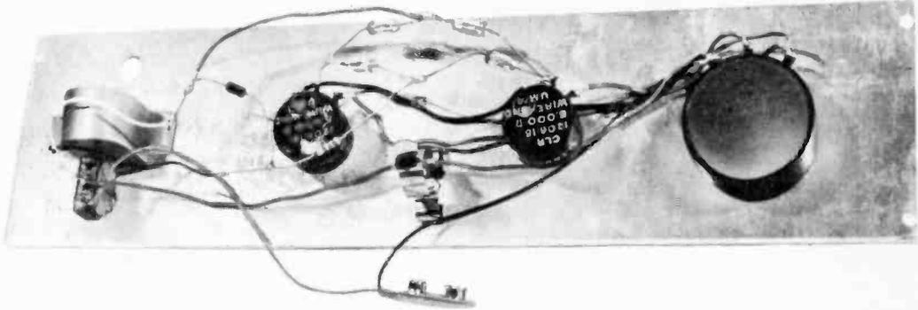
Fig. 3. Layout and wiring of the Simple Calculator. Battery B1 is mounted in a Terry clip fixed to the front panel.
