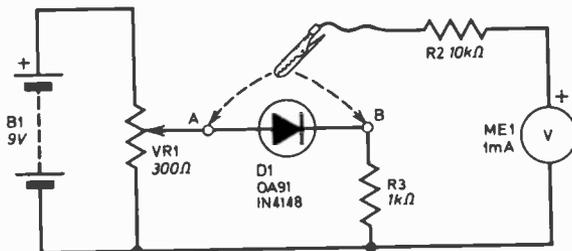
**Fig. 4(a) (above).** The circuit diagram for measuring the diode characteristics.
