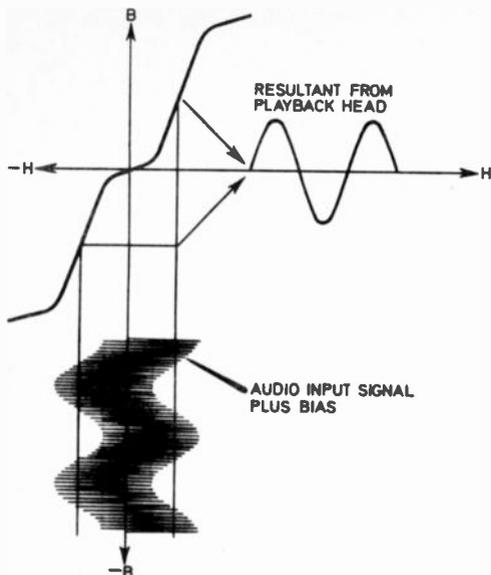
Fig. 3. High frequency bias recording system.
