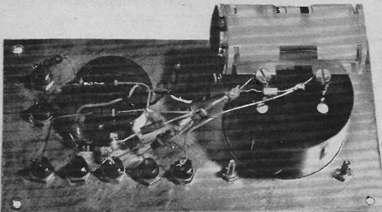
Photograph of the complete multimeter showing the construction.
