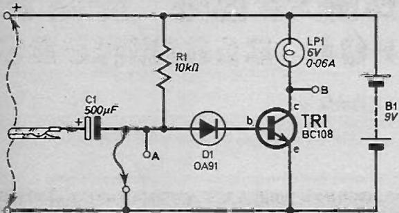
Fig. 2(a) (above). The circuit diagram to illustrate the switching action of a transistor.
