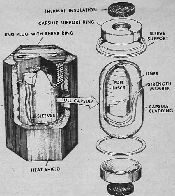
Cutaway view of the plutonium 238 fuel capsule of the SNAP 19 radioisotope thermoelectric generator (atomic battery). Four of these Atomic Energy Commission-developed generators provide a total of 120 watts of electrical power in the Pioneer 10.
