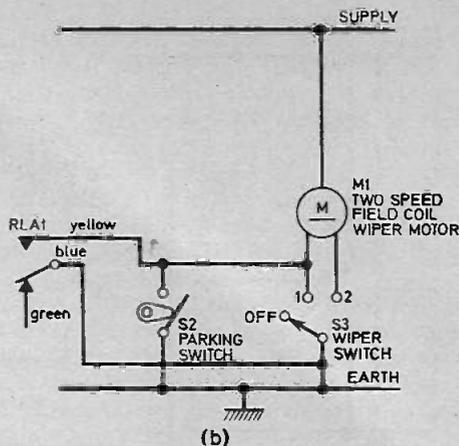
Fig. 4b. Method of connecting the controller to the circuit of Fig. 4a.
