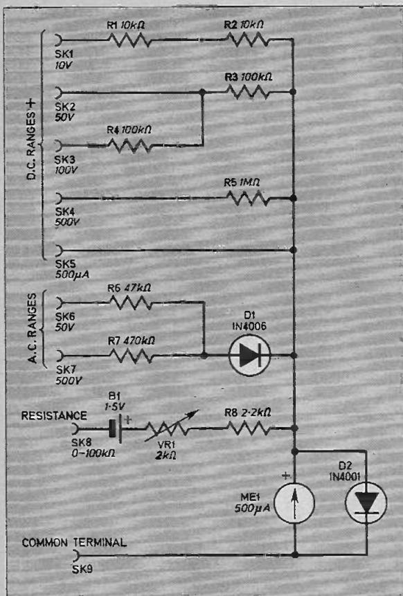
Fig. 1. Circuit diagram of the complete multi-meter using the  $500\mu\text{A}$  meter movement. For the more sensitive design Table 1 gives alternative resistor values.
