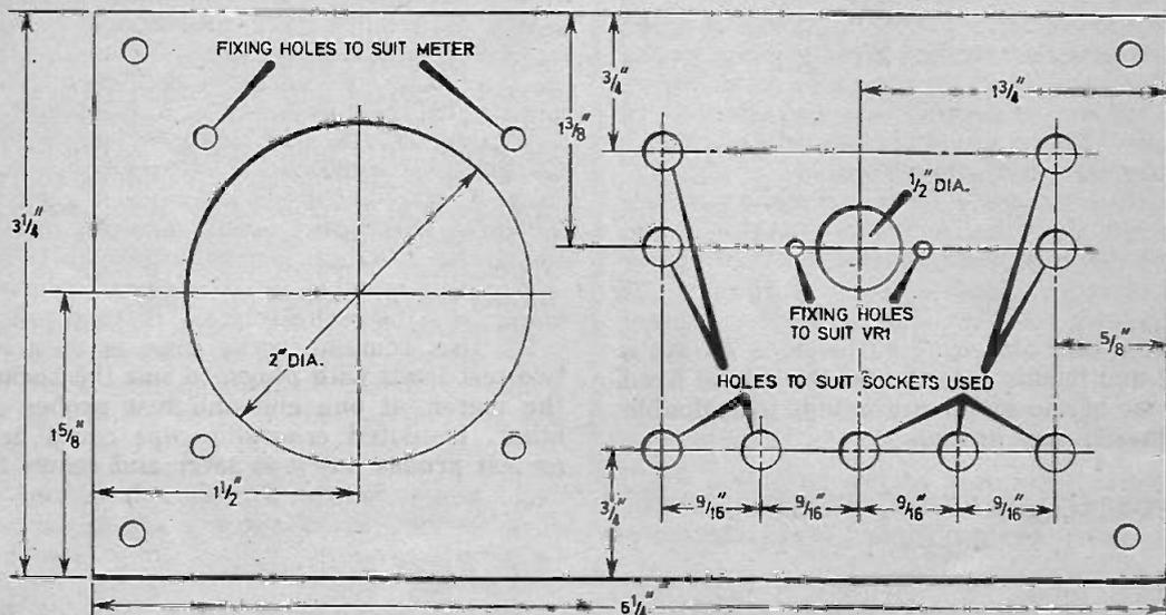
Fig. 2. Layout and drilling details of the Multimeter front panel. A larger panel would be required for larger type meters.
