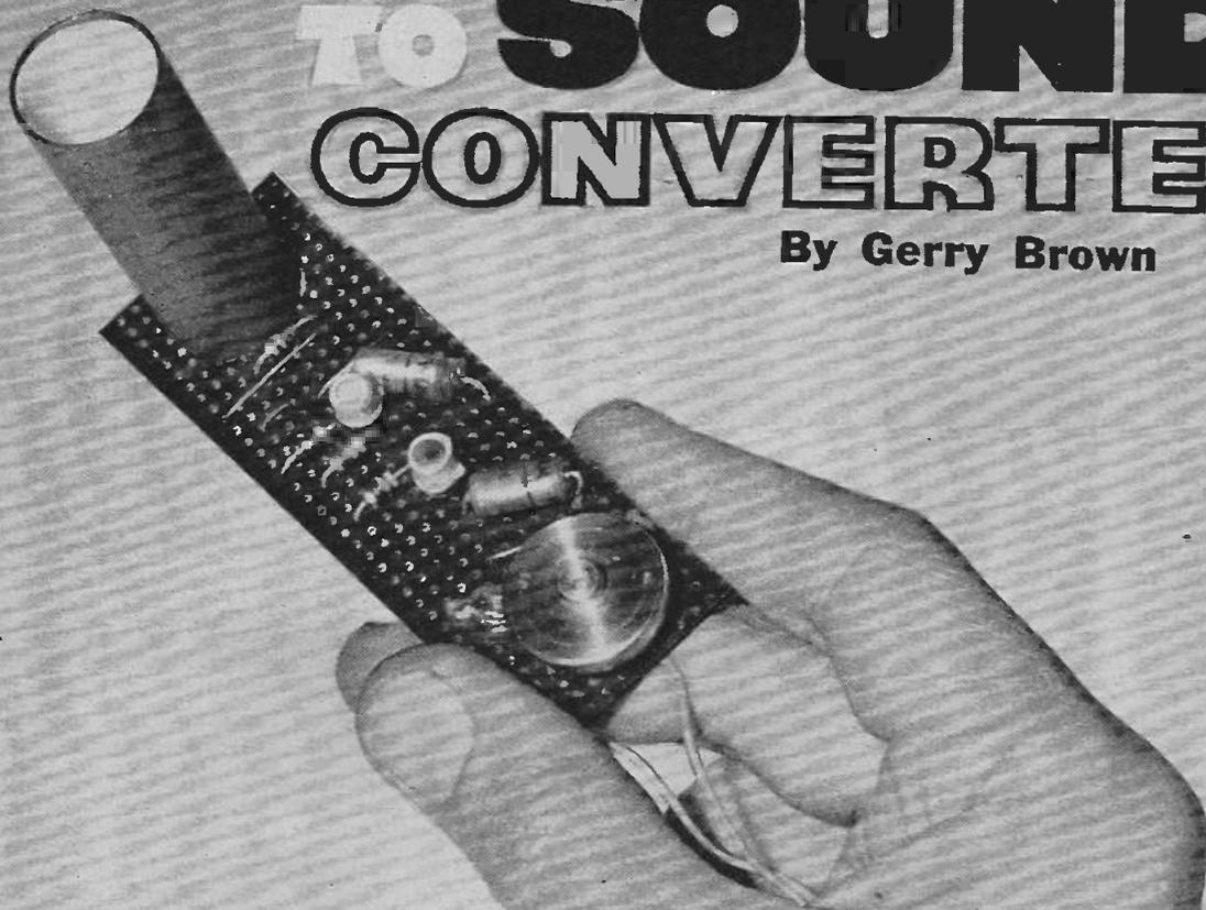
**An experimental device providing an audio output, the frequency of which depends on the light falling on a light dependent resistor.**
