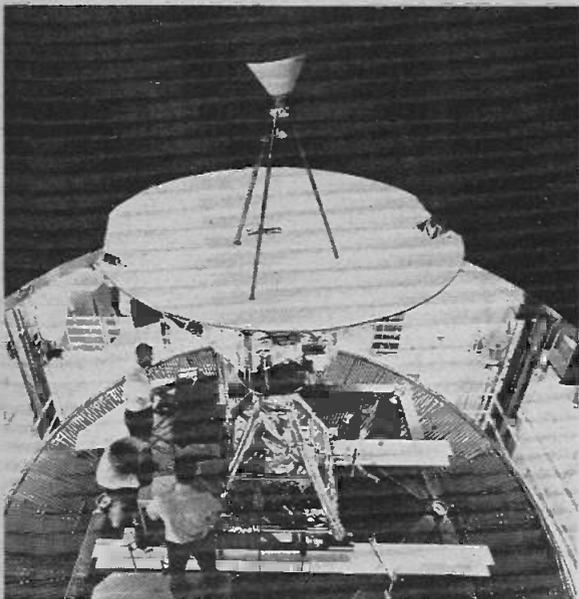
Before launch Pioneer 10 was tested in a simulation chamber which reproduced the conditions of heat, cold, vacuum and radiation expected on the flight to Jupiter and beyond.
