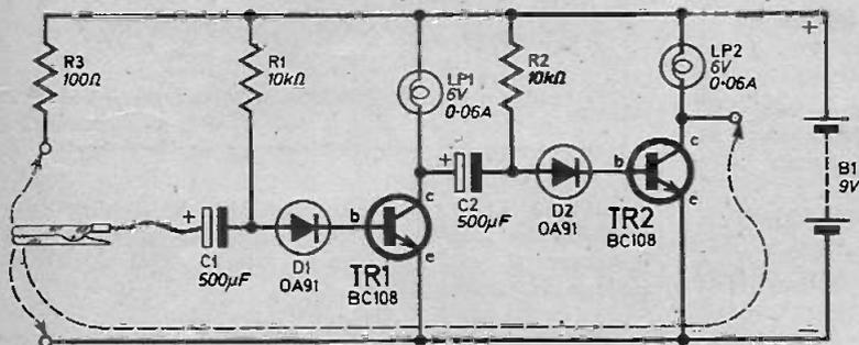
Fig. 4(a) (left). The basis of the astable multivibrator. When the positive end of  $C_1$  is connected to  $TR_2$  collector, the circuit operates automatically.
