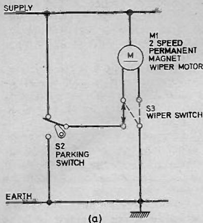
Fig. 6a. Circuit of a 2 speed permanent magnet wiper motor.
