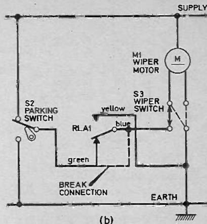
Fig. 6b. Method of connecting the controller to the circuit of Fig. 6a.
