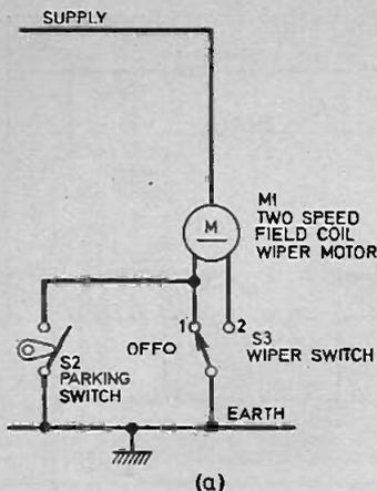
Fig. 4a. Wiring diagram of a 2 speed field coil wiper motor.
