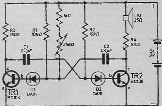
Fig. 5(a) (above). The astable multivibrator circuit for producing an audible output. To produce a variable tone, replace R1 by the dotted combination.
