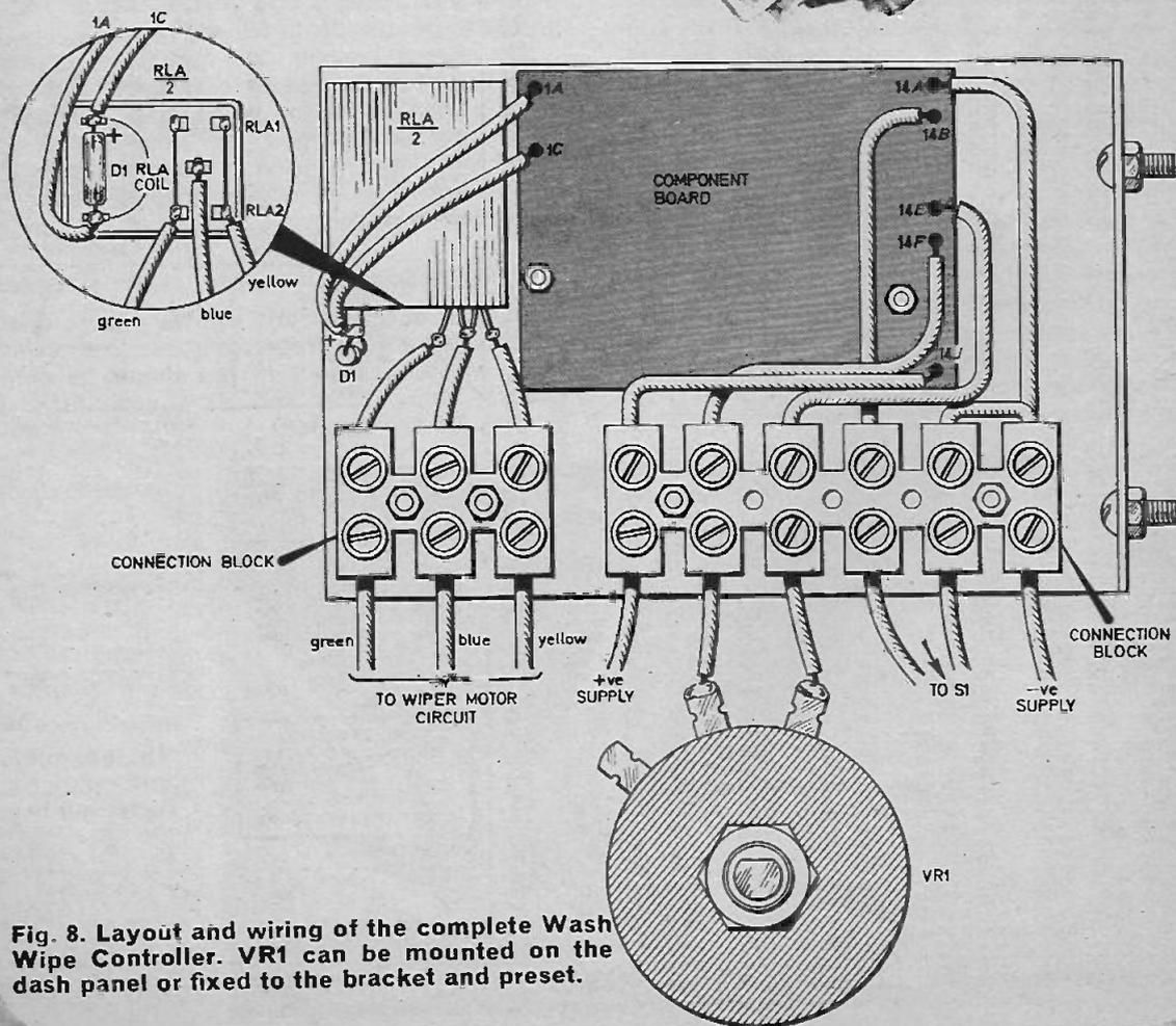
Fig. 8. Layout and wiring of the complete Wash Wipe Controller. VR1 can be mounted on the dash panel or fixed to the bracket and preset.
