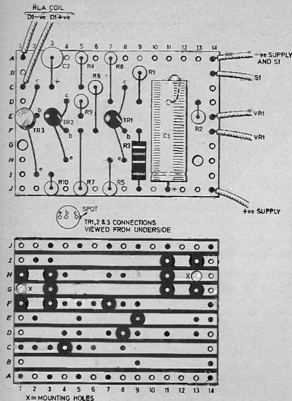
**Fig. 7. Construction of the circuit board for the Wash Wipe Control.**
