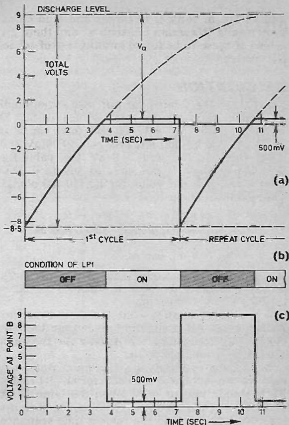
Fig. 3. (a) The graph obtained by plotting voltage at point A against time. (b) The state of LP1 with time. (c) The output voltage at point B of Fig. 2(a).
