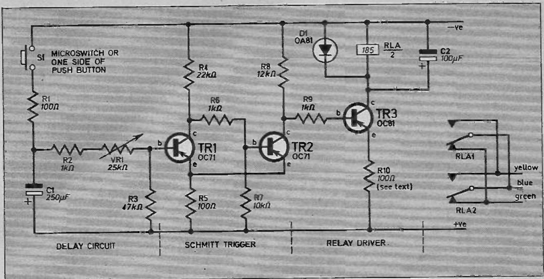
Fig. 1. Complete circuit diagram of the Wash Wipe Control. R10 is removed for 6V operation.
