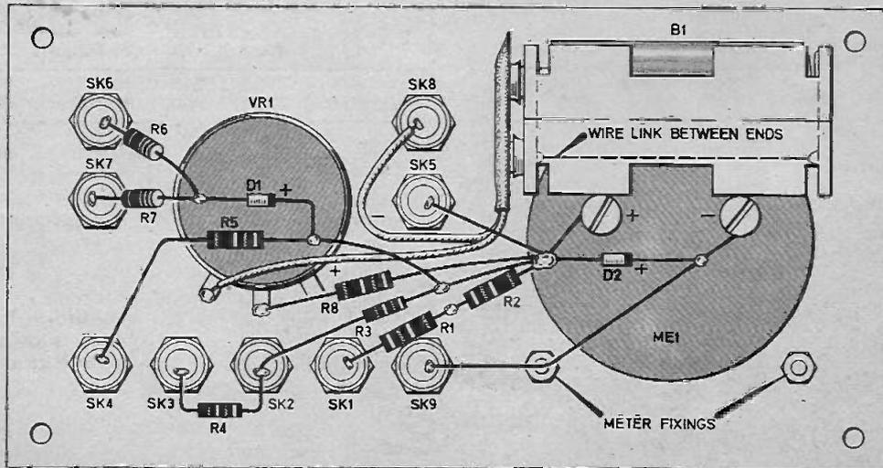
Fig. 3. Layout and wiring of the complete Multimeter. Note the wire link on the battery holder.
