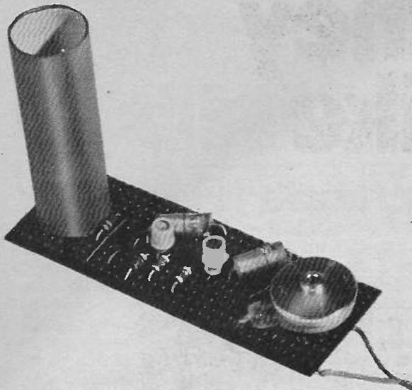
Photograph showing the prototype unit with a simple light shield.
