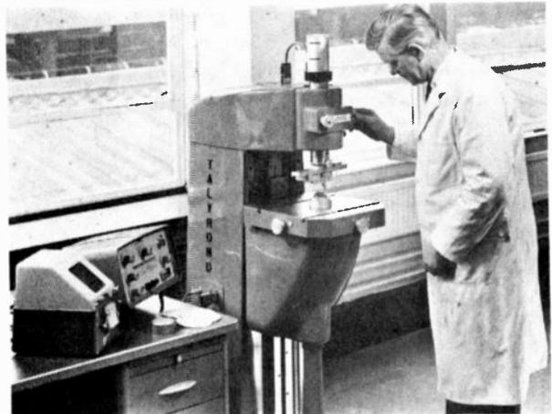
Checking the finish of a lens with the Talyrond 73 roundness measuring system. This system which can detect surface irregularities of the order of one millionth of an inch, uses a special purpose computer to correct for inaccuracies in work positioning etc. Defects of the work piece are recorded on a rotating chart. (Rank Precision Industries Ltd.)
