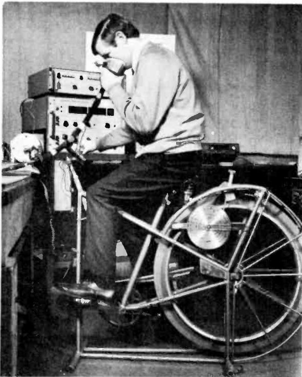
Using a Transfer Function Analyser to determine the relationship between respiration and work done by humans. (Solartron Electronic Group Ltd)
