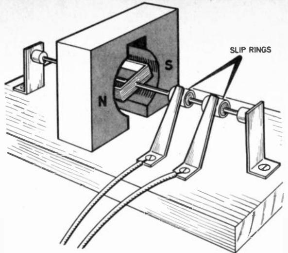
**Fig. 5.6. Simple two-pole alternator.**
