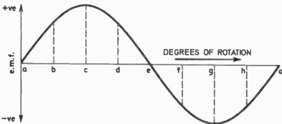
**Fig. 5.5. Graphic display of generated e.m.f. as a function of rotation angle.**
