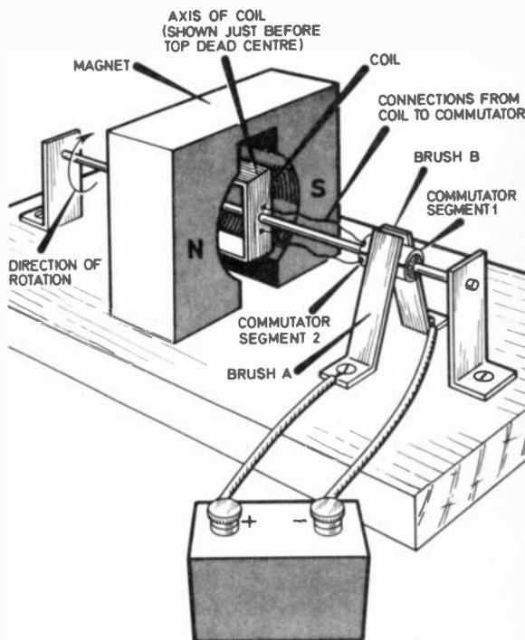
Fig. 5.1. A simple two-pole permanent magnet motor.
