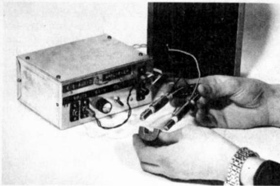
**Fig. 5.4. Experiment to demonstrate electromagnetic induction.**
