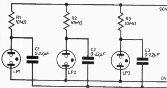
Fig. 2. Modified circuit for random flashing.
