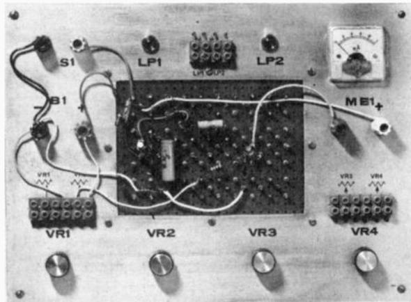
To get *any* indication on ME1 means that the voltage fed to the base of TR2 must be exceeding the 600mV base emitter forward voltage drop. When measured on proper test equipment the a.c. signal at the collector of TR1 is in the order of 1.5V,—thus bearing out that we are getting very high voltage amplification (between 600 and 700 as calculated).
