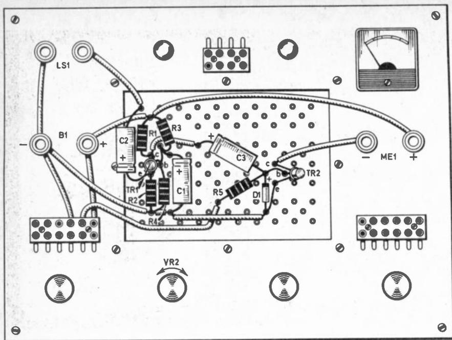
Fig. 4.3. The circuit of Fig. 4.2. Wired up on the Demo Deck. VR2 should be adjusted as mentioned in the text.
