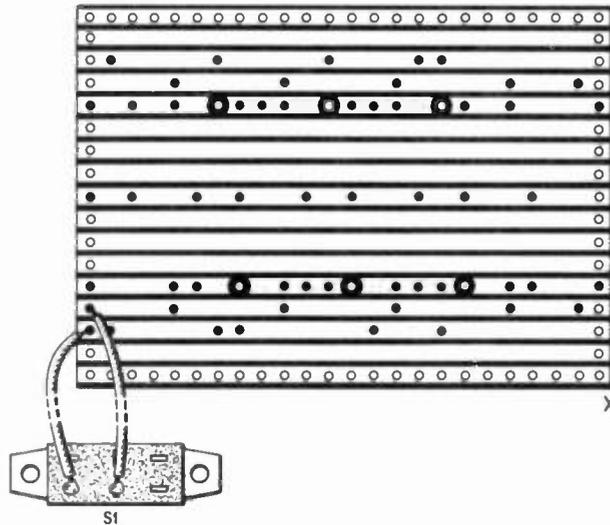
Fit the resistors, capacitors, the neon wires and the battery wires to the connector strip exactly as shown in the illustration (Fig. 3). Check carefully that all the connections are correct then push the plug into the battery. The neons should commence to flash.
