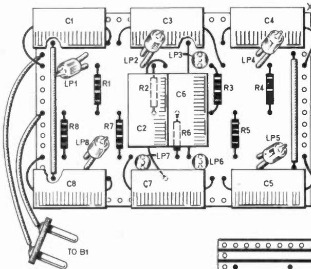
Fig. 4. Layout and wiring of the Vero-board for the 8 neon unit. The underside is shown below with cut aways and S1 wiring. To orientate the lower drawing find corner X on both views.
