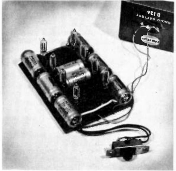
Photograph showing the completed circuit board and battery for an 8 neon "flashing block" unit.
