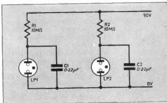
Fig. 1. Basic circuit diagram of Neon Novelty.
