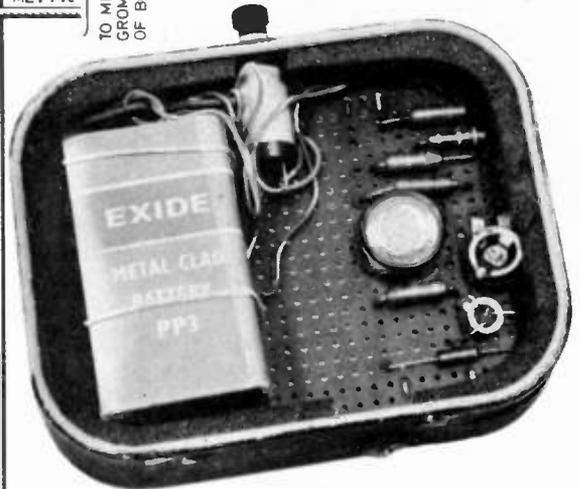
The completed sensor box with lid removed (above).
