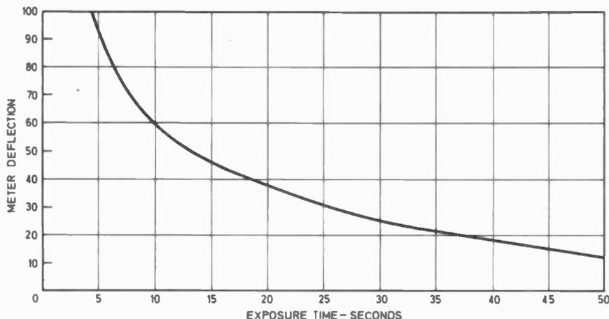
Fig. 4. Calibration curve for the prototype unit. A curve like this must be made for the meter.
