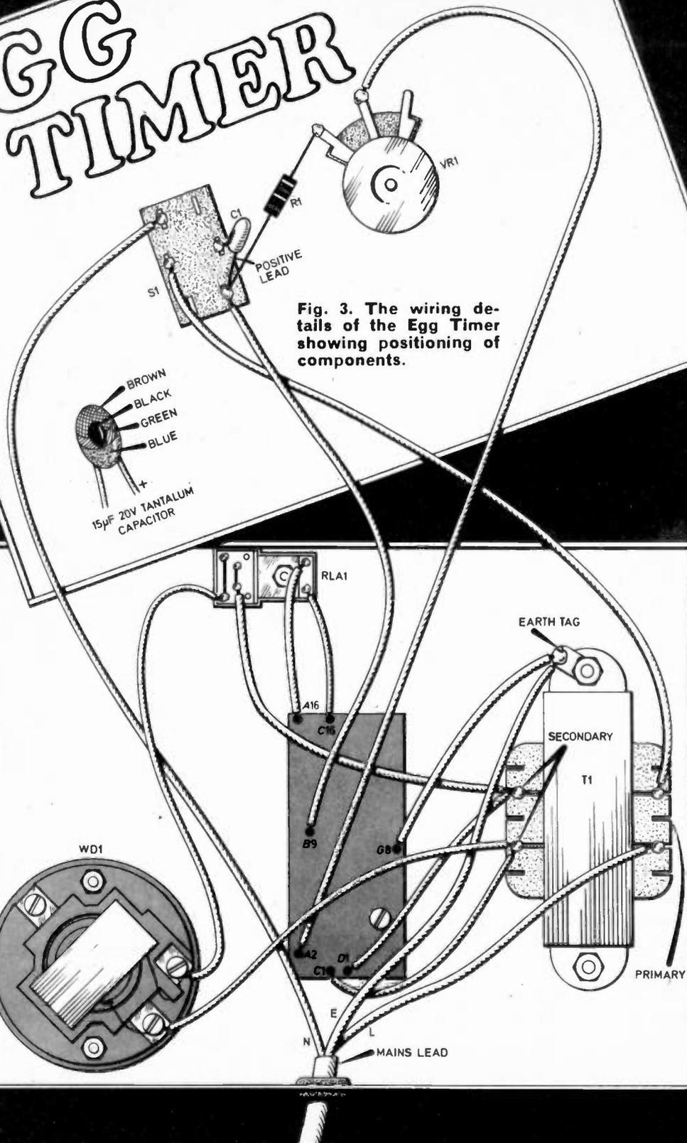
Fig. 3. The wiring details of the Egg Timer showing positioning of components.
