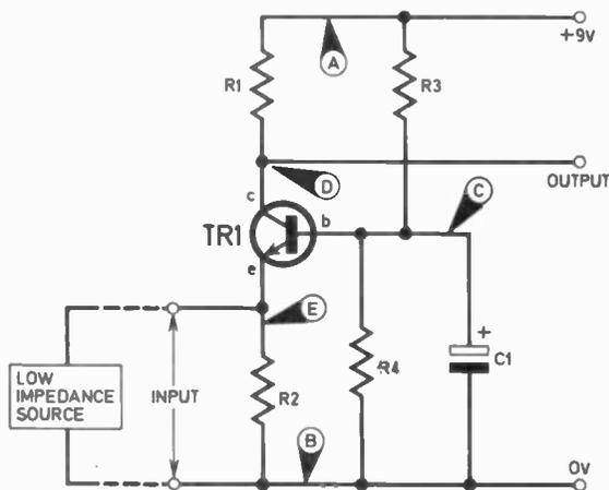
Fig. 4.1. Basic circuit of a grounded base stage.
