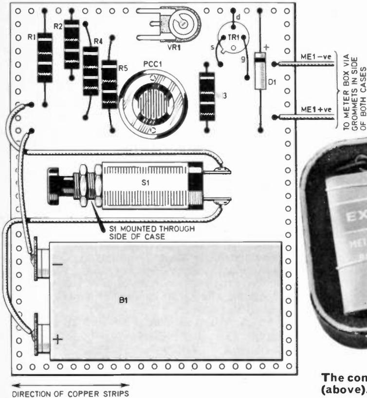
Fig. 3. Layout and wiring of the components mounted on the Veroboard. There are no breaks in the copper strips on the underside.
