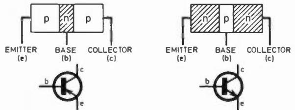
Fig. 2. Alternative arrangements of the junction transistor.
