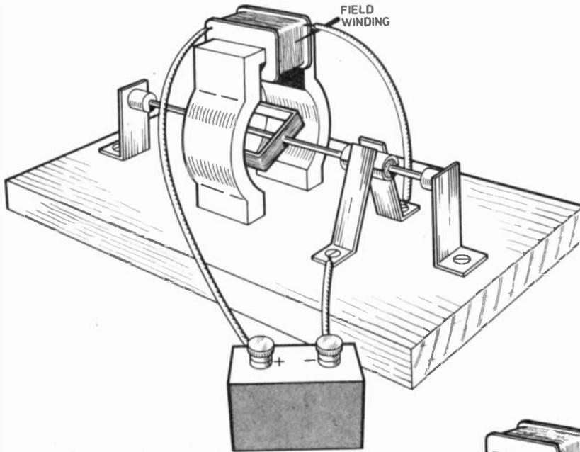
Fig. 5.3 (left). Shows a simple two-pole electromagnetic motor with series connected field winding. Below shows the parallel or shunt connection.
