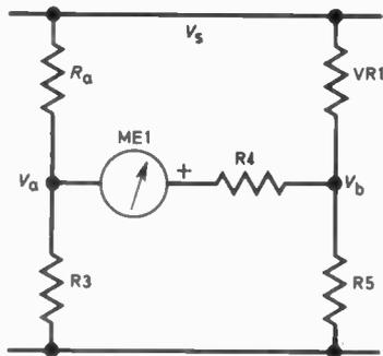
Fig. 1. Basic bridge circuit configuration.
