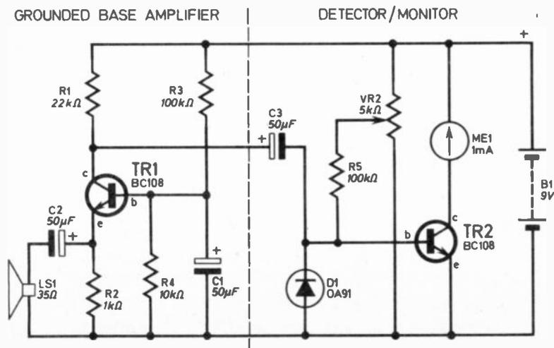
Fig. 4.2. "Working" circuit for the grounded base stage together with a simple monitoring stage.
