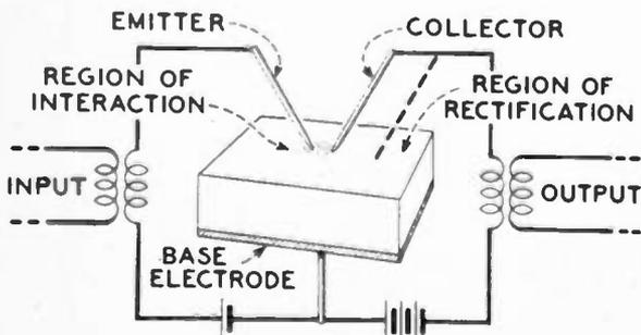
Fig. 1. The basis of the first transistor.
