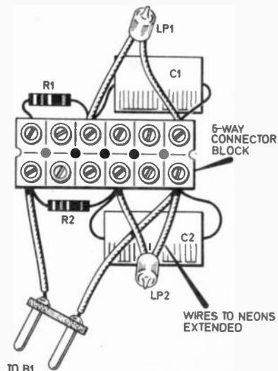
Fig. 3. Wiring for the two neon circuit.
