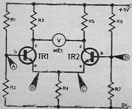
biased in exactly the same way as TR1 and if  $h_{FE}$  and the forward base/emitter drop are the same in both cases and identical biasing resistors are used, the quiescent potential at TR2's collector will be the same as at TR1 collector. Assuming both transistors are operating independently with separate emitter resistors a voltmeter (ME1) connected between the collectors would show a voltage difference of zero.
