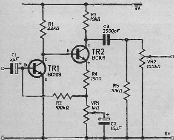
Fig. 1. The circuit diagram of the Beta Fuzz to be put on to the printed circuit board.
