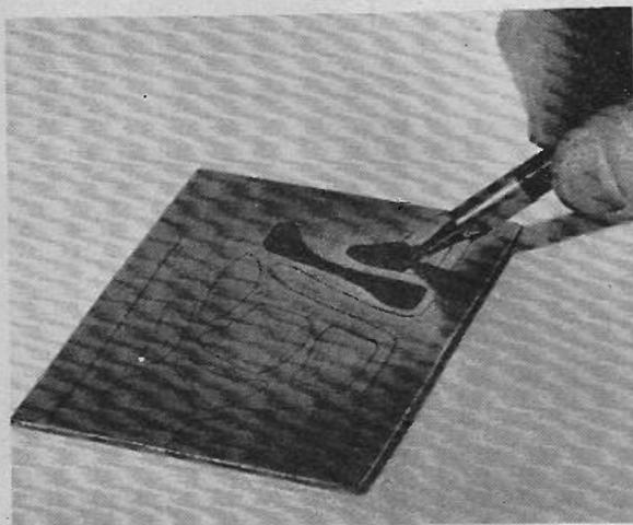
**B.** Using a printed circuit marker pen to fill in the areas of copper to remain after etching.
