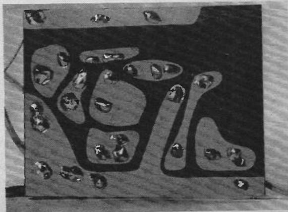
**F.** The underside of the completed board.
