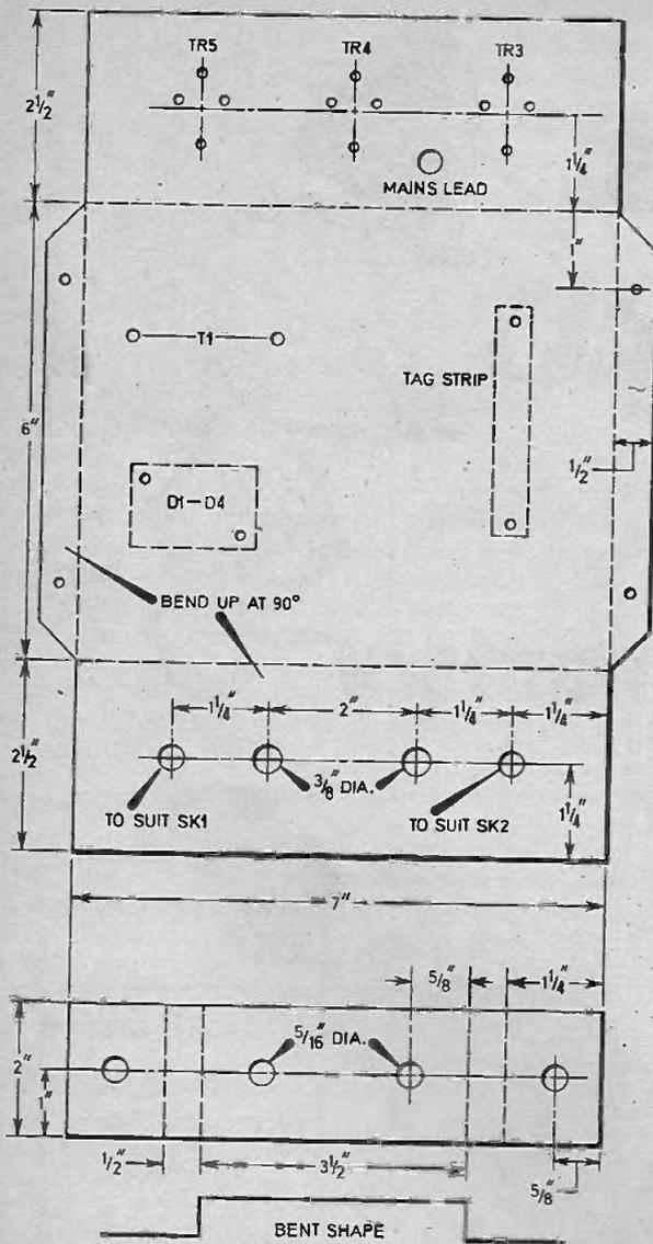
Fig. 4. Case construction details.
