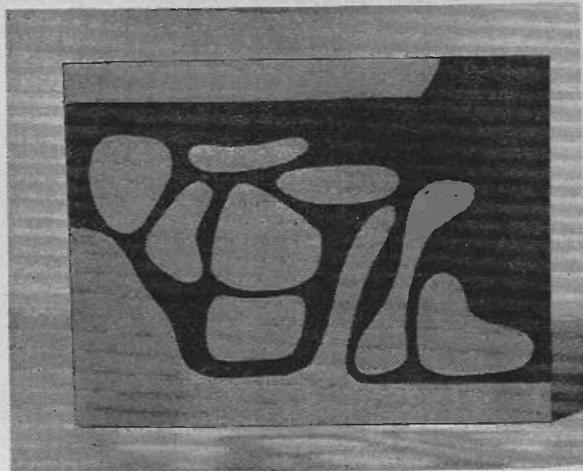
**D.** The board after etching with resist cleaned off.
