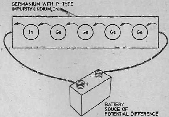
Fig. 1.2. Conduction in p-type germanium.
