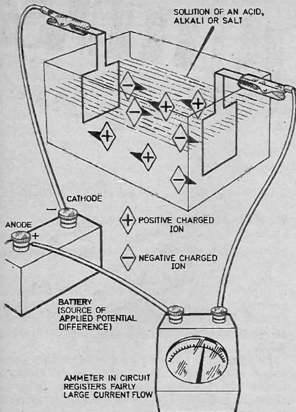
Fig. 1.1b. Electrical conduction in a solution, ionic movement.
