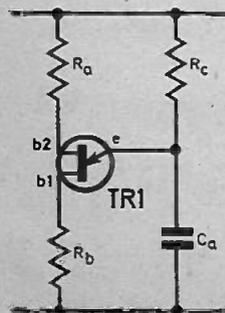
Fig. 1. (left) The basic unijunction oscillator circuit.
