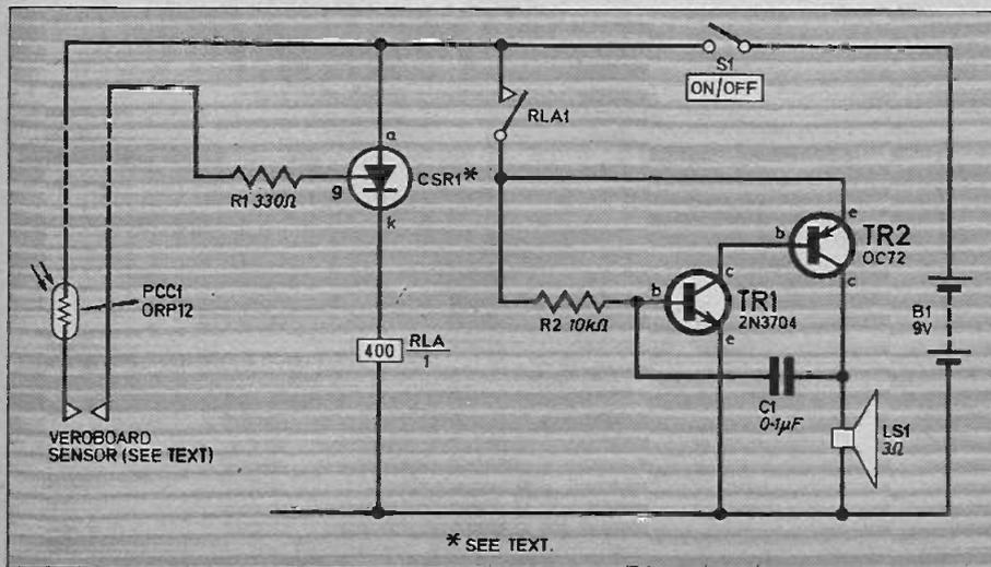
Fig. 1. The complete circuit diagram of the Rain Alarm. The l.d.r. prevents the alarm from sounding in dark conditions, i.e. at night.
