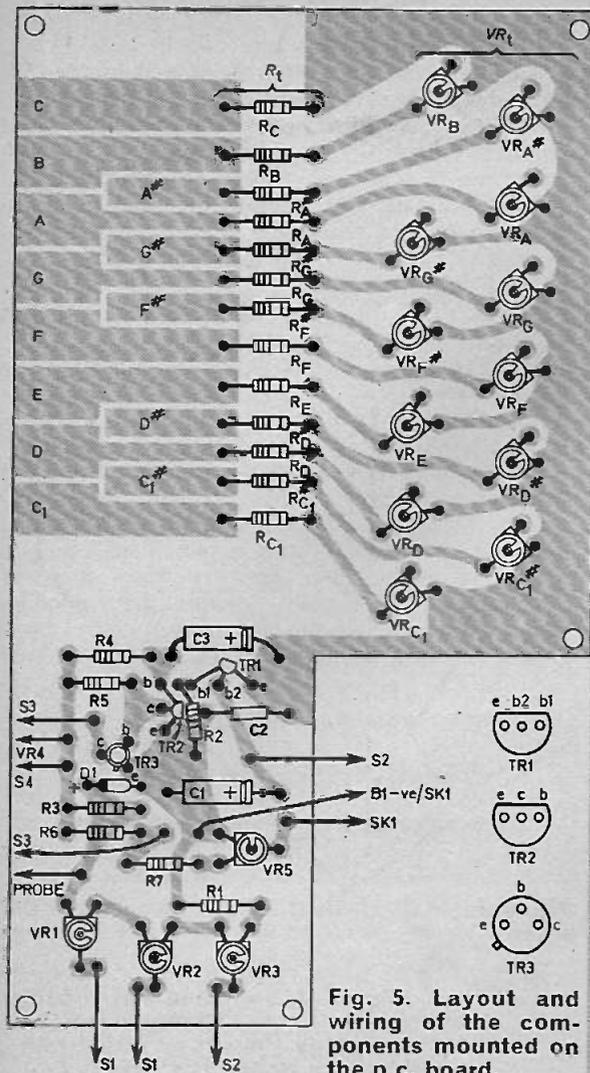
Fig. 5. Layout and wiring of the components mounted on the p.c. board.
