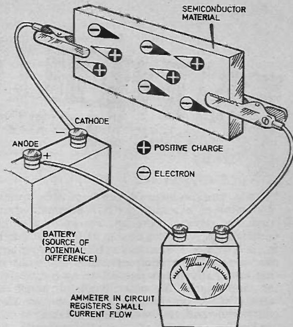
Fig. 1.1c. Schematic of electrical conduction in a semiconductor.
