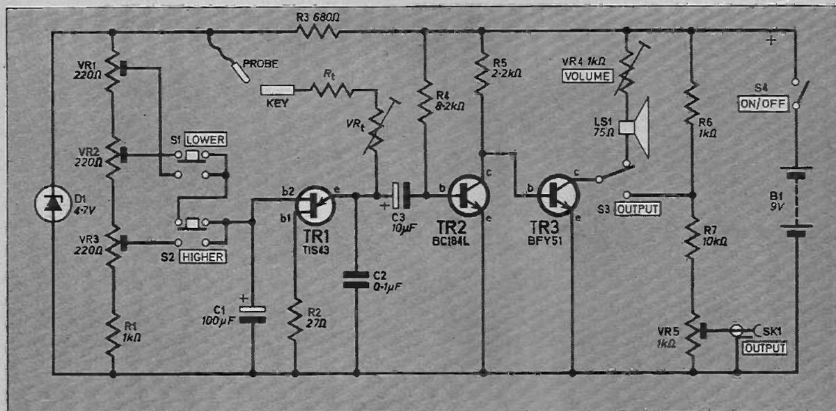
Fig. 3. Circuit diagram of the Mini Organ. Various values for  $R_t$  and  $VR_t$  for corresponding notes are given in Table 1.
