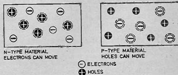
Fig. 1.4. *N* and *p*-type semiconductor materials. The broken circles show "fixed" charges.
