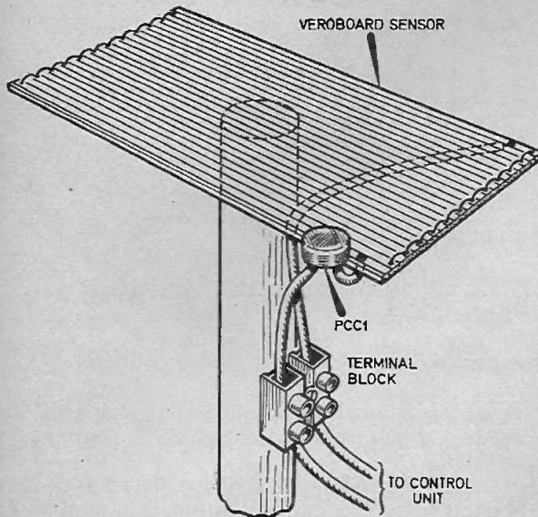
Fig. 4. Details of the Veroboard sensor.
