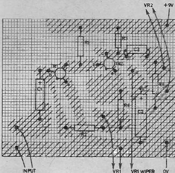
Fig. 2. The final design of printed circuit layout on graph paper.
