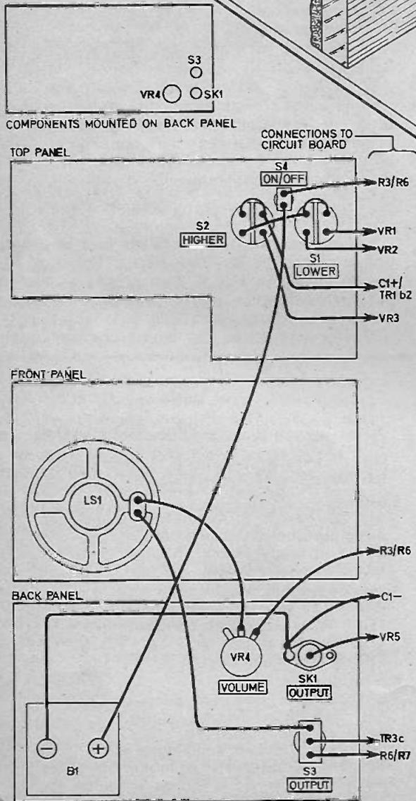
Fig. 7. (above) Layout and basic construction of the case. The size of the top is determined by the circuit board and thickness of the wood. The case is four inches high.
