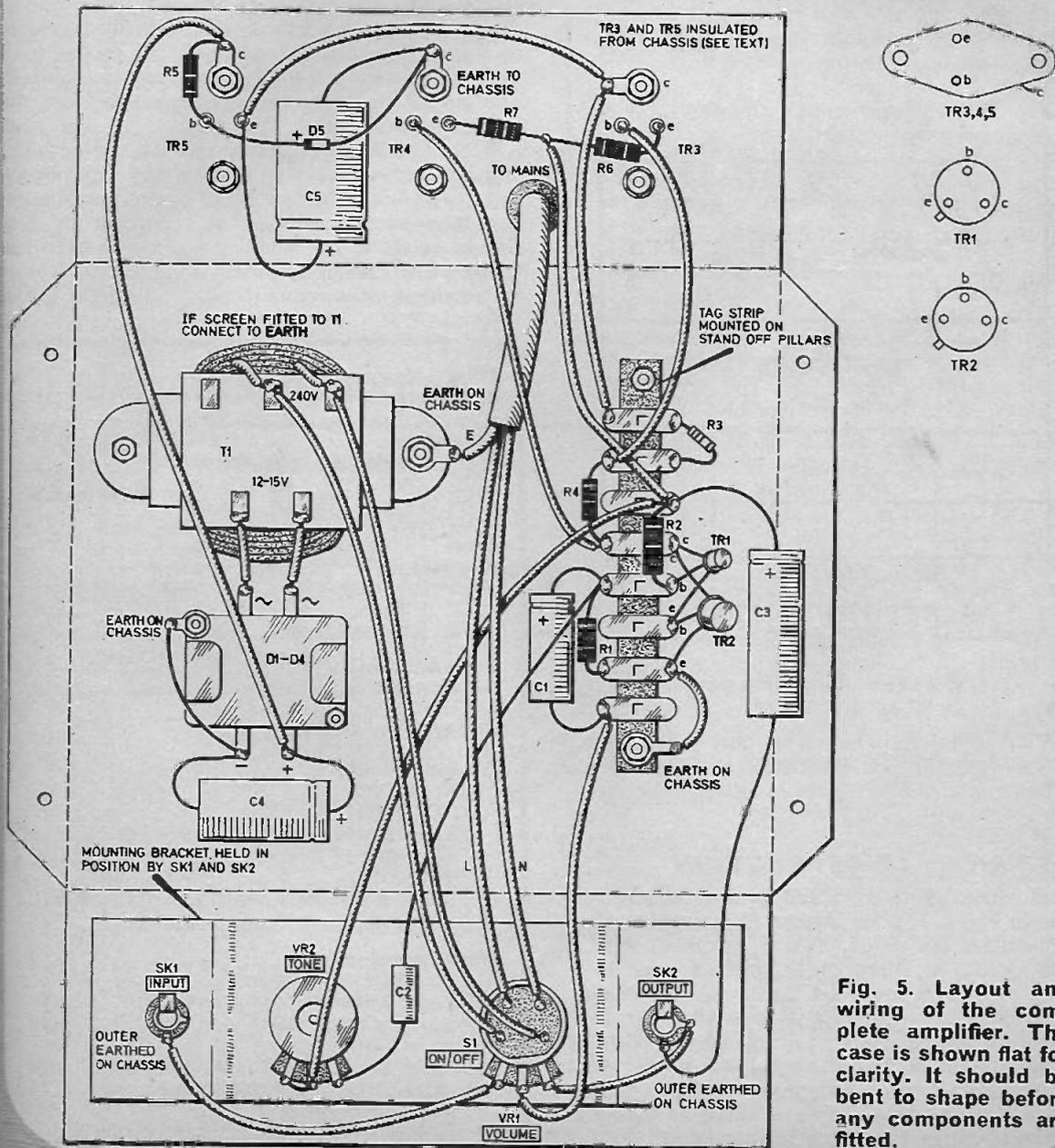
Fig. 5. Layout and wiring of the complete amplifier. The case is shown flat for clarity. It should be bent to shape before any components are fitted.
