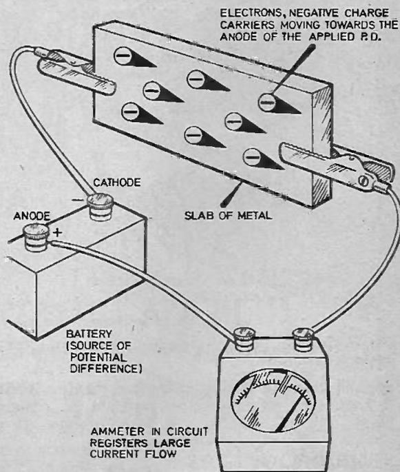
Fig. 1.1a. Schematic of conduction in a metal, movement of electrons.
