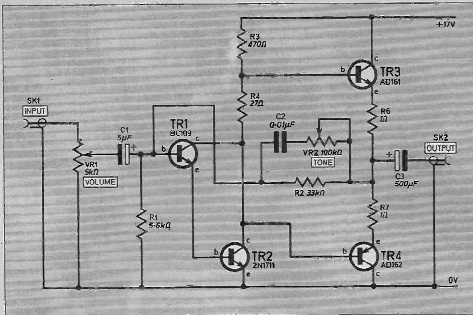
Fig. 1. Circuit diagram of the Cassette Amplifier.
