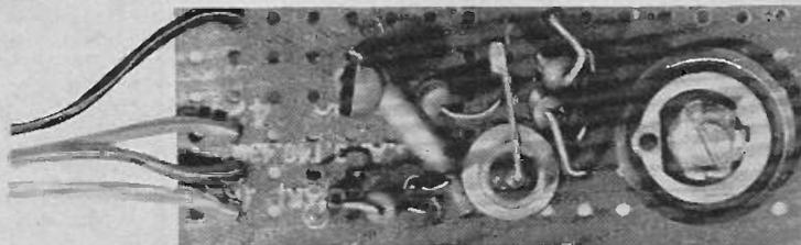
Photograph of the prototype Autofan Veroboard wiring.
