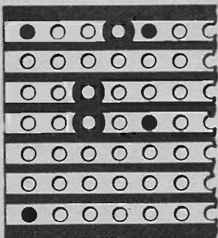
Fig. 6. Photograph and drawing of the underside of the same component board showing breaks and soldered connections.
