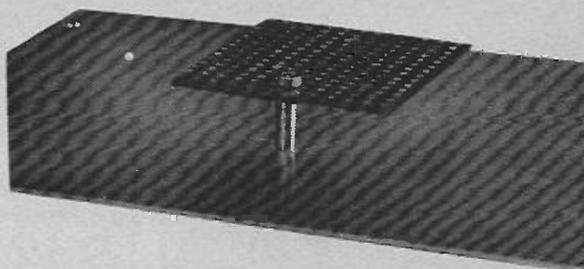
Method of mounting component board; applicable to all types of construction discussed here.
