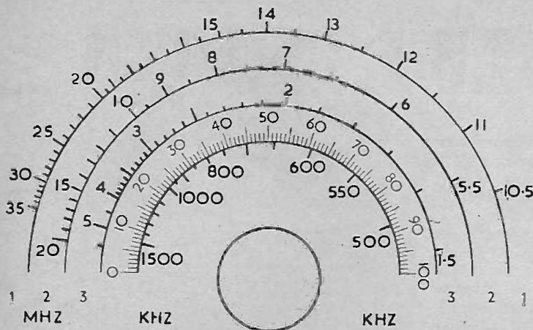
Fig. 6 Markings for the various ranges on the tuning dial this is shown full size and may be transferred directly to the scale.
