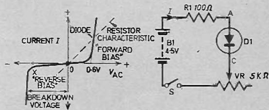
Fig. 2.8. Diode characteristics and test circuit.
