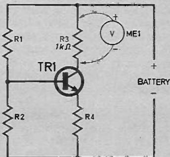
Fig. 1. Connecting ME1 as shown diverts current through R3.
