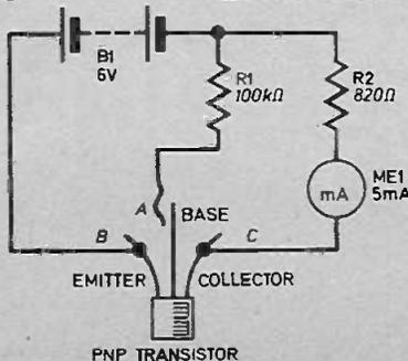
Fig. 6.1 (left). Circuit for the basic tests on an *npn* transistor.
