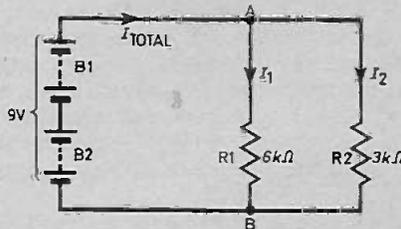
Fig. 2.4. A series parallel combination of resistors.
