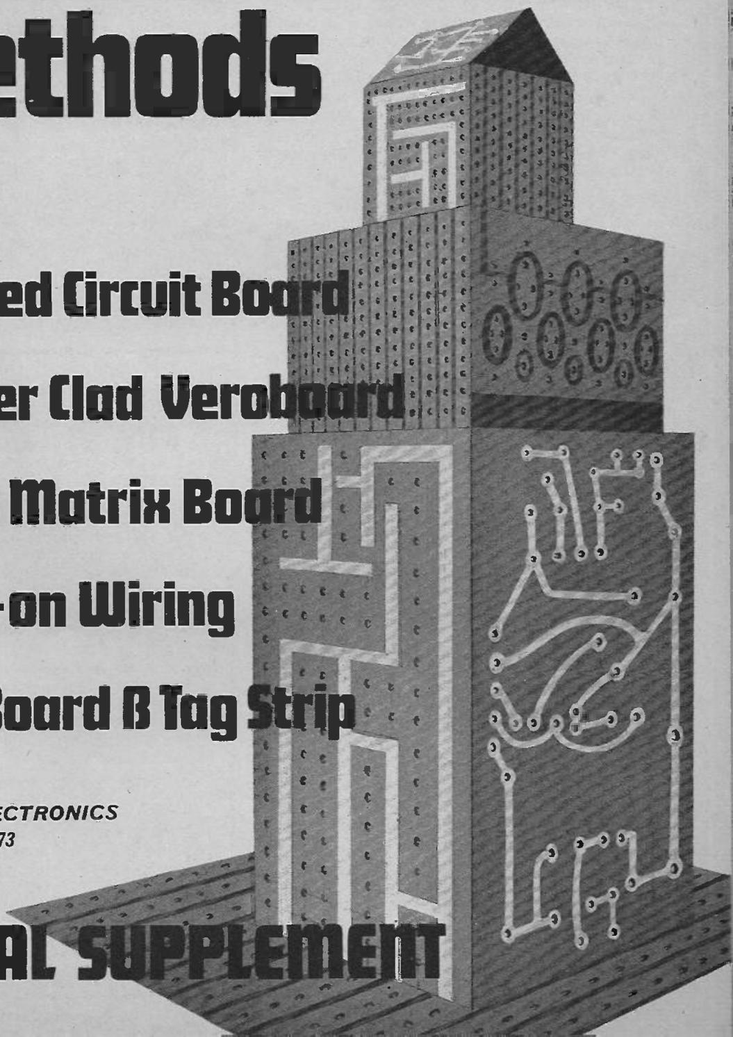
Not going back too far into the history of electrical and electronic circuits, the latter were built up in quite a different fashion from that employed today; the system used was called point-to-point wiring or the wired circuit, and this was the major (if not the only) method open to the amateur constructor at the time.
