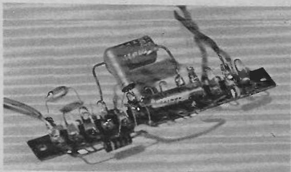
Fig. 12. Method of wiring up components on a piece of tag strip.
