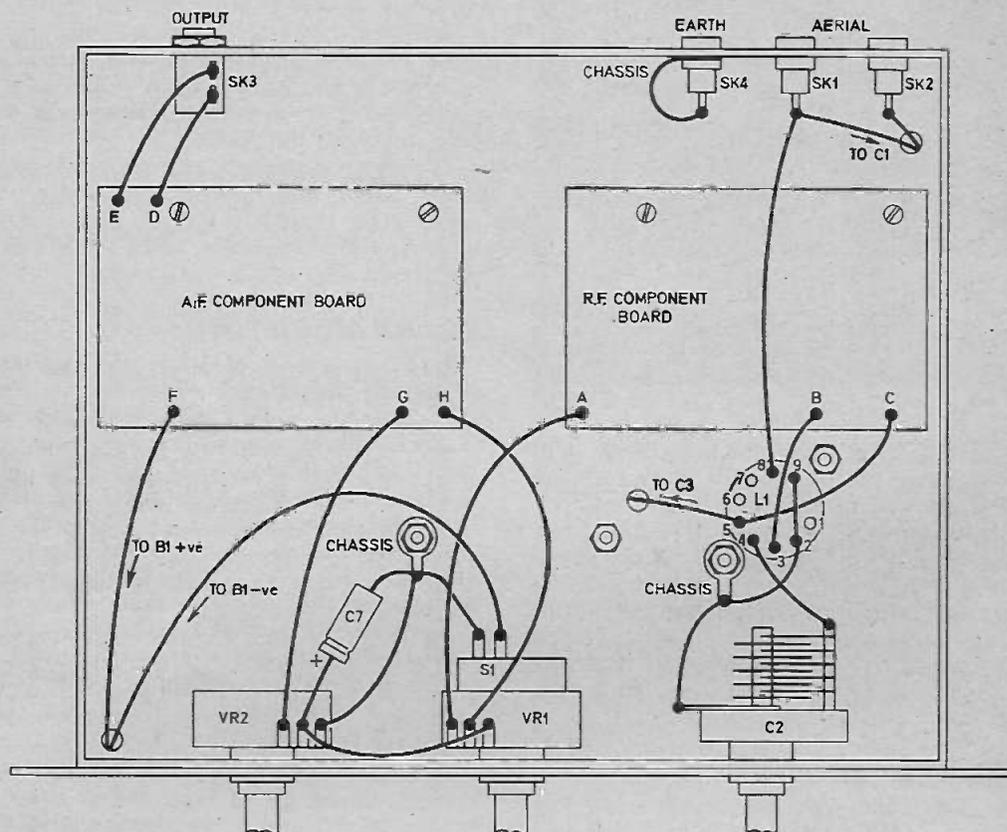
Fig. 4. Layout and wiring of parts mounted on the underside of the chassis.
