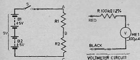
The red voltmeter lead should always be connected to the point at which current enters the component, otherwise the meter pointer will try to turn backwards. Repeat the test with  $R1=R2=10$  kilohms and then with  $R1=R2=100$  kilohms. In this last case the readings for  $V_{AB}$  and  $V_{BC}$  will both be lower than before at about 3.0 volts, whereas  $V_{AC}$  will still be approximately 9.0 volts. By reviewing Fig. 2.4 try to explain these results
