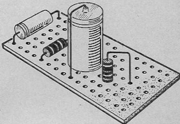
Fig. 8. Details of the two methods, horizontal and vertical, of mounting components on the component board.
