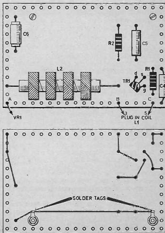
connect as shown for the underside wiring. A 20 s.w.g. tinned copper or similar wire is soldered between the tags for the metal chassis return points. In other places, the wire ends of the components are bent over and soldered as shown, and excess wire is then snipped off.
