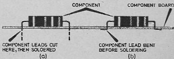
Fig. 5. Method of securing components to the component board.
