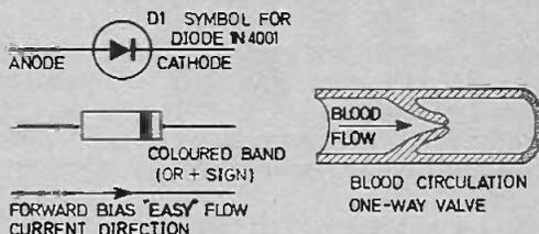
Fig. 2.7. The Diode and representation of its action.
