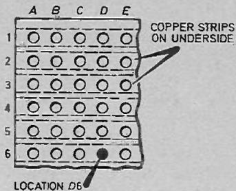
Fig. 7. Hole location using system of co-ordinates.
