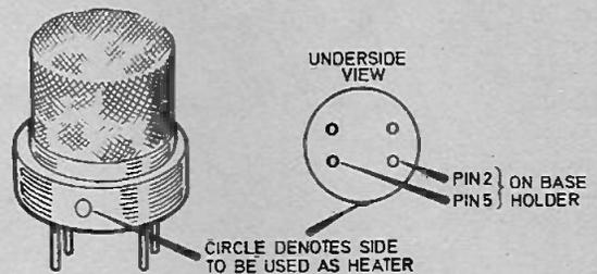
Fig. 4. Details of the sensor.
