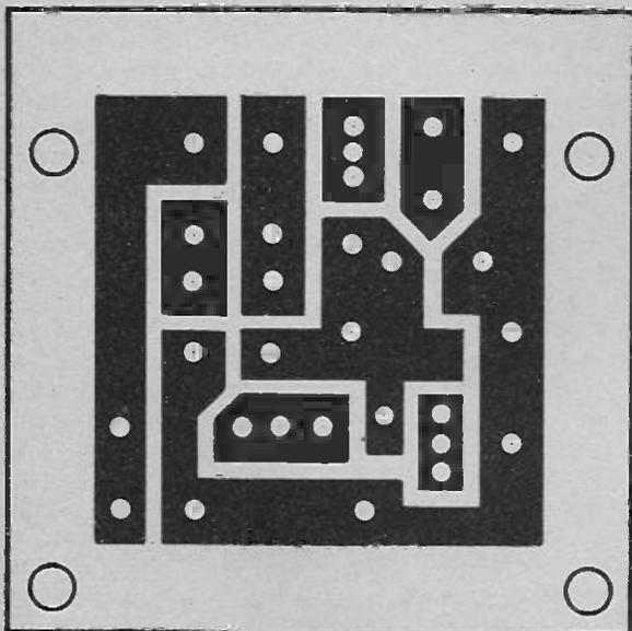
Fig. 2. The master drawing of the printed circuit.
