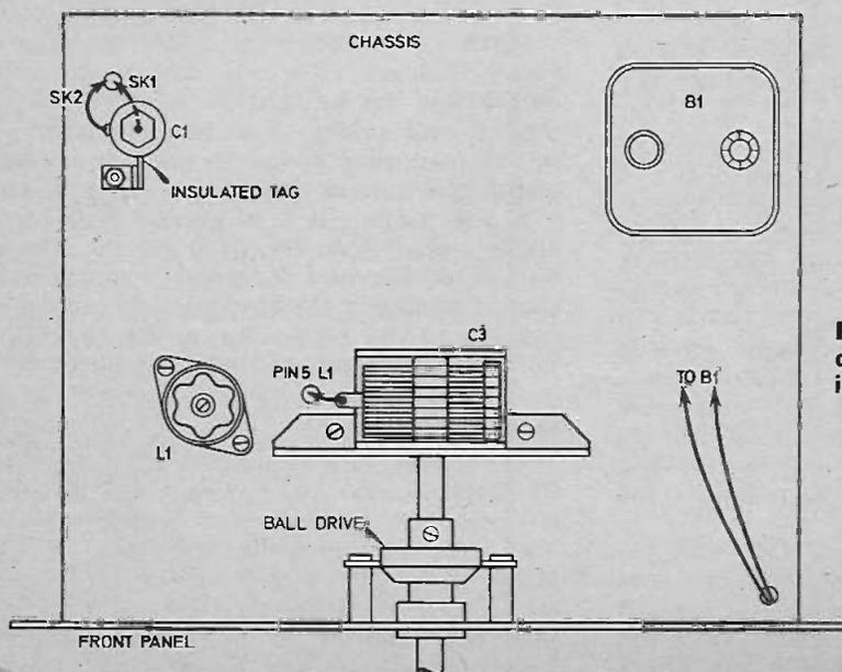
Fig. 5. Showing the positioning of the components and mounting for C3 on top of the chassis.
