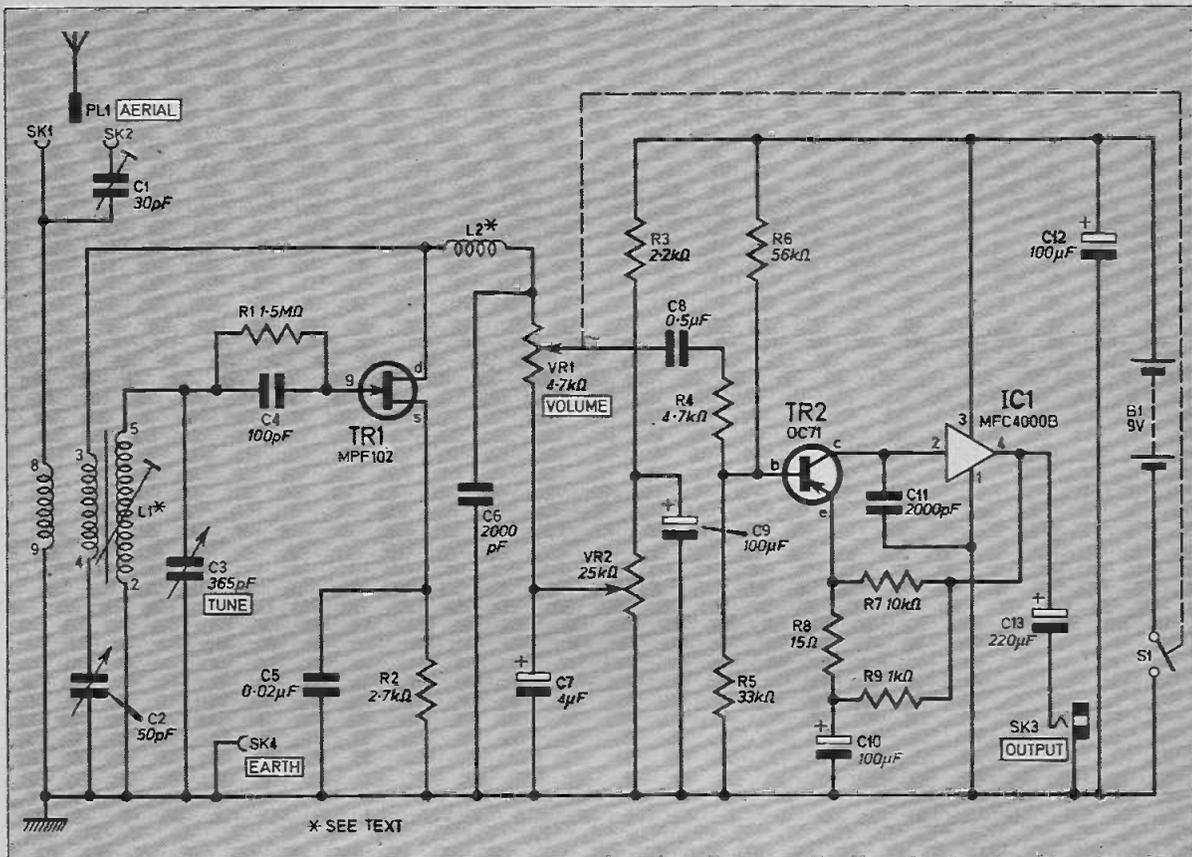
Fig. 1 Complete circuit diagram of the Four Band T.R.F. Receiver.
