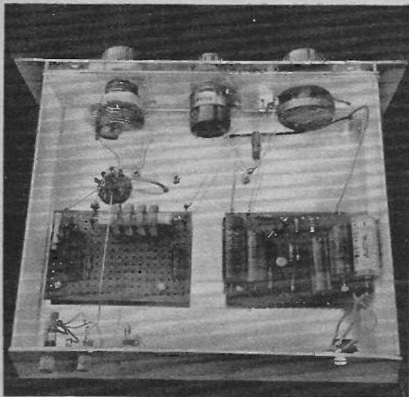
When fitting TR2, place emitter, base and collector leads in the positions e, b and c. The collector is marked by a spot on the case. The audio integrated circuit IC1 has two long and two short tags, and fits as in Fig. 3. These joints should be soldered without prolonged heating and preferably a heat shunt should be clipped on the leads while soldering.
