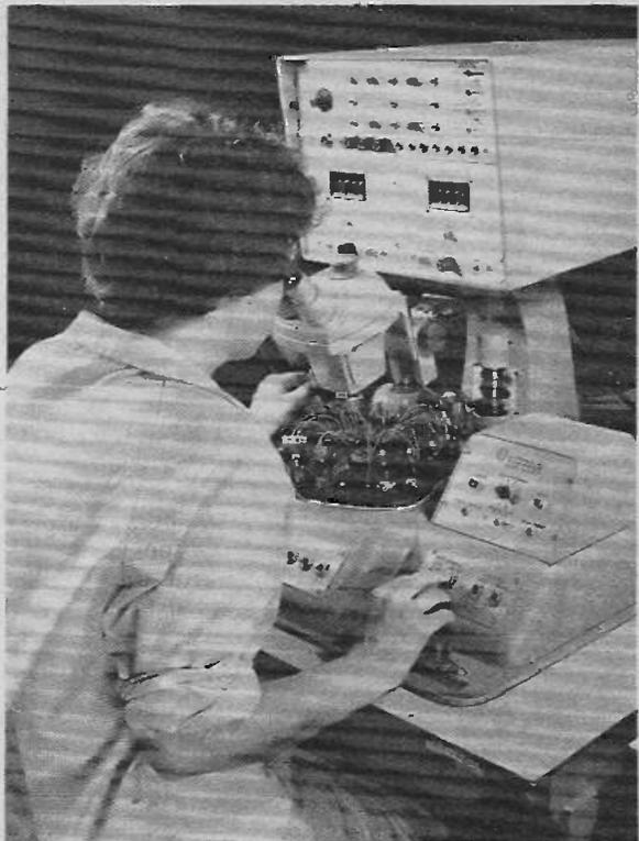
Pre-testing of integrated circuits at Mullard's. Silicon slices are being electrically checked.
