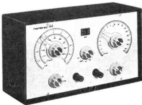
**Fig. 8. The inductance bridge marketed by Nombrex. This type of instrument will meet the needs of most private constructors.**
