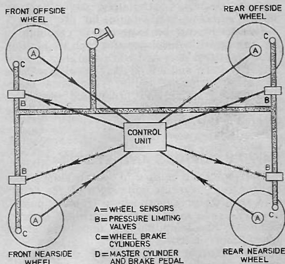
Fig. 3. Block diagram of an antilock braking system for vehicles.
