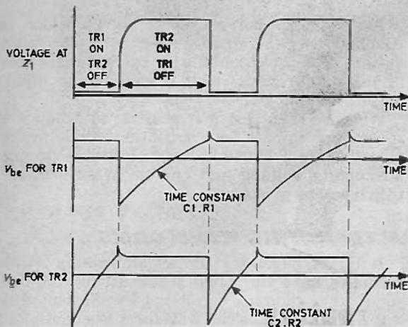
Fig. 8.2. Voltage waveforms for the astable multivibrator.
