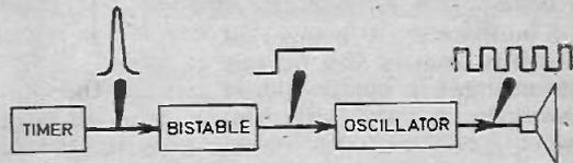
Fig. 1. The block diagram of the Egg Timer.
