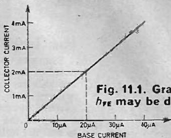
Fig. 11.1. Graph from which  $h_{FE}$  may be determined.
