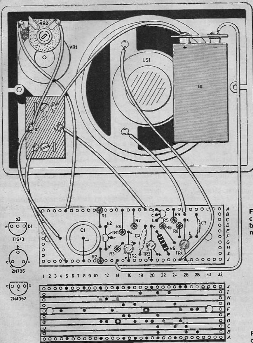
Fig. 3. The layout of the components on the Veroboard wired to the components mounted in the case.
