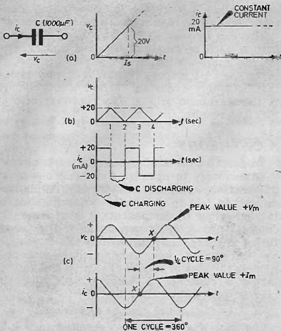
Fig. 8.7. Voltage and current waveforms for a capacitor.
