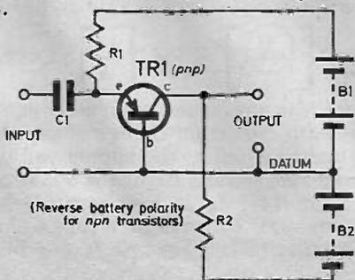
Fig. 8.4. Common base amplifier using two power supplies.
