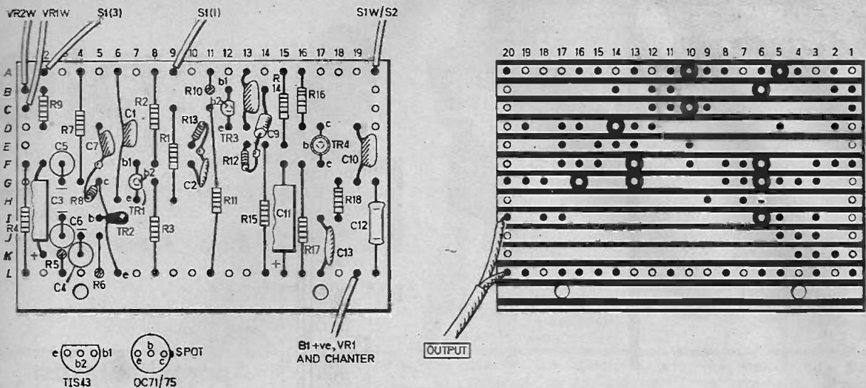
Fig. 2. Component layout and wiring on the Veroboard.
