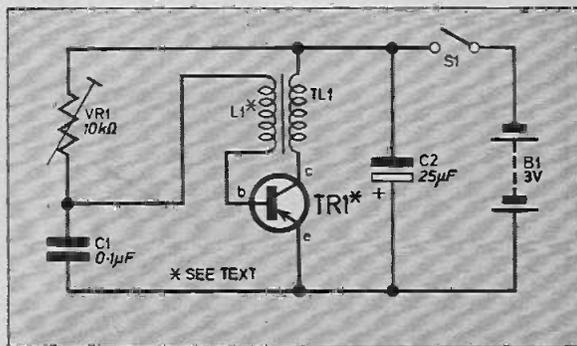
Fig. 1. Circuit diagram of the complete Simple Buzzer.
