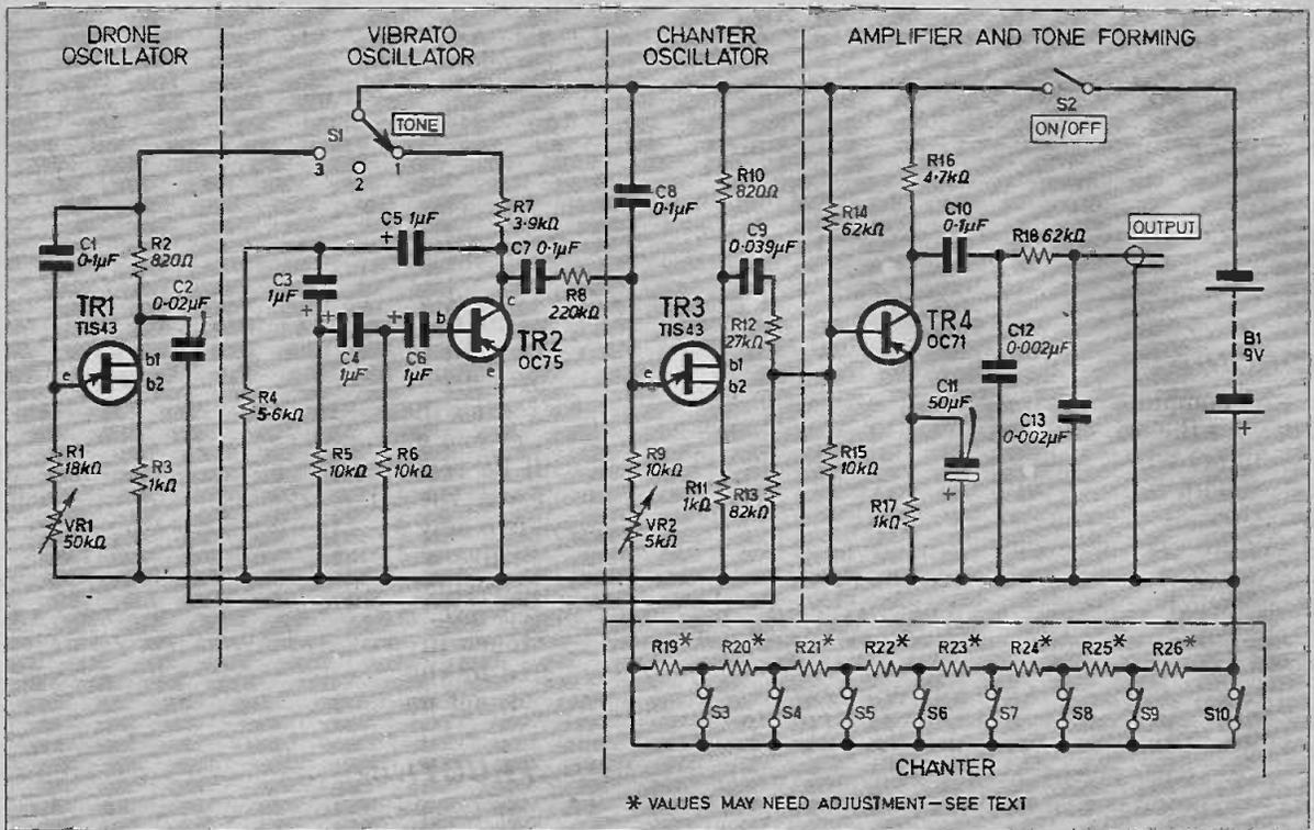
Fig. 1. Complete circuit diagram of the Electronic Bagpipes.
