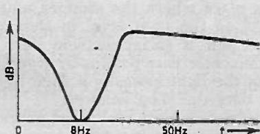
Fig. 3. Overall frequency response characteristic of the transistor stage.
