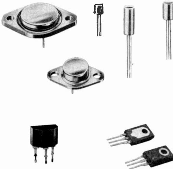
Photograph showing a few of the many different types of transistor encapsulations. (a) AD149 (b) BC107 (c) OC72 (d) AC128 (e) AD161 (f) BD201 (g) BC147—Lockfit. (Mullard)
