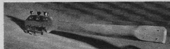
Photograph of the curved area of the neck/head showing required contours where the neck meets the head and the neck meets the body end fixing region.
