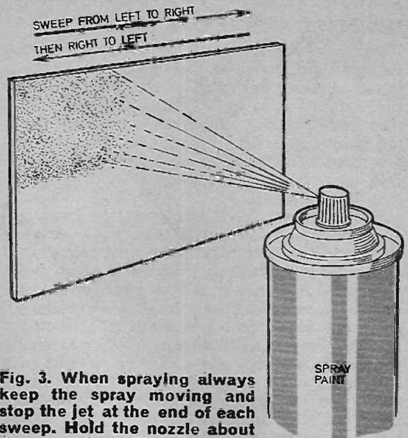
Fig. 3. When spraying always keep the spray moving and stop the jet at the end of each sweep. Hold the nozzle about 6in. away from the workpiece.
