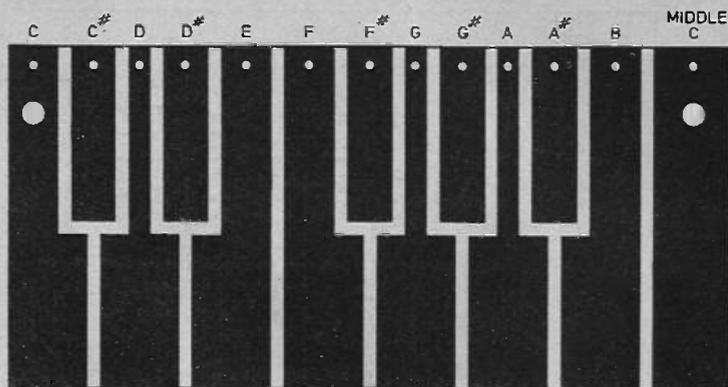
**Fig. 3. The master drawing of the Minstrel Keyboard, shown full size. The black areas indicate the regions of copper to remain after etching.**
