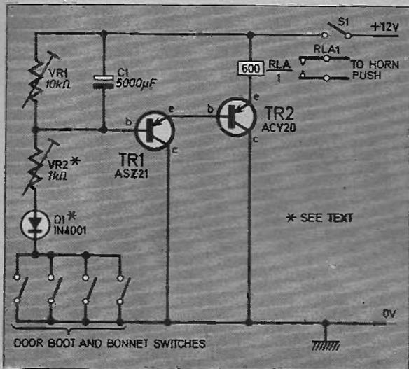
Fig. 1. The circuit diagram for the Car Alarm.
