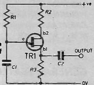
Fig. 1. A unijunction oscillator, the basis of the Minstrel.
