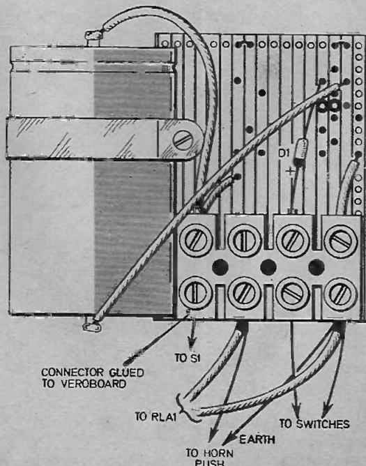
Fig. 2. The layout of the components on the Veroboard and complete wiring up details.
