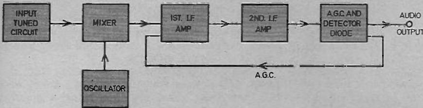
Fig. 1. Block diagram of a superhet. circuit.
