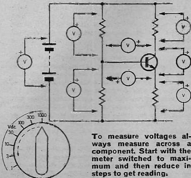
**To measure voltages always measure across a component. Start with the meter switched to maximum and then reduce in steps to get reading.**
