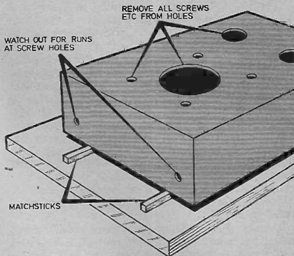
Fig. 2. When painting, stand the back of the box on match-sticks and try to keep the most important face horizontal.
