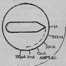
To measure current you must break the circuit and insert the meter across the break. Start with the highest range and reduce in steps to get a reading.
