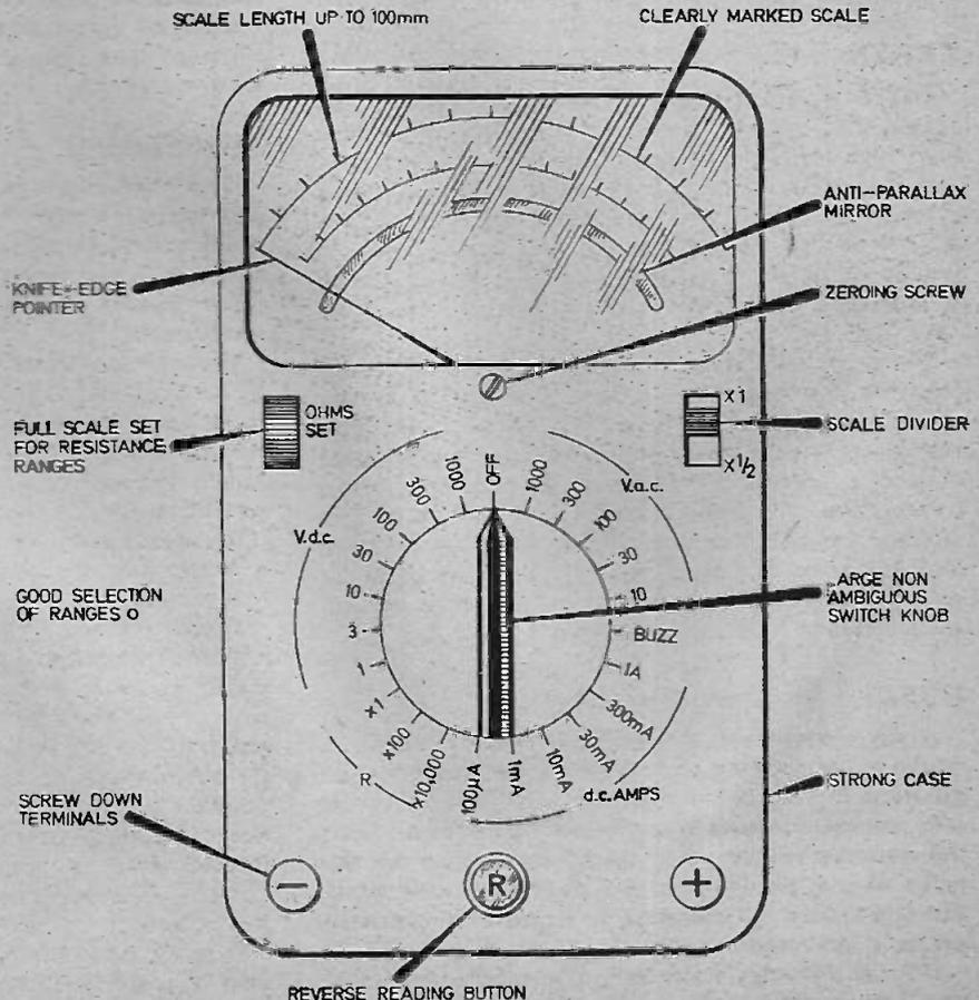
movement must have a full scale deflection of  $50\mu\text{A}$ .
