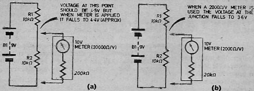
**Fig. 1.** The 20,000 $\Omega$ /V meter would read about 2 per cent low (a). Whereas the error would be over 15 per cent if a 2,000  $\Omega$ /V meter was used (b).
