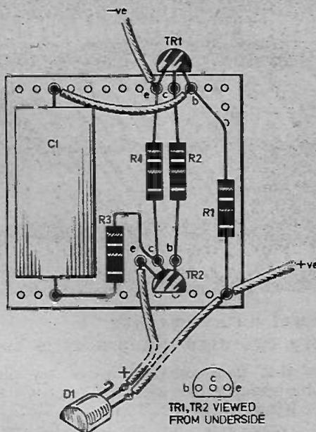
**Fig. 2.** The layout of the components on the matrix board and wiring up details.
