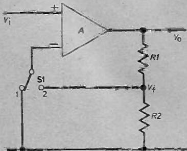
Fig. 1. An operational amplifier with negative feedback.
