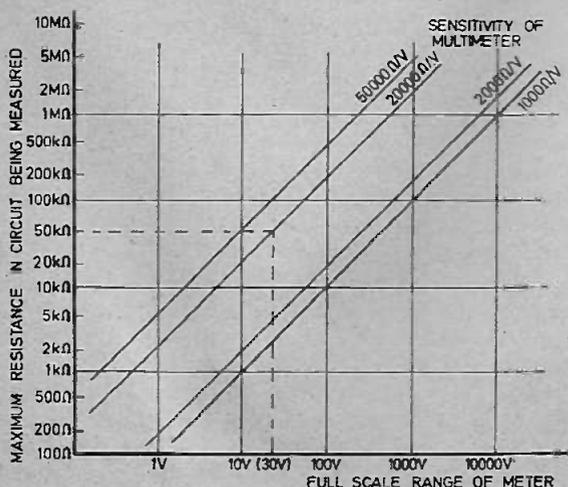
Graph showing maximum advisable resistor value across which you should measure. Example shown dotted—for a 20,000  $\Omega/\text{V}$  meter on 30V range maximum value is 50k $\Omega$
