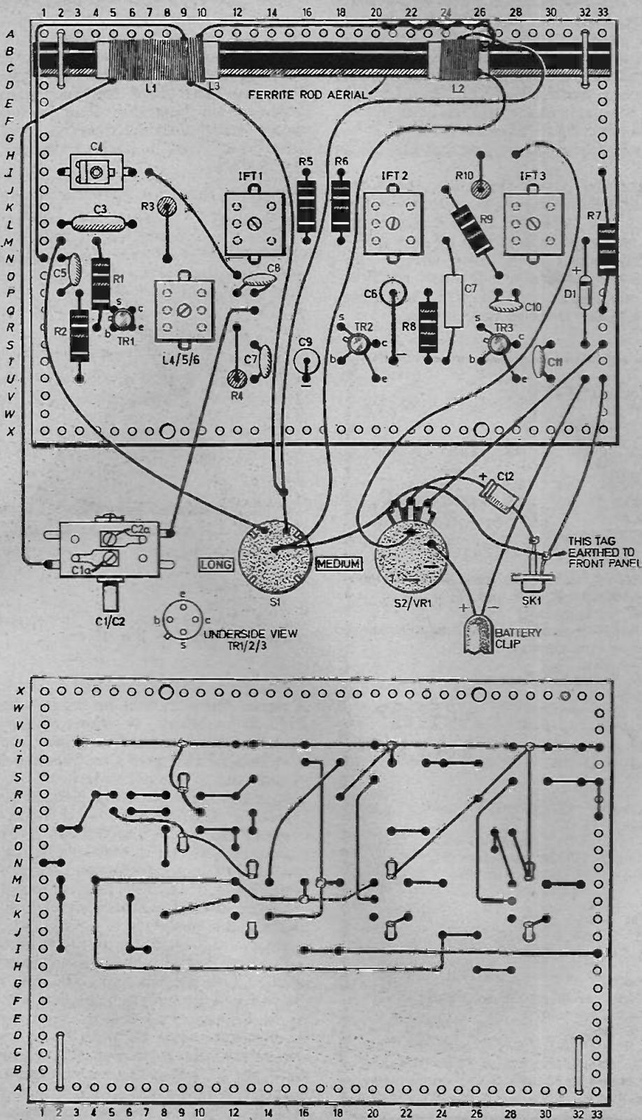
Fig. 5. Construction and wiring of the complete tuner.
