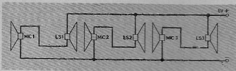
Fig. 4. The carbon granule amplifier.
