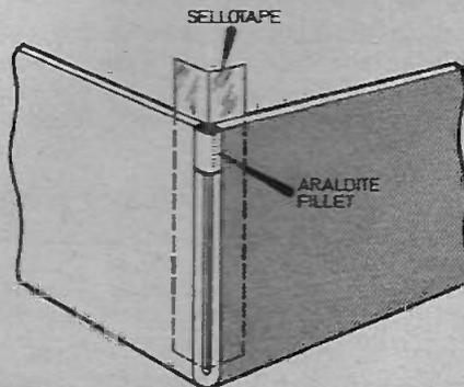
Fig. 4. Filling the gap along the edge of a bent aluminium case.
