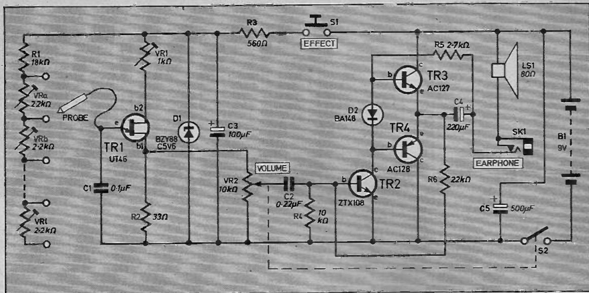
Fig. 2. The complete circuit diagram for the Minstrel.
