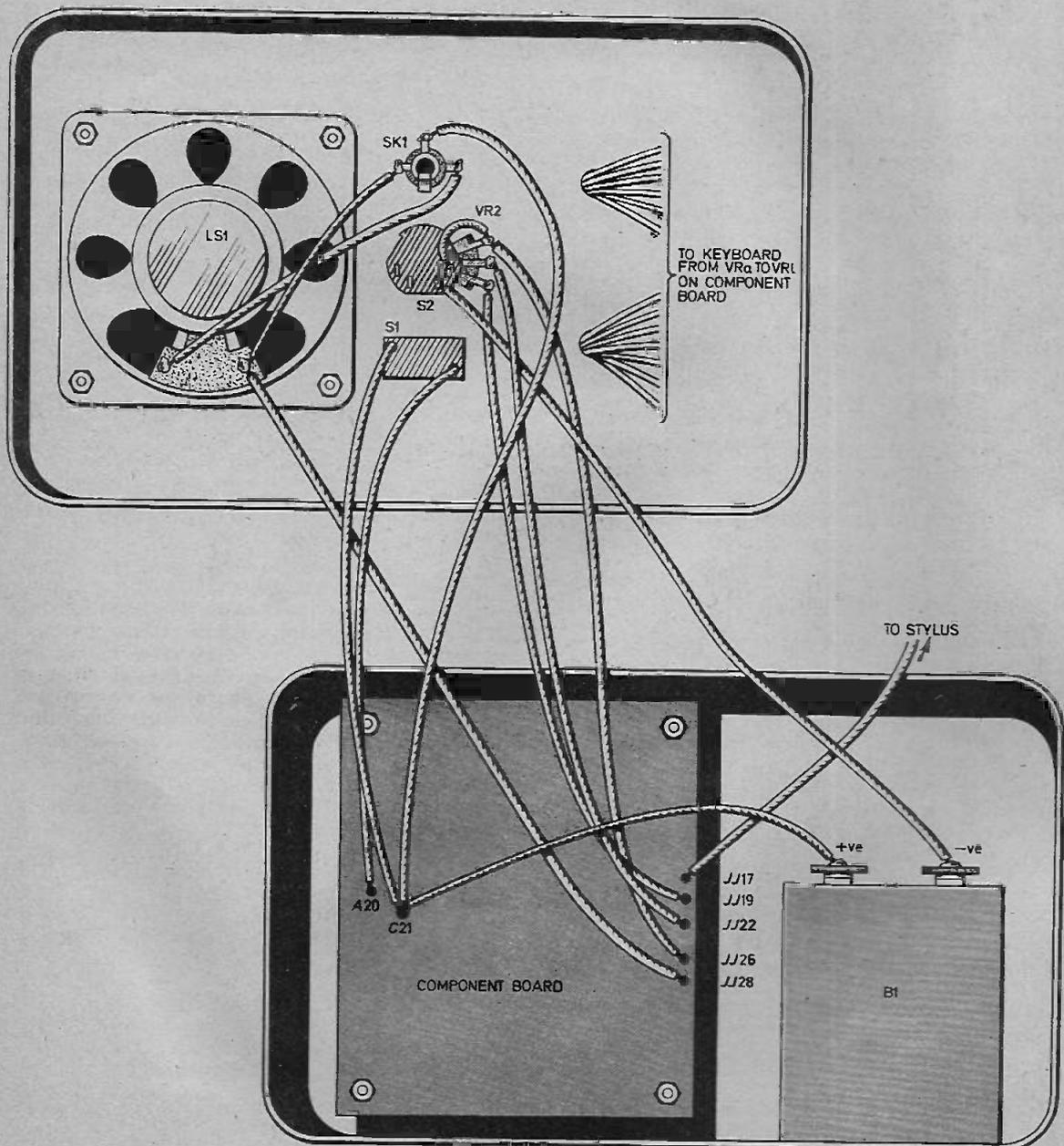
Fig. 5. Complete wiring up details and layout of the components.
