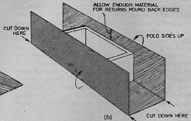
Fig. 4. Stages in covering a box with "Contact" or "Fablon".
