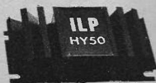
The HY50 is a complete solid state hybrid Hi-Fi amplifier. Incorporating its own high conductivity heatsink hermetically sealed in black epoxy resin. Only five connections are provided, input, output, power lines and earth.
