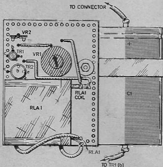
Fig. 2. The layout of the components on the Veroboard and complete wiring up details.
