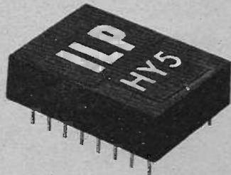
The HY5 is a complete mono hybrid preamplifier. Ideally suited for both mono and stereo applications. Internally the device consists of two high quality amplifiers—the first contains frequency equalisation and gain correction, while the second caters for tone control and balance.
