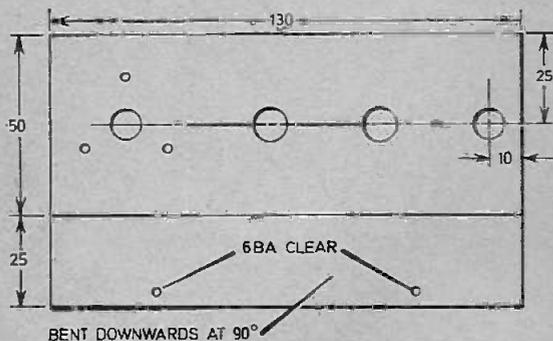
Fig. 4. Front panel and mounting bracket for component panel.
