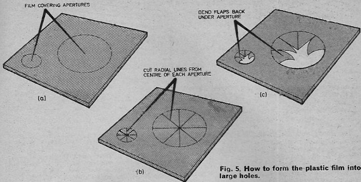
Fig. 5. How to form the plastic film into large holes.
