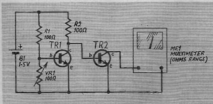
Fig. 2. One transistor is seen by the meter as a resistor whose resistance is varied by the other (TR1).
