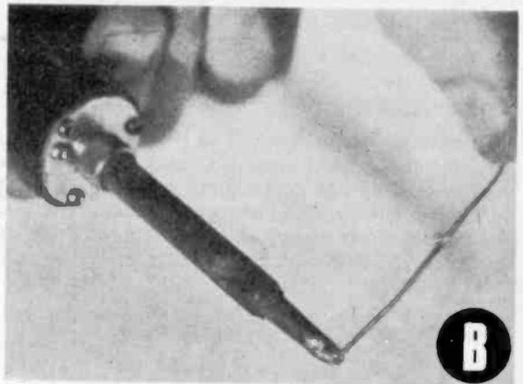
crystallised, is weak and probably has a high resistance. This could have been caused by carrying the solder to the joint on the iron, keeping the iron on the joint too long, thus burning off the flux, or by moving the wires before the solder has cooled.
