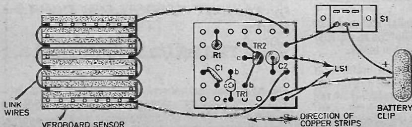
Fig. 2 The layout and wiring up details. Also shown are details for a sensor using 0.1 inch matrix Veroboard.
