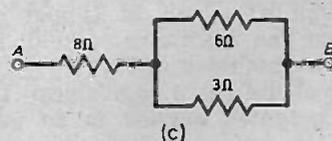
Fig. 2.1c. Shows resistors connected in series and parallel.
