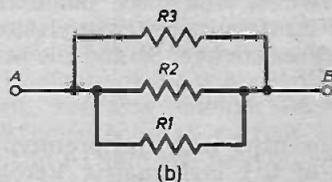
Fig. 2.1b. Resistors R1, R2 and R3 are said to be "in parallel" when connected as shown above.
