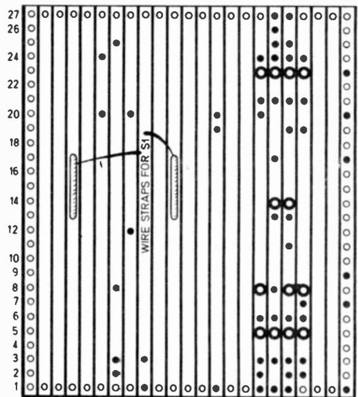
Fig. 2. The layout of the components on the Veroboard and wiring details.
