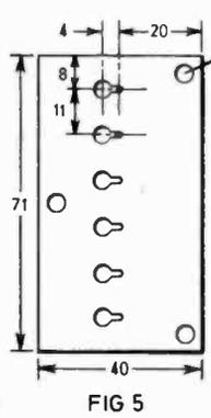
FIXING HOLES (4mm DIA)
