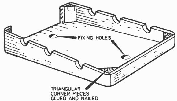
Fig. 8. Details of the head lower section.
