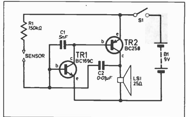
**Fig. 1.** The circuit diagram of the Rain/Water Alarm.
