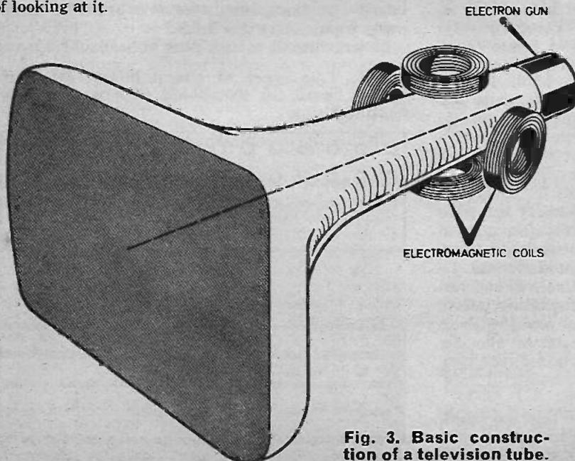
Fig. 3. Basic construction of a television tube.
