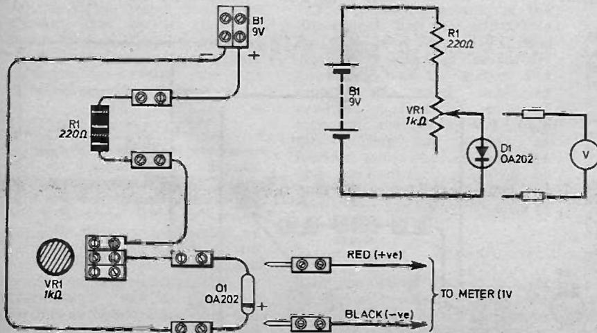
Fig. 5B1. Component layout on the Circuit Deck and complete wiring up details for experiment 5B. Also shown is the theoretical circuit diagram.
