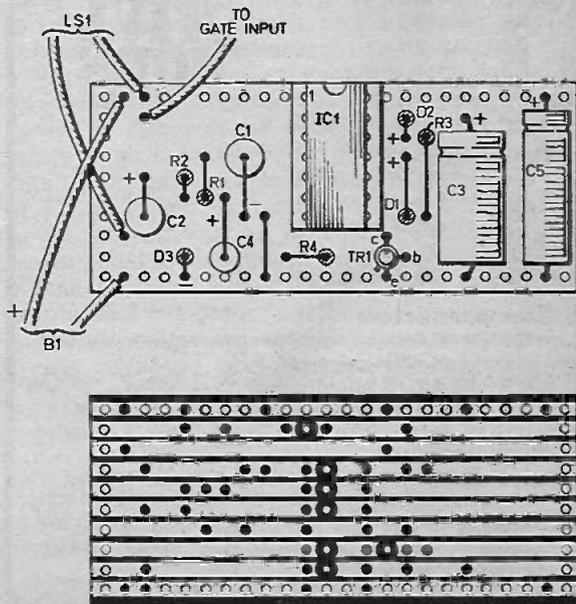
of the board and solder connections made as required on the copper strip side. The necessary breaks can be made in the copper strips either with a special spot face cutter, a 5mm twist drill or even a sharp craft knife.
