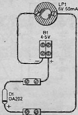
Fig. 5A.2. The layout of the component and wiring up details on the Circuit Deck for experiment 5A.
