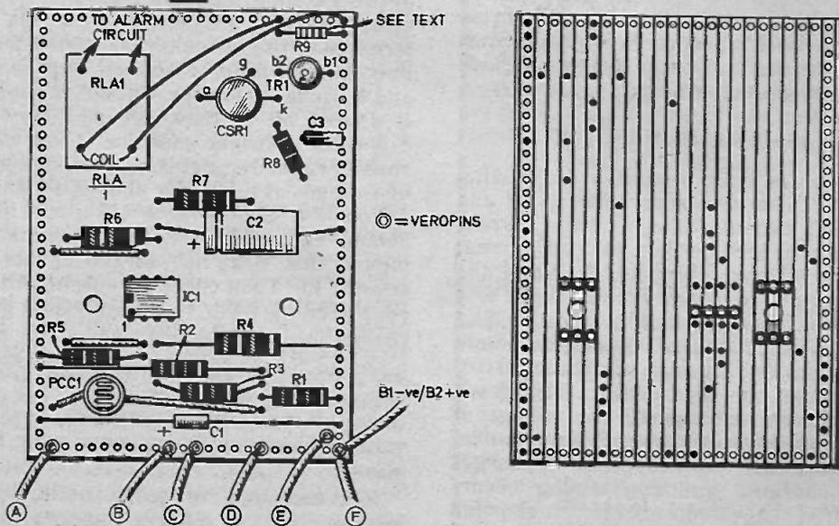
Fig. 5. Layout and wiring of the complete unit.
