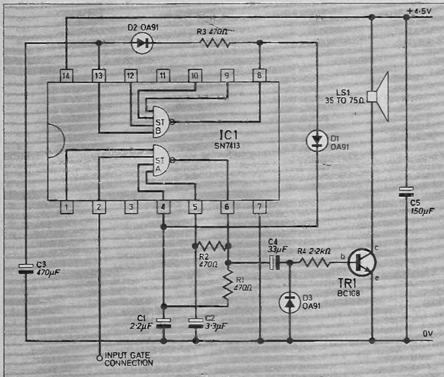
Fig. 1. Circuit diagram of the Two Tone Audio Oscillator
