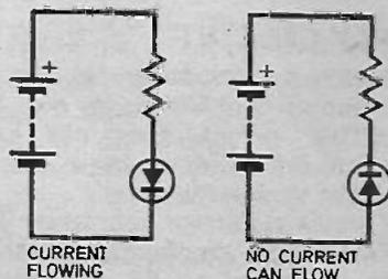
Fig. 5.1b. A simple circuit to illustrate the uni-direction property of a diode.
