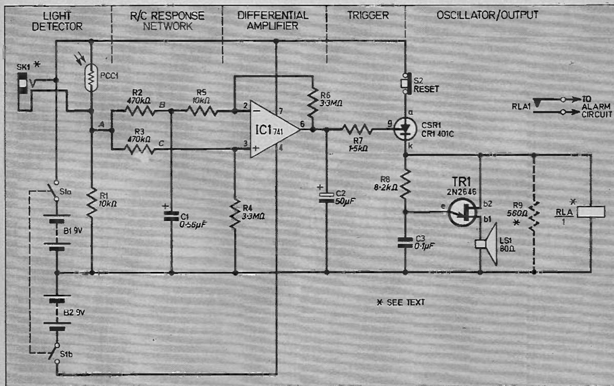
Fig. 4. Complete circuit diagram of the Electronic Watchdog.
