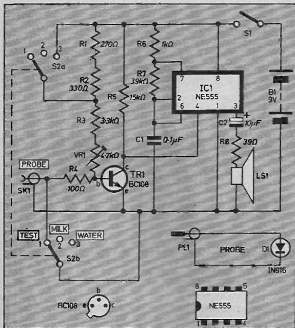
Fig. 1. Complete circuit diagram of the Boiling Liquid Alarm.
