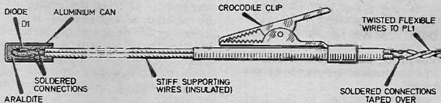
Fig. 3. Showing the construction of the temperature sensor probe.
