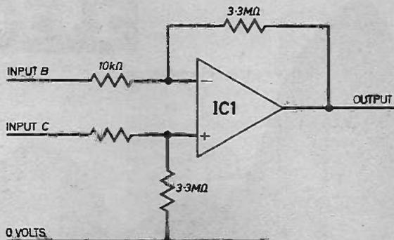
Fig. 3. Differential amplifier circuit.
