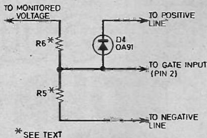
Fig. 2. Input gate circuit for an excess voltage alarm.
