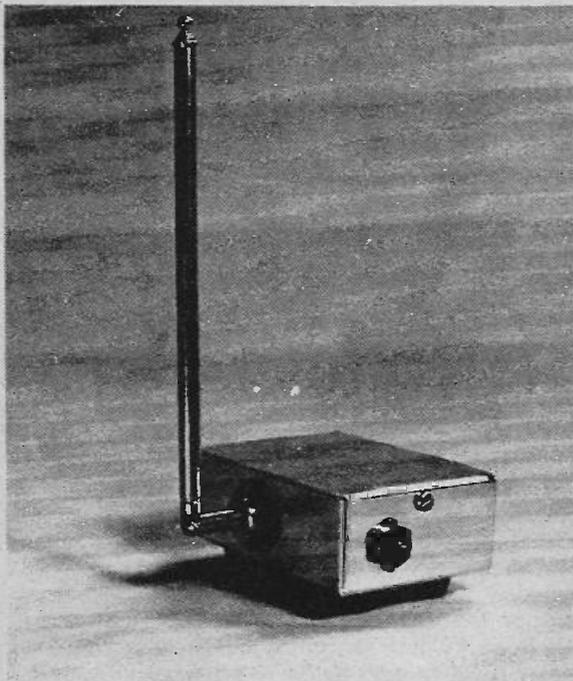
from the top of the coil. Place an operating 27MHz band radio control transmitter in the proximity of the monitor, with each aerial extended and parallel to each other. Set C1 at about half way, and then adjust C2 for peak reading on the meter.
