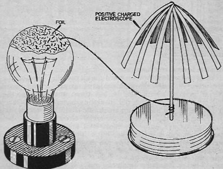
Fig. 2. Electroscope and light bulb to demonstrate electron polarity.
