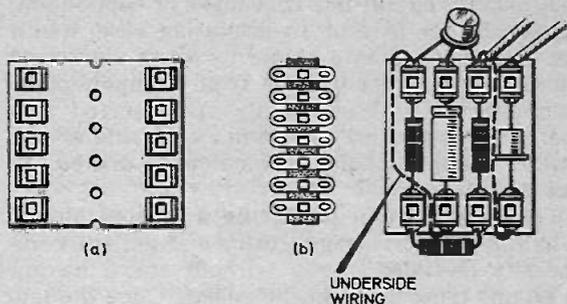
Fig. 3 (a and b). Two types of tagboard often used for construction. Also shown is a typical component layout.
