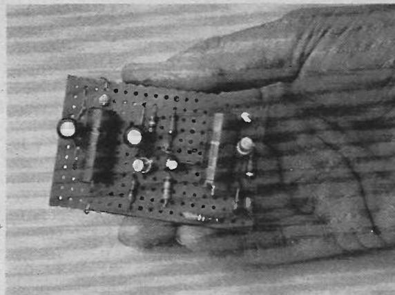
**Typical appearance of a circuit wired on Veroboard. The use of a file on the edges of the bare board would have given a better finished appearance.**
