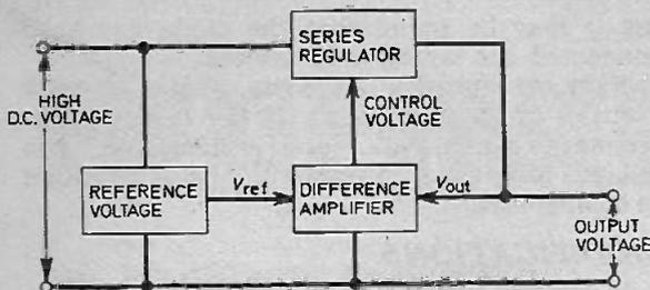
Fig. 1. Block diagram of a constant voltage power supply.
