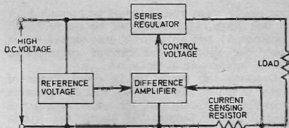
Fig. 2. Block diagram of a constant current power supply.
