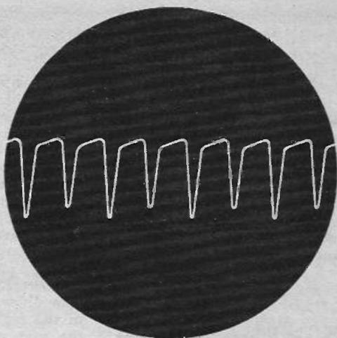
Fig. 2. The distorted waveform produced with the neon in circuit.
