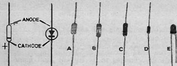
Fig. 5.1a. Schematic and circuit symbol of a diode. Photograph shows diodes used in this series (A) rectifier (B) point contact germanium (C) general purpose silicon (D) Zener (E) l.e.d.
