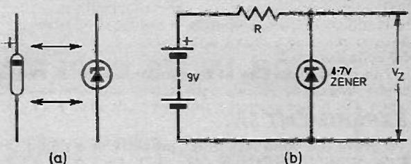
Fig. 5.4a. Shows the circuit symbol and appearance of a Zener diode (b) correct polarity to ensure Zener action.
