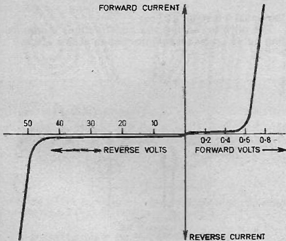
Fig. 5.2a. Graph showing forward and reverse characteristics for a silicon diode.
