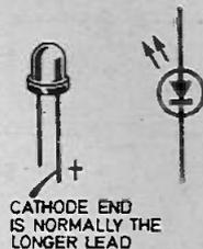
Fig. 5.5a. Shows physical appearance of a common light emitting diode oval circuit symbol. Sometimes the cathode is marked with a spot on the body.
