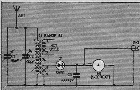
**Fig. 1. Complete circuit diagram of the Field Strength Meter.**
