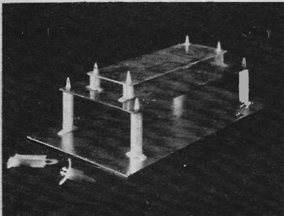
The Ilex mounting pillar's used to hold two printed circuit boards.
