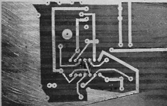
by no means critical but it is advisable to make the solution as strong as possible if you want the etching process to be reasonably quick. We suggest you start by mixing about 100 grams of hydrated ferric chloride into 100 millilitres of warm tap water; stir thoroughly and when all has dissolved try and dissolve a further 50 grams.
