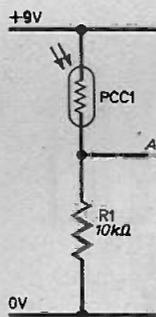
Fig. 1. Potential divider circuit.
