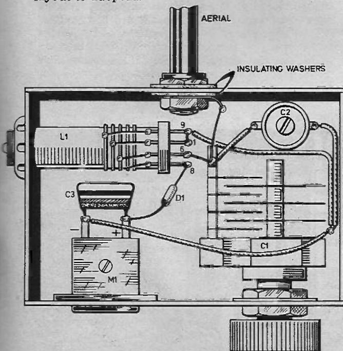
Fig. 2. Layout and wiring of the Field Strength Meter. Socket SK1 is not shown but this is simply wired across M1 if desired.
