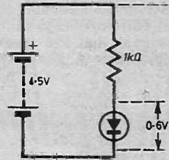
Fig. 5.2bA forward biased diode "drops" 0.6 volts.
