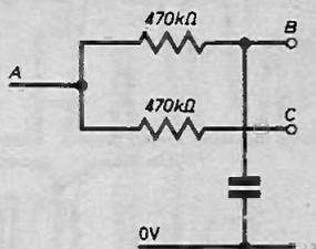
Fig. 2. Basic response circuit.
