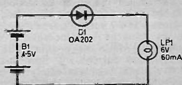
Fig. 5A.1. The theoretical circuit diagram to illustrate the "one way" property of a diode.
