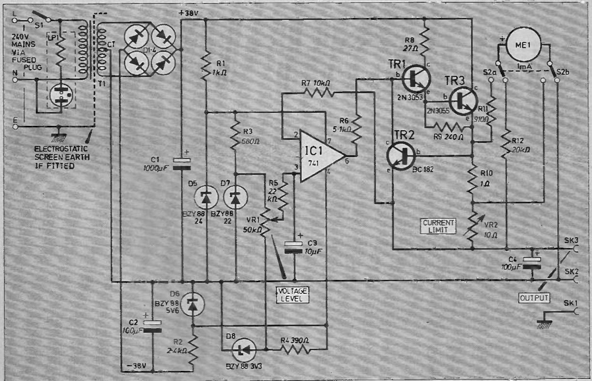
Fig. 3. Typical circuit diagram of a constant voltage supply with current limit.
