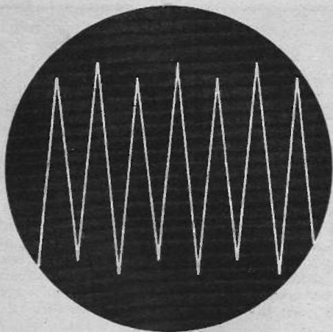
Fig. 1. The sawtooth triangular waveform produced by the tester.
