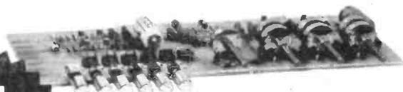
A top quality stereo pre-amplifier and tone control unit. The six push-button selector switch provides a choice of inputs together with two really effective filters for high and low frequencies, plus tape output.
