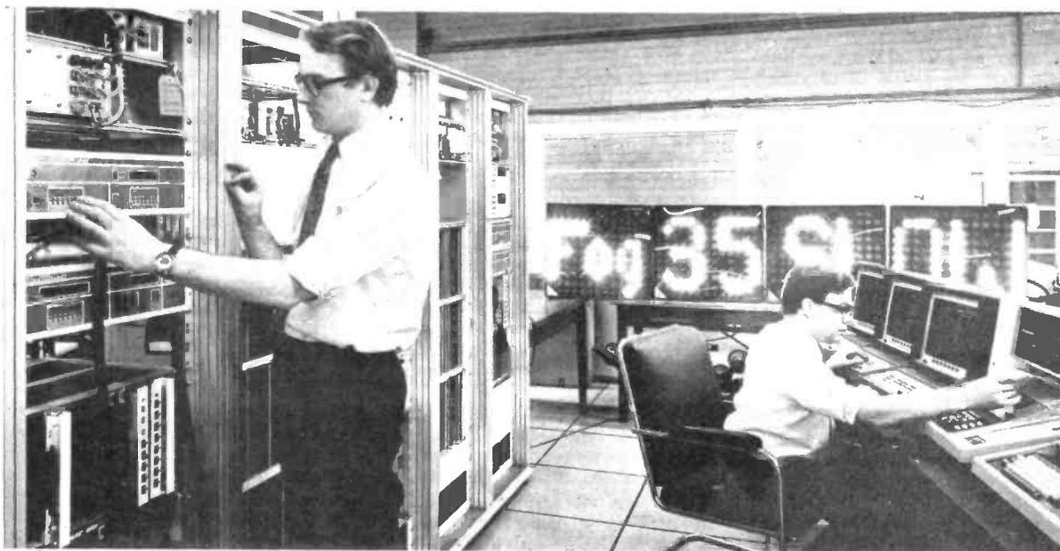
Checking out a computer-controlled hazard system for motorways at Ferranti, Manchester, before delivery to Australla. The computer does the toll-booth accounting and provides statistical data as well as controlling the hazard signs which can be seen in the background.
