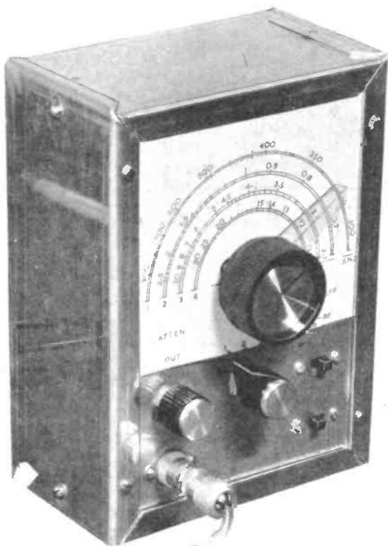
the 3-pole 4-way switch selects L1, L2, L3 or L4, for the four r.f. ranges. On ranges 2 and 4, tuning is by the section C1b of the 2-gang capacitor. To obtain suitable frequency coverage, the other part of this gang, C1a, is also in use on ranges 1 and 3, being brought into circuit by section S1b of the switch. The four ranges are calibrated as follows:
