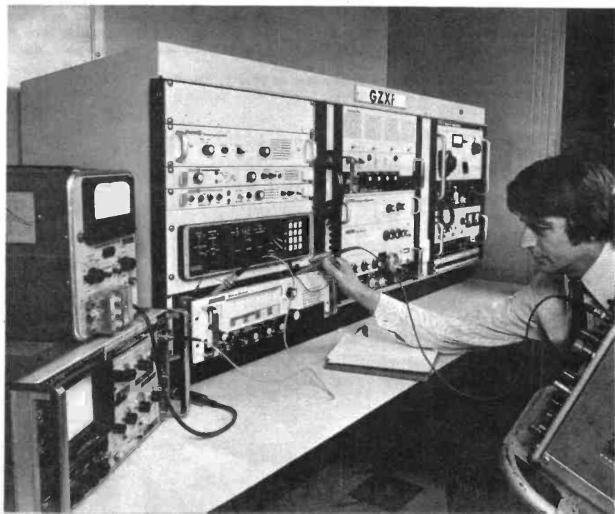
Checking out units of a ship's main radio console.
