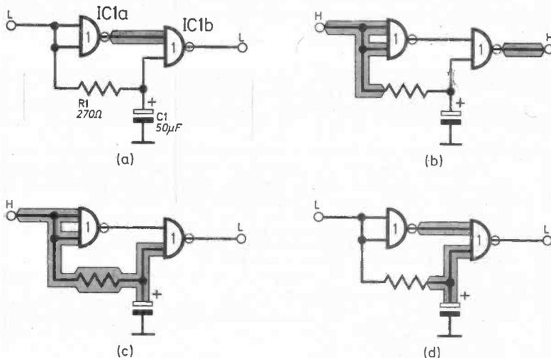
Fig. 7.1. Single pulse generator (a) shows the circuit before it is activated. The shaded areas indicate a high level. (b) shows the state of the circuit just after the input has gone high (c) shows the state after the capacitor has had time to charge and (d) shows the circuit when the input returns to low.
