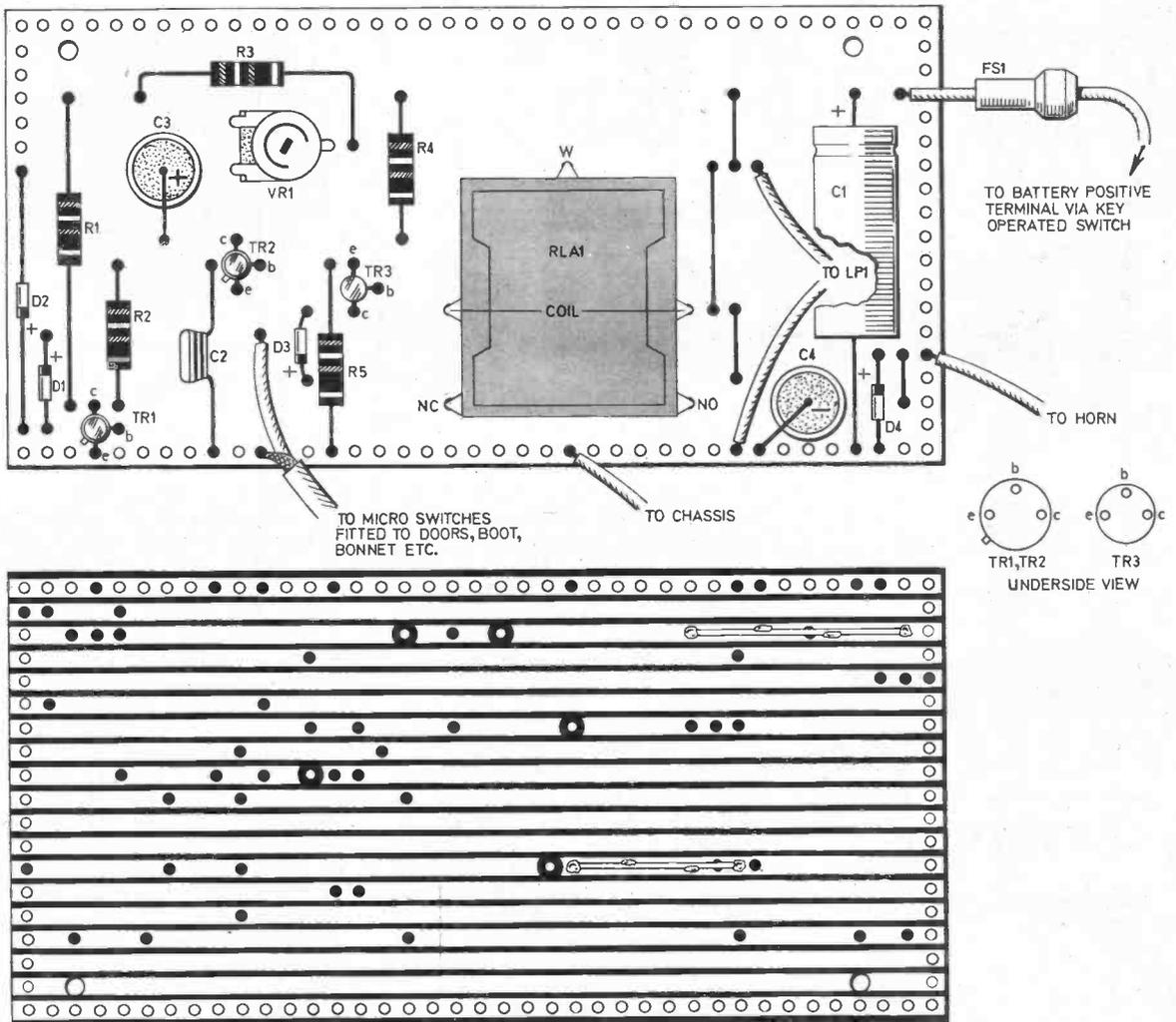
Fig. 2. The layout of the components on the topside of the stripboard and the cut-outs to be made on the underside and wiring details to the car. Note the stout copper wire soldered along the strips to enable high current flow.
