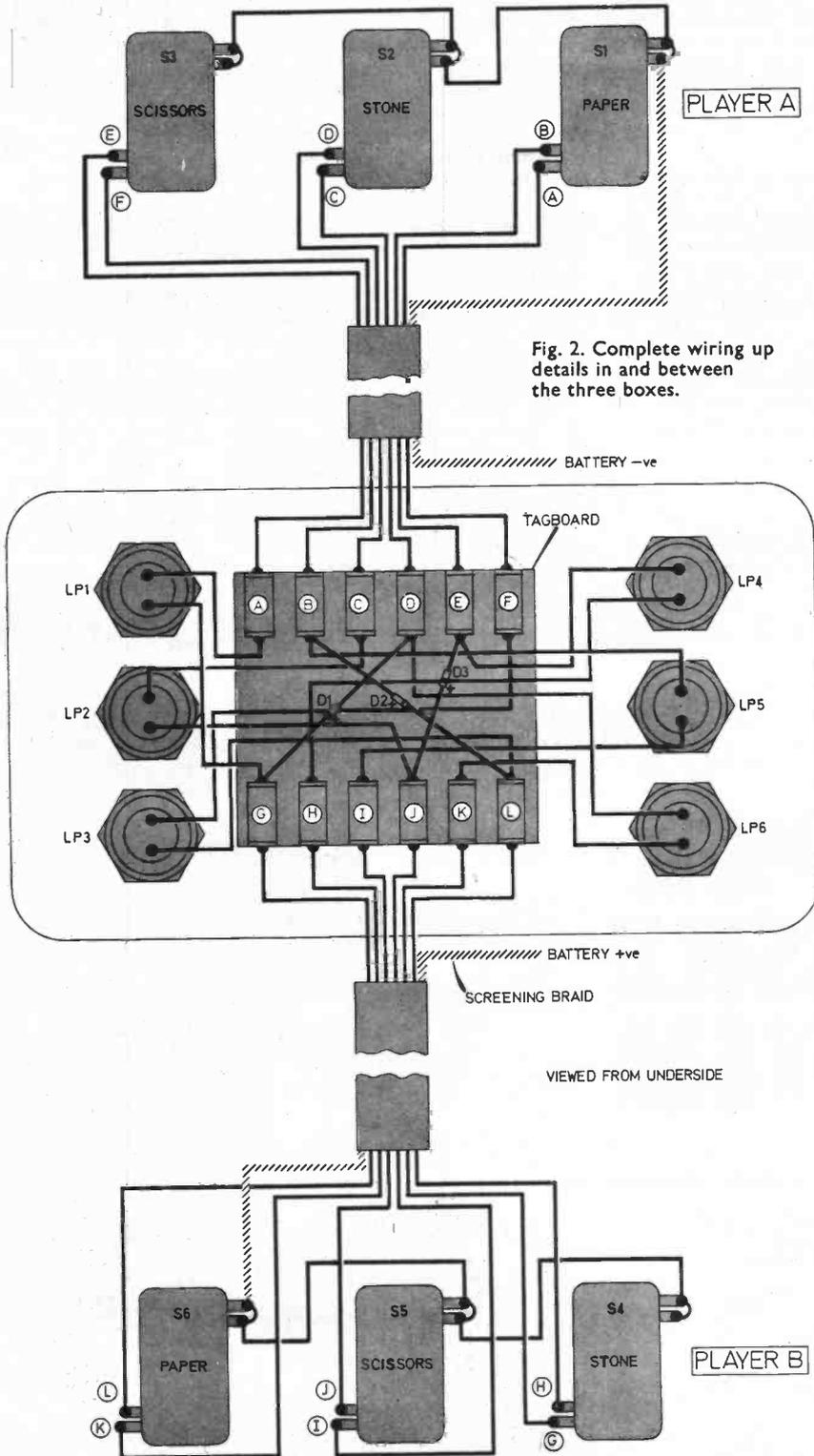
Fig. 2. Complete wiring up details in and between the three boxes.
