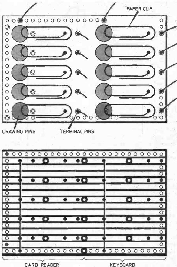
Fig. 7.12. Layout of the card reader (left) and keyboard (right) on the 0.15in matrix stripboard. Note the cuts in the strips under the board. The board can be sawn in half if the two units are to be used separately.
