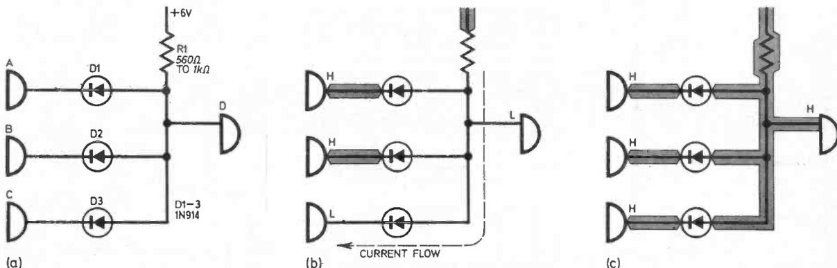
Fig. 7.3.(a) An AND gate using three diodes and a resistor connected to the output of three gates. Gates A, B, C and D can be any type of gate. (b) Current flow when the output of one of the gates is low (c) State of the circuit when the output from all gates are high.
