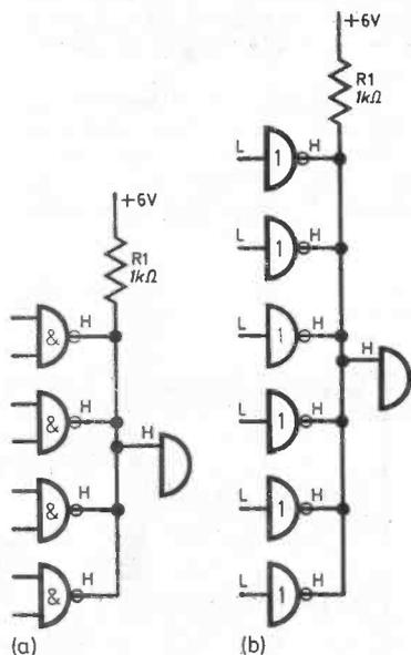
Fig. 7.5. (a) Type 7403 or 7401 i.c.s. wired together to form a WIRED-AND gate (b) Gates in a 7405 wired together form a WIRED-NOR gate.
