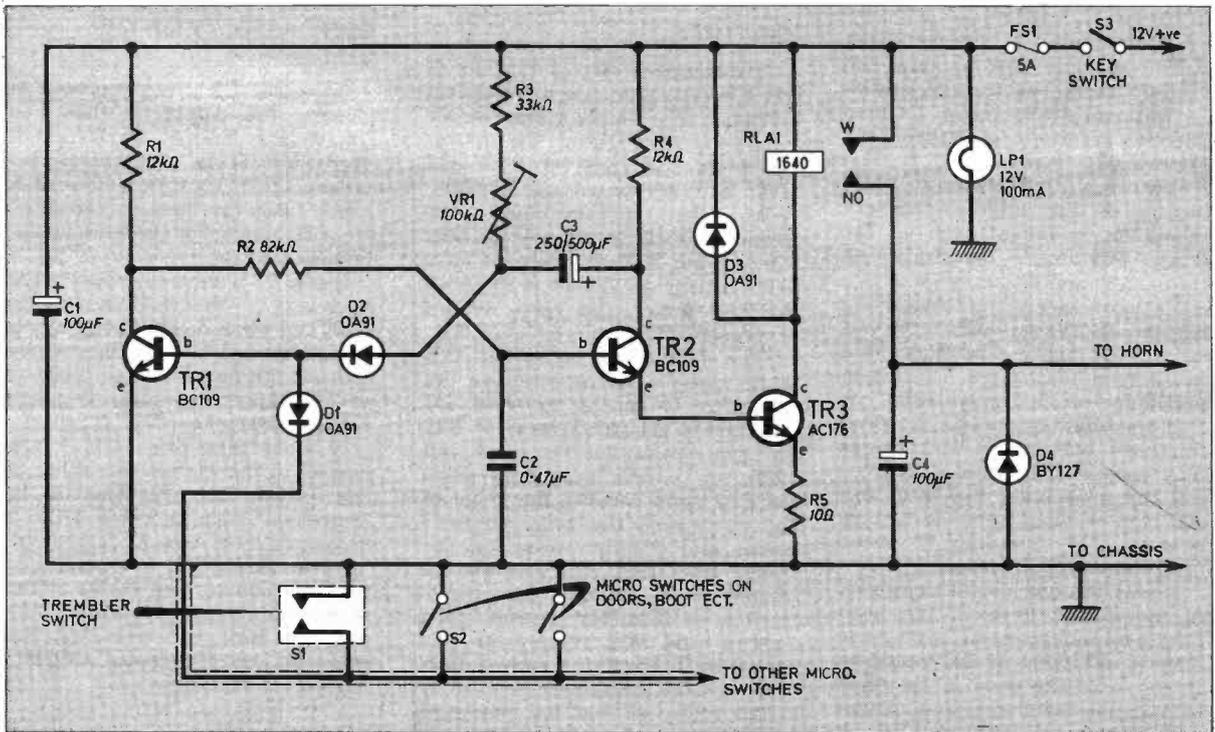
Fig. 1. The Complete circuit diagram of the Car Burglar Alarm.
