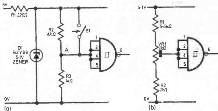
Fig. 7.11.(a) Circuit for a low battery indicator. The potential divider can be made from a preset and two resistors for setting the switching point, as at (b).
