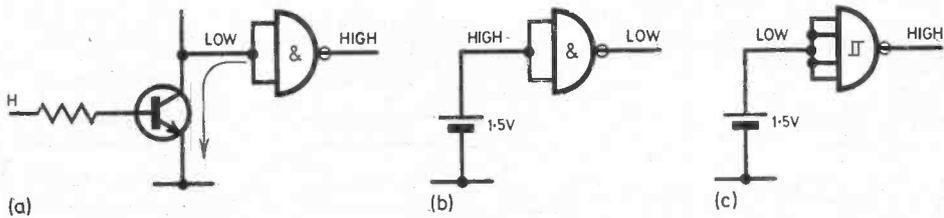
Fig. 7.8(a). A transistor connected to an ordinary gate provides a path for current to ground (b) A battery connected to an ordinary gate does not provide a current path to ground. (c) A 1.5V battery connected to a Schmitt gate acts as a low input
