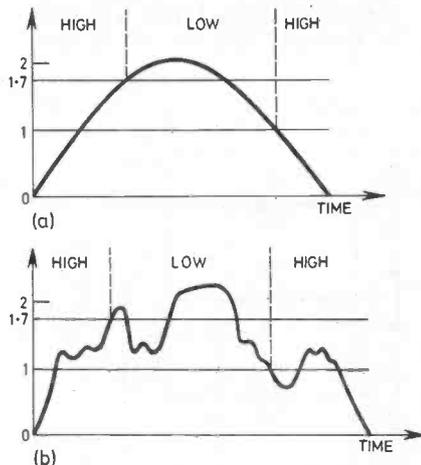
Fig. 7.7. (a) The output of the 7413 with a slowly changing input (b) the elimination of noise using the Schmitt.
