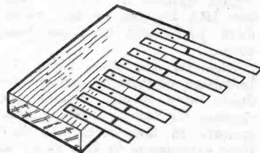
Fig. 2. The construction of a Kaffir Piano.
