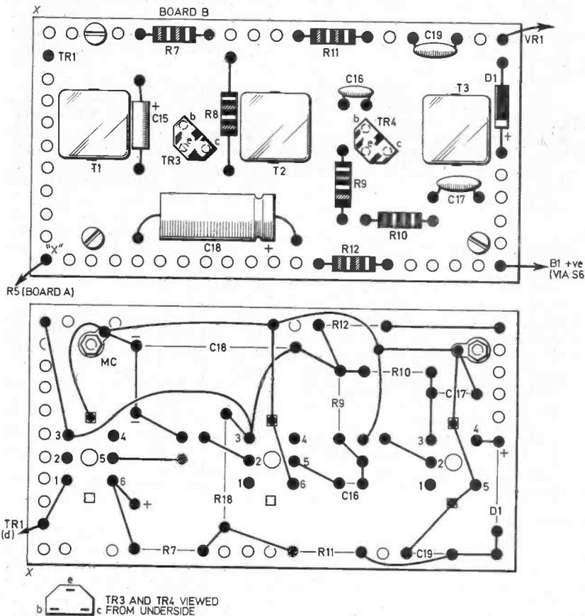
Fig. 4. Layout and wiring of the i.f. amplifier.
