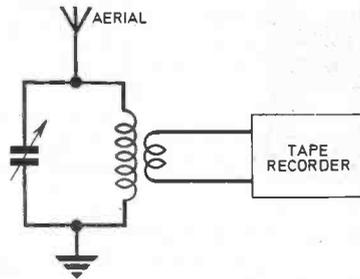
Fig. 2. Tuned circuit arrangement for experimentation.
