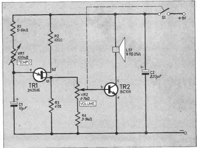
Fig. 2. Complete circuit diagram of the Metronome.
