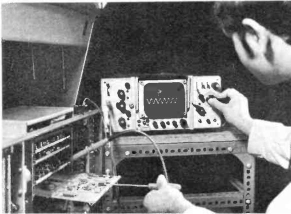
Type 21 marine radar console under test.
