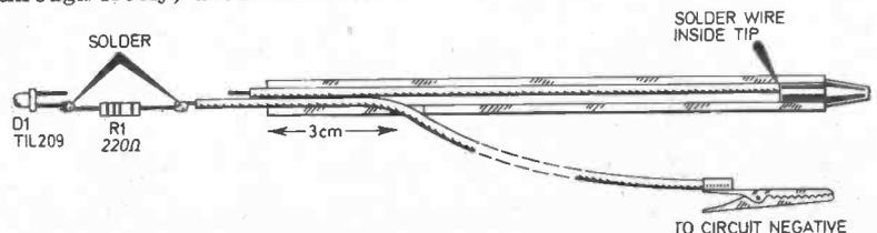
Fig. 8.1. The logic probe just before completion. The wire with the crocodile clip must be pulled to bring the resistor inside the tube and the free end of the l.e.d. must be soldered to the end of the wire.
