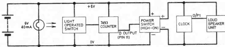
Fig. 8.5. To switch on the alarm after eight laps wire up the system as shown.
