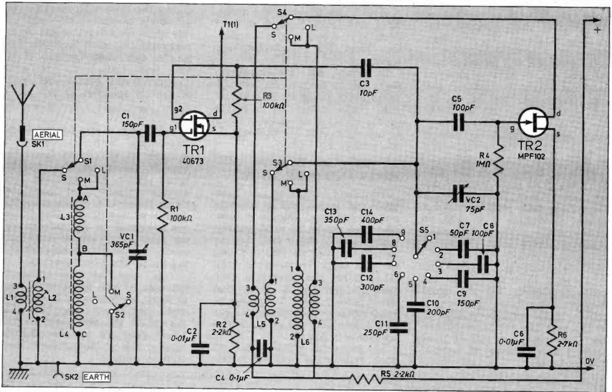
Fig. 1. The mixer and oscillator circuit of the Multi-band Tuner.
