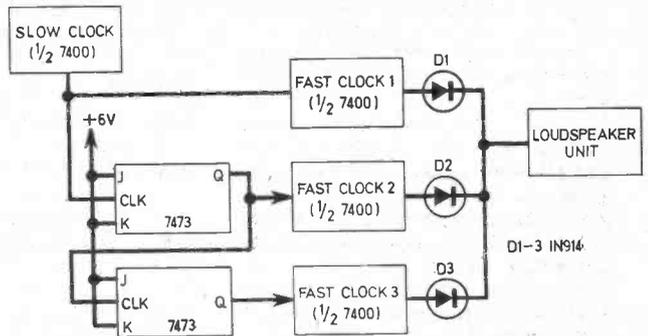
Fig. 8.12. An automatic tone generator. The circuit shown could be used as a door chime.
