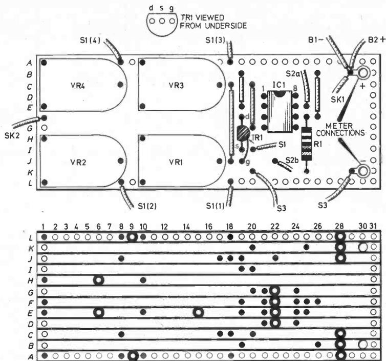
Fig. 3. The layout of the components on the stripboard and the breaks to be made along the tracks on the underside of the board.
