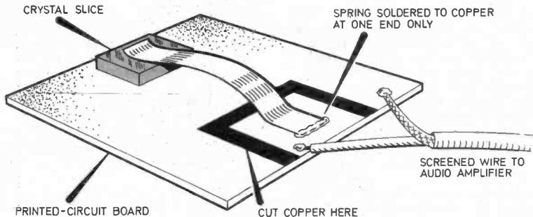
Fig. 1. The simple mounting the Prof. made for the crystal.
