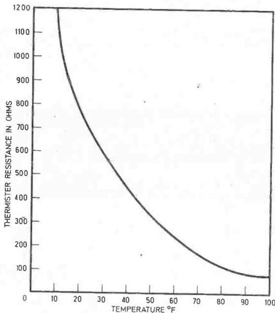
Fig. 1. Graph showing how the resistance of the thermistor varies with temperature.
