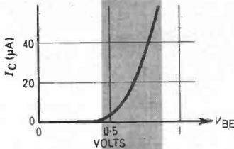
Fig. 1. Graph showing collector current against base/emitter voltage.
