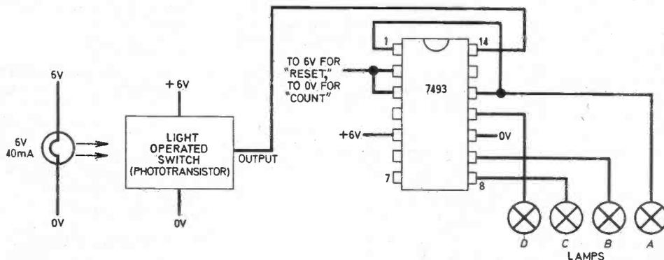
Fig. 8.4. Circuit diagram of the lap counter. The lamp is placed on one side of the track and the light operated switch on the other so that a passing car interrupts the light beam.
