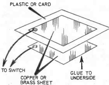
Fig. 8.2a Construction of the battery sandwich. In use the sandwich is placed between two batteries.
