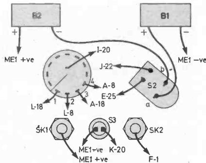
Fig. 4. Wiring up details from panel mounted components to component board locations.
