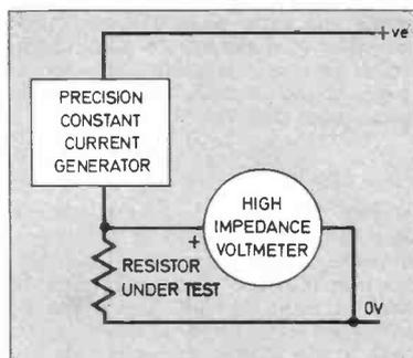
Fig. 1. Method of operation of the Resistance Meter.
