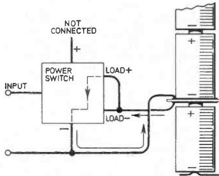
Fig. 8.3. To switch a radio or cassette recorder on and off the battery sandwich is placed between two batteries and connected to a power switch.
