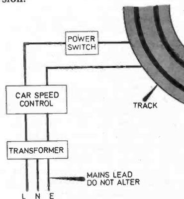
Fig. 8.8. The power switch must be connected between the car speed control and the track. **DO NOT** touch the mains connections.
