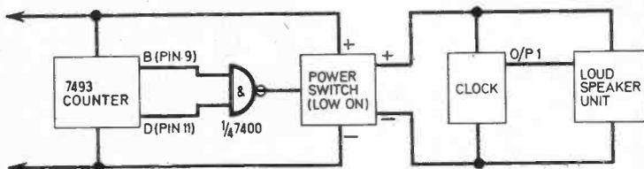
Fig. 8.6. For an alarm after ten laps one gate of a 7400 must be used to detect when the B and D outputs of the counter go high.
