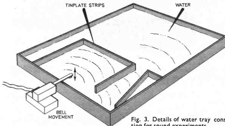
Fig. 3. Details of water tray construction for sound experiments.
