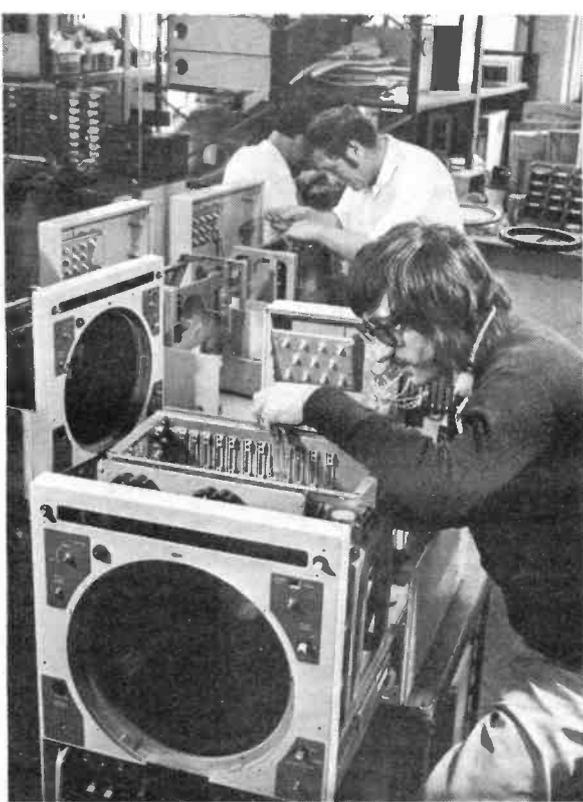
Assembly of Type 1006 navigation radars developed for the Royal Navy.
