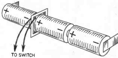
Fig. 8.2b. The battery sandwich of Fig. 8.2a in position.
