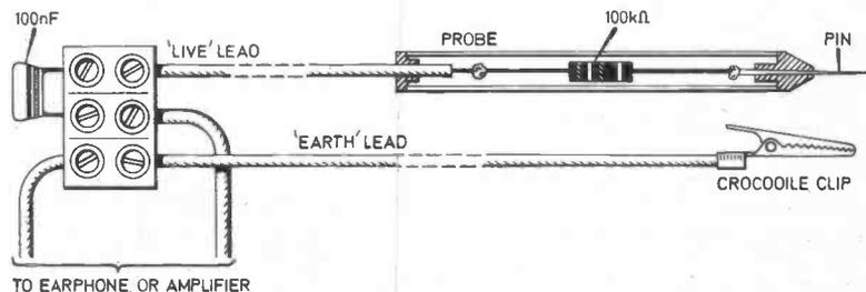
Fig. 1.3. Construction details for a handy test-probe for feeding to an earpiece or amplifier.
