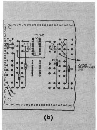
Fig. 8.10. Interrupted tone alarm. The circuit diagram is shown at (a) and the layout on the experimental deck at (b).
