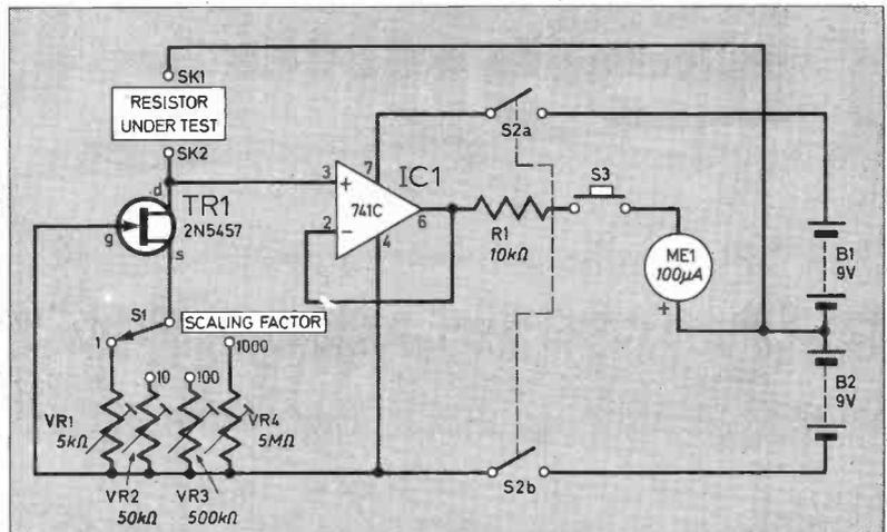
Fig. 2. The complete circuit diagram of the linear scale Resistance Meter.
