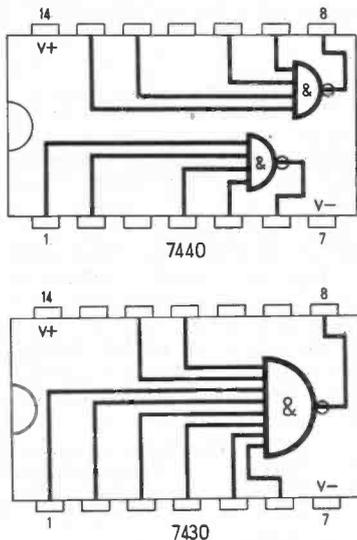
Fig. 8.7. Pin connection details of the 7440 and 7430 integrated circuits.
