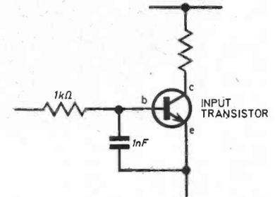
Fig. 3. Low pass filter to reduce unwanted r.f. signals.
