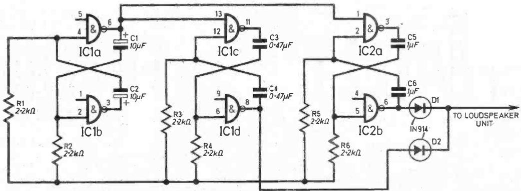
Fig. 8.11. Two-tone alarm. Circuit diagram above and layout on the experimental deck left.
