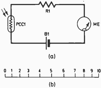
Fig. 2. By adding a series resistor the scale is made more linear.
