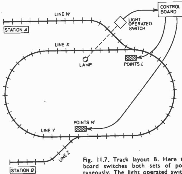
Fig. 11.7. Track layout B. Here the control board switches both sets of points simultaneously. The light operated switch is operated by the train approaching along line *X* or *W*.
