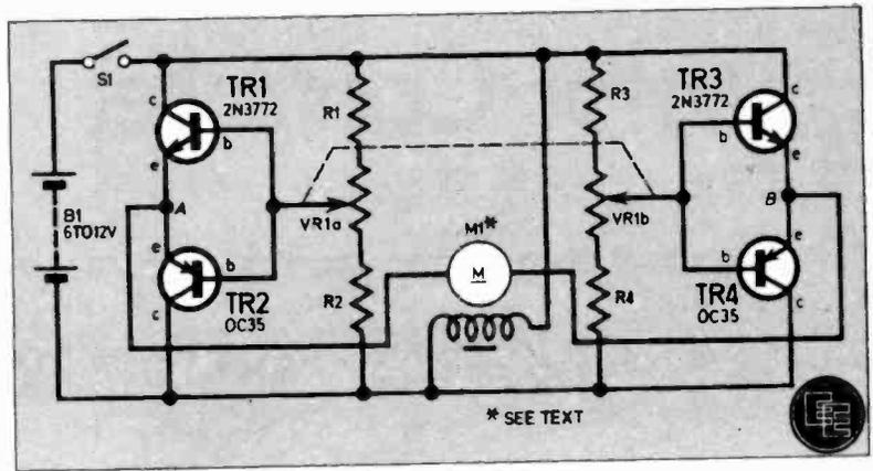
Fig. 1. Complete circuit diagram of the Motor Controller. As mentioned in the text, different types of motors may be used. In this case the field windings (shown as a coil) may be omitted.
