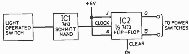
Fig. 11.8. Block diagram showing how the control board in Fig. 11.7. is constructed. The Schmitt is used to "clean up" the output of the light operated switch.
