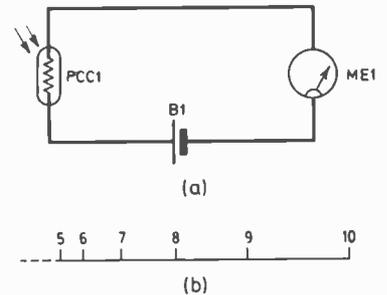
Fig. 1. This arrangement produces an unsatisfactory scale as shown.
