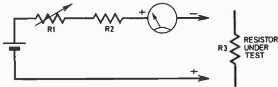
Fig. 4.3. Typical ohmmeter circuit used in many multimeters and VOM's
