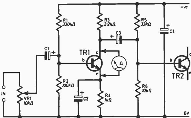
Fig. 4.6. The first stage of a modern amplifier, shown here to illustrate typical fault conditions.
