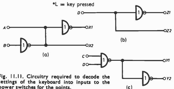
Fig. 11.11. Circuitry required to decode the settings of the keyboard into inputs to the power switches for the points.
