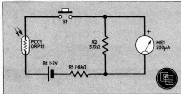
Fig. 3. The complete circuit diagram of the Exposure Unit. Values for  $R_1$  and  $R_2$  have been calculated for the meter listed in component box and  $R_d$  equal to 100 ohms.
