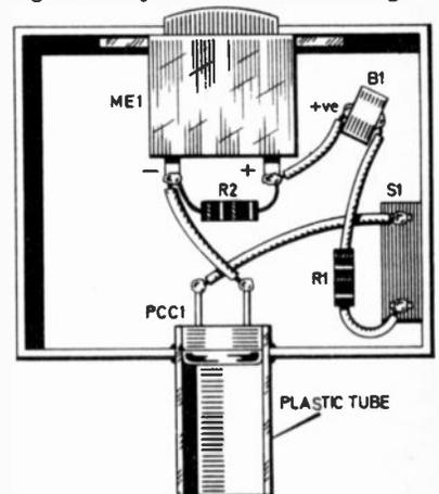
Fig. 4. A suggested layout for the components in a case separate from the camera.
