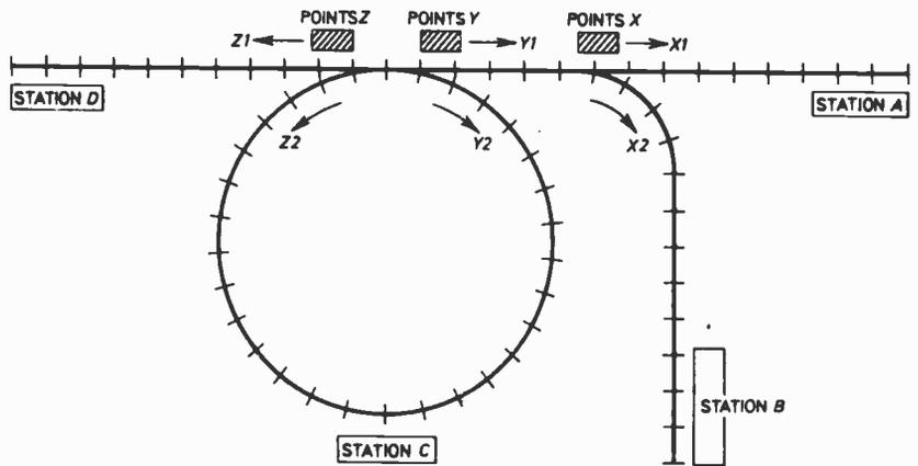
Fig. 11.10. Track layout C. Here the route is selected by the operator before the train is started. Each set of points can take one of two positions as indicated by X1, X2, Y1 etc.
