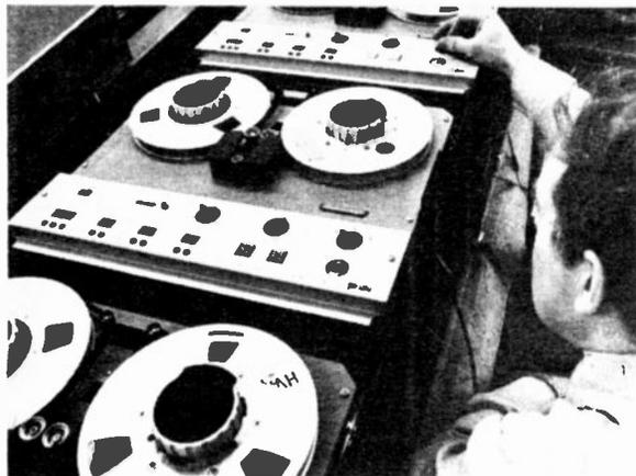
These special quality tape recorders by Racal-Thermionic are merely equipment modules for systems engineers, in this case those specialising in systems or recording and analysis of seismic data.
