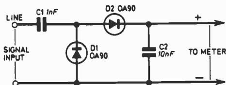
Fig. 4.2. Rectifying probe, which can be used with VOMs to measure r.f. voltages.
