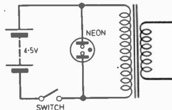
Fig. 4. Even on this side of the coil, the neon flashes when the switch is opened. Nothing happens when it is closed.
