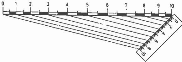
Method of producing a meter scale from the master. Draw a line at any angle to master scale to pass through '10'. Measure length of scale from '10' along angle. Join this point to master '0', then draw lines parallel to this from 1, 2, 3, 4 etc. to meet angle.
