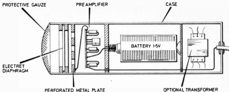
Fig.3. Construction of an electrostatic microphone.
