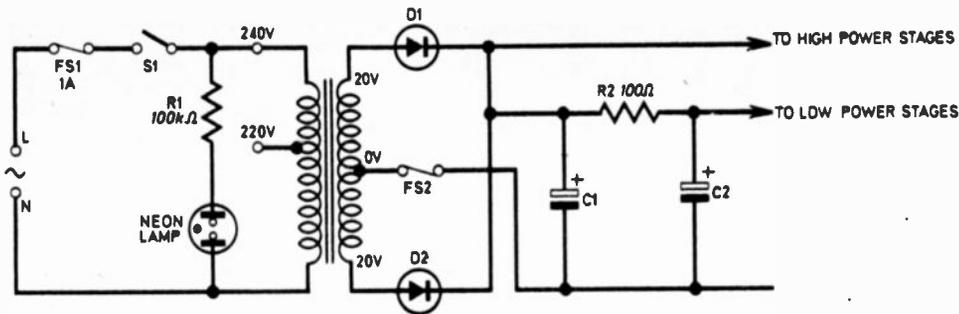
Fig. 4.1. A typical mains supply unit, using full wave rectification.
