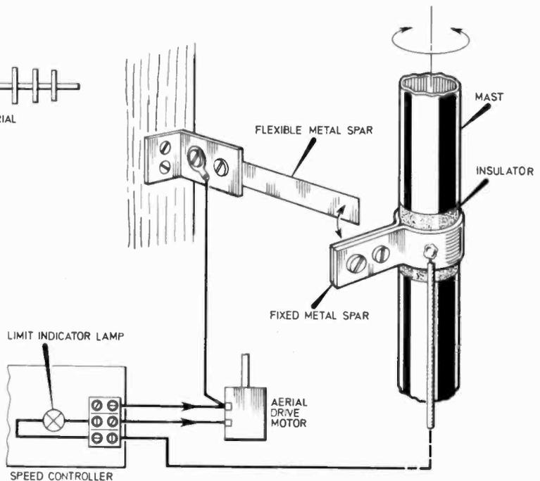
Fig. 5. Typical method of mounting the aerial mast. The two metal spars make contact when the aerial is pointing north.
