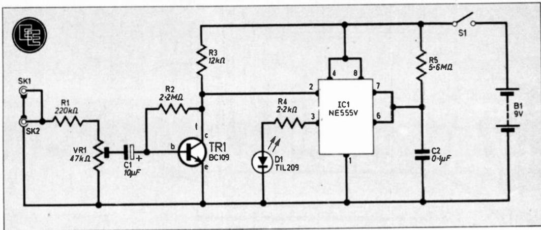
Fig. 1. Circuit diagram of the Audio Peak Level Indicator.
