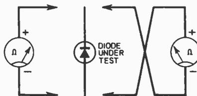
Fig. 4.4. Testing a semiconductor diode
