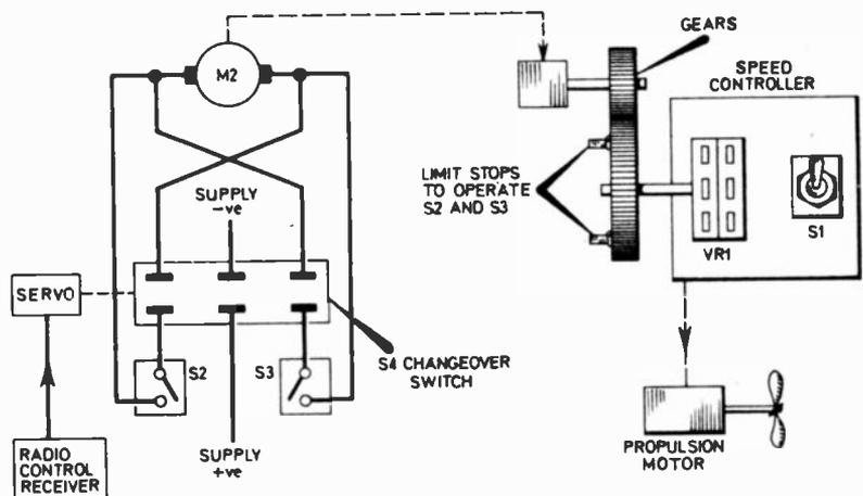
Fig. 6. Model boat system. The changeover switch S4 is a type which has a centre off position. The servo is normally available from a model shop. Make sure when purchasing, that an operating bar is also bought.
