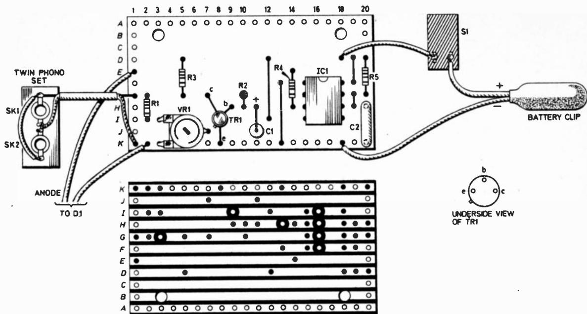
Fig. 2. Stripboard layout, also showing the breaks required on the underside.
