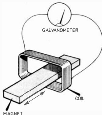
Fig. 1. When the magnet is moved to and fro a current flows and registers on the meter. No movement—no current.
