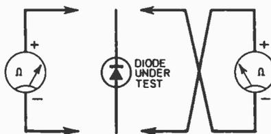
Fig. 4.4. Testing a semiconductor diode
