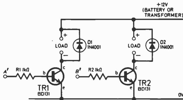
Fig. 11.4. Circuit of the power switches suitable for operating points. The diodes are necessary to protect the transistors from the high voltages produced by the point coils as current is switched off.
