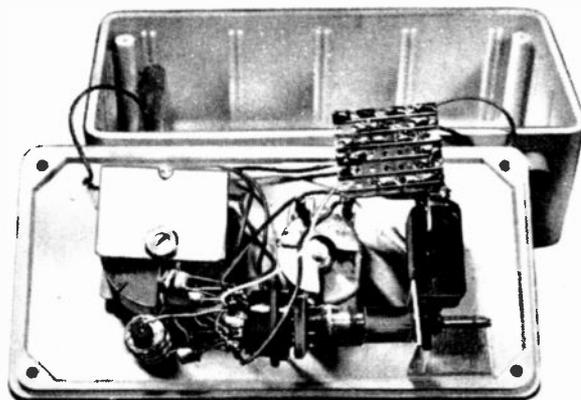
Internal photograph showing the positions taken up by the coil and circuit board.
