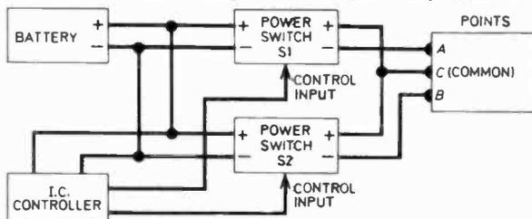
Fig. 11.1. Block diagram showing how a system using power switches can be constructed to operate a pair of electrically operated points.
