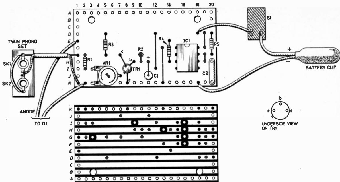
Fig. 2. Stripboard layout, also showing the breaks required on the underside.
