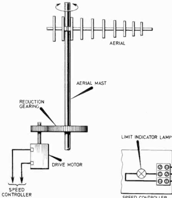
Fig. 4. Suggested arrangement for rotating a t.v. aerial.
