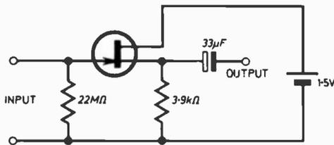
Fig.4. Typical circuit used in many electrostatic microphones.
