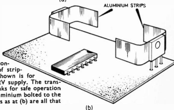
Fig. 11.3. Construction of the points controller on a piece of stripboard. The wiring shown is for points requiring a 12V supply. The transistors require heatsinks for safe operation and small strips of aluminium bolted to the transistors metal faces as at (b) are all that is necessary.
