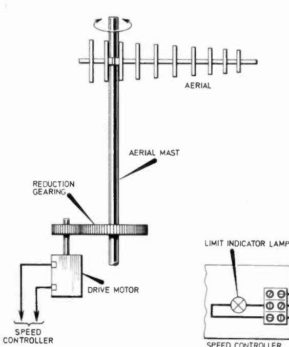
Fig. 4. Suggested arrangement for rotating a t.v. aerial.
