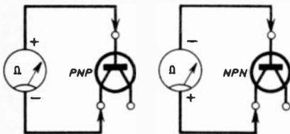
Fig. 4.5. Checking one of the two junctions in a transistor.
