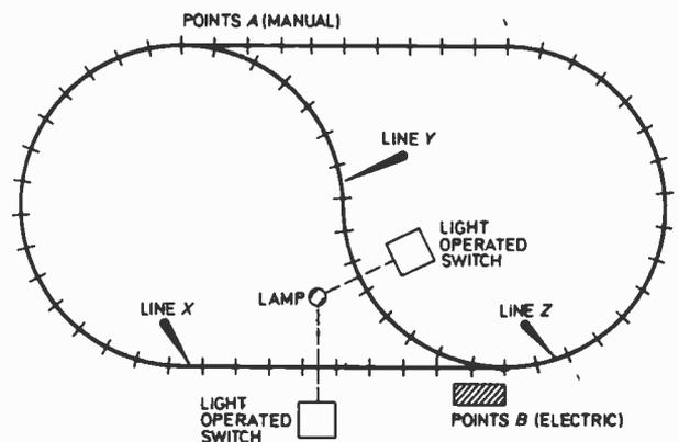
Fig. 11.6. Track layout A. Points A are manually operated and are placed near to the operator.
