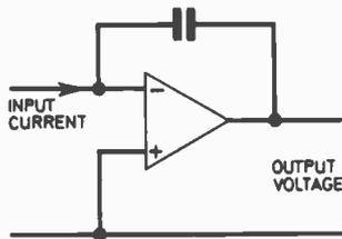
Fig. 1. Fundamental circuit for an integrating op. amp.
