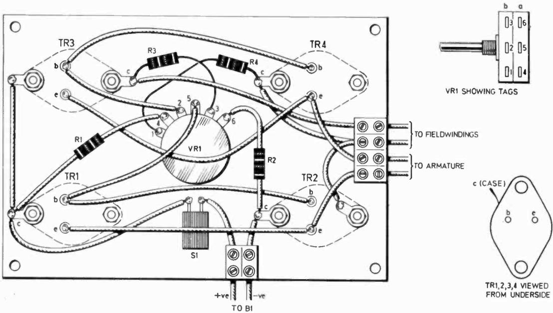
Fig. 2. Wiring diagram for the Motor Controller. This is mounted on a sheet of aluminium, which also acts as the heatsink
