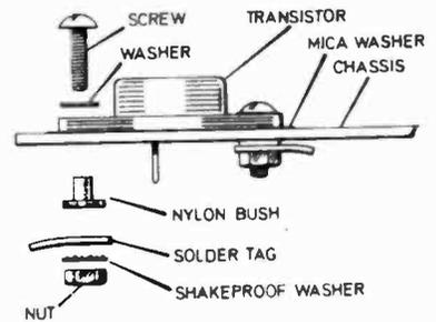
Fig. 3. Mounting details for the four transistors.
