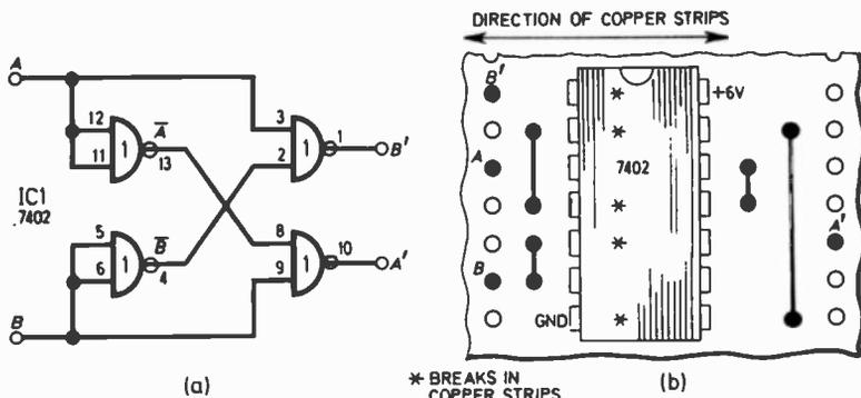
Fig. 11.2. The circuit for the i.c. controller of the points circuit in Fig. 11.1. is shown at (a) and the wiring of the 7402 i.c. at (b).
