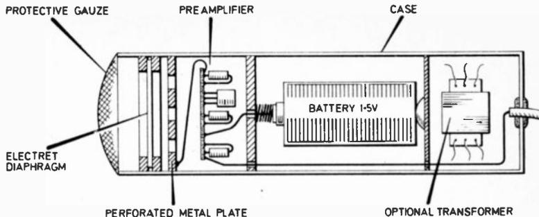
Fig.3. Construction of an electrostatic microphone.
