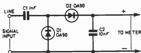
Fig. 4.2. Rectifying probe, which can be used with VOMs to measure r.f. voltages.
