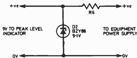
Fig. 3. This circuit is only required if the equipment supply is more than 9V.
