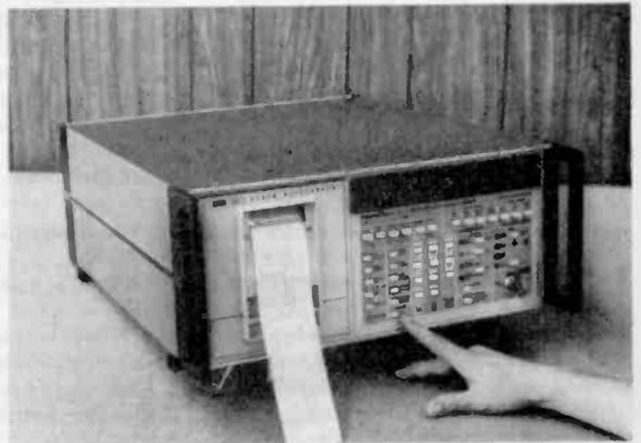
A programmable data logger by Fluke. This is the sort of instrument that might be specified by a systems engineer or an industrial automation system. It can scan and record up to 60 different inputs in the form shown, up to 1,000 inputs with ancillary equipment.
