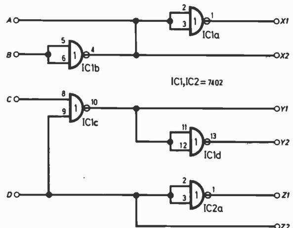
Fig. 11.12. The complete circuit of the controller for Fig. 11.10 using two 7402 i.c.s. All the outputs must go to pulse generators (six off) and then to power switches.
