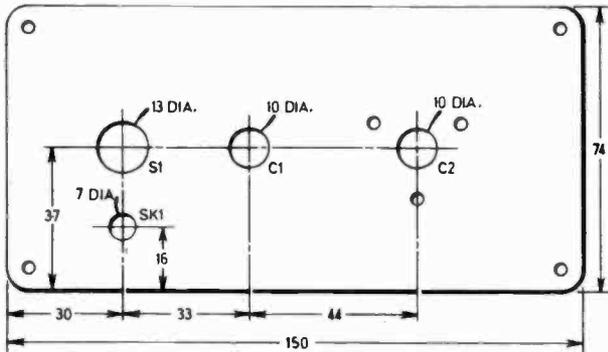
Fig. 2. The drilling details for the front panel. It is recommended that the dimensions be strictly adhered to.
