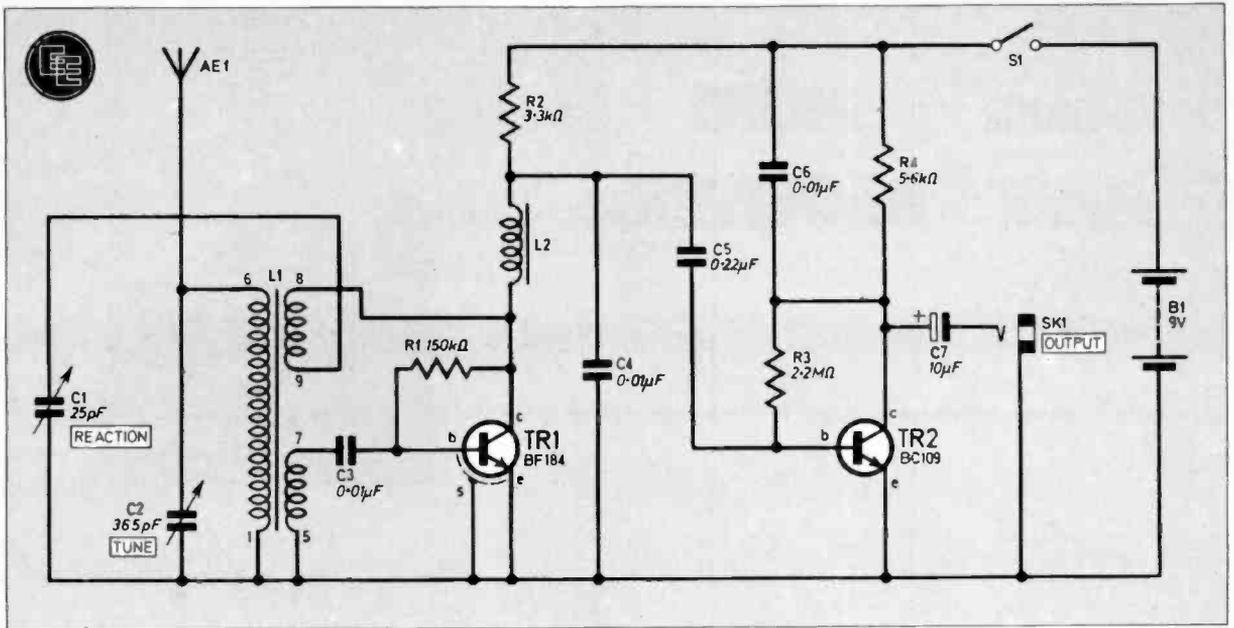
Fig. 1. Complete circuit diagram of the Portable Short Wave Receiver
