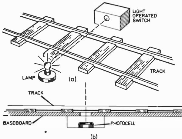
Fig. 11.5. Two methods of using photocells to detect the presence of the train. In (a) the light operated switch is mounted on one side of the tracks and the lamp on the other; (b) is more elegant with the photocell mounted under the baseboard, light entering through a small hole drilled in it.
