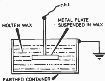
Fig.2. Apparatus required to produce a "wax" electret.
