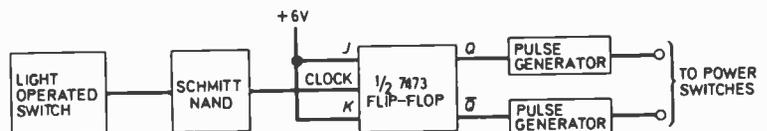
Fig. 11.9. The addition of two pulse generators ensures that the points are not supplied with power continuously.
