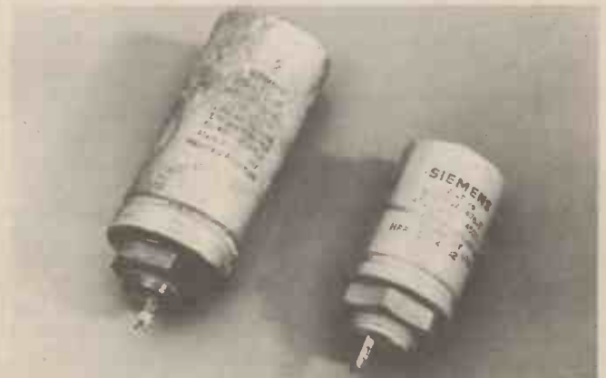
How components shrink. The Siemens electrolytic capacitor on the left was found to be still working after 15 years submerged in Lake Constance. In the meantime, capacitors have become smaller. The modern version on the right is only half the volume but has the same capacity and working voltage.
