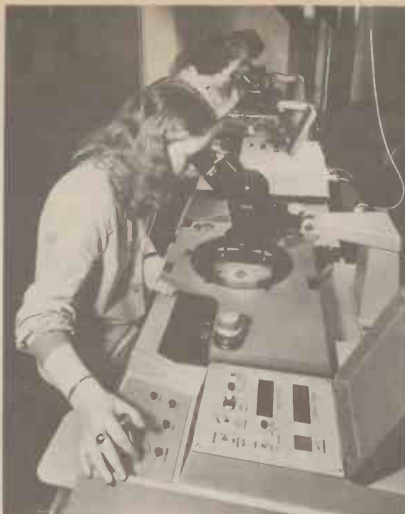
Automatic wafer-probing at Motorola's MOS integrated circuit plant in Scotland. Apart from their own sales engineers based on Wembley, Motorola products reach the UK market through six distributors.
