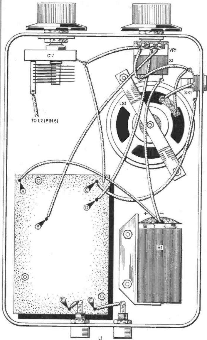
Fig. 3. The layout of the components and board within the case and complete wiring up details.
