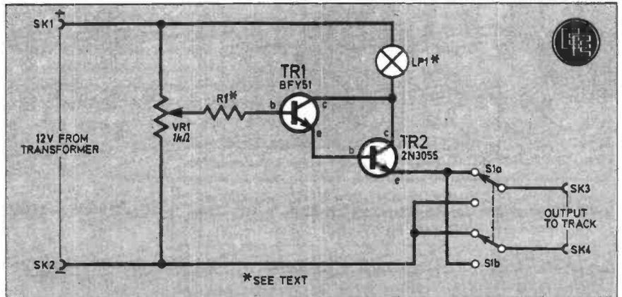
Fig. 2. The complete circuit diagram of the Train Controller.
