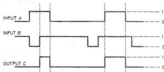
Fig. 3. The output is high only when both inputs are high.
