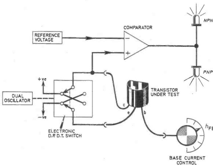
Two oscillators in anti-phase produce in effect a double-pole double-throw electronic switch that supplies positive and negative supply lines to the transistor under test. The polarity of the supply lines alternates at a rate of about 3 hertz.
