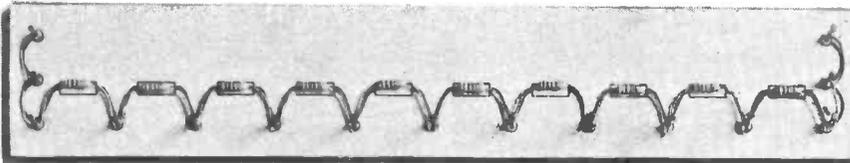
Fig 1.1. The resistor chain as used in this series. Shown here is the method of construction, and is represented by either of the two circuit symbols shown below.
