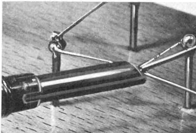
Soldering a piece of wire to a nail. Note carefully how the iron and solder are applied.
