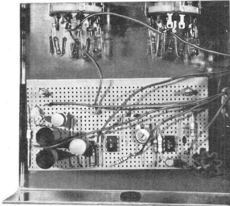
Detailed photograph showing the stripboard and in particular the method of wiring S4 and S5.
