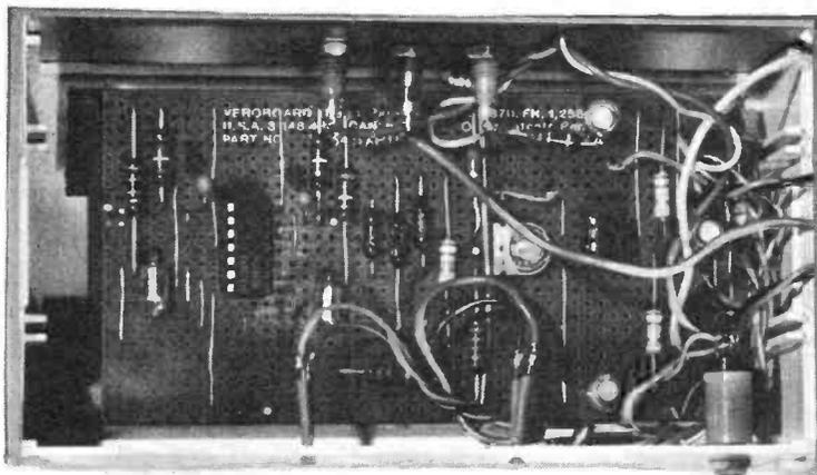
General view of the completed Transistor Tester.
