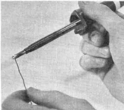
Tinning the bit of a soldering iron.
