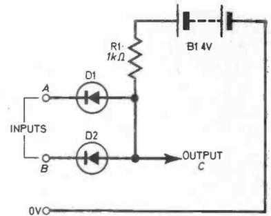
Fig. 2. Experimental AND gate.
