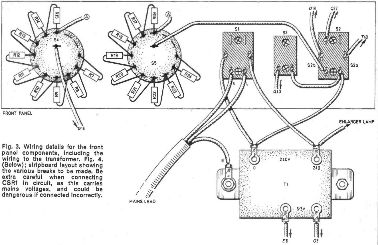
Fig. 3. Wiring details for the front panel components, including the wiring to the transformer. Fig. 4. (Below); stripboard layout showing the various breaks to be made. Be extra careful when connecting CSR1 in circuit, as this carries mains voltages, and could be dangerous if connected incorrectly.
