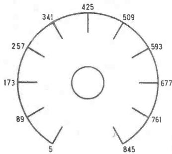
Fig. 4. Scale of  $h_{FE}$  used on the prototype unit. This is reproduced full size and may be traced.
