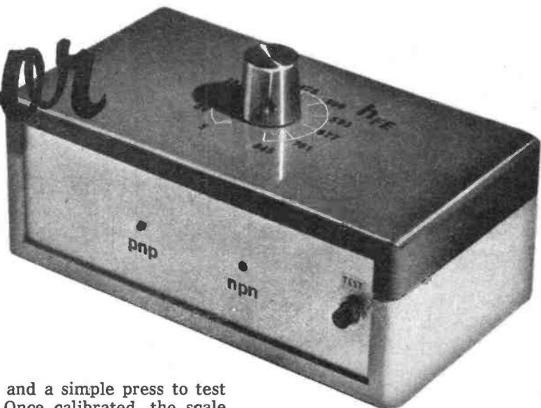
The method of connection to the transistor under test may be a matter of personal choice. The prototype uses flexible leads into banana sockets but there is no reason why a cluster of suitable transistors sockets cannot be used—there is plenty of room for them.
